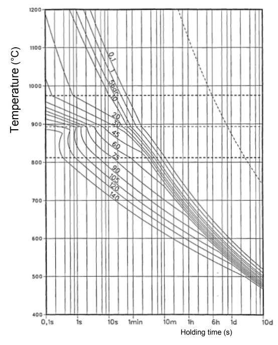
Bursting criterion for constant temperature Maximum expansion 10%
