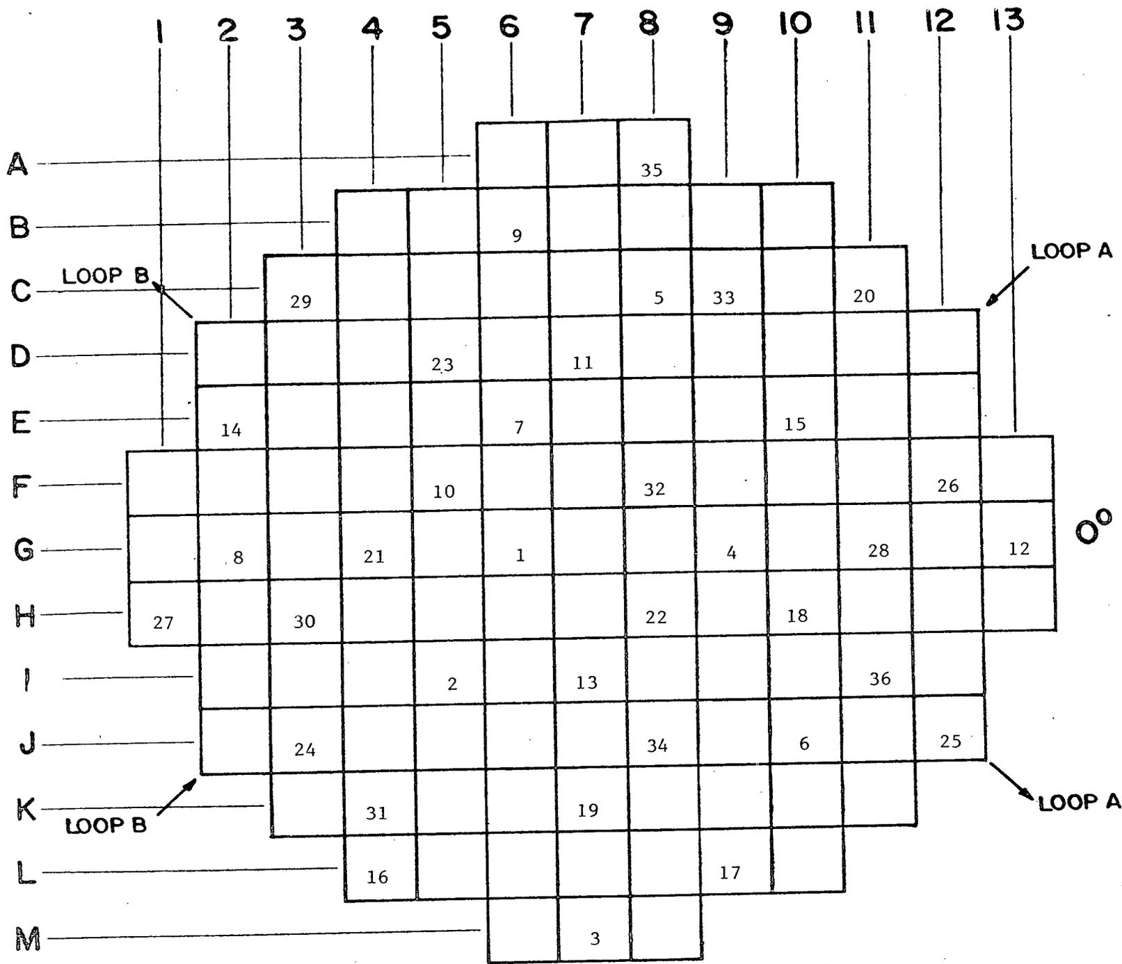
FIGURE 2.6-1 Location and I.D. Number of Moveable In-Core Fission Chambers
