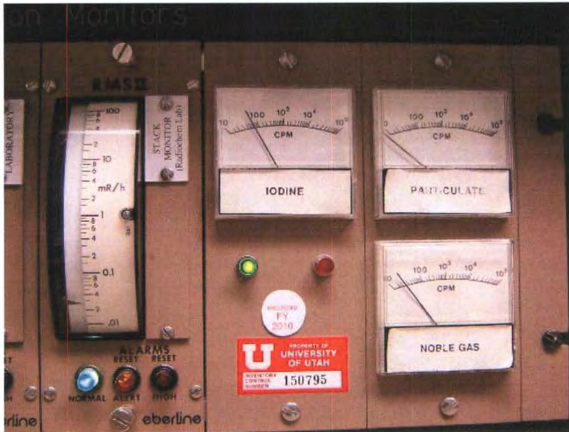
Figure 5.6-2 CAM monitor for iodine, noble gas and particulates
