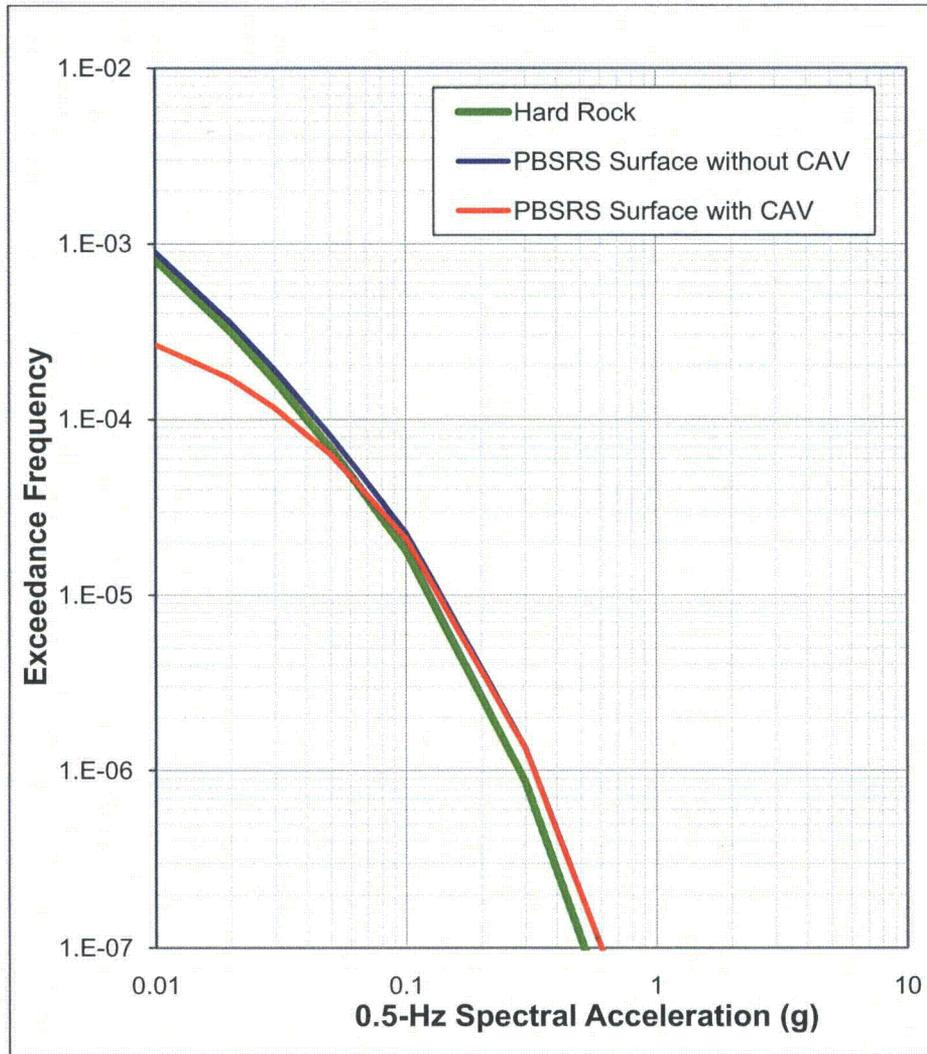
**Figure 3.7.1-214: Surface Hazard Curves at Finished Ground Level Grade for the Full Soil Column Profile Computed With and Without CAV for 0.5 Hz Spectral Acceleration.**
