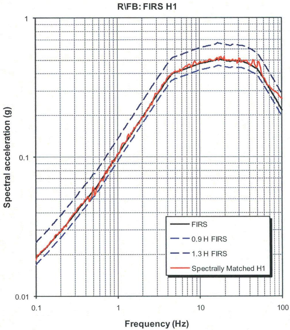
**Figure 3.7.1-234:** Response Spectrum for Spectrally Matched Horizontal (H1) Component for the Fermi 3 RB/FB SSI FIRS.
