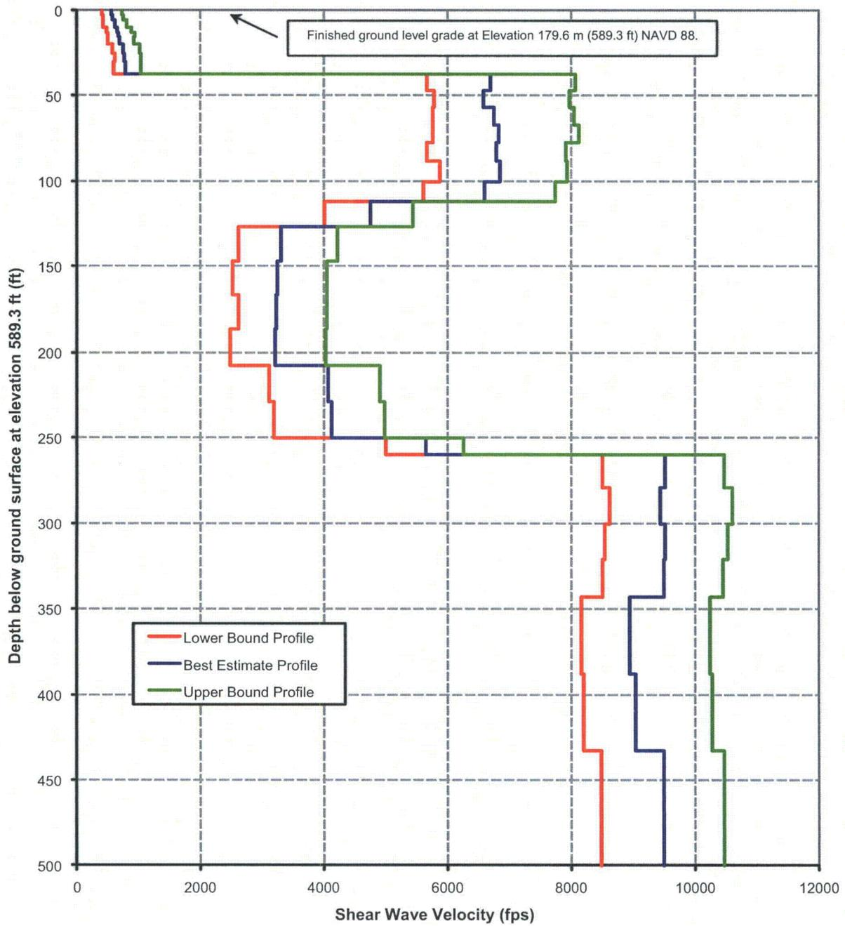
**Figure 3.7.1-225: Lower Bound, Best Estimate and Upper Bound Shear Wave Velocity Profiles for the Full Soil Column.**
