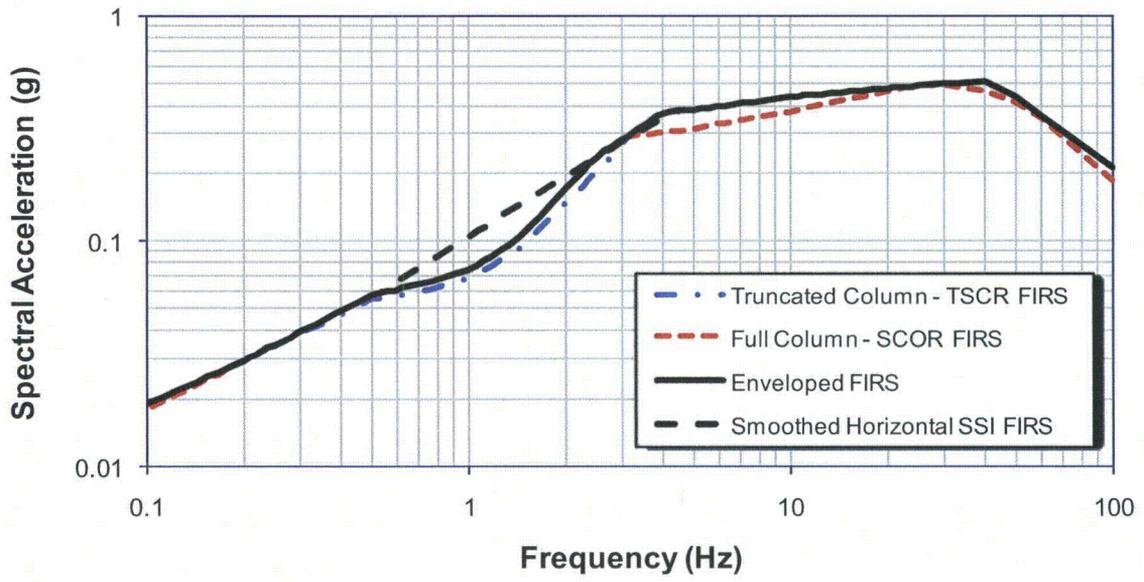
Figure 3.7.1-229: Development of Horizontal Fermi 3 SSI FRS for the CB.
