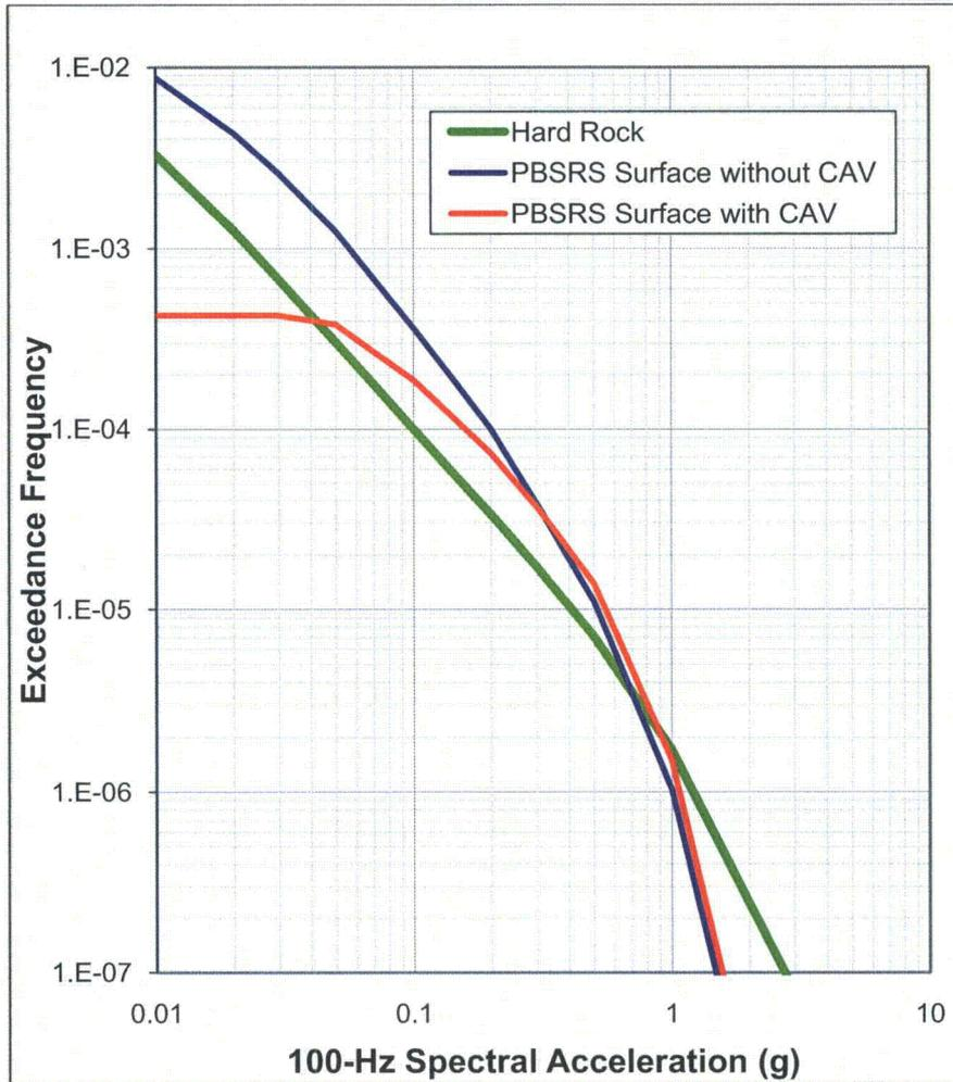
**Figure 3.7.1-220: Surface Hazard Curves at Finished Ground Level Grade for the Full Soil Column Profile Computed With and Without CAV for 100 Hz Spectral Acceleration.**
