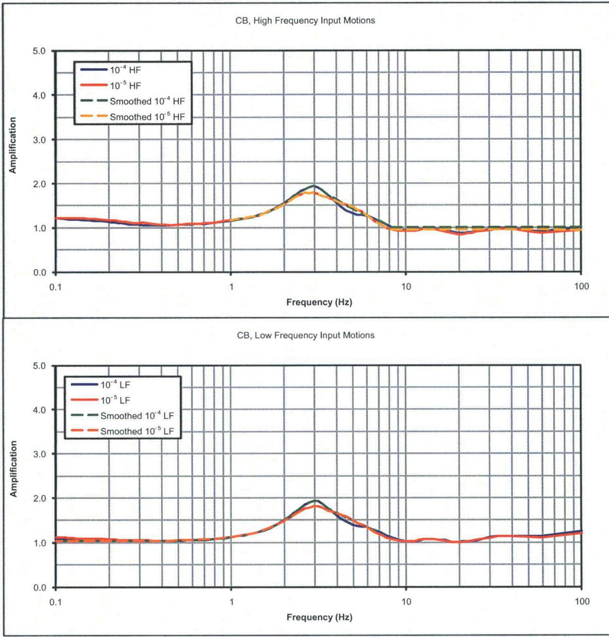
Figure 3.7.1-211: CB SCOR Amplification Functions for the Fermi 3 Site.
