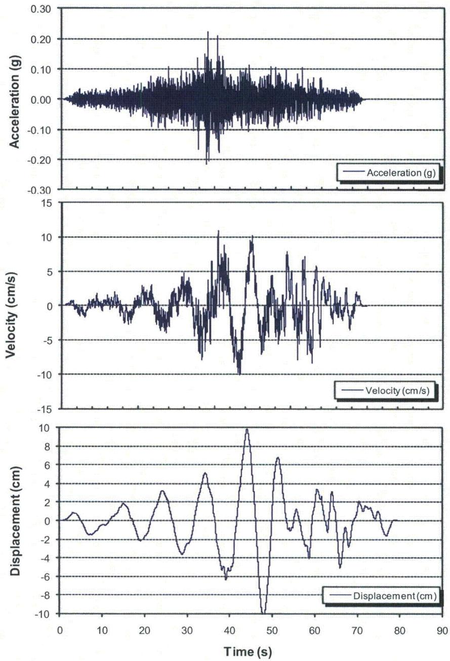
**Figure 3.7.1-243: Acceleration, Velocity, and Displacement Time Histories for the SSI FIRS Horizontal (H1) Component Compatible with the CB Horizontal SSI FIRS.**
