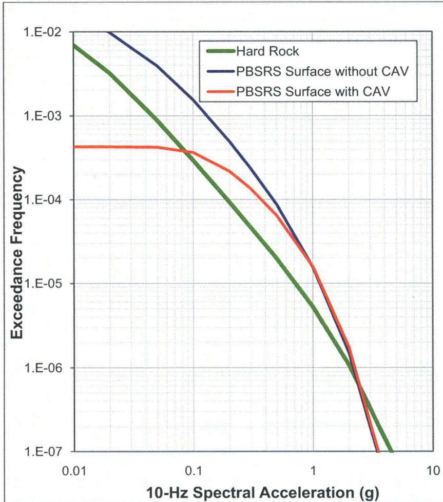
**Figure 3.7.1-218: Surface Hazard Curves at Finished Ground Level Grade for the Full Soil Column Profile Computed With and Without CAV for 10 Hz Spectral Acceleration.**
