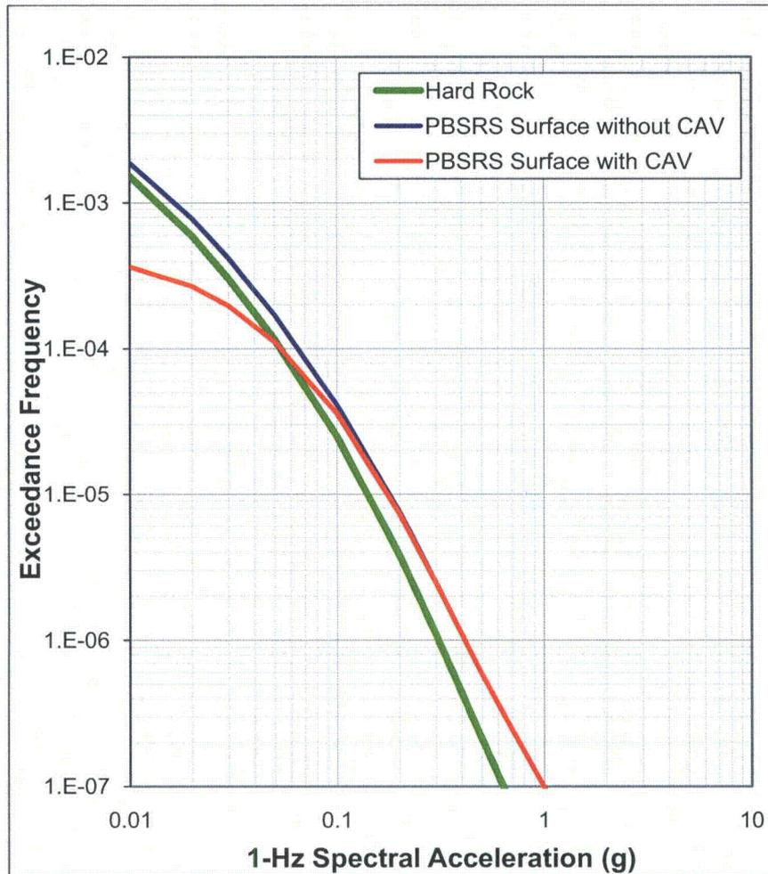
**Figure 3.7.1-215: Surface Hazard Curves at Finished Ground Level Grade for the Full Soil Column Profile Computed With and Without CAV for 1 Hz Spectral Acceleration.**
