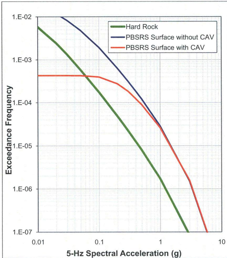
**Figure 3.7.1-217: Surface Hazard Curves at Finished Ground Level Grade for the Full Soil Column Profile Computed With and Without CAV for 5 Hz Spectral Acceleration.**
