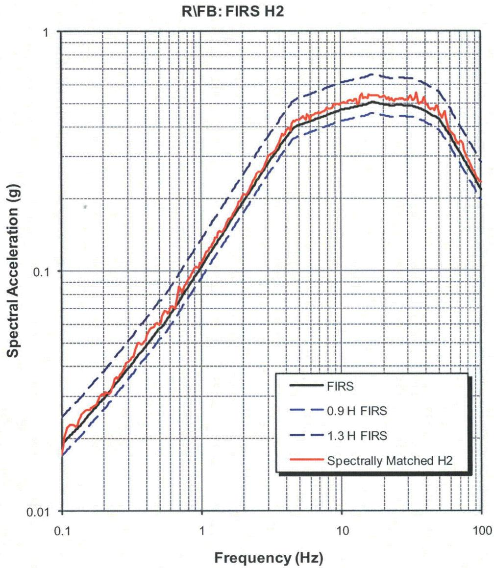
**Figure 3.7.1-235:** Response Spectrum for Spectrally Matched Horizontal (H2) Component for the Fermi 3 RB/FB SSI FIRS.
