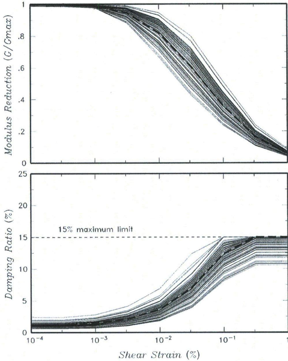
**Figure 3.7.1-207: Randomized Shear Modulus Reduction and Damping Relationships Used for 20 to 50 Feet Depth Engineered Granular Backfill Material.**
