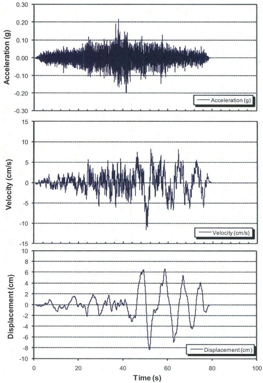
**Figure 3.7.1-245: Acceleration, Velocity, and Displacement Time Histories for the SSI FIRS Vertical (V) Component Compatible with the CB Vertical SSI FIRS.**
