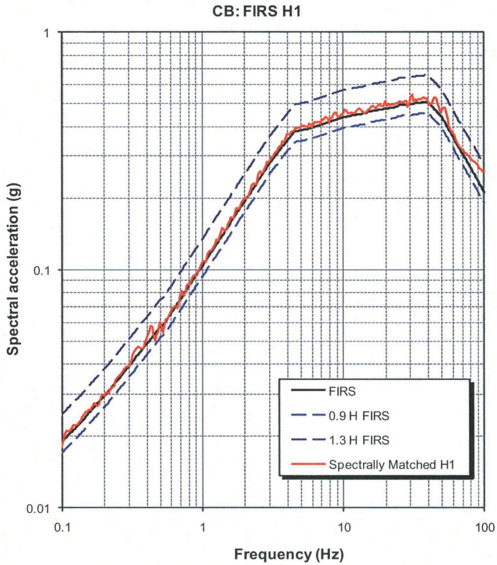
**Figure 3.7.1-237:** Response Spectrum for Spectrally Matched Horizontal (H1) Component for the Fermi 3 CB SSI FIRS.
