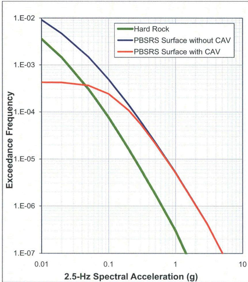
**Figure 3.7.1-216:** Surface Hazard Curves at Finished Ground Level Grade for the Full Soil Column Profile Computed With and Without CAV for 2.5 Hz Spectral Acceleration.
