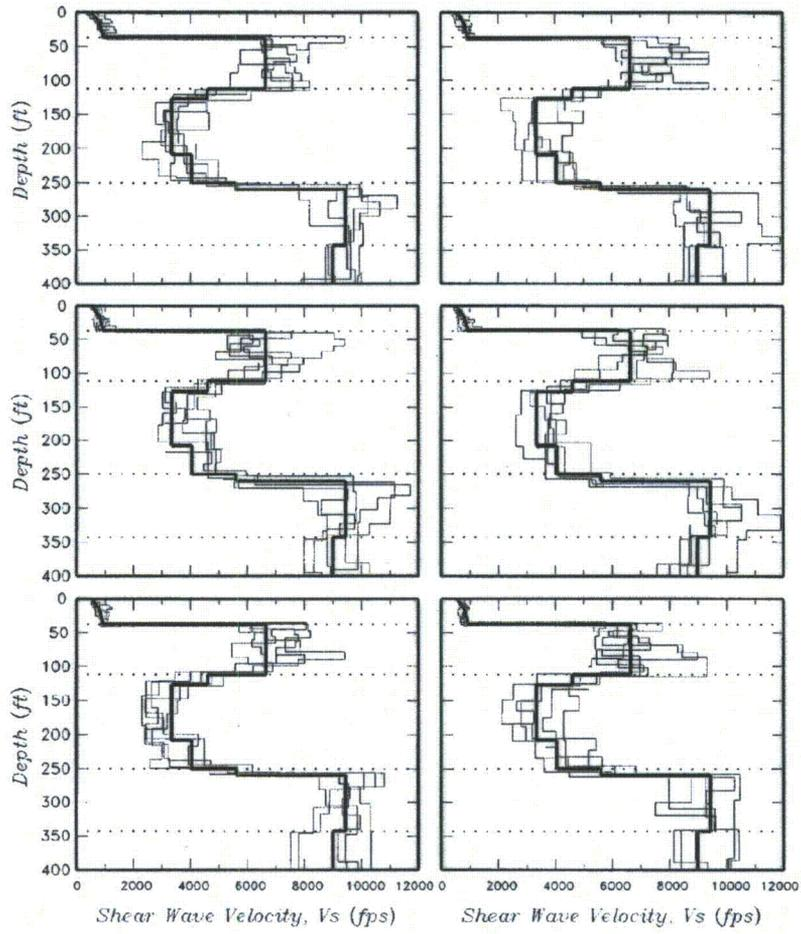
**Figure 3.7.1-203: Randomized Shear Wave Velocity Profiles 1-30 for the Intermediate Range Site Response Analysis Profile.**
