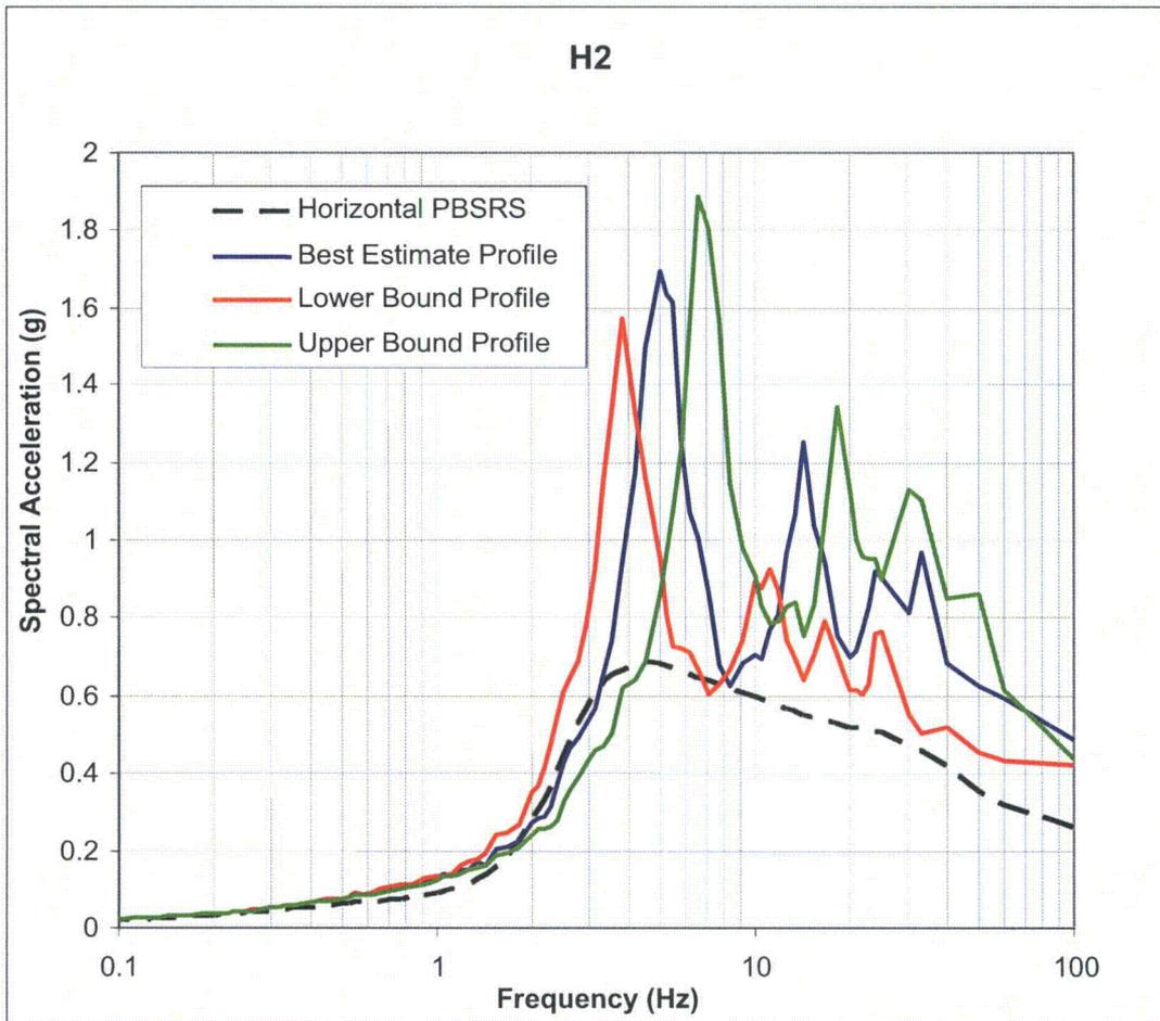
**Figure 3.7.1-247:** Comparison of Response Spectra of Computed Horizontal (H2) Component Surface Motions for SSI Profiles Using the RB/FB SCOR FIRS Input Motion to the Horizontal PBSRS.
