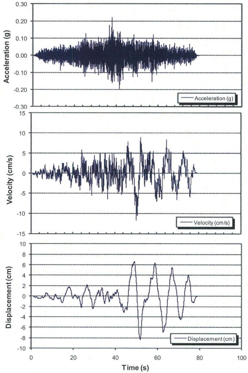
**Figure 3.7.1-242: Acceleration, Velocity, and Displacement Time Histories for the SSI FIRS Vertical (V) Component Compatible with the RB/FB Vertical SSI FIRS.**
