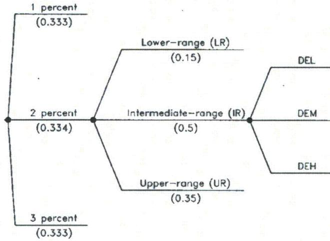
**Figure 3.7.1-208: Site Response Logic Tree for Full Soil Column Profile.**
