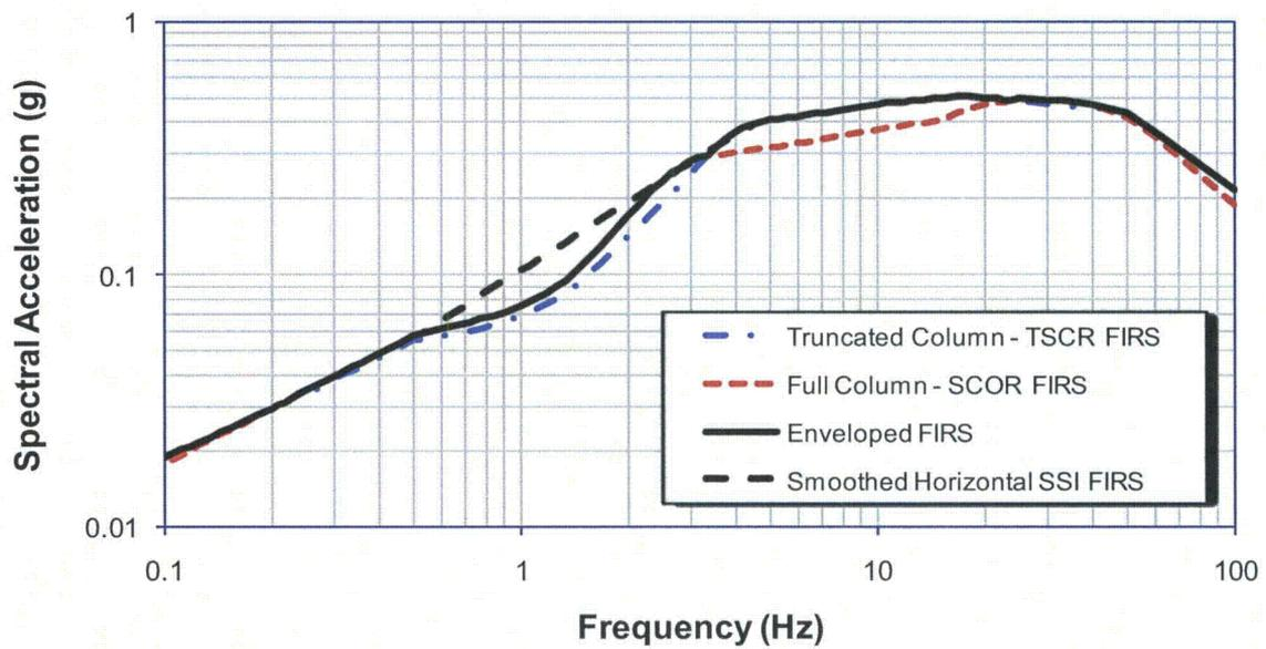
Figure 3.7.1-228: Development of Horizontal Fermi 3 SSI FIRS for the RB/FB.
