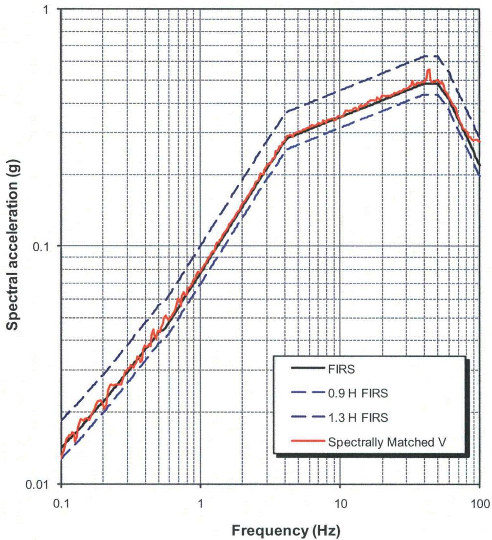
Figure 3.7.1-236: Response Spectrum for Spectrally Matched Vertical (V) Component for the Fermi 3 RB/FB SSI FIRS.
