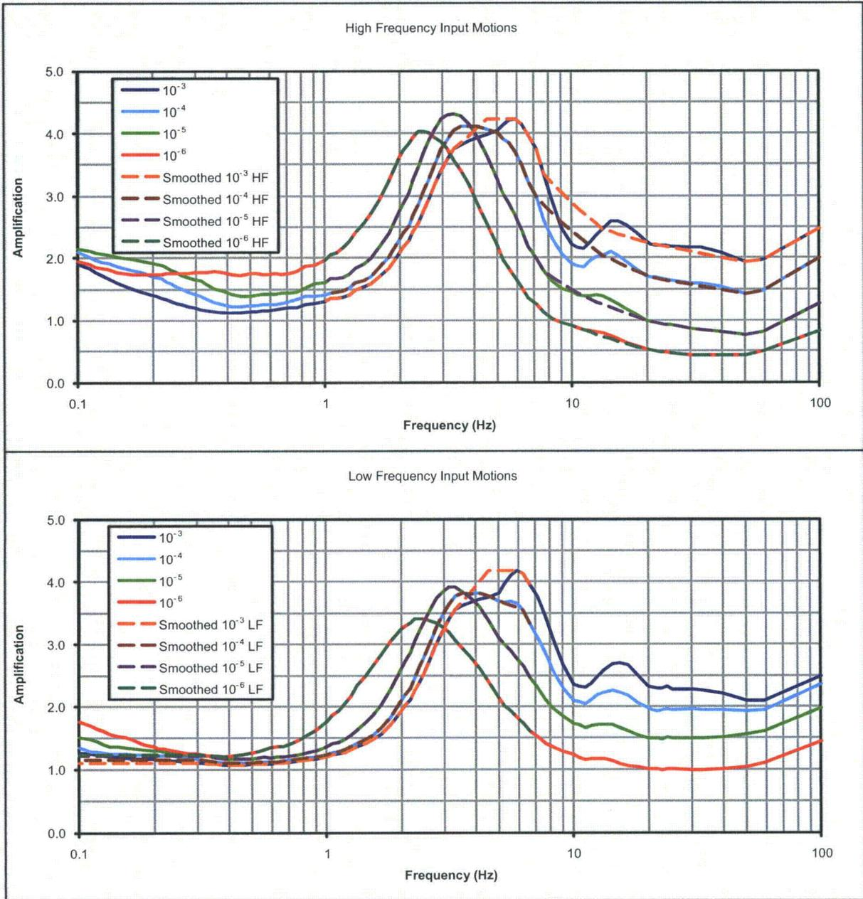
Figure 3.7.1-209: PBSRS Amplification Functions for the Fermi 3 Site.
