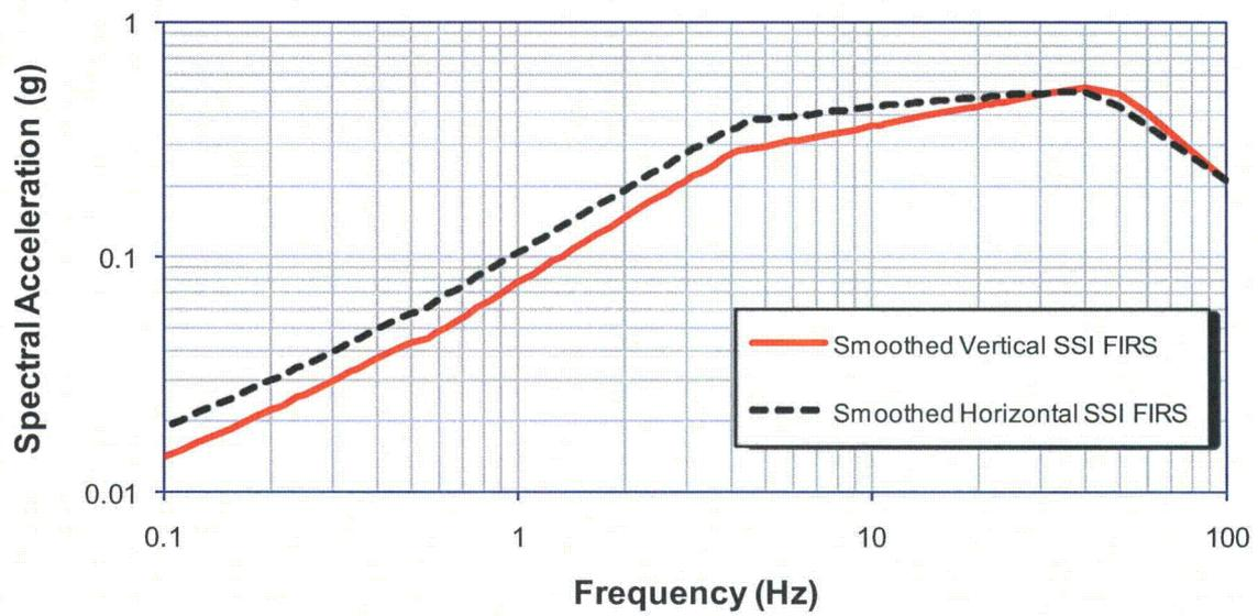
**Figure 3.7.1-233: Horizontal and Vertical Fermi 3 SSI FIRS for the CB.**
