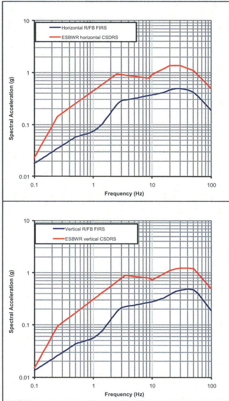
Figure 3.7.1-226: Fermi 3 RB/FB SCOR FIRS (5% Damping).
