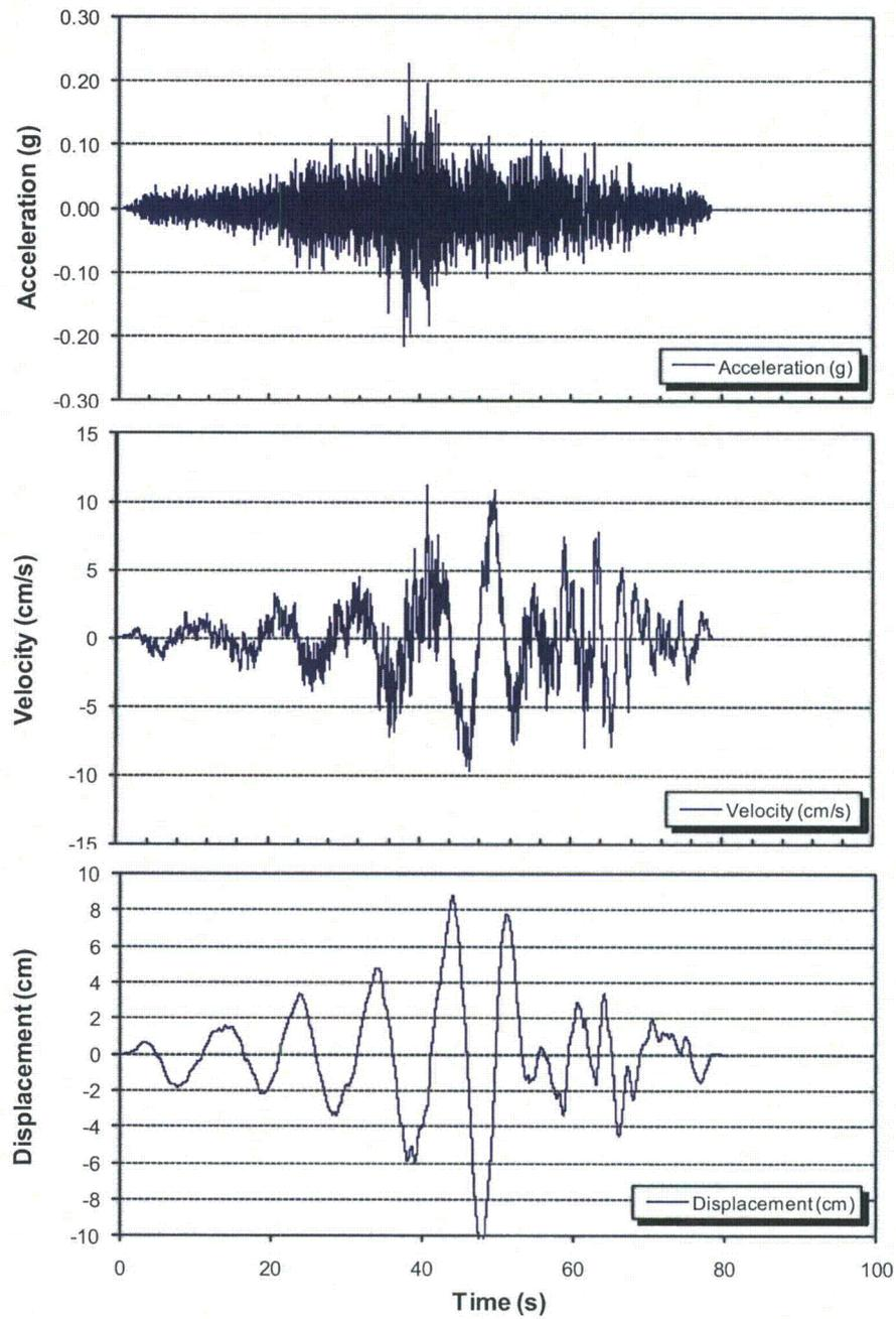
**Figure 3.7.1-240: Acceleration, Velocity, and Displacement Time Histories for the SSI FIRS Horizontal (H1) Component Compatible with the RB/FB Horizontal SSI FIRS.**
