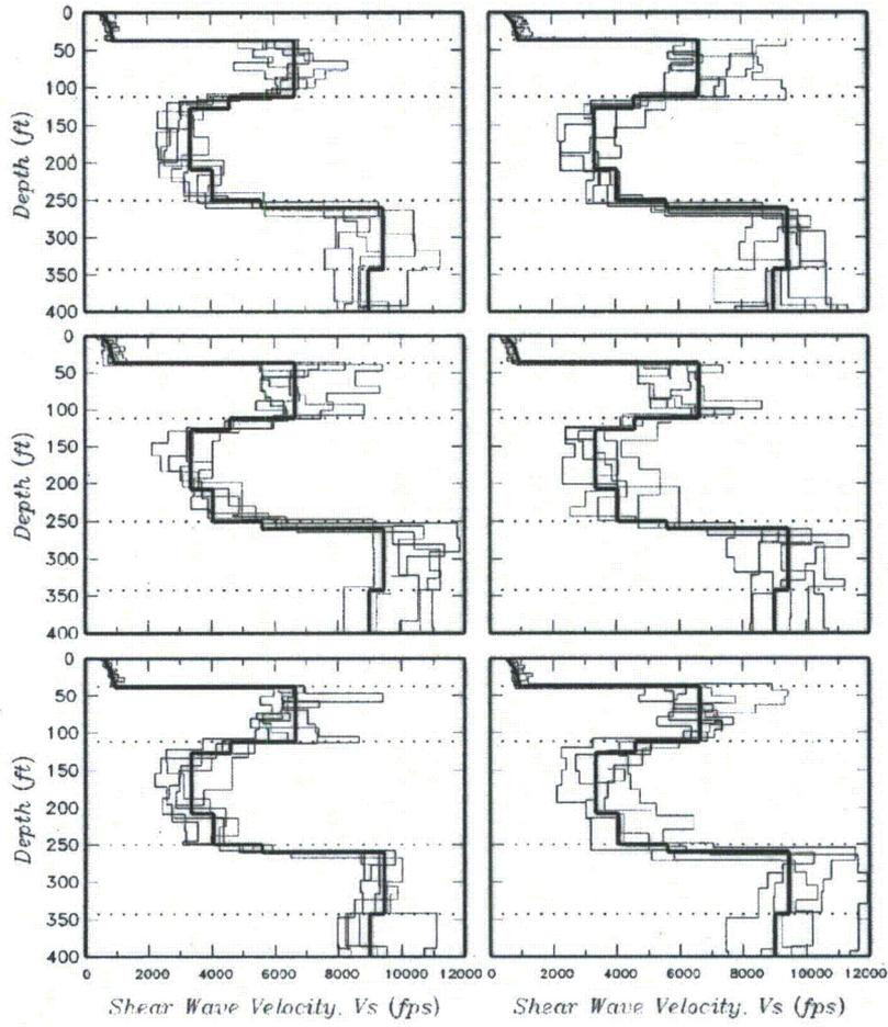
**Figure 3.7.1-204: Randomized Shear Wave Velocity Profiles 31-60 for the Intermediate Range Site Response Analysis Profile.**
