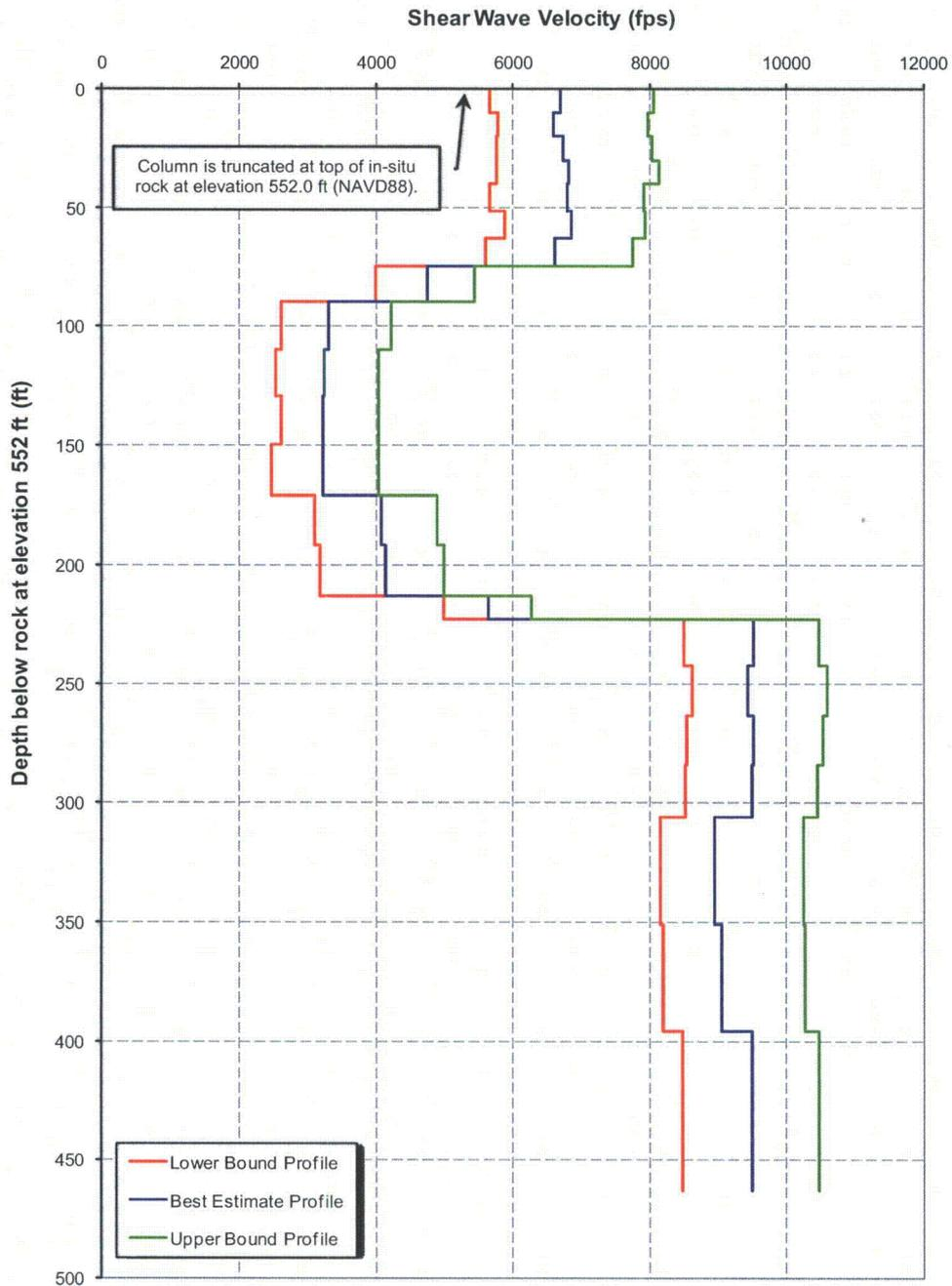
**Figure 3.7.1-252: Lower Bound, Best Estimate and Upper Bound Shear Wave Velocity Profiles for the Fermi 3 Site-Specific SSI Analyses.**
