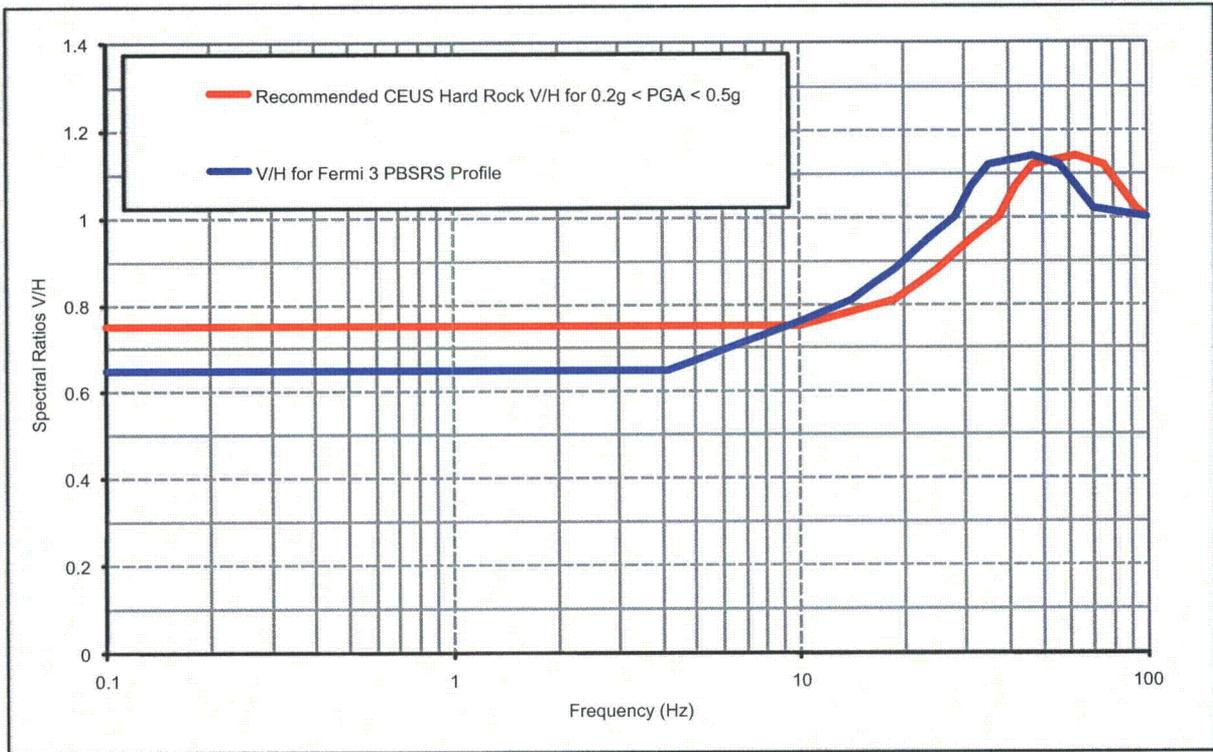
**Figure 3.7.1-223: Vertical to Horizontal Spectral Ratios Developed for Fermi 3 Full Soil Column Profile.**
