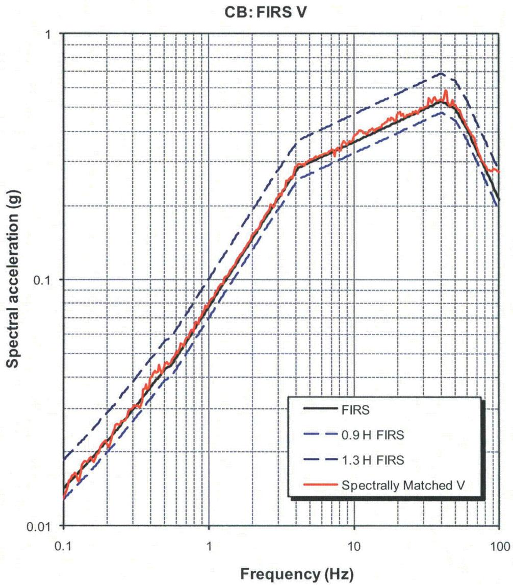
**Figure 3.7.1-239: Response Spectrum for Spectrally Matched Vertical (V) Component for the Fermi 3 CB SSI FIRS.**
