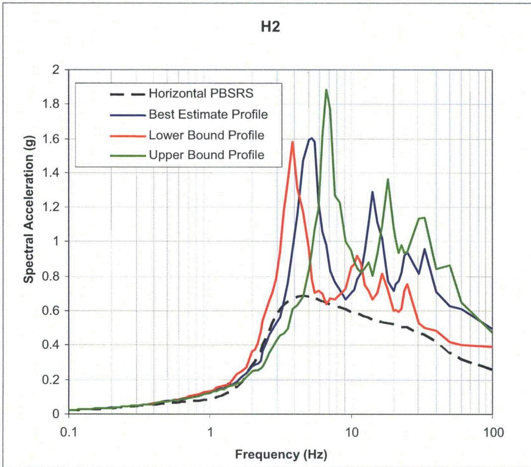
**Figure 3.7.1-250:** Comparison of Response Spectra of Computed Horizontal (H2) Component Surface Motions for SSI Profiles Using CB SCOR FIRS Input Motion to the Horizontal PBSRS.
