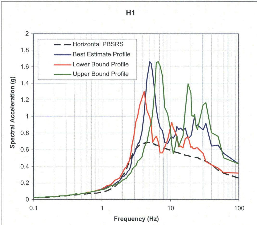
**Figure 3.7.1-246:** Comparison of Response Spectra of Computed Horizontal (H1) Component Surface Motions for SSI Profiles Using the RB/FB SCOR FIRS Input Motion to the Horizontal PBSRS.
