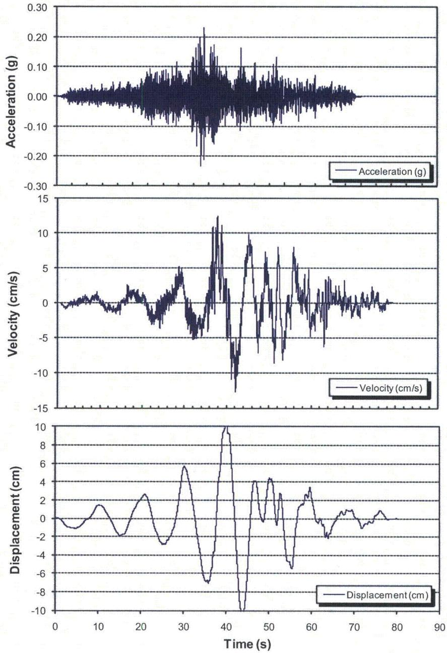
**Figure 3.7.1-241: Acceleration, Velocity, and Displacement Time Histories for the SSI FIRS Horizontal (H2) Component Compatible with the RB/FB Horizontal SSI FIRS.**
