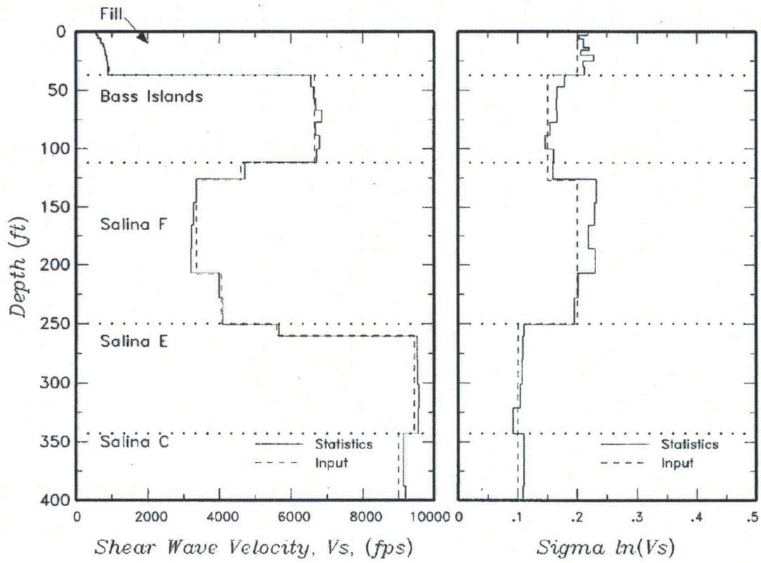
**Figure 3.7.1-205: Statistics of Randomized Shear Wave Velocity Profiles for the Intermediate Range Site Response Analysis Profile.**
