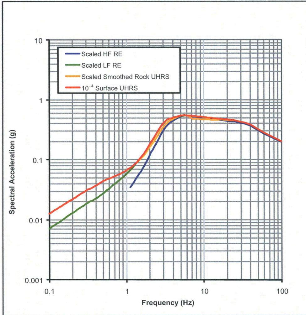
**Figure 3.7.1-212:** Development of 10<sup>-4</sup> Surface UHRS at the Finished Ground Level Grade for the Full Soil Column Profile.
