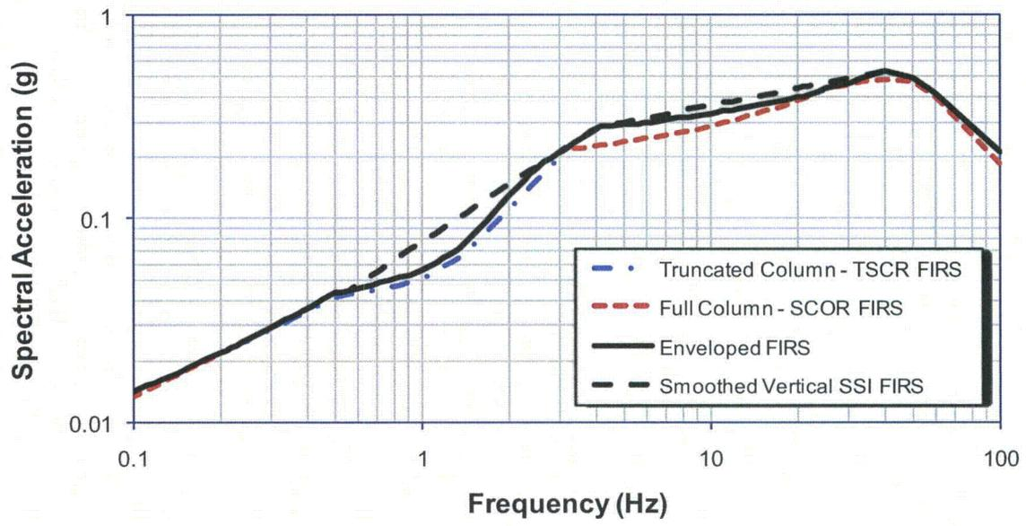
Figure 3.7.1-231: Development of Vertical Fermi 3 SSI FIRS for the CB.
