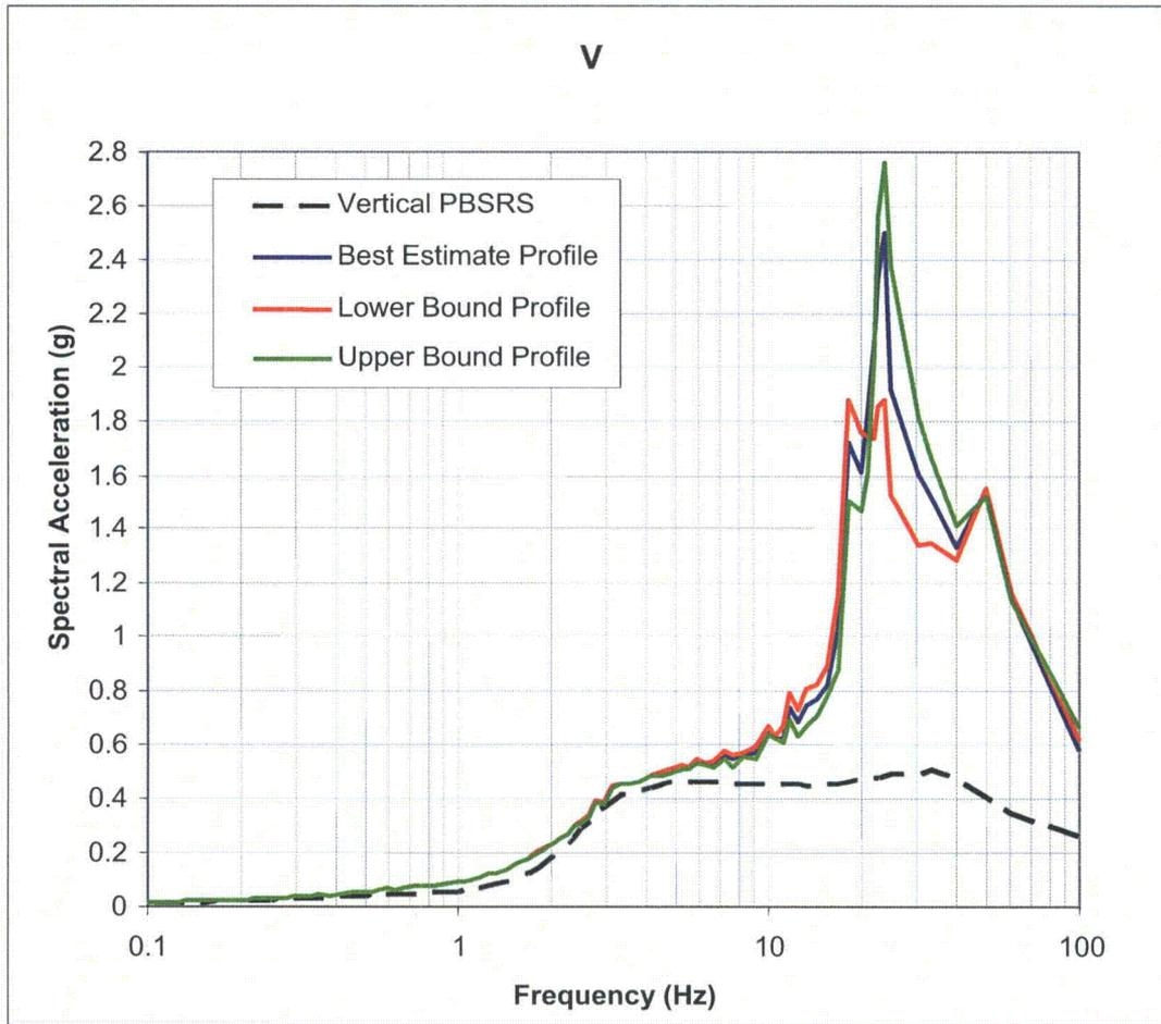
**Figure 3.7.1-248:** Comparison of Response Spectra of Computed Vertical (V) Component Surface Motions for SSI Profiles Using RB/FB SCOR FIRS Input Motion to the Vertical PBSRS.
