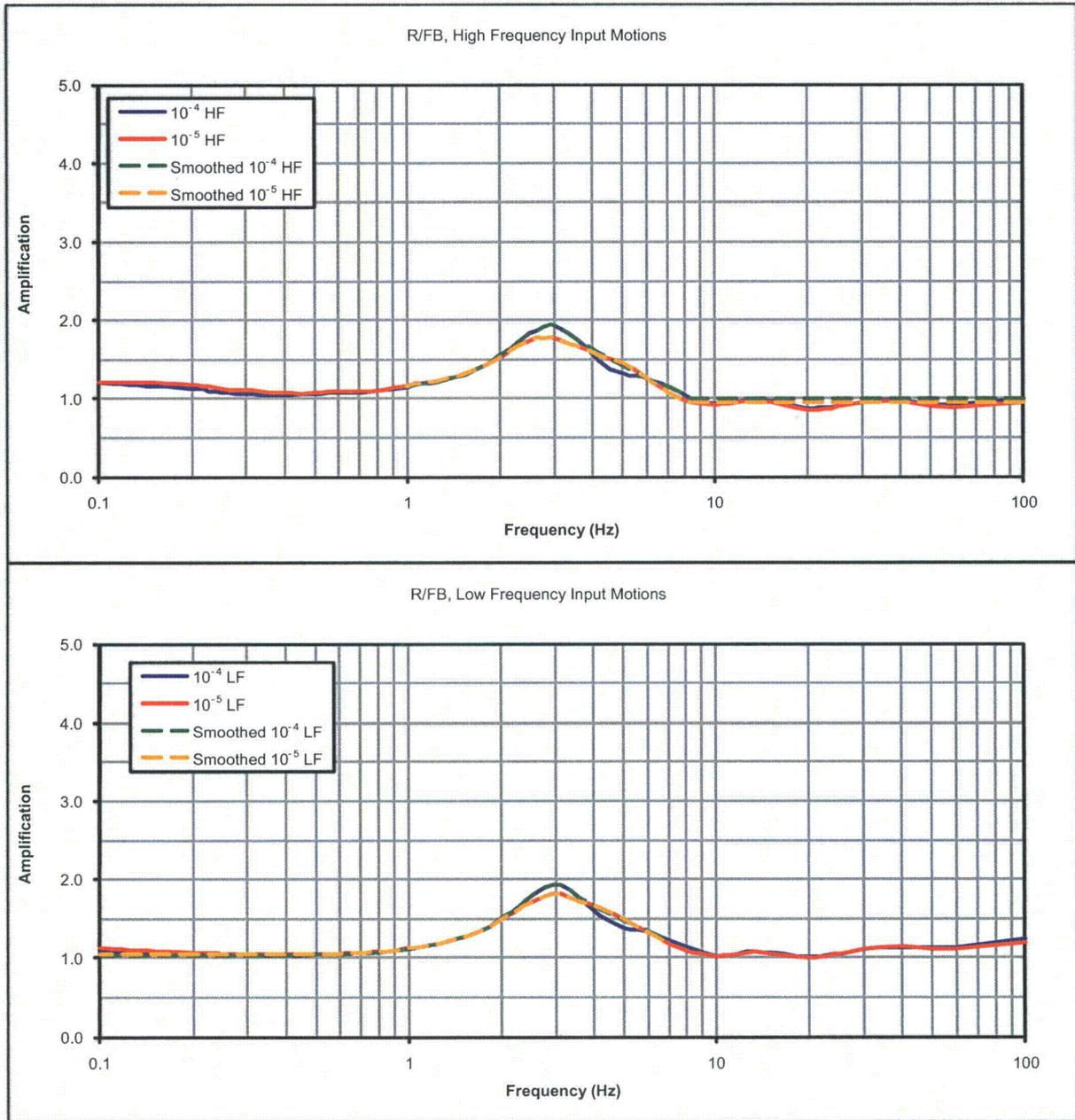
Figure 3.7.1-210: RB/FB SCOR Amplification Functions for the Fermi 3 Site.
