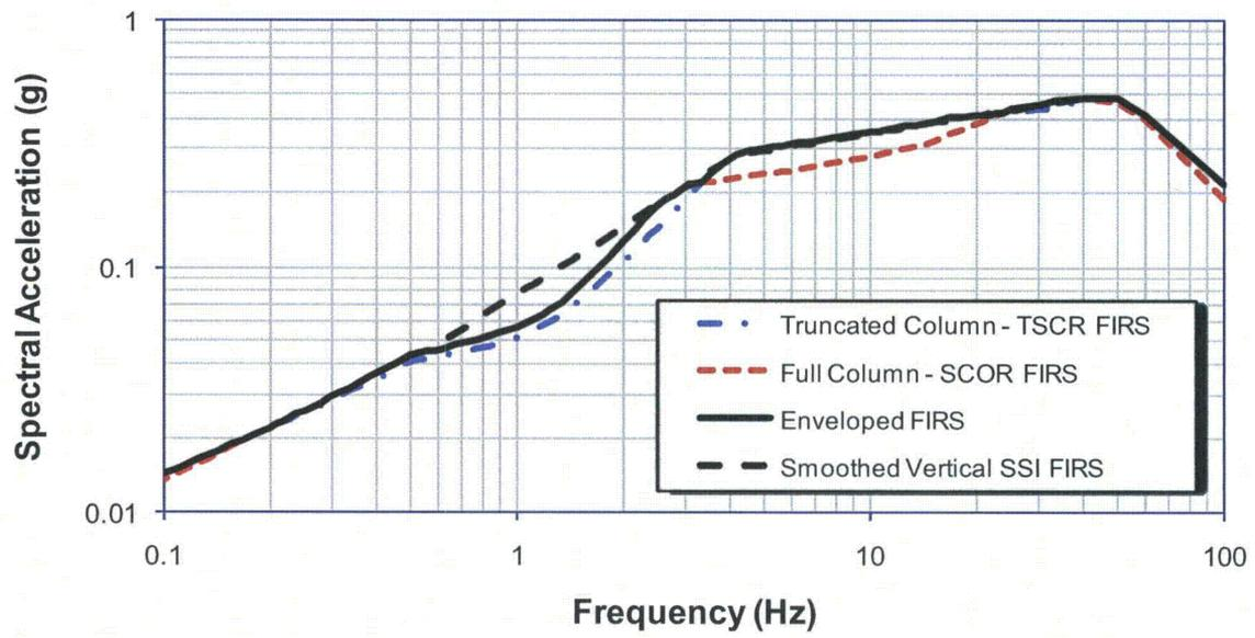
**Figure 3.7.1-230: Development of Vertical Fermi 3 SSI FIRS for the RB/FB.**
