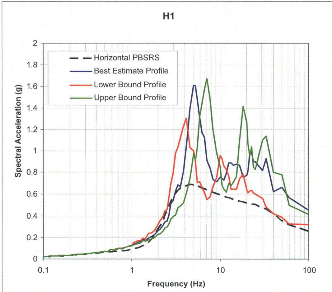
**Figure 3.7.1-249:** Comparison of Response Spectra of Computed Horizontal (H1) Component Surface Motions for SSI Profiles Using CB SCOR FIRS Input Motion to Horizontal PBSRS.
