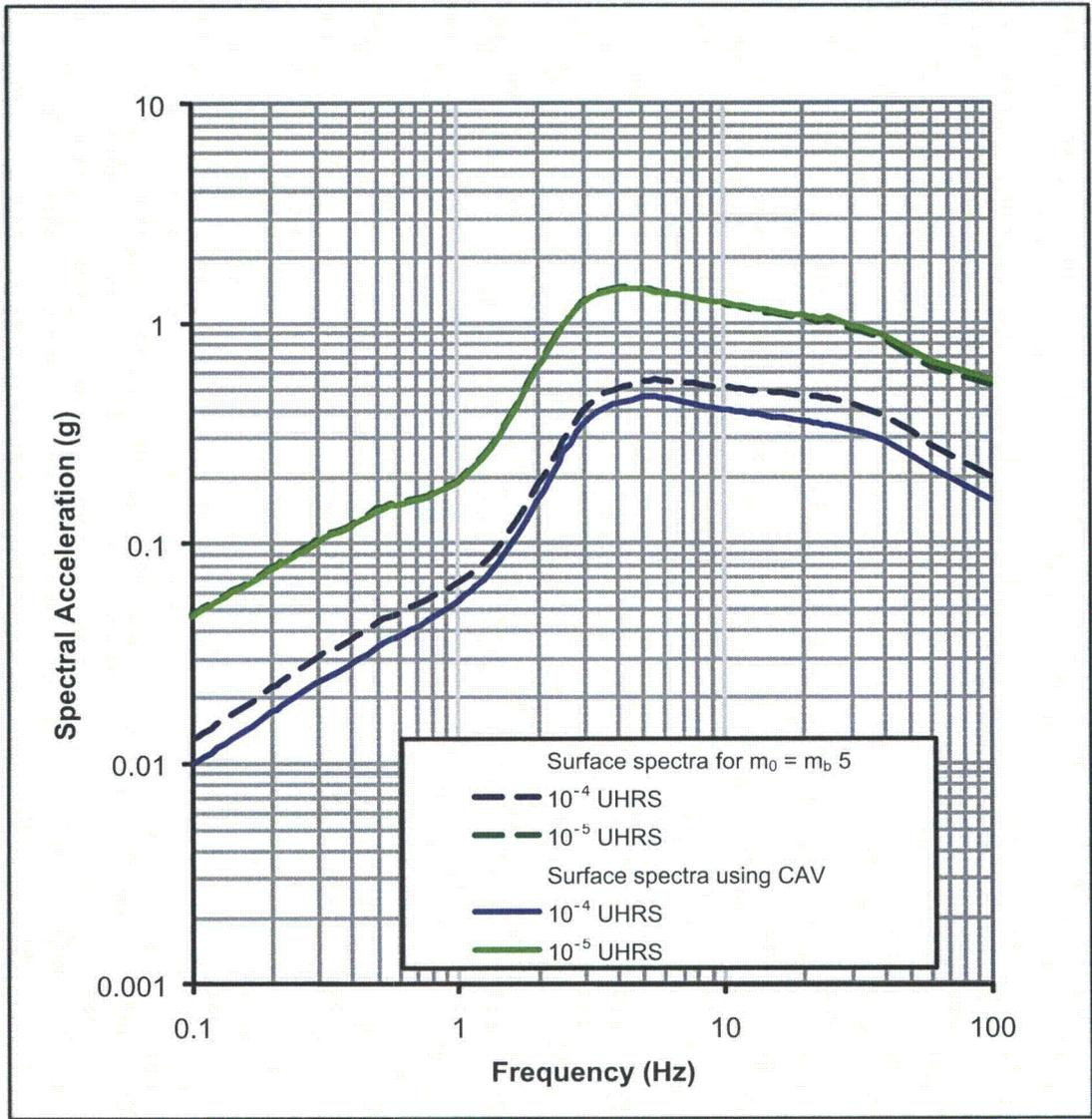
**Figure 3.7.1-221: Surface UHRS at the Finished Ground Level Grade Computed With and Without CAV.**
