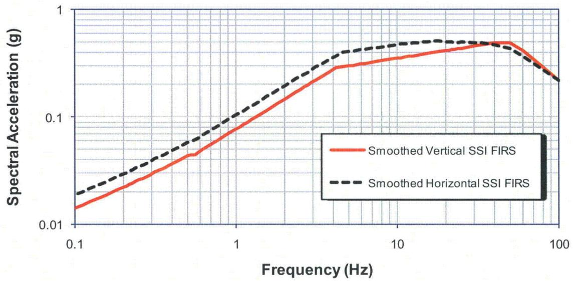
Figure 3.7.1-232: Horizontal and Vertical Fermi 3 SSI FIRS for the RB/FB.
