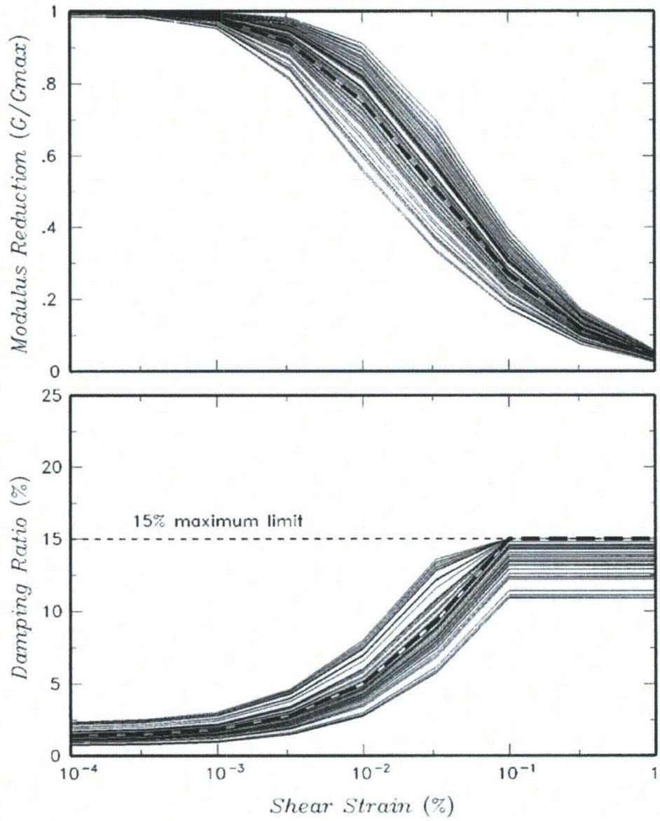
**Figure 3.7.1-206:** Randomized Shear Modulus Reduction and Damping Relationships Used for 0 to 20 Feet Depth Engineered Granular Backfill Material.
