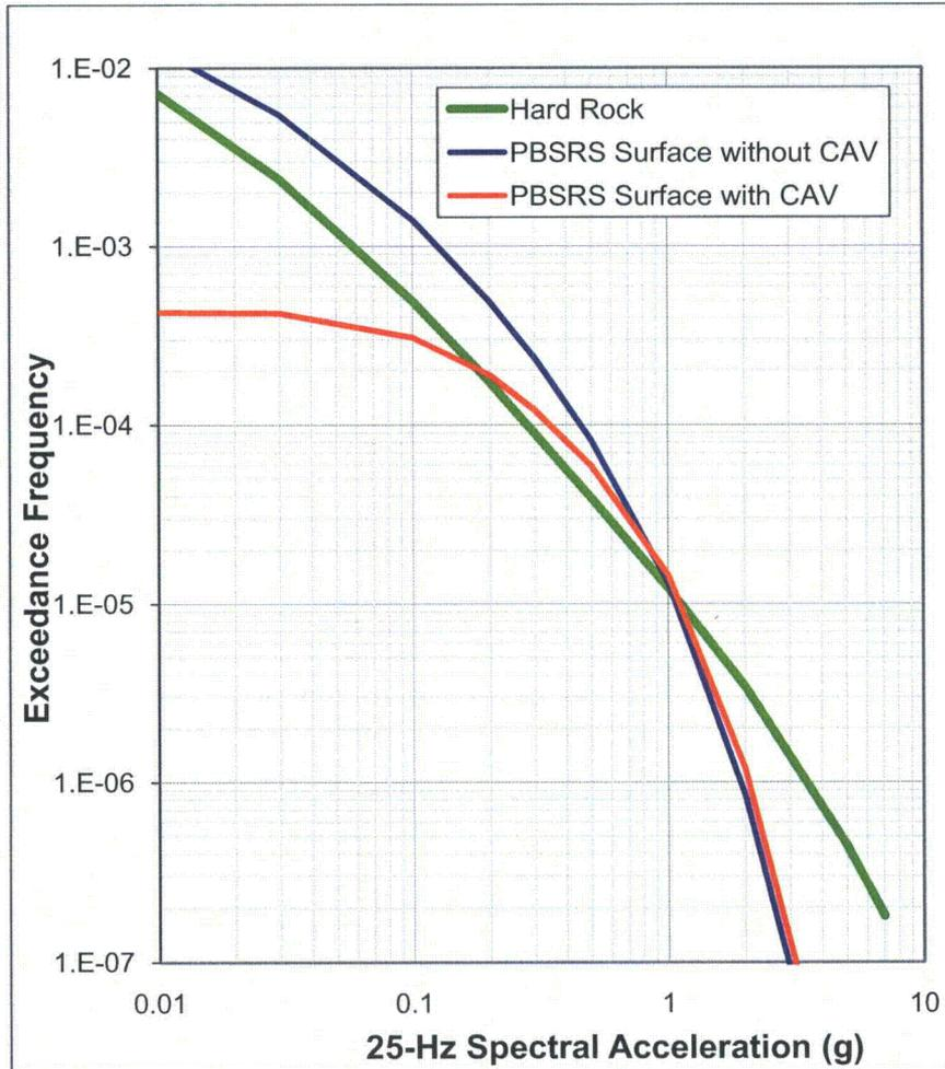
**Figure 3.7.1-219:** Surface Hazard Curves at Finished Ground Level Grade for the Full Soil Column Profile Computed With and Without CAV for 25 Hz Spectral Acceleration.
