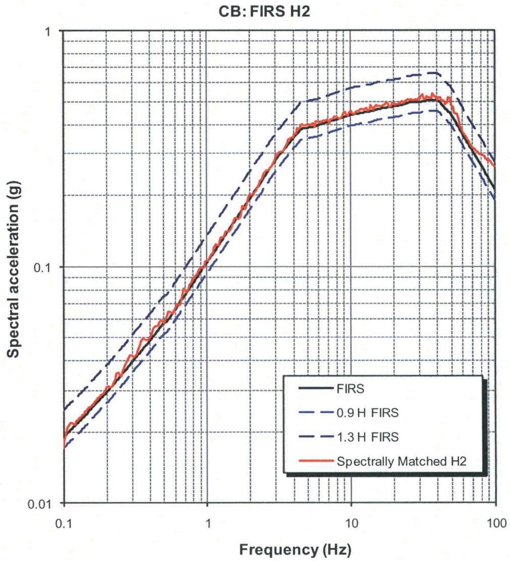
**Figure 3.7.1-238: Response Spectrum for Spectrally Matched Horizontal (H2) Component for the Fermi 3 CB SSI FIRS.**
