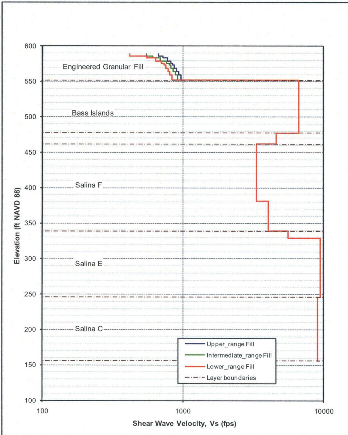
**Figure 3.7.1-201: Shear Wave Velocity Profiles for Site Response Analysis Representing the Intermediate and Bounding Estimates.**
