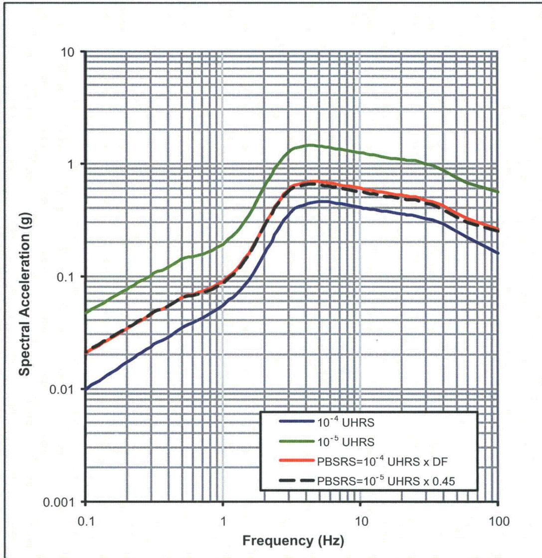
Figure 3.7.1-222: Horizontal PBSRS for the Fermi 3 Site.
