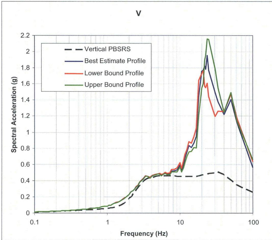
**Figure 3.7.1-251: Comparison of Response Spectra of Computed Vertical (V) Component Surface Motions for SSI Profiles Using CB SCOR FIRS Input Motion to the Vertical PBSRS.**
