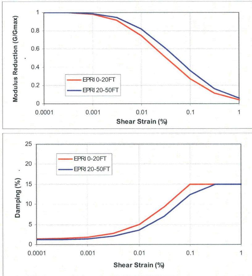
**Figure 3.7.1-202: Modulus Reduction and Damping Relationships Used for the Engineered Granular Backfill Material.**
