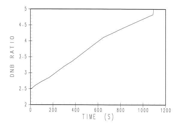
Figure 15.5.2-6 **DNBR Transient for Chemical and Volume Control System Malfunction**
