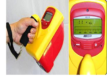
Pressurized ion chambers are more efficient and widely used in the industry. Both types of ion chambers are useful in determining dose rates from gamma radiation.
