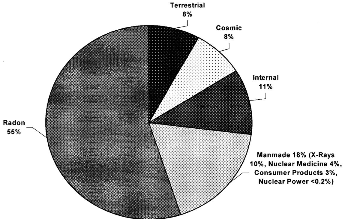
Figure 4: The most significant annual dose received by an individual of the public is that received from naturally occurring radon. A very small annual dose to the public results from producing electricity by nuclear power.
