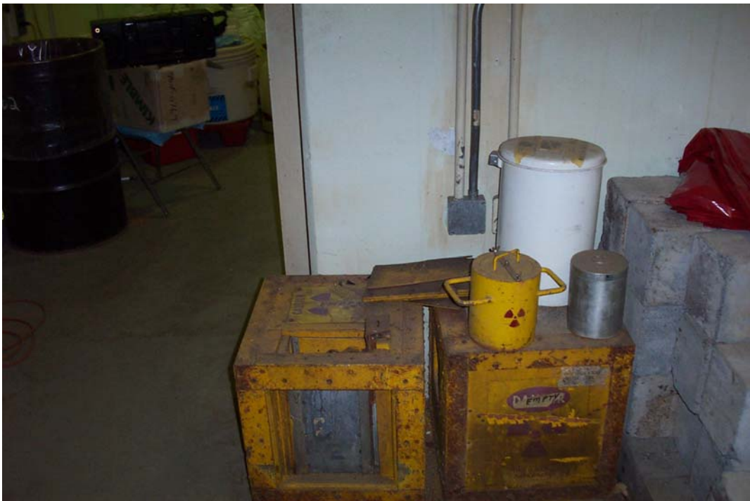
Lower Floor – Lead Shielded Boxes and Entrance to "Warm" Room
