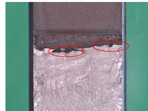
Example of local crack extension
