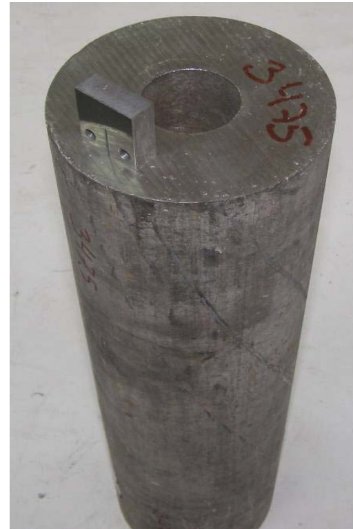
CRDM Alloy 690TT tube supplied by Valinox (heat WP 787)
