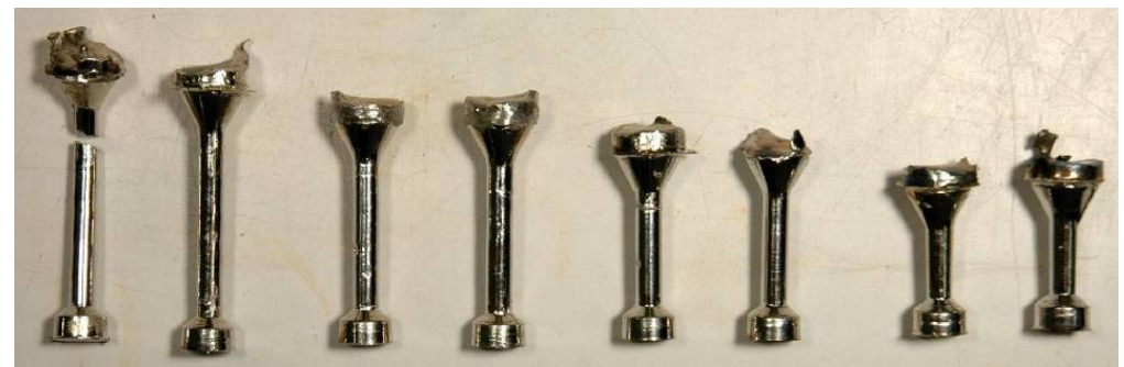
3/8" diameter pins are cast from 3/8" to 2-1/8" gauge length in 1/8" increments. Head and foot of pin restrain gauge length during cooling
