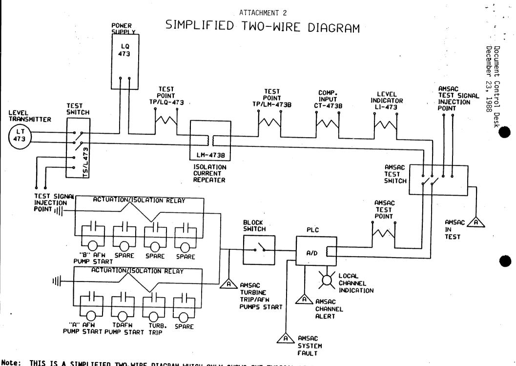
OTE: THIS IS A SIMPLIFIED TWO-WIRE DIAGRAM WHICH ONLY SHOWS ONE TYPICAL LEVEL TRANSMITTER LOOP GOING INTO THE PLC. THIS HAS BEEN DONE FOR EXPLANATORY PURPOSES. IN ACTUALITY THERE ARE FOUR LEVEL TRANSMITTER LOOPS GOING INTO THE PLC AND A THREE OF FOUR COINCIDENCE IS REQUIRED FOR AMSAC ACTUATION.
