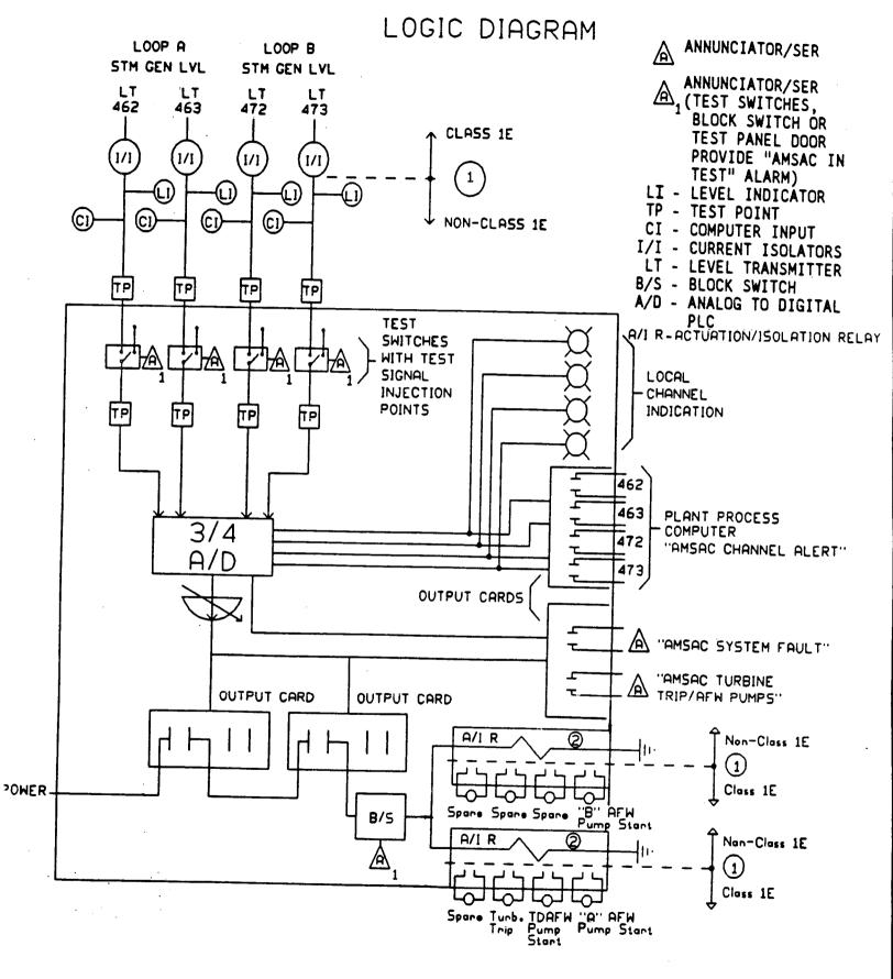
THE CLASS 1E/NON-1E INTERFACE ISOLATION DEVICES ARE THE CURRENT ISOLATORS AND THE ACTUATION/ISOLATION RELAY.
