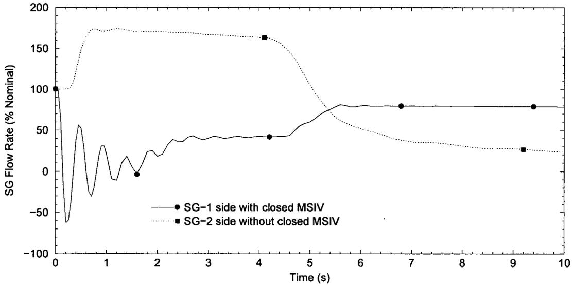
**Figure 2.3.9-9 ASGT: Steam Flow Rates (Instantaneous MSIV Closure)**
