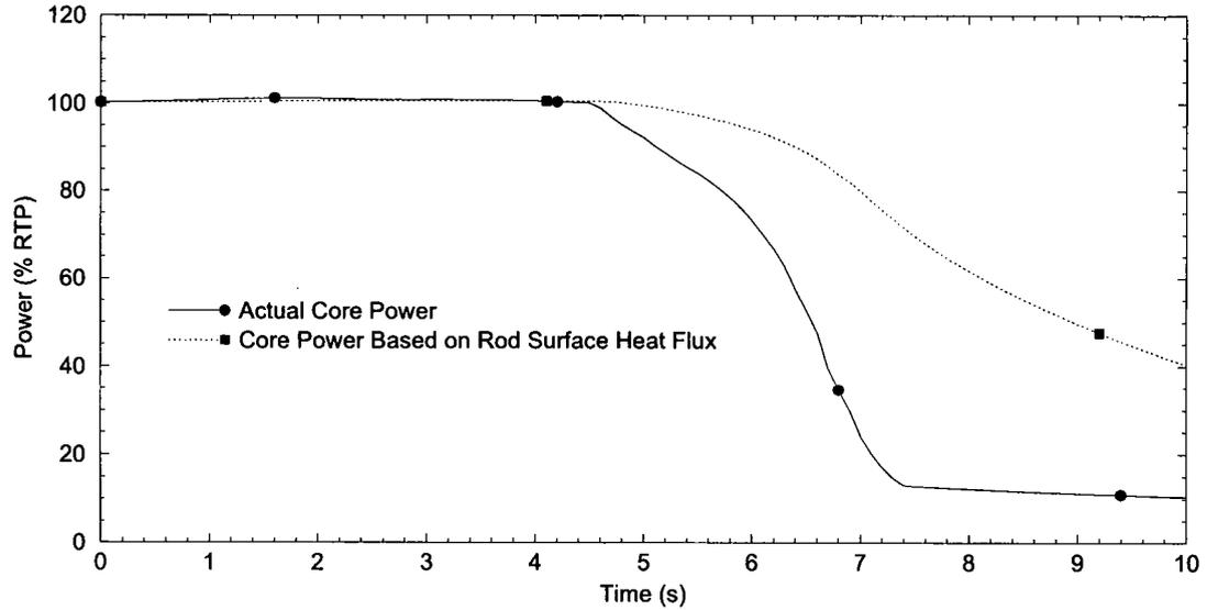
Figure 2.3.9-1 ASGT: Reactor Power (Instantaneous MSIV Closure)
