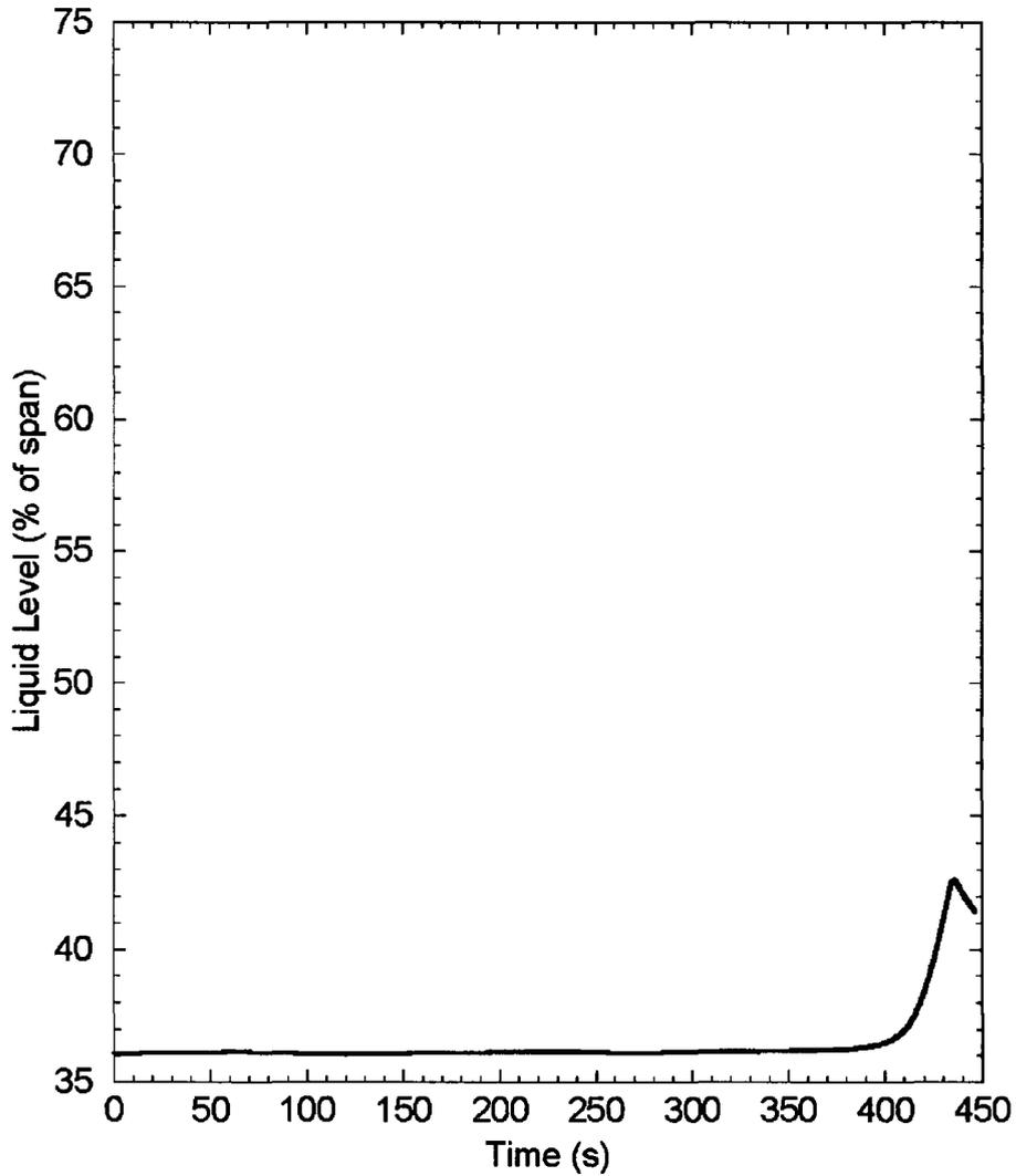
**Figure 2.3.10-4 Uncontrolled Control Rod Assembly Withdrawal from a Subcritical or Low-Power Startup Condition: Pressurizer Level (BOC RCS Overpressure)**
