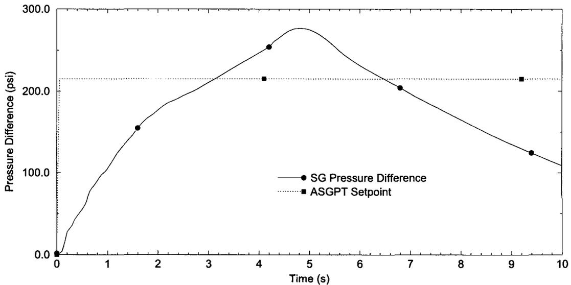
**Figure 2.3.9-4 ASGT: SG Pressure Difference vs. ASGPT Setpoint (Instantaneous MSIV Closure)**
