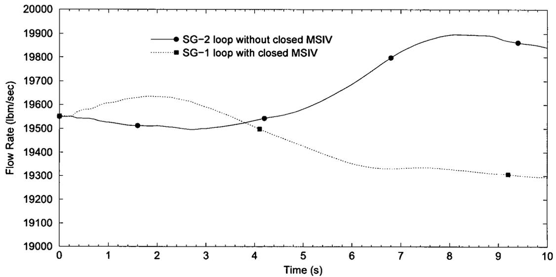
**Figure 2.3.9-6 ASGT: RCS Loop Flow Rates (Instantaneous MSIV Closure)**
