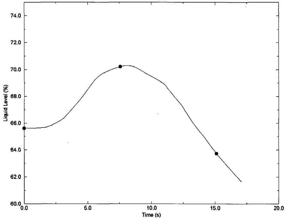
**Figure 2.3.10-3 Loss of Forced Reactor Coolant Flow: Pressurizer
