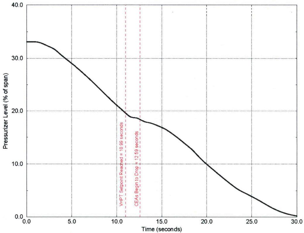
**Figure 2.3.10-1 Increase in Steam Flow (HZP): Pressurizer Liquid Level**
