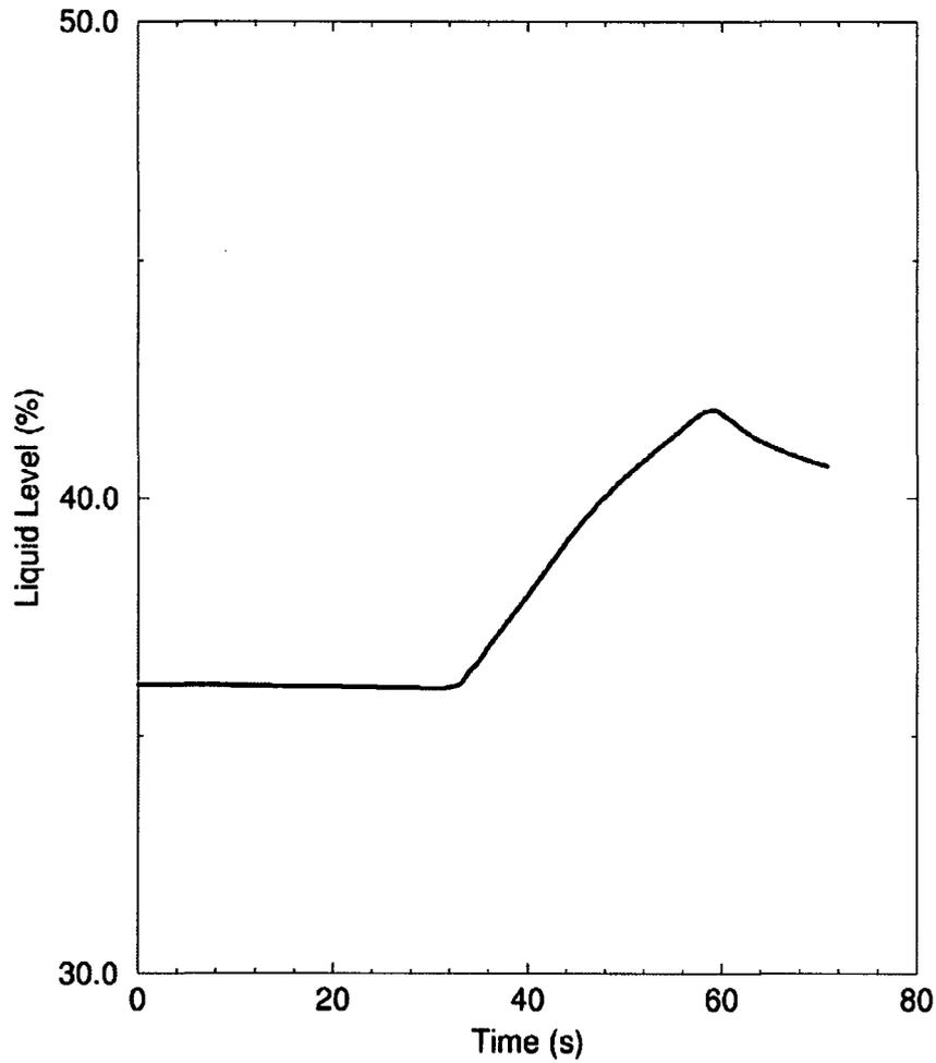
**Figure 2.3.10-5 Uncontrolled Control Rod Assembly Withdrawal from a Subcritical or Low-Power Startup Condition: Pressurizer Level (EOC RCS Overpressure)**
