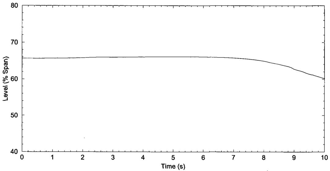
**Figure 2.3.9-8 ASGT: Pressurizer Level (Instantaneous MSIV Closure)**
