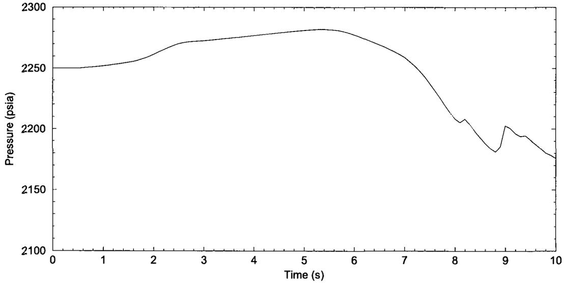
**Figure 2.3.9-7 ASGT: Pressurizer Pressure (Instantaneous MSIV Closure)**
