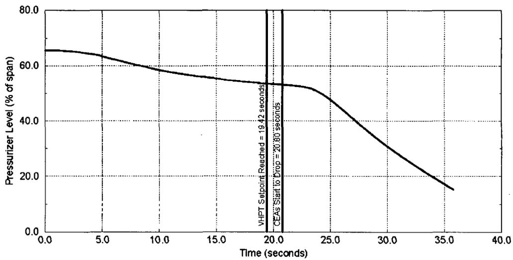
Figure 2.3.10-2 Increase in Steam Flow (HFP): Pressurizer Liquid Level
