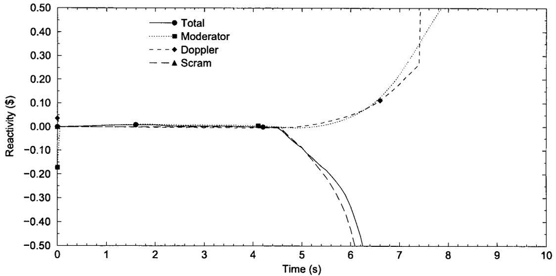
Figure 2.3.9-2 ASGT: Reactivity Feedback (Instantaneous MSIV Closure)
