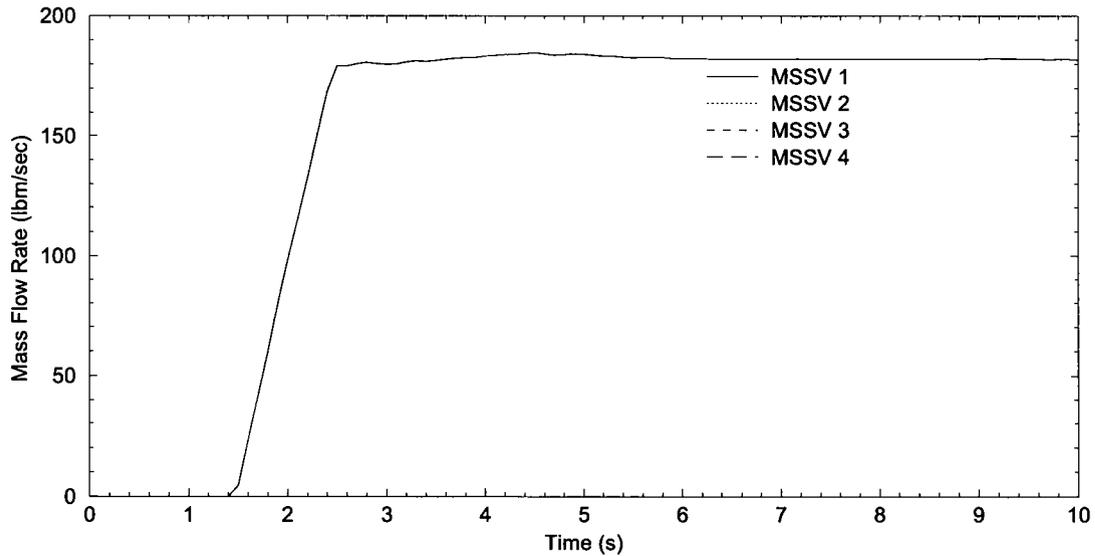
**Figure 2.3.9-10 ASGT: MSSV Flows (Instantaneous MSIV Closure)**
