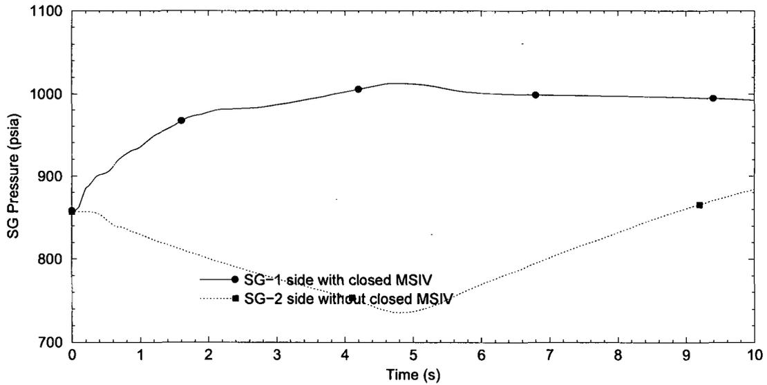
**Figure 2.3.9-3 ASGT: SG Pressures (Instantaneous MSIV Closure)**
