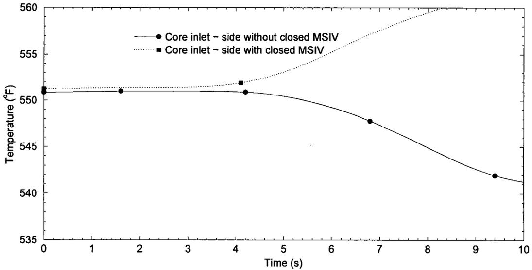
**Figure 2.3.9-5 ASGT: Core Inlet Temperatures (Instantaneous MSIV Closure)**
