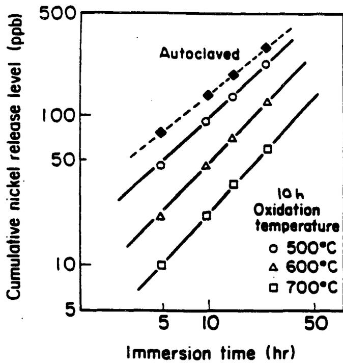
Figure 1. Cumulative Nickel Release from Autoclaved and Pre-oxidized Alloy X-750 [2]
