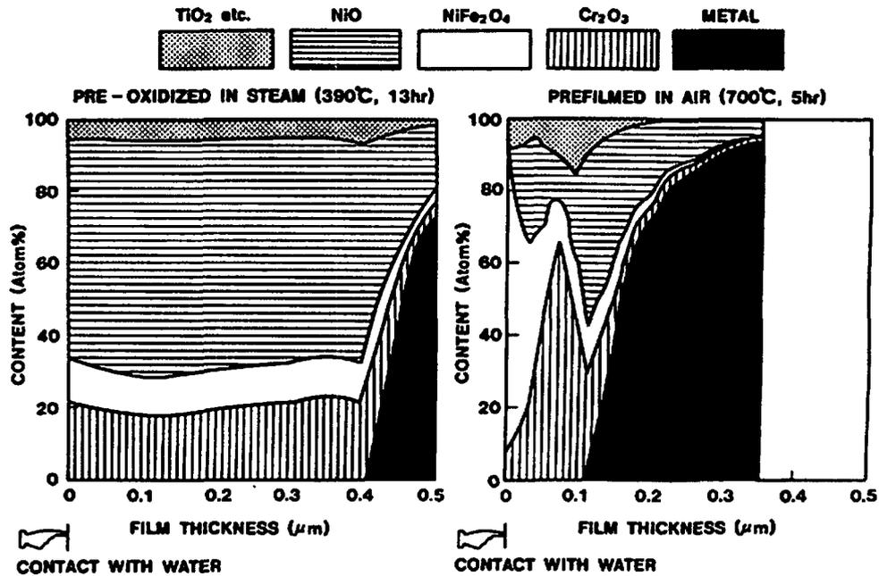
Figure 4. Distribution of Oxides formed on Pre-oxidized in Steam and Air on Alloy X-750 [3, 4]
