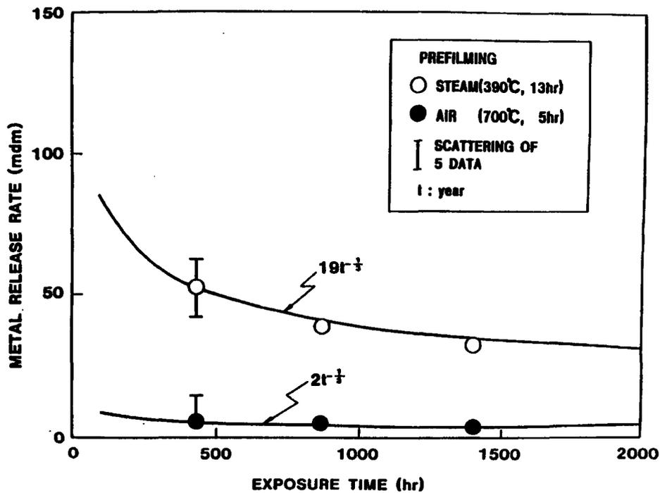
Figure 5. Metal Release Rate for Pre-oxidized in Steam and Air Alloy X-750 [3, 4]
