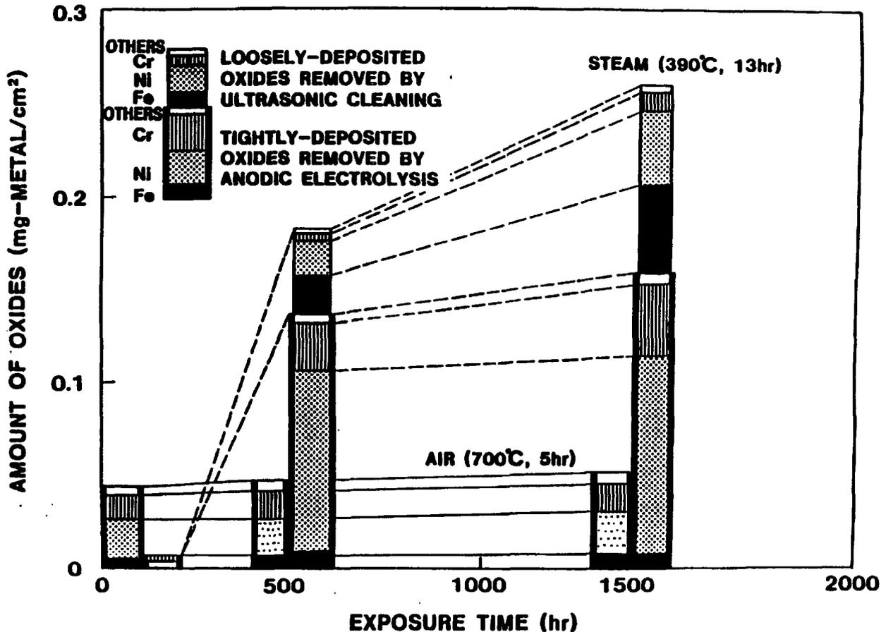
Figure 3. Comparison of Corrosion Oxides on Alloy X-750 [3, 4]
