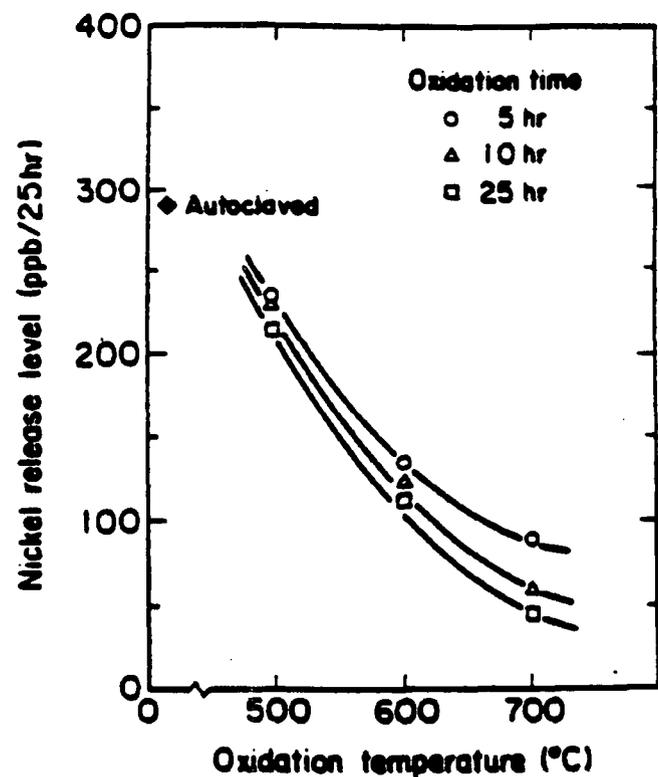
Figure 2. Effect of Pre-Oxidation Temperature on Nickel Release [2]
