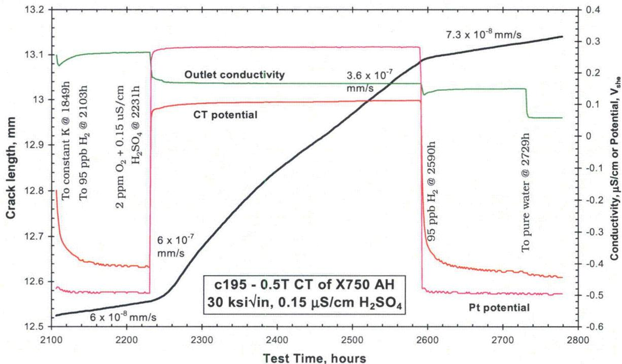
Figure 10. Crack Length vs. Time for Alloy X-750 AH Tested in 288°C Water [17, 18]
