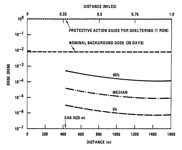
Fig. A-1. Whole body gamma dose for DBE-7 versus distance for an individual with no protective actions
