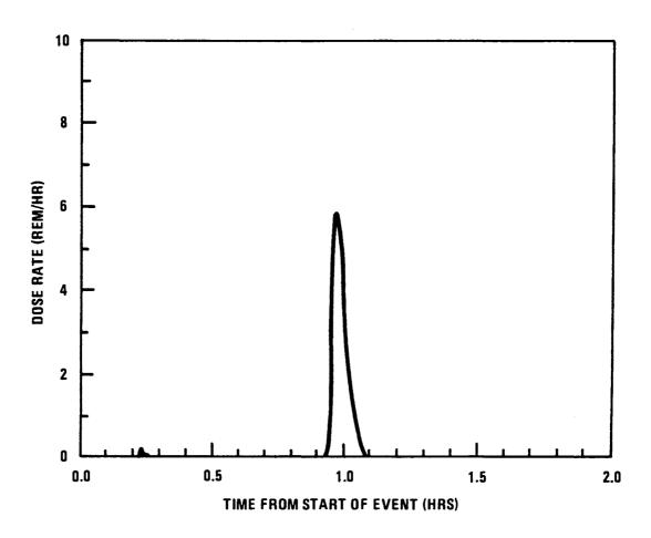
Fig. A-14. Thyroid inhalation dose rate at the EAB for EPBE-1 for an individual with no protective actions
