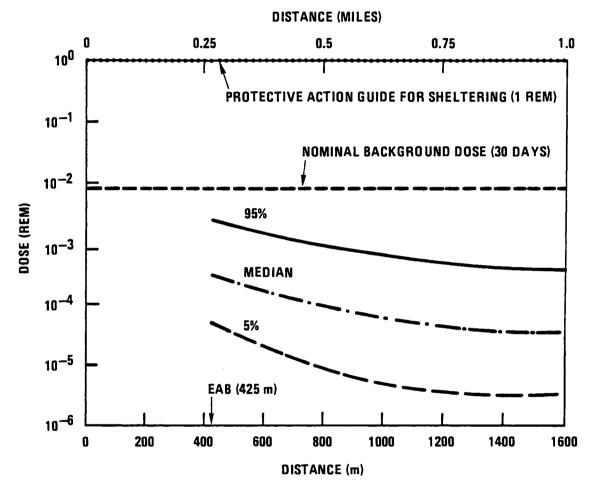
Fig. A-6. Whole body gamma dose for EPBE-3 versus distance for an individual with no protective actions
