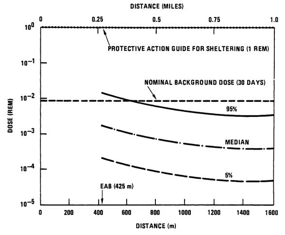
Fig. A-5. Whole body gamma dose for EPBE-2 versus distance for an individual with no protective actions
