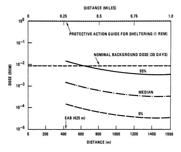
Fig. A-4. Whole body gamma dose for EPBE-1 versus distance for an individual with no protective actions
