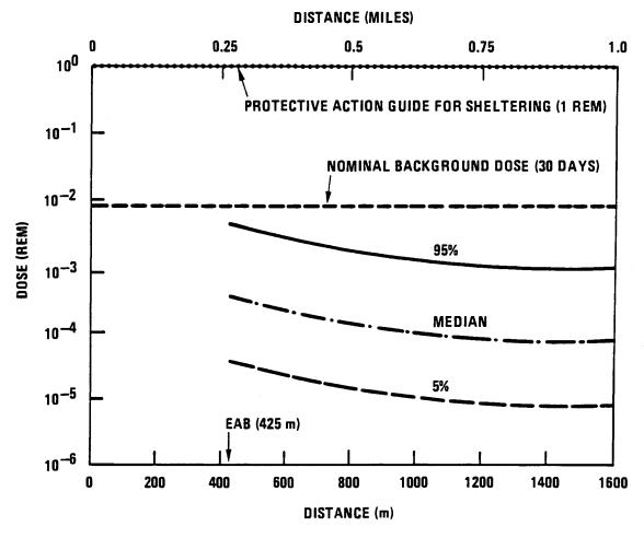
Fig. A-2. Whole body gamma dose for DBE-10 versus distance for an individual with no protective actions
