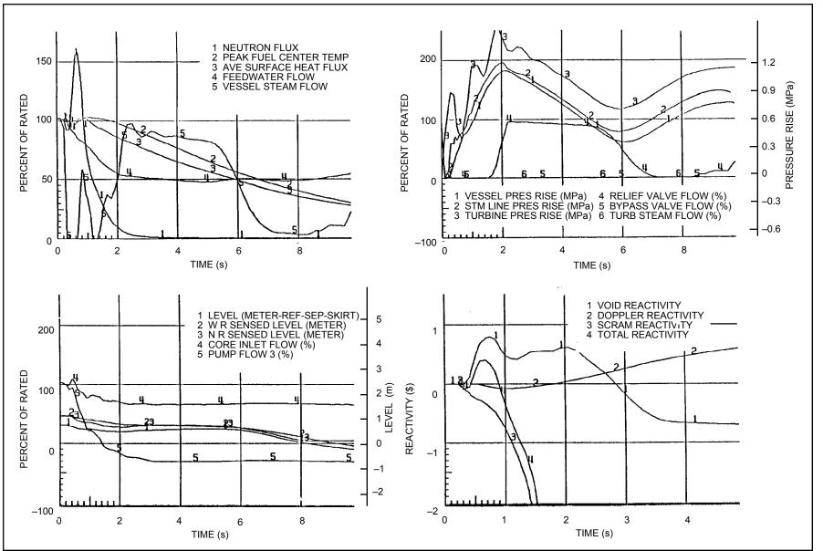
Figure 15.2-8 Turbine Trip with All Bypass Valves Failure
