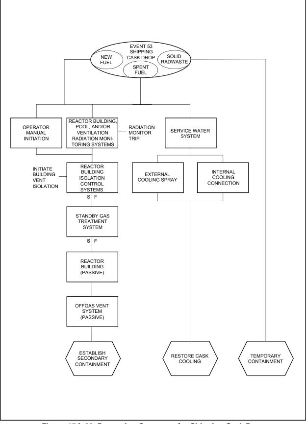
Figure 15A-60 Protection Sequence for Shipping Cask Drop
