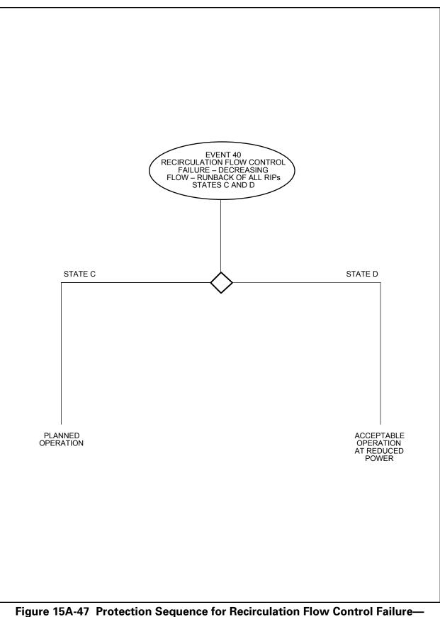
Igure 15A-47 Protection Sequence for Recirculation Flow Control Failure— Decreasing Flow—Runback of All Reactor Internal Pumps (RIPs)
