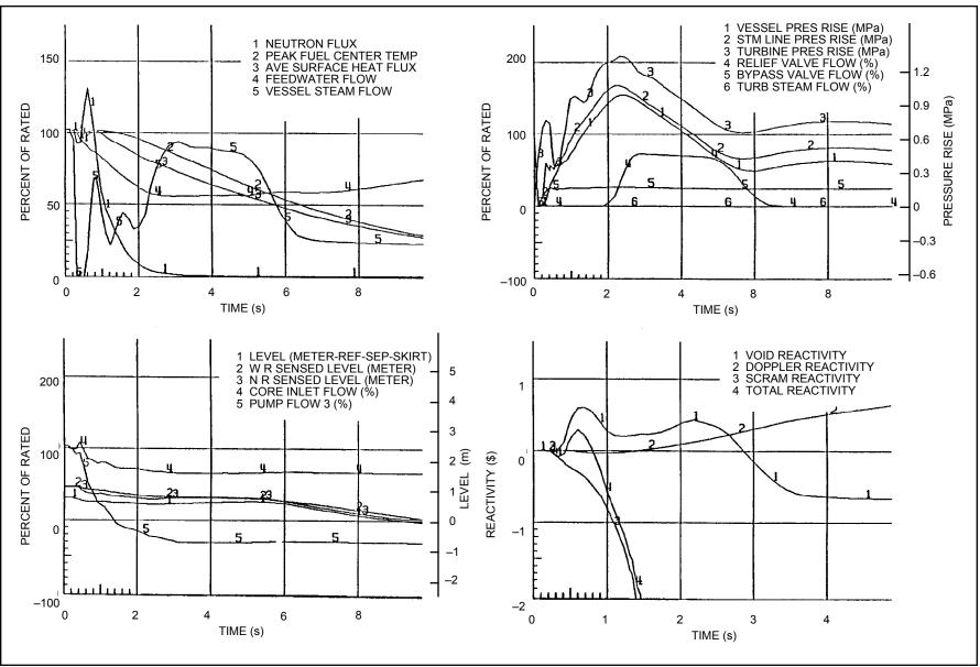
Figure 15.2-7 Turbine Trip with One Bypass Valve Failure
