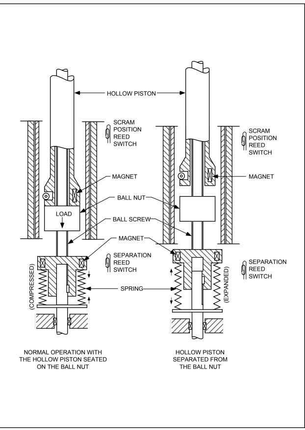
Figure 15B-5 Control Rod Separation Detection
