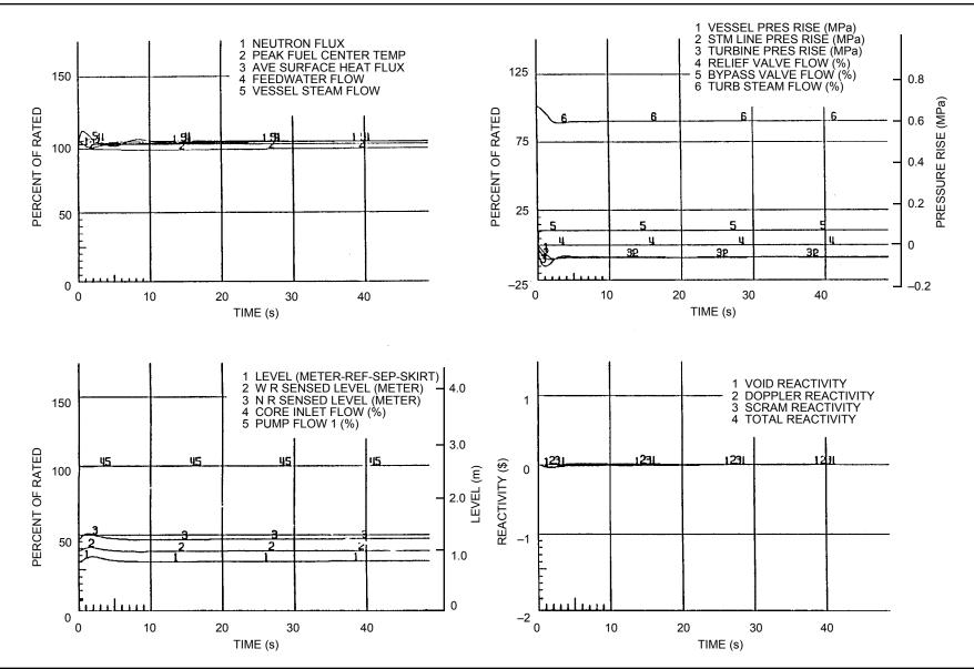
Figure 15.1-4 Inadvertent Opening of One Bypass Valve
