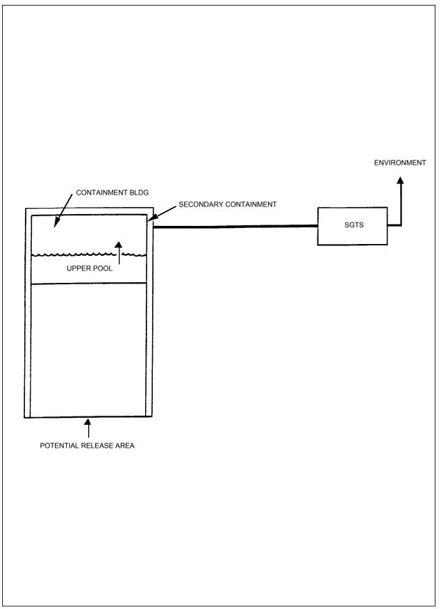
Figure 15.7-1 Leakage Path for Fuel-Handling Accident
