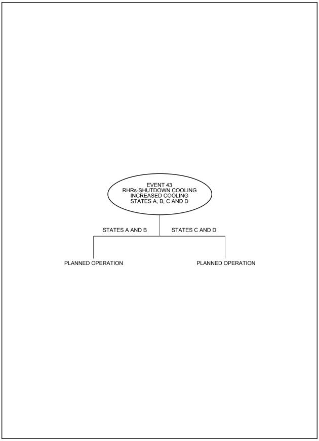
Figure 15A-50 RHR—Shutdown Cooling Failure—Increased Cooling
