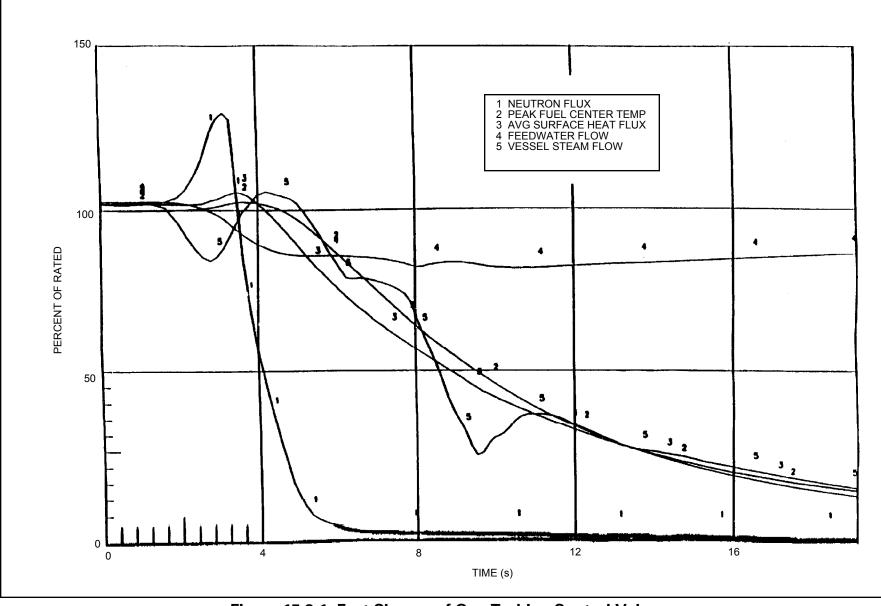
Figure 15.2-1 Fast Closure of One Turbine Control Valve
