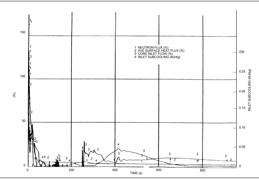
Figure 15E-17 ABWR Turbine Trip w/ Bypass, ARI (Continued)
