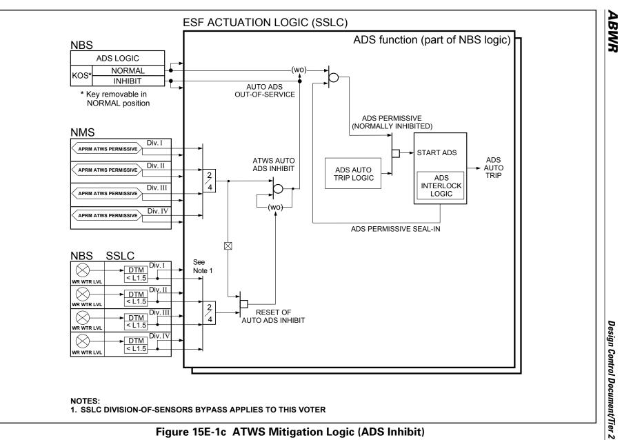
Figure 15E-1c ATWS Mitigation Logic (ADS Inhibit)
