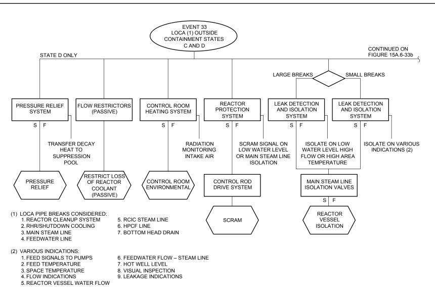
Figure 15A-39 Protection Sequences for Liquid and Steam, Large and Small Piping Breaks Outside Containment
