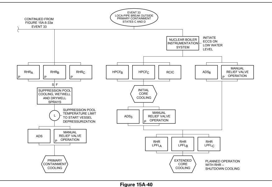
Protection Sequence for Liquid and Steam, Large and Small Piping Breaks Outside Primary Containment
