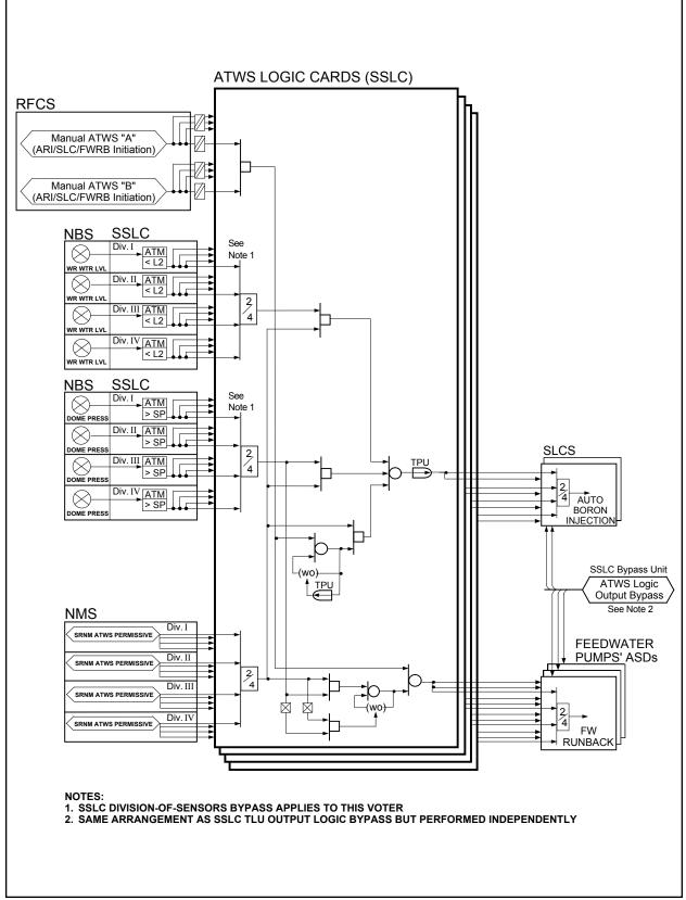
Figure 15-1b ATWS Mitigation Logic (SLCS Initiation, Feedwater Runback)
