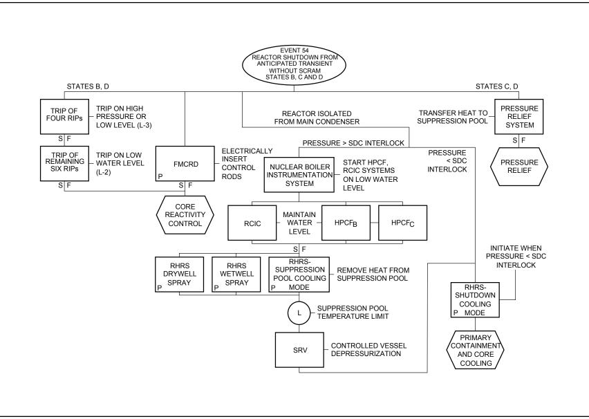
Figure 15A-61 Protection Sequence for Reactor Shutdown—from Anticipated Transient Without Scram
