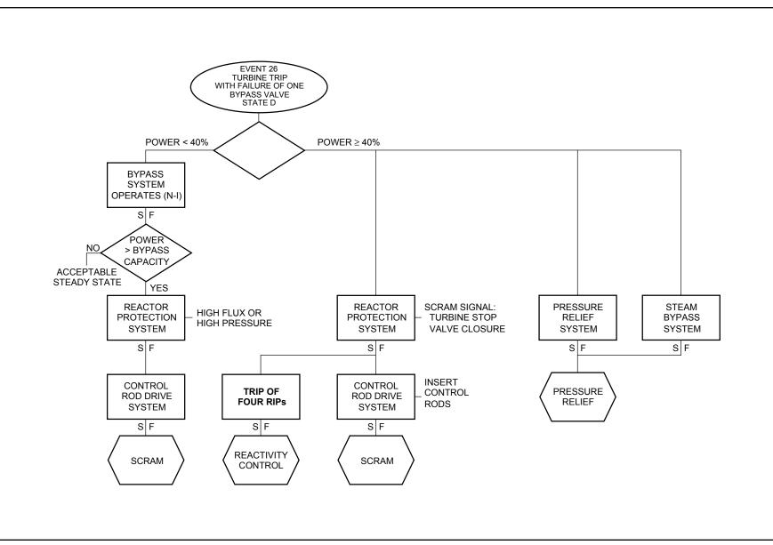
Figure 15A-31 Protection Sequences for Main Turbine Trip with Failure of One Bypass Valve
