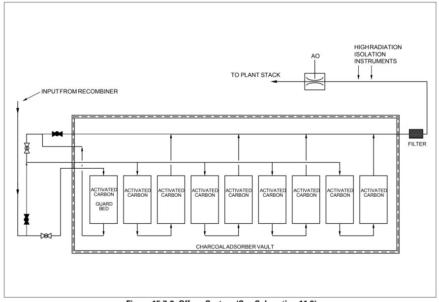
Figure 15.7-2 Offgas System (See Subsection 11.3)
