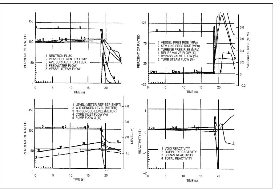
Figure 15.1-3 Feedwater Controller Failure—Maximum Demand
