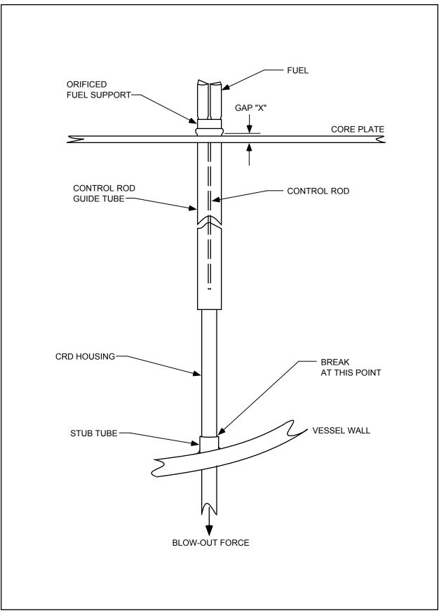
Figure 15B-7 FMCRD Internal Support
