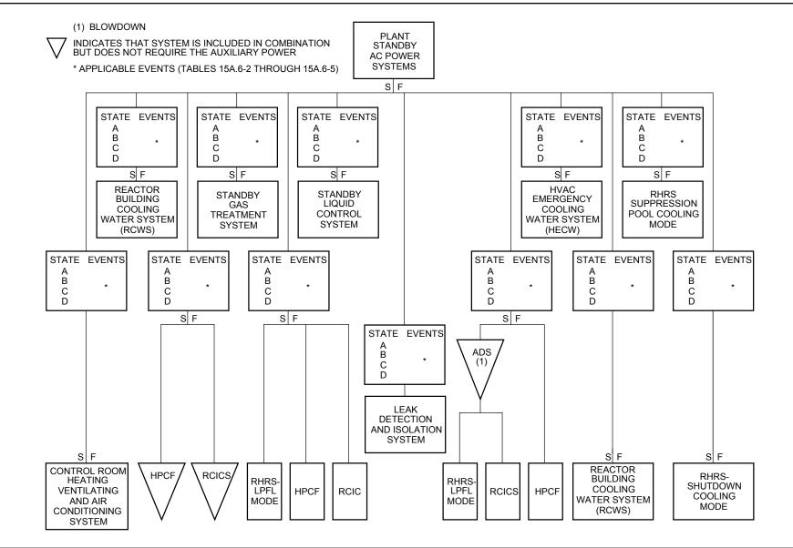
Figure 15A-66 Commonality of Standby AC Power Systems (120/480/6900 Volts)
