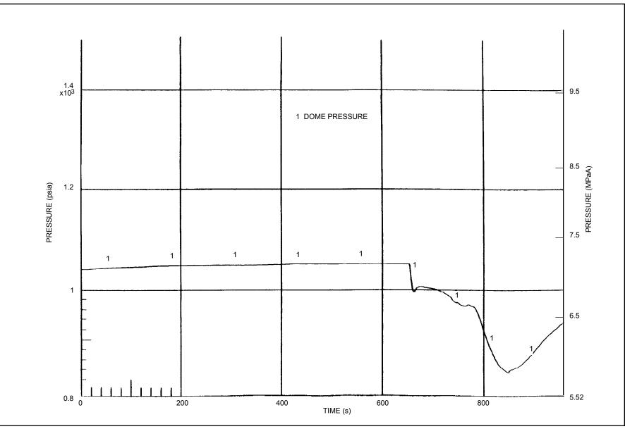
Figure 15E-13 ABWR Loss of Feedwater Heating, FMCRD Run-in
