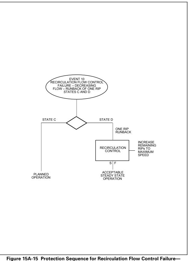
gure 15A-15 Protection Sequence for Recirculation Flow Control Failure– Decreasing Flow Runback of One Reactor Internal Pump (RIP)
