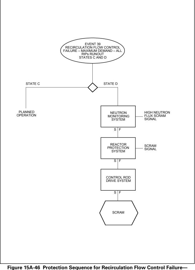
Maximum Demand—All Reactor Internal Pumps (RIPs) Runout
