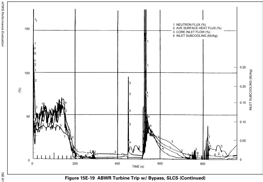
Figure 15E-19 ABWR Turbine Trip w/ Bypass, SLCS (Continued)
