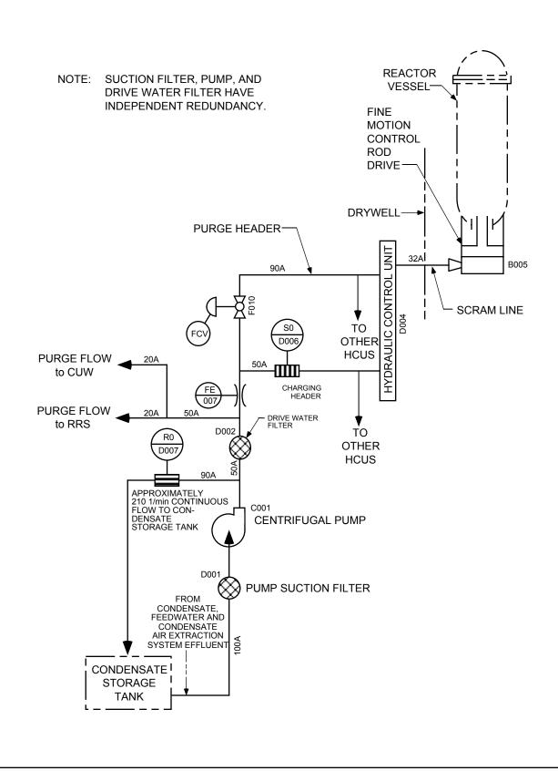
Figure 15B-1 Simplified CRD System Process Flow Diagram
