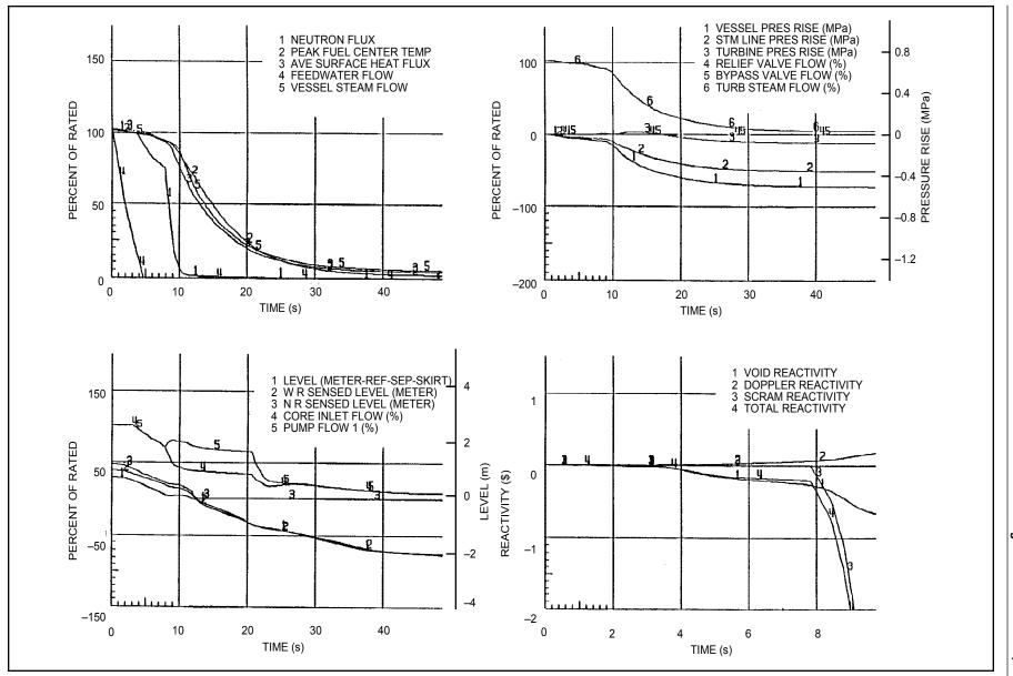
Figure 15.2-12 Loss of All Feedwater Flow
