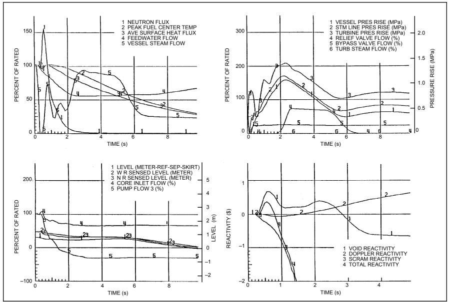
Figure 15.2-4 Load Rejection with One Bypass Valve Failure
