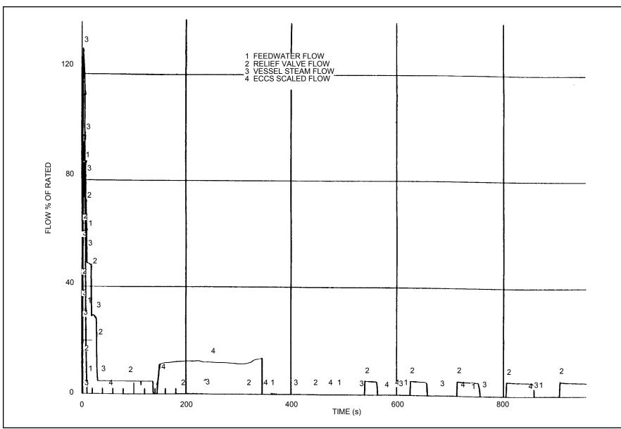
Figure 15E-20 ABWR Loss of Condenser Vacuum, ARI (Continued)
