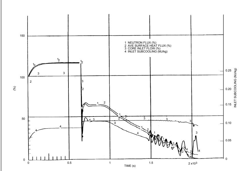
Figure 15E-14 ABWR Loss of Feedwater Heating, SLCS (Continued)
