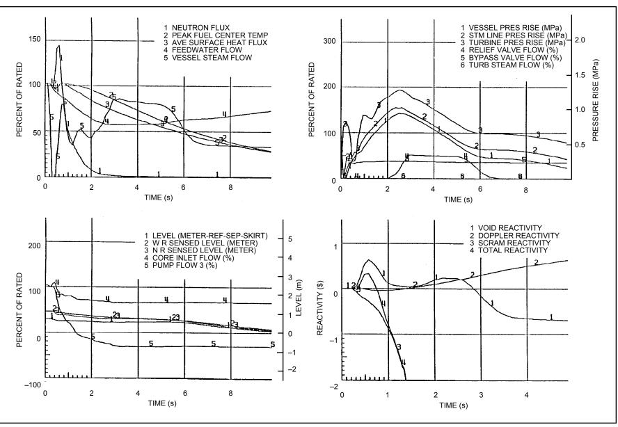
Figure 15.2-3 Generator Load Rejection with Bypass
