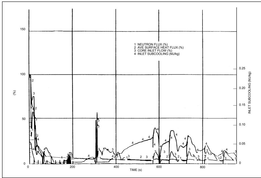
Figure 15E-10 ABWR Loss of Feedwater Flow, FMCRD Run-in (Continued)
