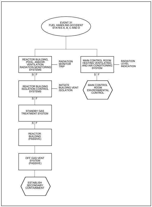
Figure 15A-36 Protection Sequences for Fuel-Handling Accident
