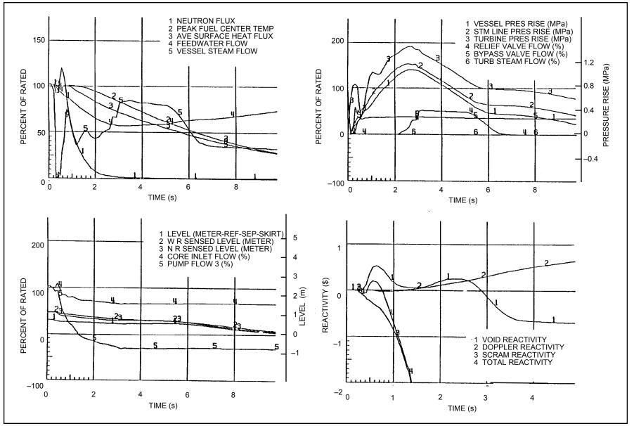
Figure 15.2-6 Turbine Trip with Bypass
