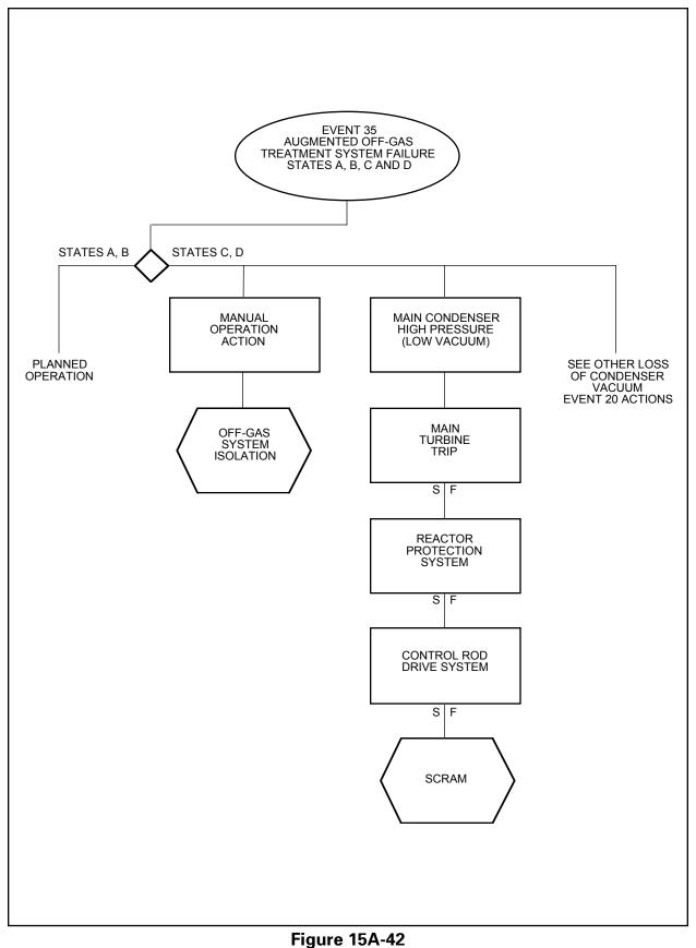
Protection Sequence for Augmented Offgas Treatment System Failure
