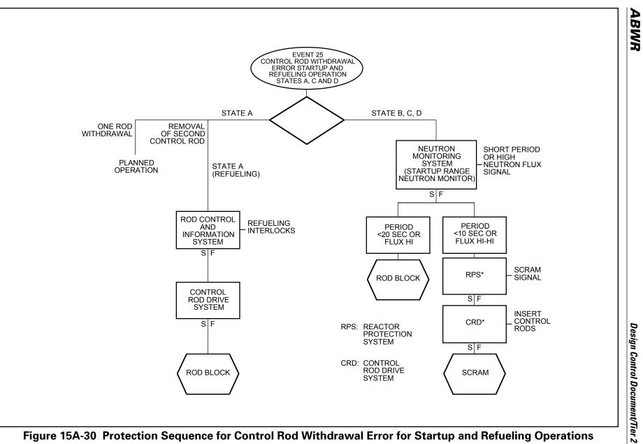
Figure 15A-30 Protection Sequence for Control Rod Withdrawal Error for Startup and Refueling Operations
