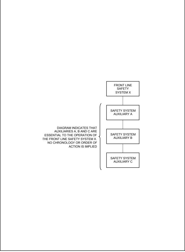
Figure 15A-4 Format for Safety System Auxiliary Diagrams
