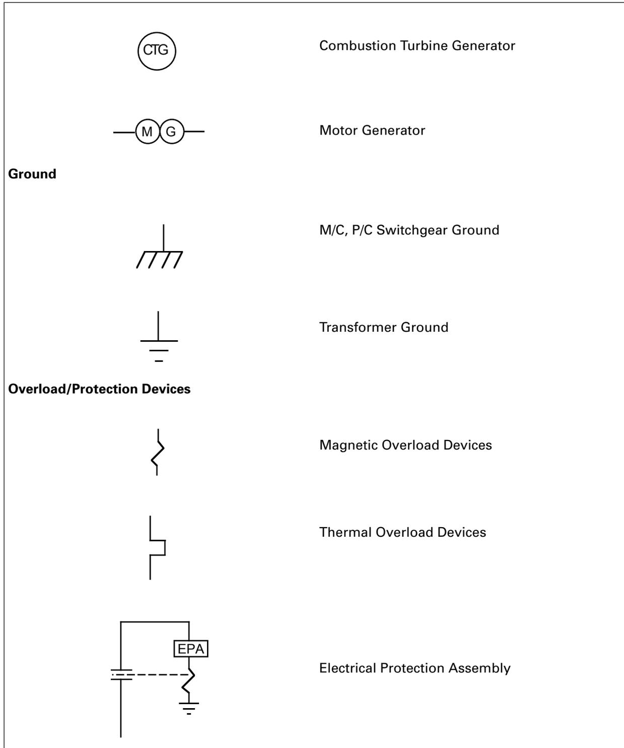
Figure 1.7-3 Graphical Symbols for Use in Electrical SLDs (Sheet 4 of 4)
