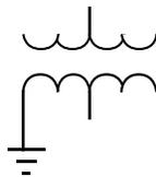
Two winding - 3 $\phi$  center tap ground
