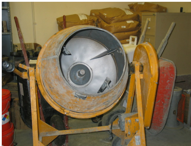
Figure 3-2. Three Cubic-Foot Concrete Mixer.
