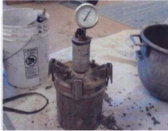
Figure 3-4. Air Content Test Apparatus.
