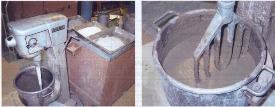
Figure 3-1. Hobart Mixer and Example of Reducing Grout after Mixing.
