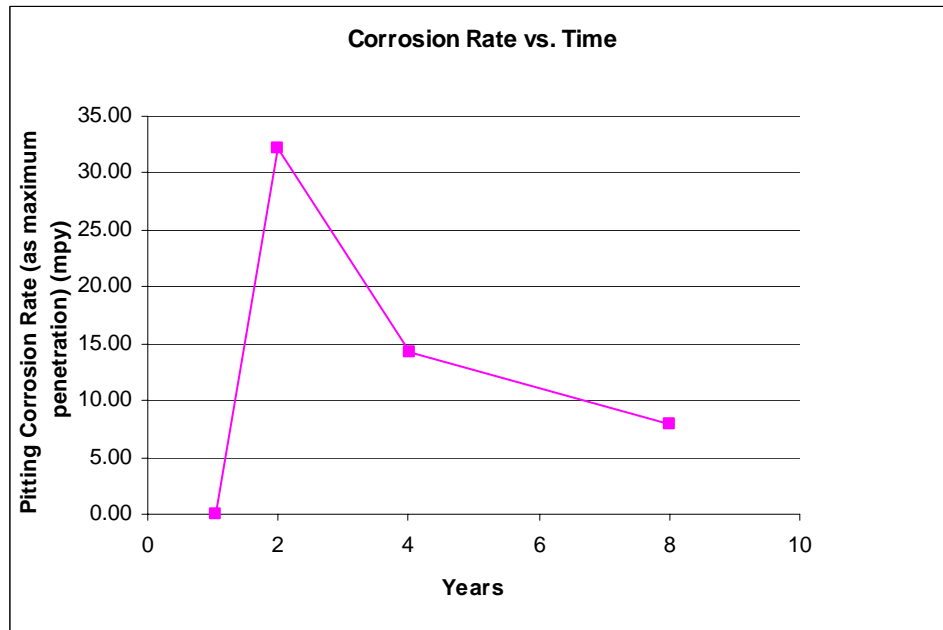
Figure 5: Corrosion Rate as Maximum Penetration Rate vs. Time of Type 304-SS Exposed to Site ‘D’.
