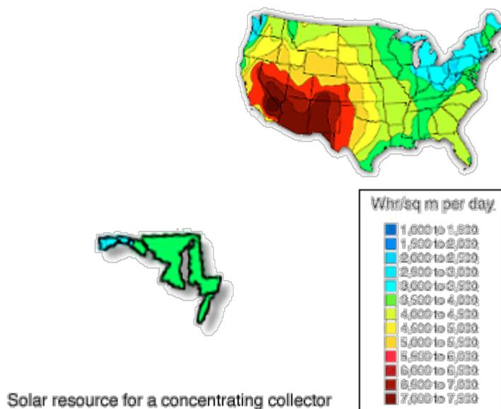
temperatures and efficiencies. These are called concentrating collectors. Typically, these collectors are on a tracker, so they always face the sun directly. Because these collectors focus the sun's rays, they only use the direct rays coming straight from the sun.
