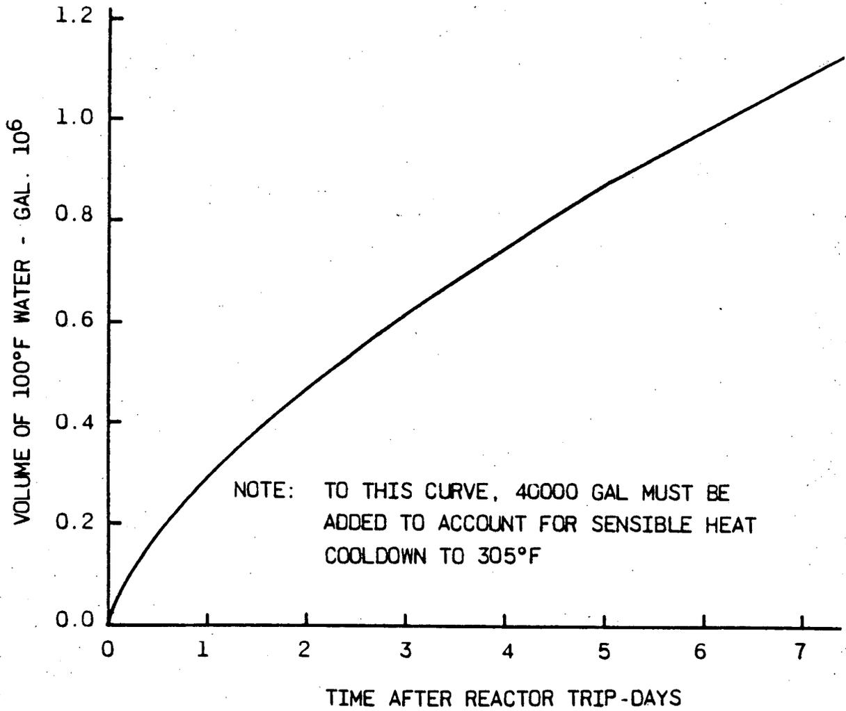
Figure 8 Natural Circulation Cooldown Temperature Vs Time
