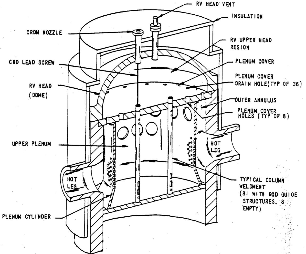
Figure 3 Upper Plenum and RV Upper Head
