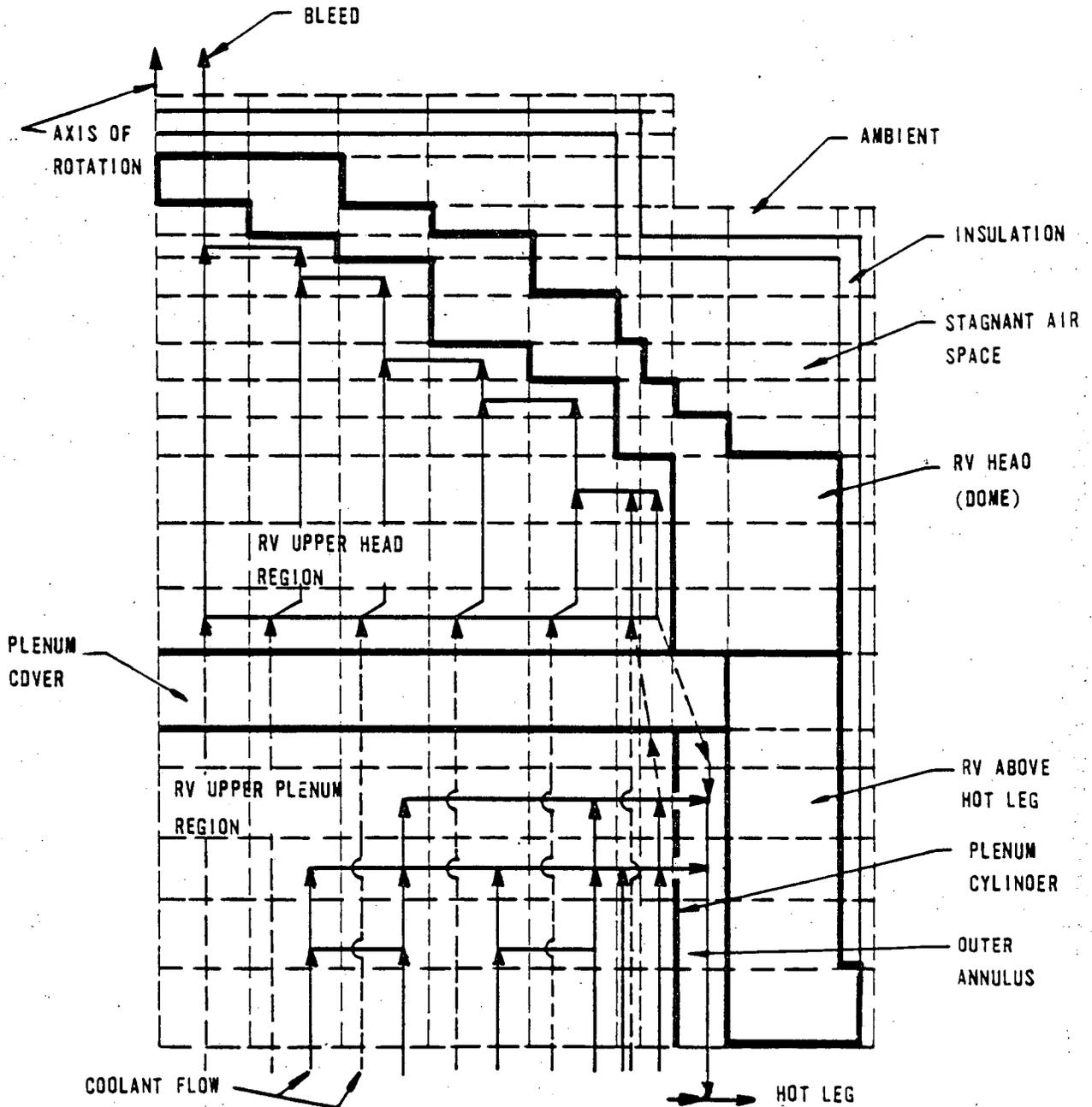
Note: This noding diagram is only a one-half cross section of the upper reactor vessel and internals. In the analysis, this noding diagram is rotated about the left side vertical axis so that the RV and internals are modeled in three dimensions. Each node thus becomes a ring.
