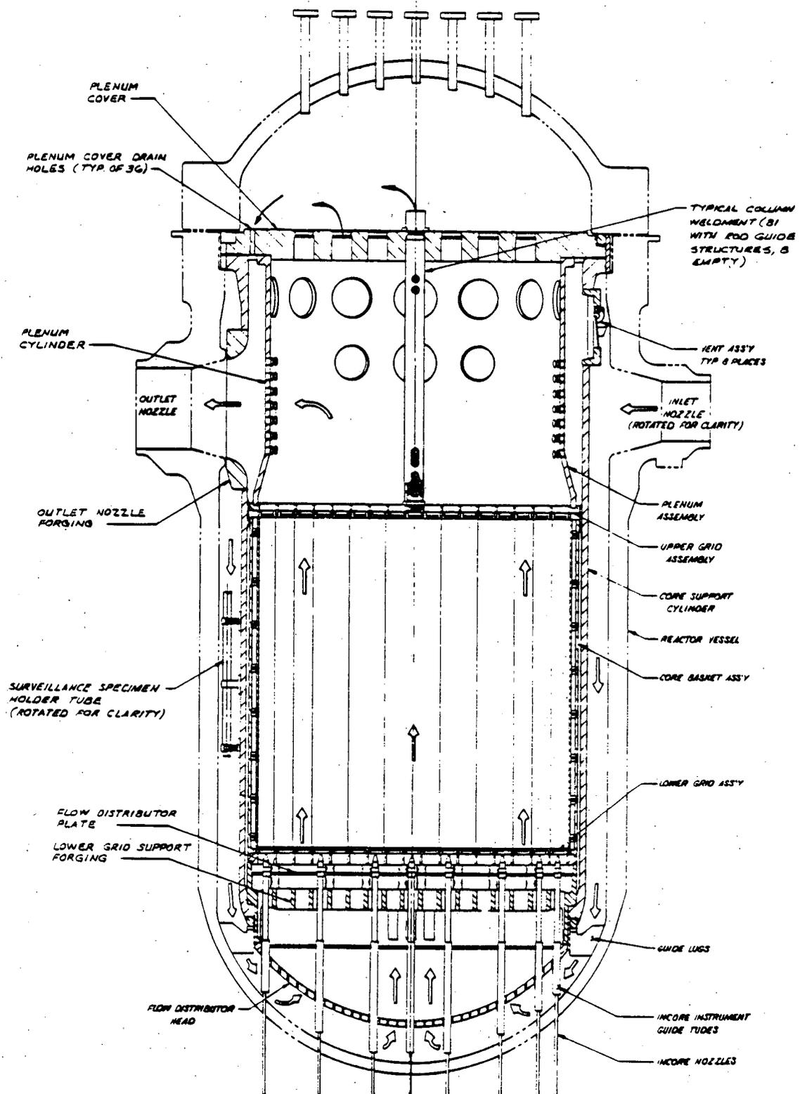
Figure 2. Schematic Diagram of Upper Portion of Reactor Vessel and Internals
