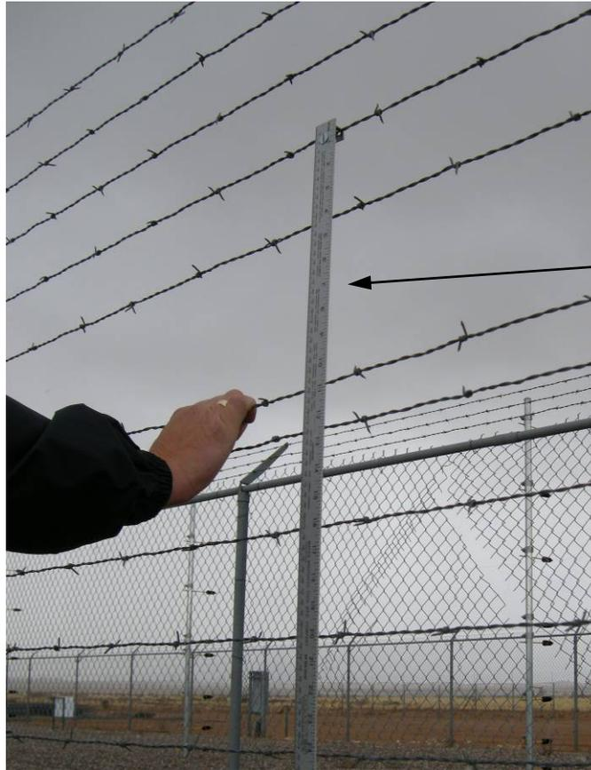
**Figure 30: A hanging yardstick allows for easy measurement of the deflection possible on a taut wire sensor before an alarm occurs.**
