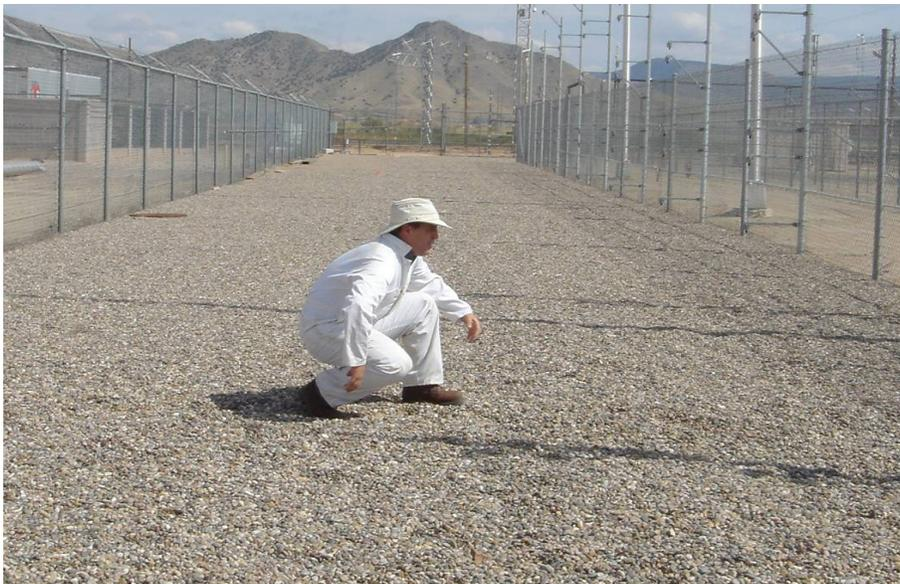
**Figure 22:** The “duck walk” seems to produce the smallest disturbance in a ported coaxial system and is therefore ideal to use to test the system.
