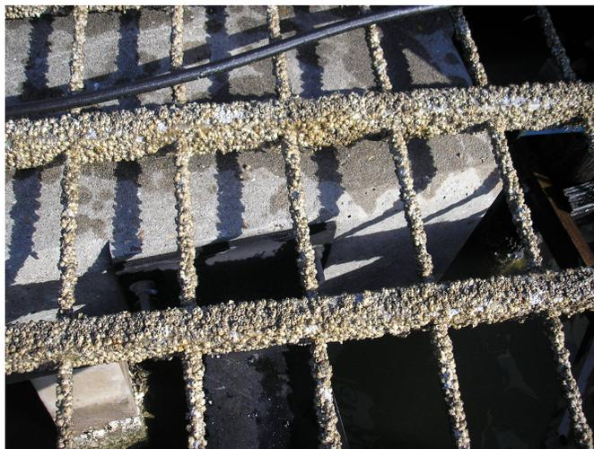
**Figure 58:** *This fiber-optic grid was tested under water for about 6 weeks and shows biofouling through barnacles, which can eventually degrade the integrity of the materials.*
