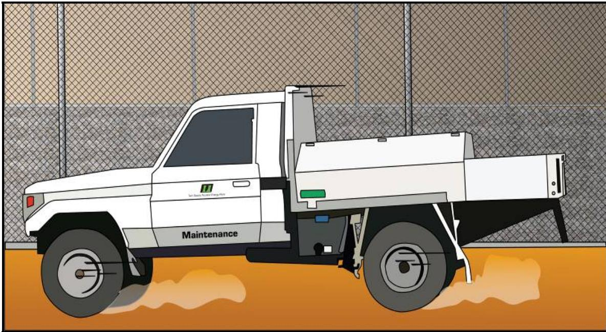
**Figure 19:** Sources of nuisance alarms for ported coaxial cable detection systems include nearby moving vehicles, larger animals, large and wet plants moving in the wind, and moving water, as well as the ripples caused by wind blowing across standing water.
