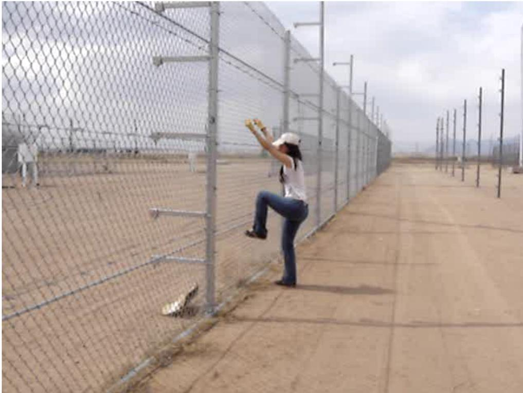
**Figure 35: Test climbing the fence from the outer (unprotected) side.**
