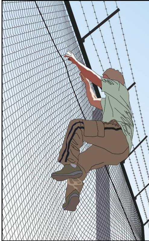
**Figure 31: This diagram illustrates the deflection caused by climbing on chain-link fence fabric; this disturbance of the fabric is one of the ways that fence disturbance sensors work.**
