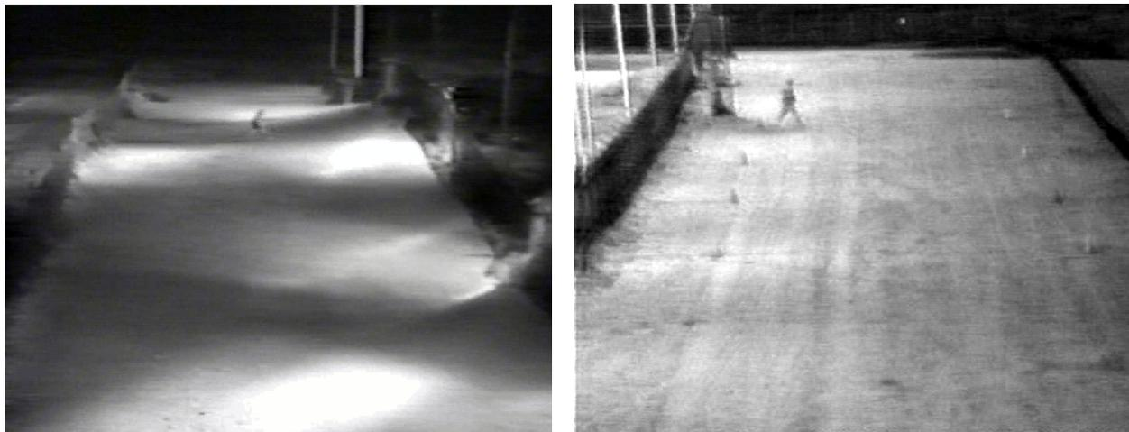
**Figure 74:** *The scene at left has a high light-to-dark ratio of approximately 20:1, which is not considered sufficient. The scene at right has a low light-to-dark ratio of approximately 4:1, which maximizes the ability to assess an alarm.*
