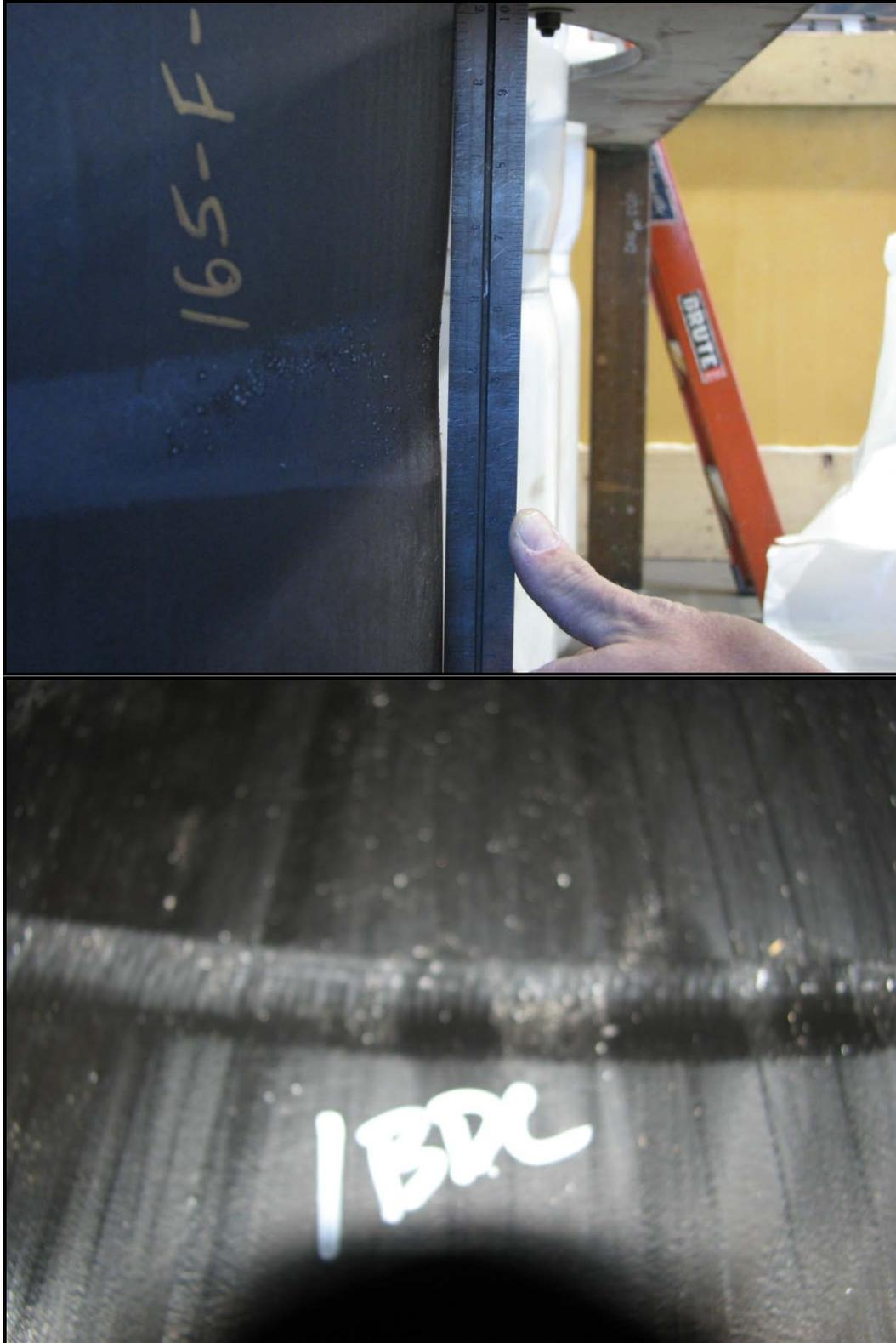
**Figure 5.1-17 – Hot Drop Body Pipe Dents and Gouges**
