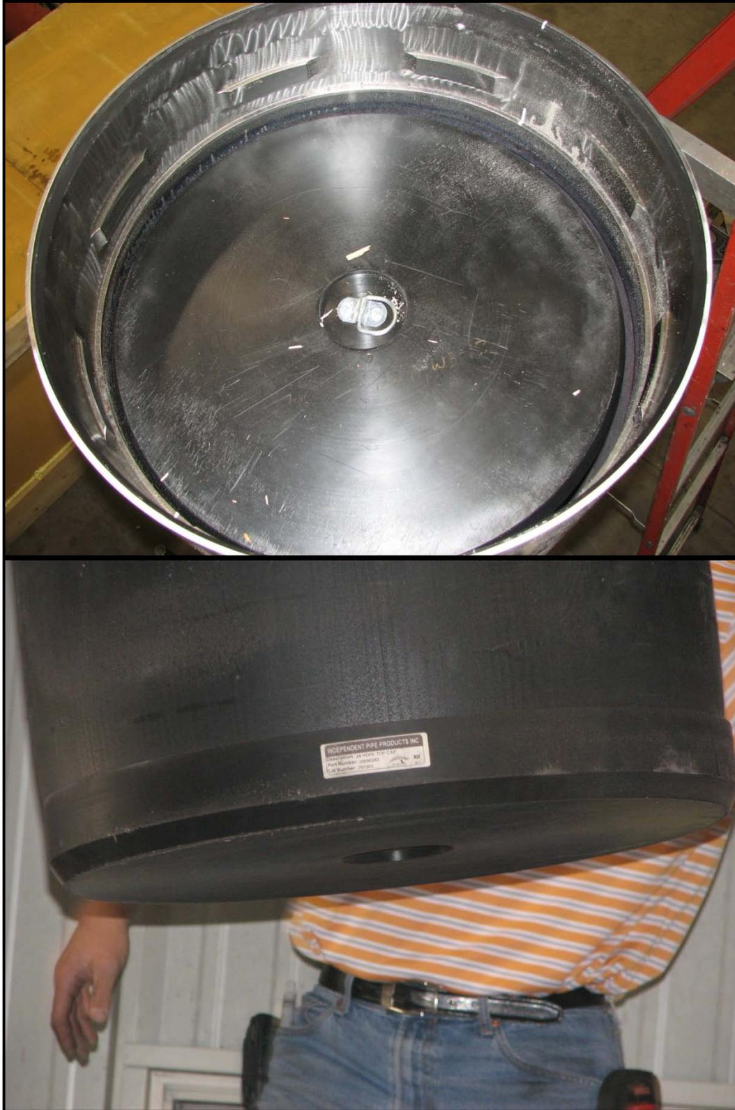
**Figure 5.1-16 – Hot Drop End Cap and Body Pipe Engagement**
