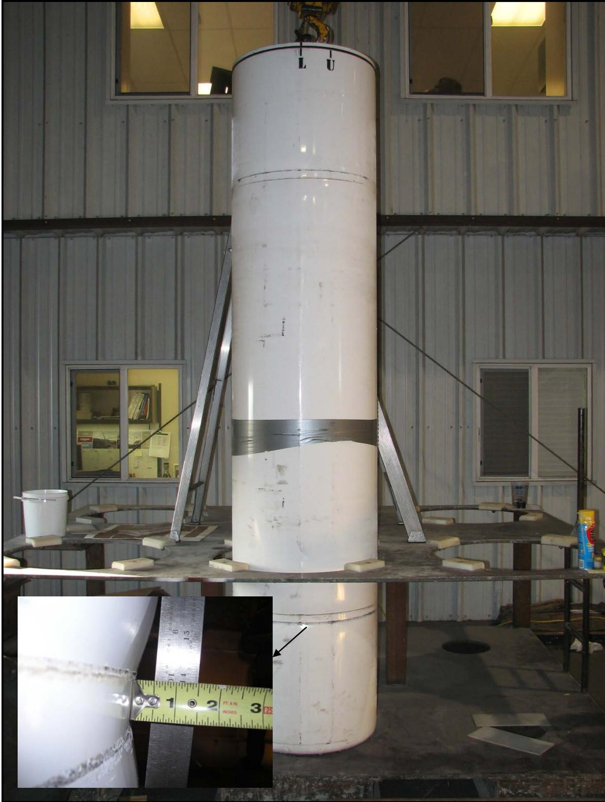
**Figure 5.1-12 – Cold Drop Canister Metallic Component Deformations**
