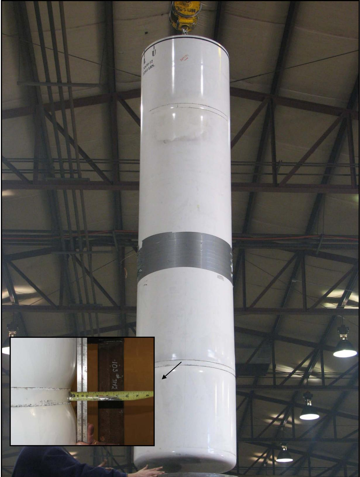
**Figure 5.1-18 – Hot Drop Canister Metallic Component Deformations**
