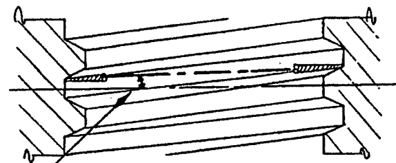
FIG. 4 INTERNAL MAJOR DIAMETER (NOTE DIAMETER MEASURED WITH MINIMUM ANGULARITY)
