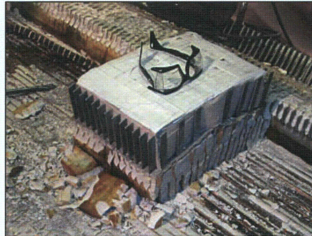
»SAMPLE N°1 »DELIMITATION DURING FINS + RESIN REMOVAL
