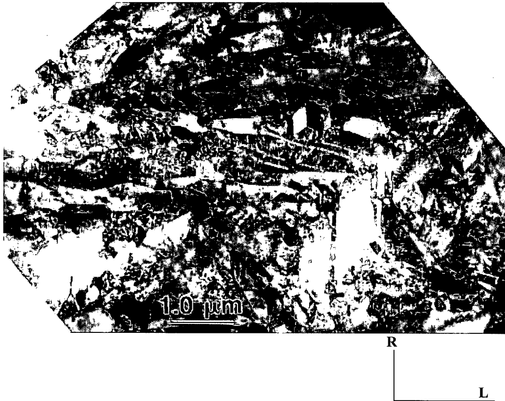
Fig.3.5. Microstructure of RBMK pressure tube with TMT-1 treatment.
