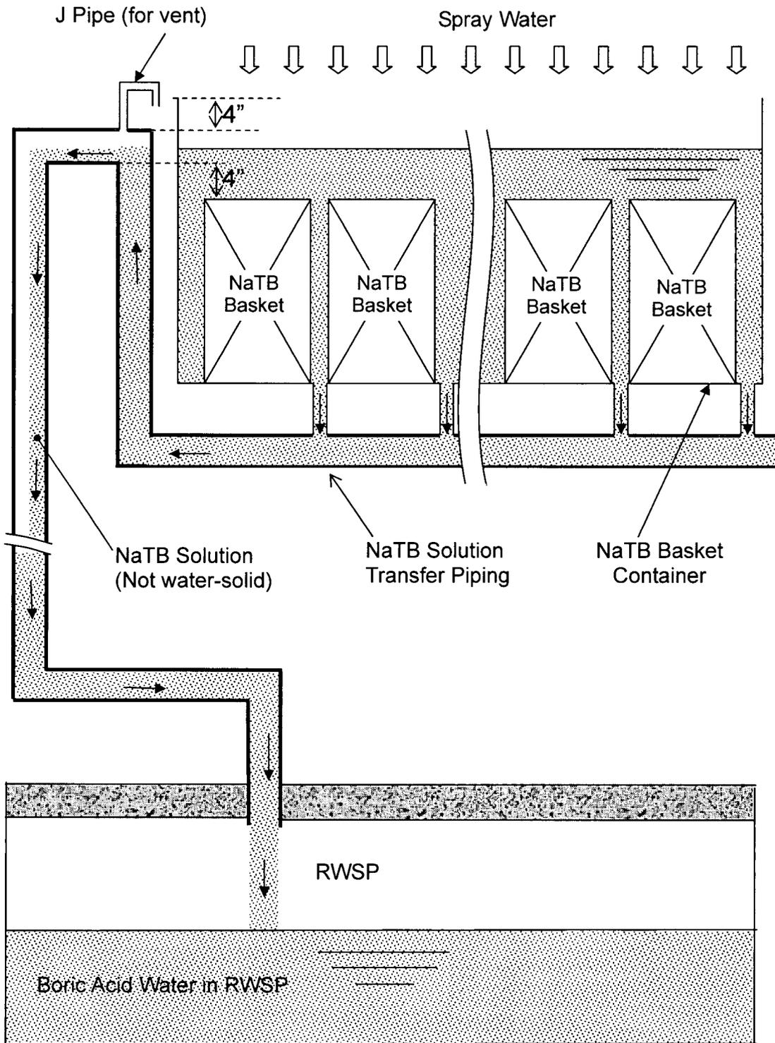
RAI Figure 6.3.88-4 NaTB Solution Flow during an Accident
