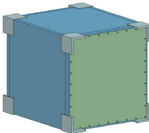
The proposed Transport System consists of the IP-2 packaging, which is used to contain the Class 7 (radioactive) materials and a Transportation and Emergency Response Plan.
