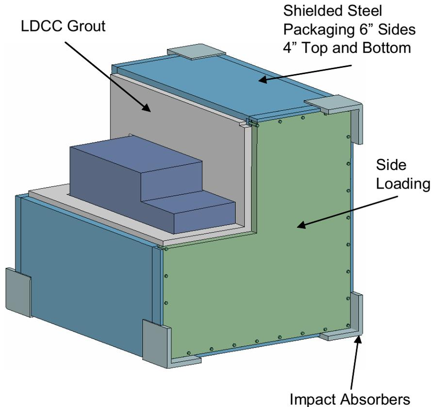
The container has an overall envelope dimension of 14' 11" long x 12' 8" wide x 12' 6" high with box dimensions of 13' 5" long x 12' 6" wide x 12' 4" high. It has a removable side cover as shown on Figure 1-2. The side cover is recessed into the container. It is sealed with a neoprene gasket and bolted in place with thirty six (36) 1-1/2 inch diameter bolts.
