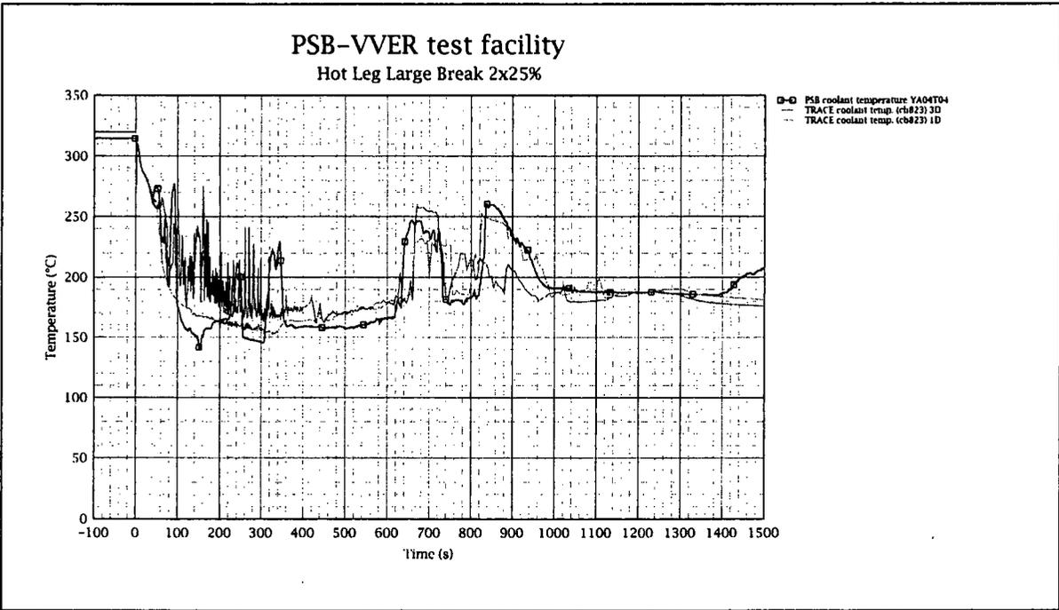
Figure 15: Intact Loop 4 Temperatures (Inlet of SG3)
