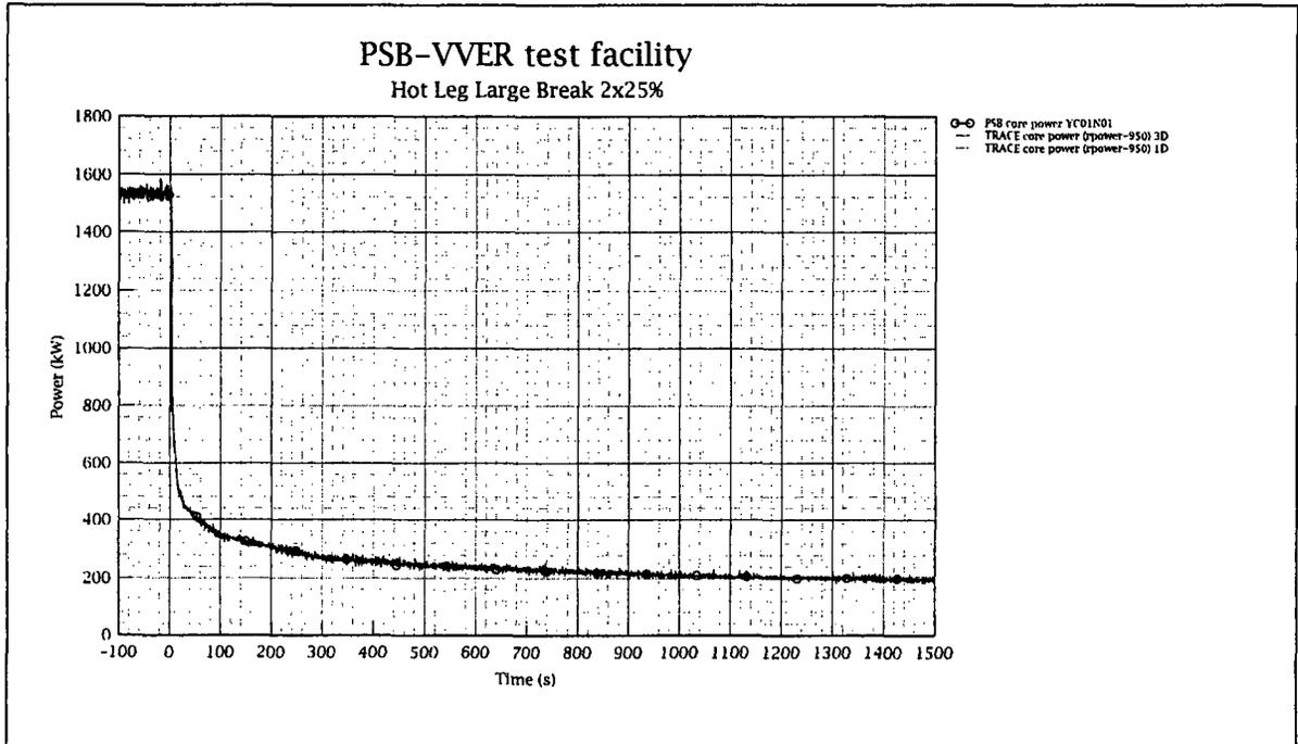
Figure 10: Fuel Rod Simulator Power (Boundary Condition)
