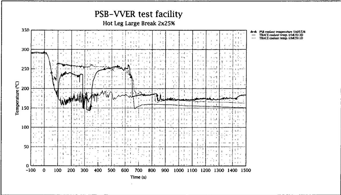
Figure 16: Intact Loop 4 Temperatures (Loop Seal)
