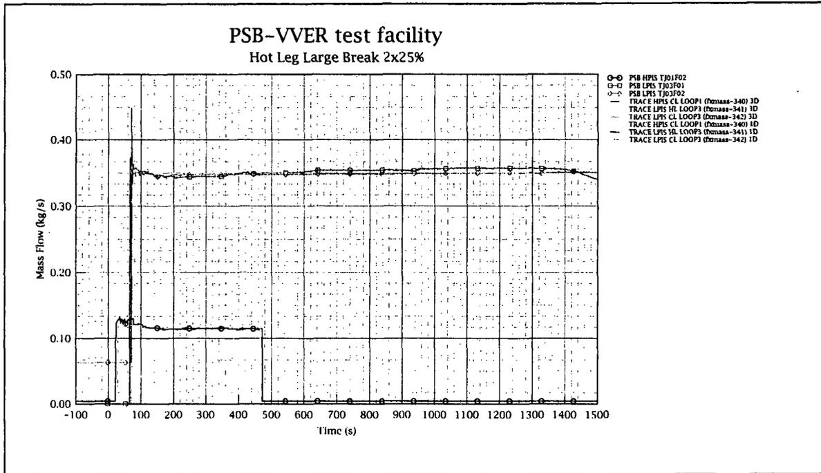
Figure 7: HPIS + LPIS Flow (Boundary Condition)
