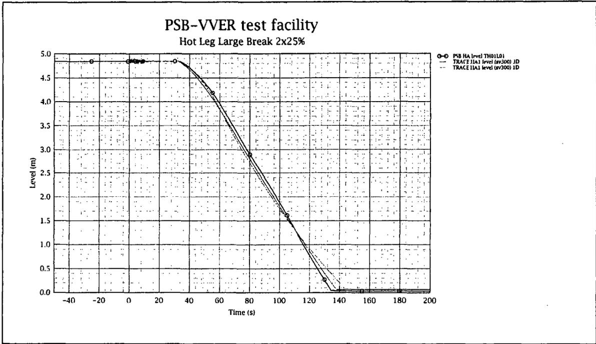
Figure 9: Hydroaccumulators Levels
