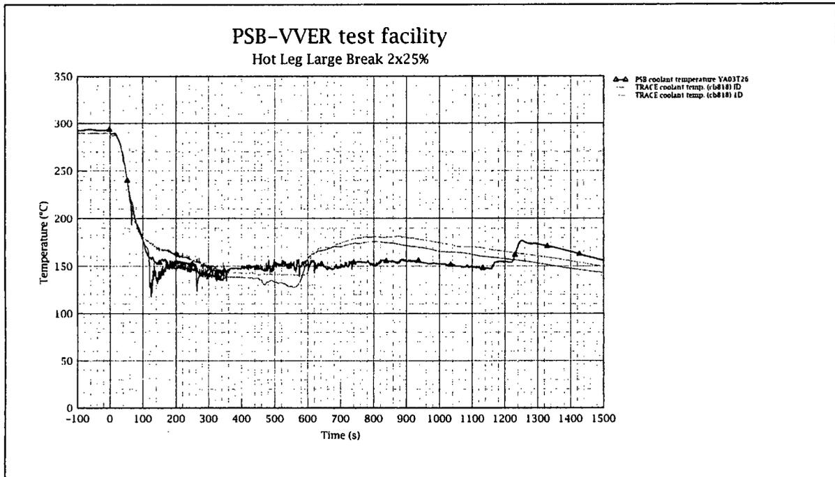
Figure 14: Broken Loop 3 Temperatures (Loop Seal)
