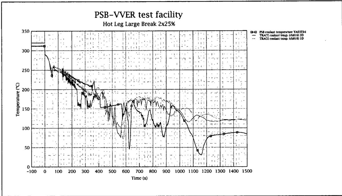
Figure 13: Broken Loop 3 Temperatures (Inlet of SG3)
