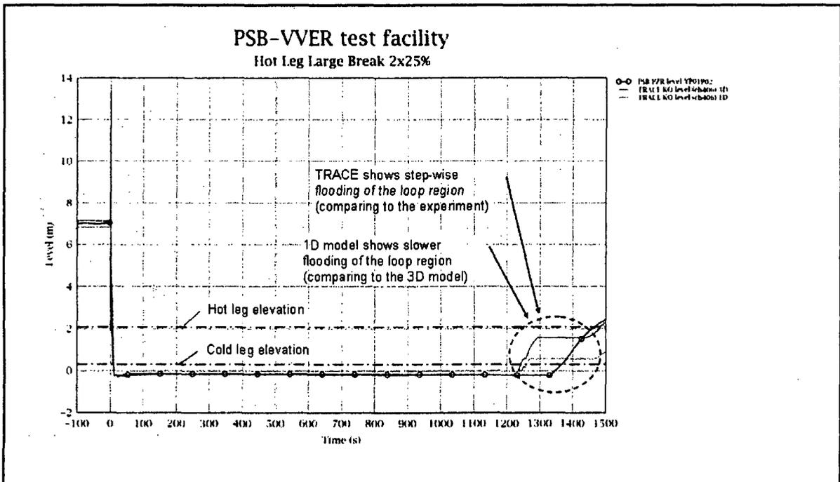
Figure 6: Pressurizer Level
