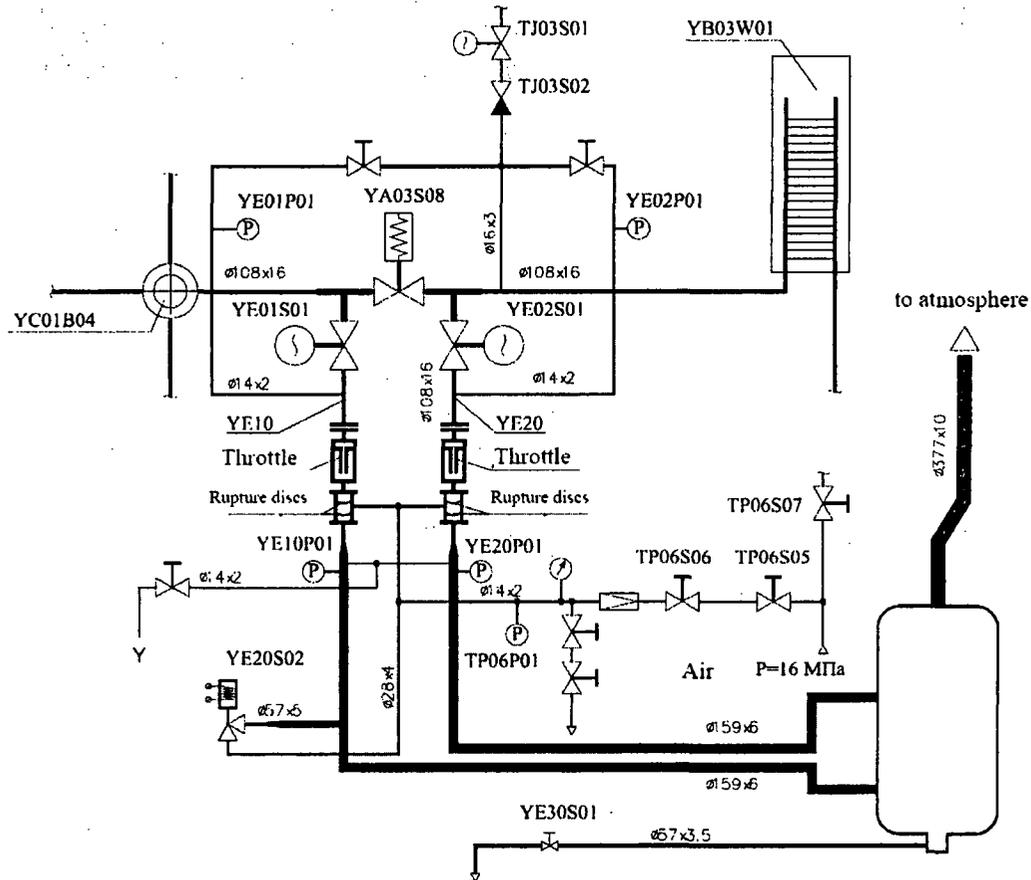
Figure 2: Principal Scheme of PSB-VVER Large Break Unit
