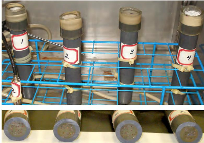
**Figure 2-9. Posttest Photographs of the Test 1 Carbon Steel Probes**
