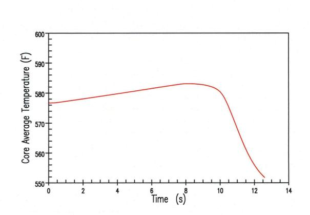
Core Coolant Average Temperature Transient for an Uncontrolled RCCA Bank Withdrawal from Full Power With Maximum Reactivity Feedback (75 pcm/s)
