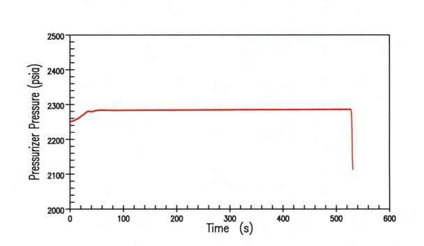
Pressurizer Pressure Transient for an Uncontrolled RCCA Bank Withdrawal from Full Power With Maximum Reactivity Feedback (3 pcm/s)
