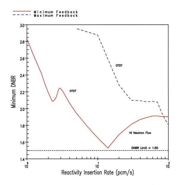
Minimum DNBR Versus Reactivity Insertion Rate for Rod Withdrawal at 60-percent Power
