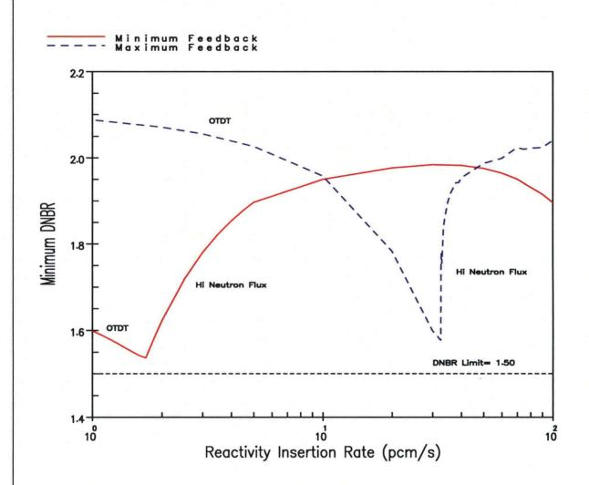
Minimum DNBR Versus Reactivity Insertion Rate for Rod Withdrawal at 100-percent Power
