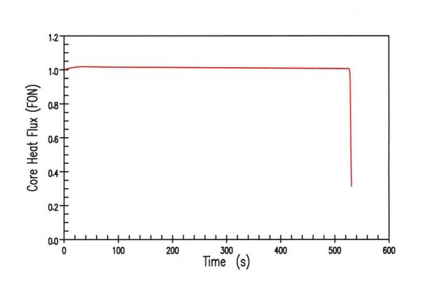
Thermal Flux Transient for an Uncontrolled RCCA Bank Withdrawal from Full Power With Maximum Reactivity Feedback (3 pcm/s)
