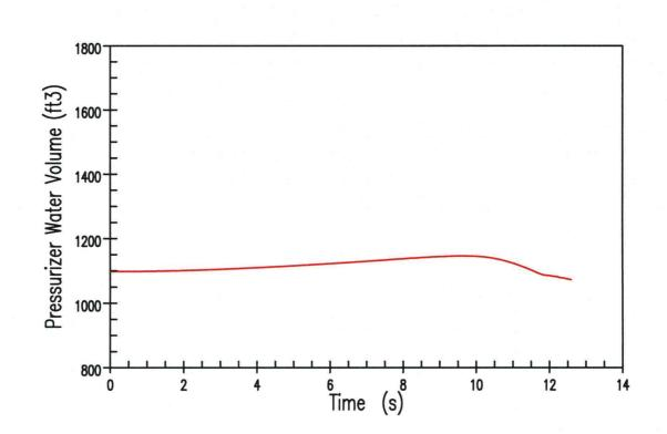
Pressurizer Water Volume Transient for an Uncontrolled RCCA Bank Withdrawal from Full Power With Maximum Reactivity Feedback (75 pcm/s)
