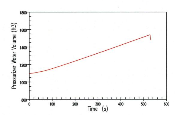
Pressurizer Water Volume Transient for an Uncontrolled RCCA Bank Withdrawal from Full Power With Maximum Reactivity Feedback (3 pcm/s)
