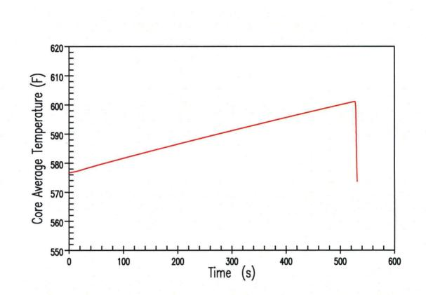
Core Coolant Average Temperature Transient for an Uncontrolled RCCA Bank Withdrawal from Full Power With Maximum Reactivity Feedback (3 pcm/s)
