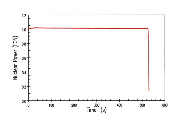
Nuclear Power Transient for an Uncontrolled RCCA Bank Withdrawal from Full Power With Maximum Reactivity Feedback (3 pcm/s)
