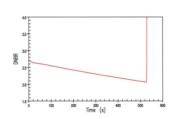
DNBR Transient for an Uncontrolled RCCA Bank Withdrawal from Full Power With Maximum Reactivity Feedback (3 pcm/s)
