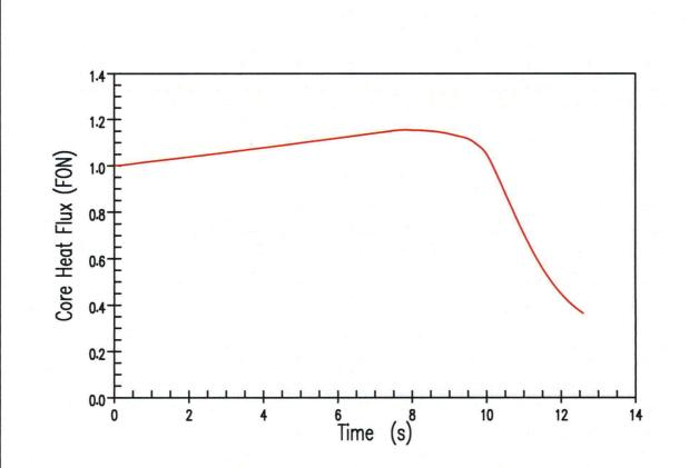
Thermal Flux Transient for an Uncontrolled RCCA Bank Withdrawal from Full Power With Maximum Reactivity Feedback (75 pcm/s)
