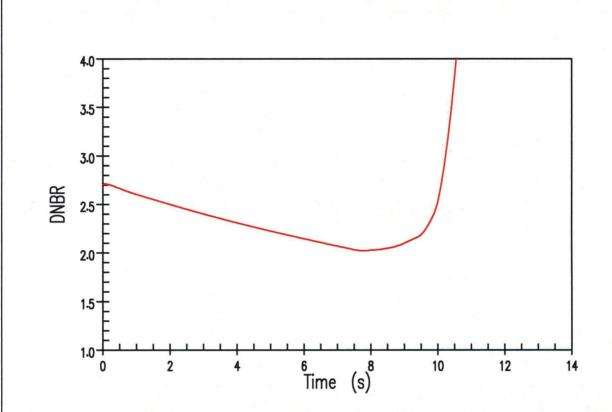
DNBR Transient for an Uncontrolled RCCA Bank Withdrawal from Full Power With Maximum Reactivity Feedback (75 pcm/s)
