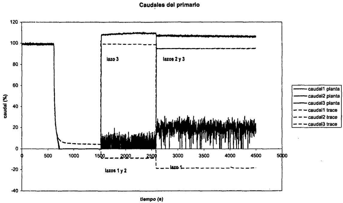
**Figure 11. Primary (mass and volume) flow rates**
