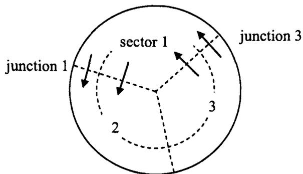
**Figure 20. Sketch of the nomenclature followed in the VESSEL component (arrows represent positive directions)**
