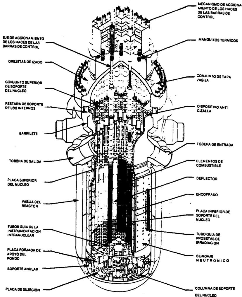
Figure 1. Outline of the inner part of the reactor vessel.
