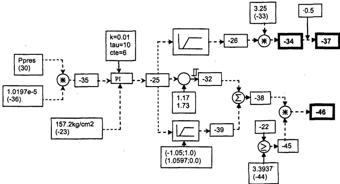
Figure 8. Diagram of the pressurizer pressure control
