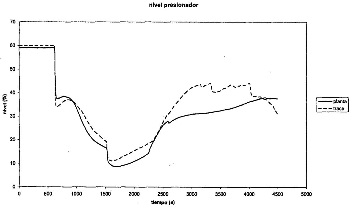
**Figure 14. Pressurizer level**
