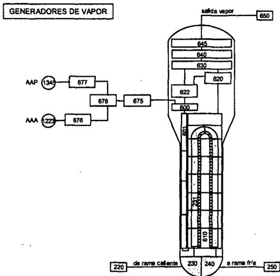
**Figure 6.** Drawing of the hydrodynamic model of the steam generators
