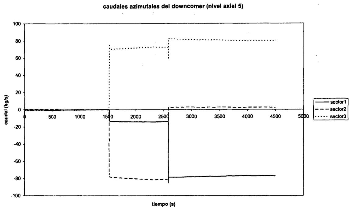
**Figure 17. Azimuthal downcomer flows in axial level 5**
