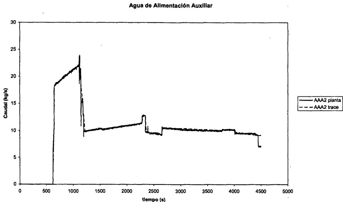
**Figure 9. Auxiliary Feed Water mass flow rate**
