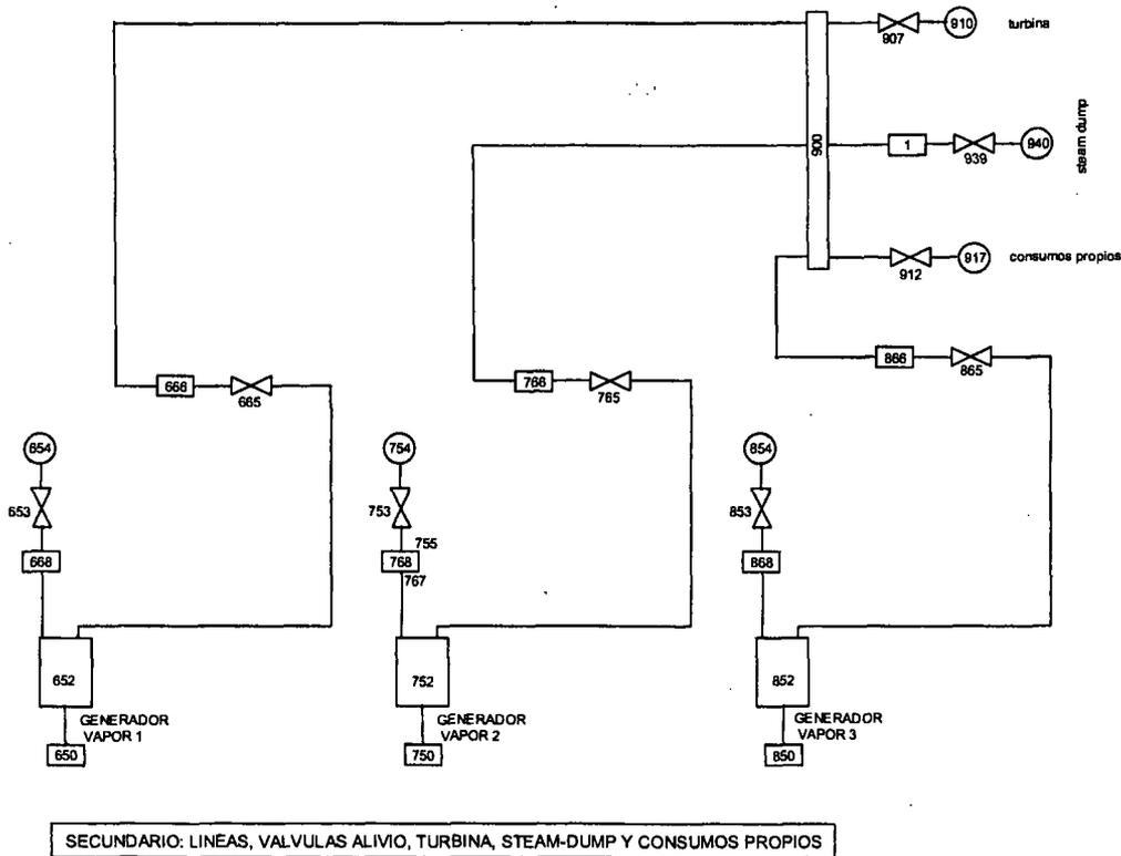
Figure 7. Sketch of the simulation of secondary system lines in the CNV II model.
