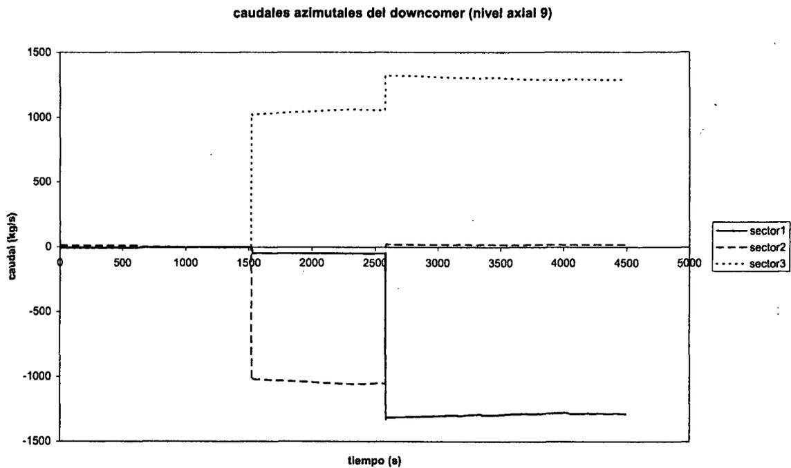
**Figure 19. Azimuthal downcomer flows in axial level 9**
