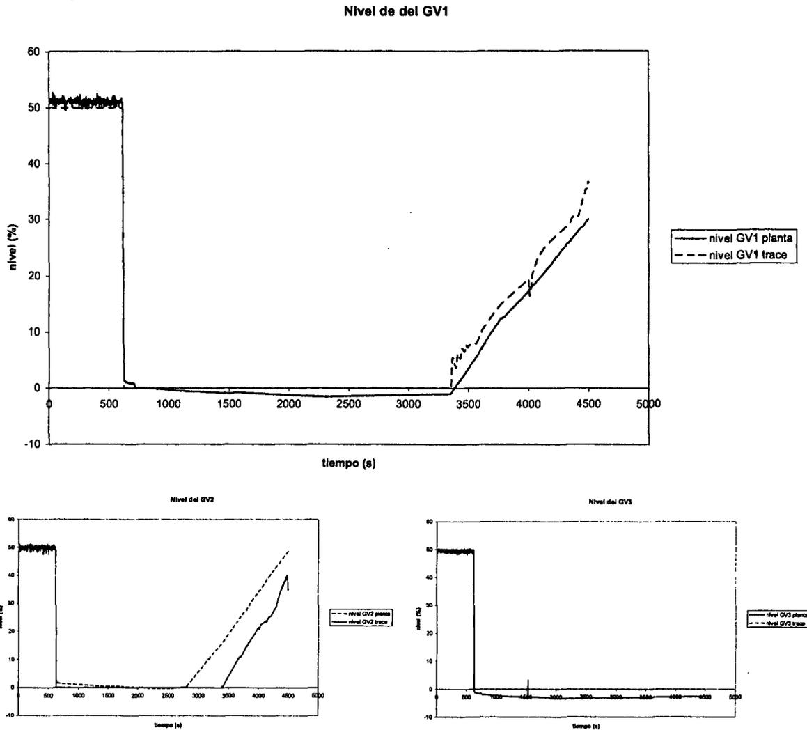
**Figure 16. Steam generators level**
