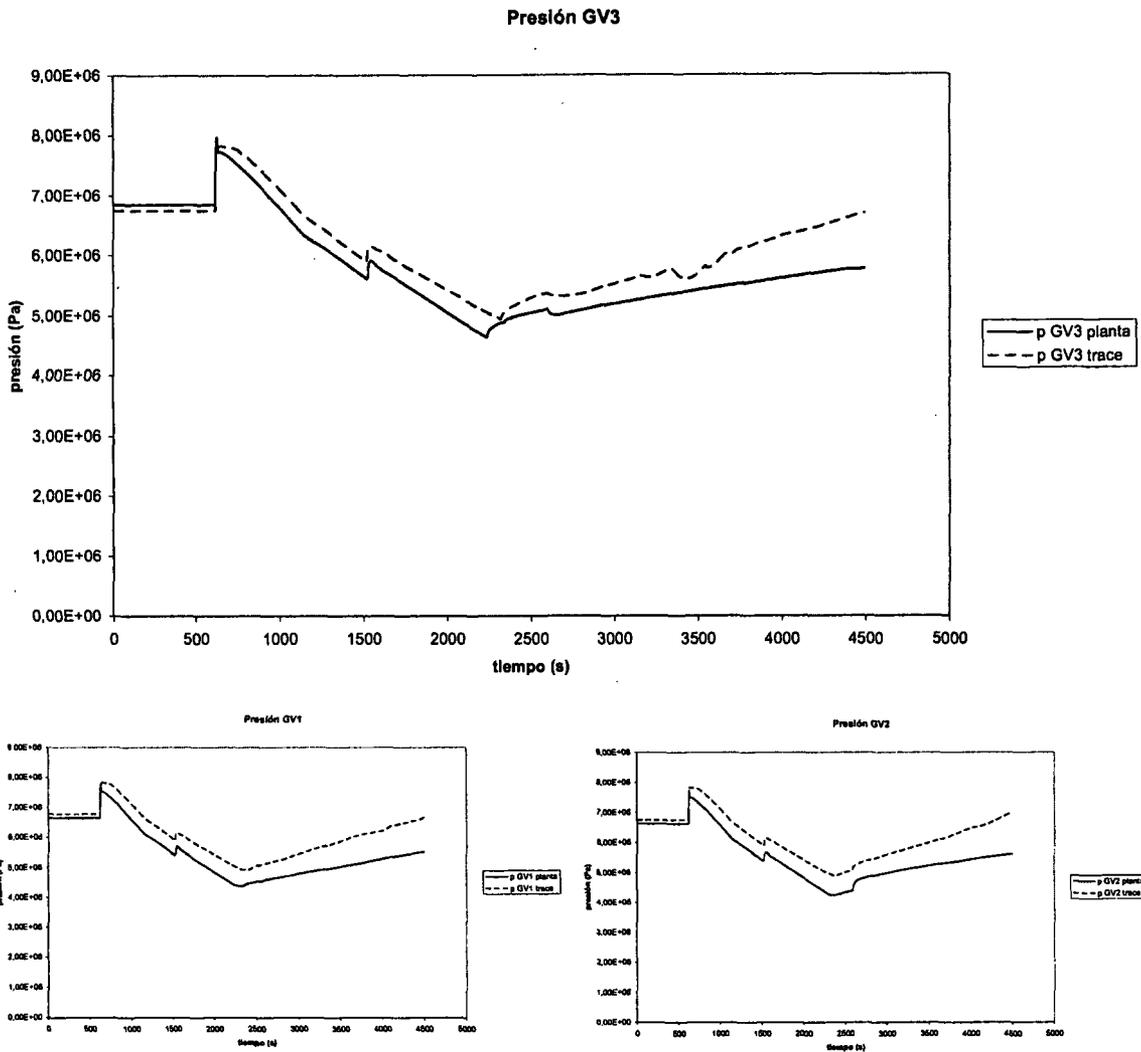
**Figure 15. Secondary pressure (SG)**
