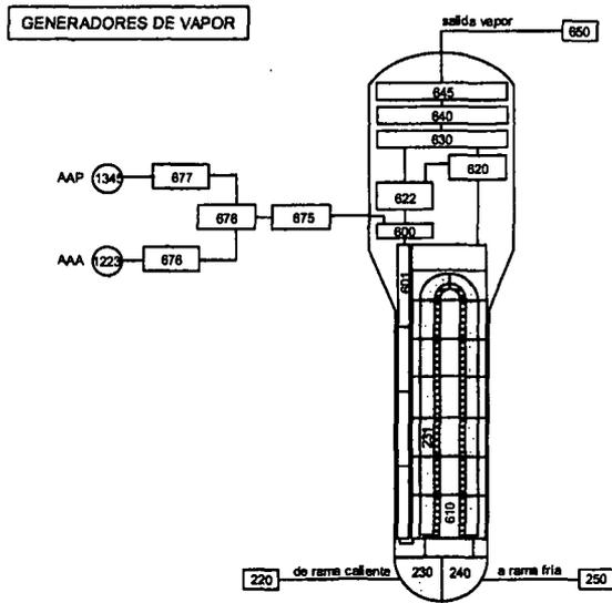
**Figure 5.** Represents the hydrodynamic model of one SG. The three steam generators are identical.
