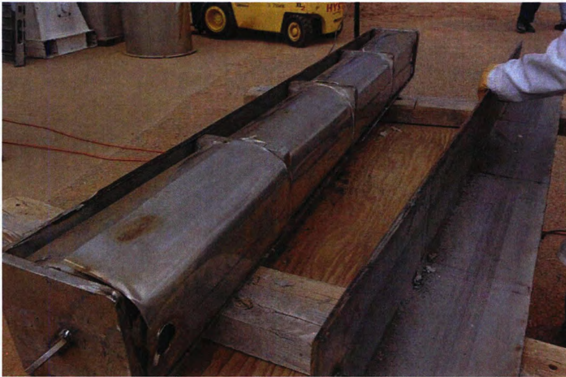
Figure 2.12.1-48 - Exposure of Thermal Shield
