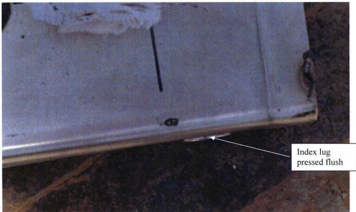
Figure 2.12.1-38 - Side View of CTU Following CD2.C-1 Drop
