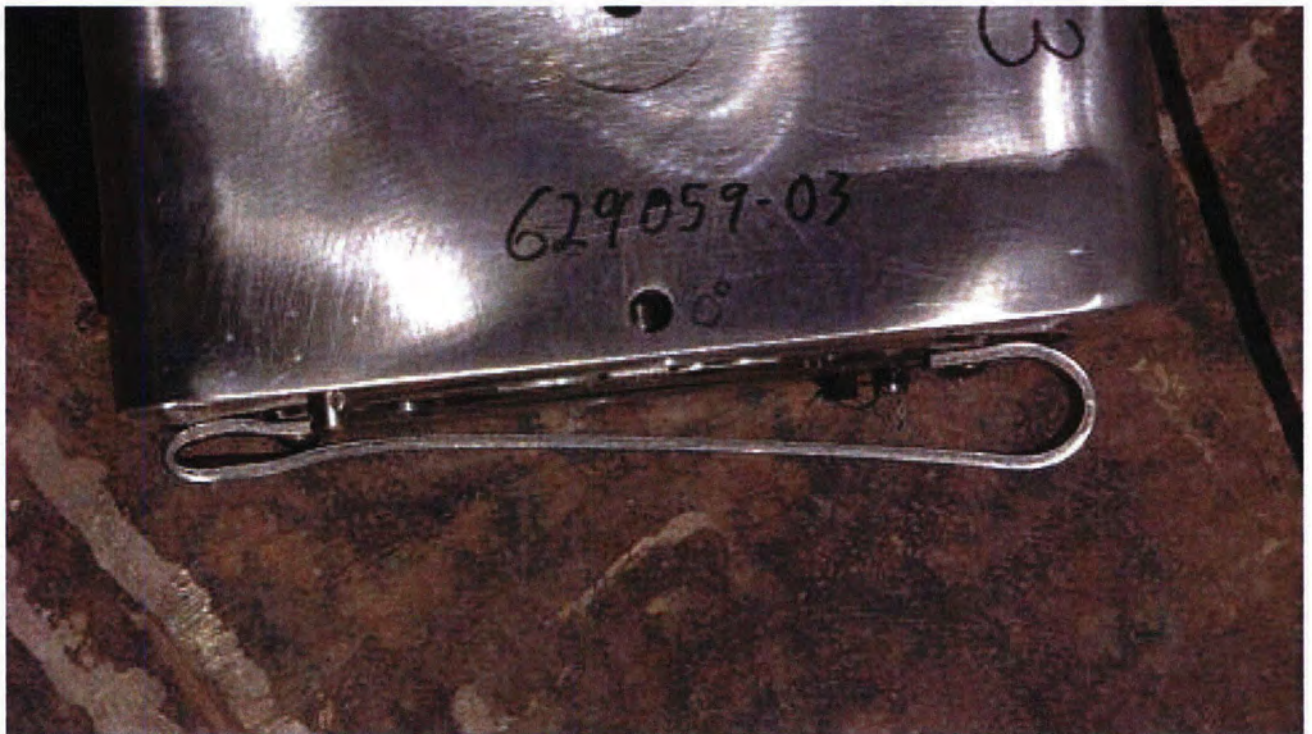
Figure 2.12.1-7 - CN1-1 Impact on Closure Handle
