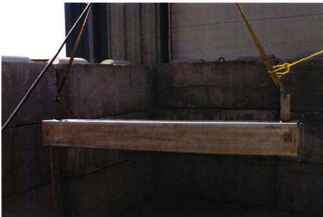
Figure 2.12.2-8 - CD3-2 Drop Orientation
