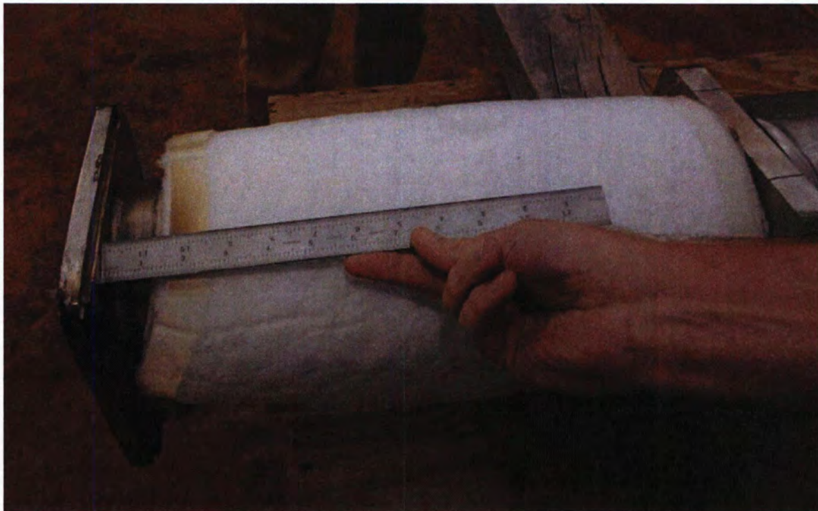
Figure 2.12.1-49 - Insulation After Removal of Thermal Shield
