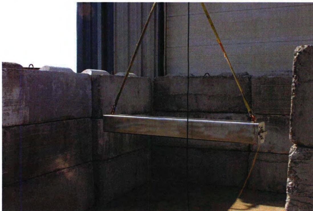
Figure 2.12.2-5 - CD1-2 Drop Orientation
