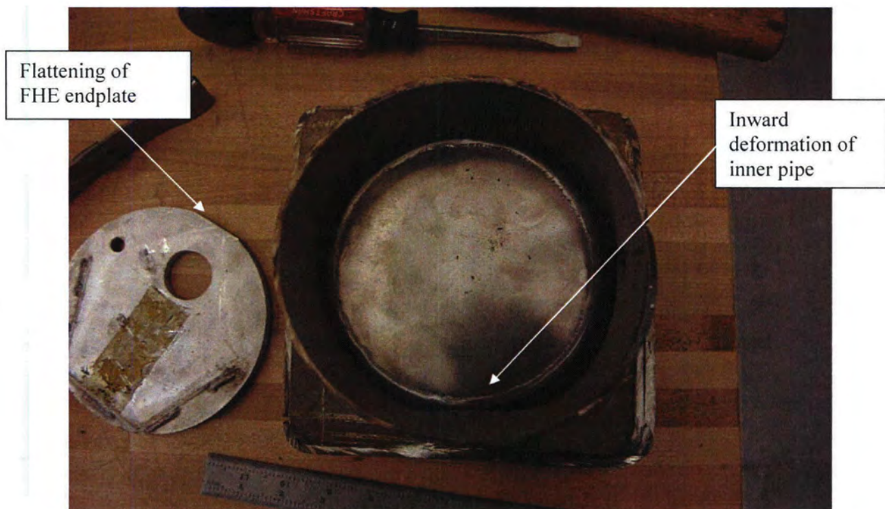
Figure 2.12.1-53 - Inner Tube Deformation at Closure End
