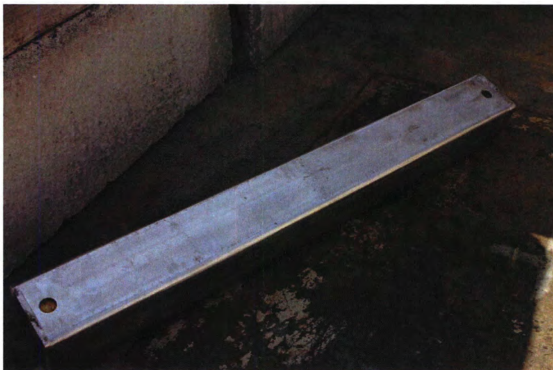
Figure 2.12.2-6 - CTU Following CD1-2 Impact (impact side facing up)
