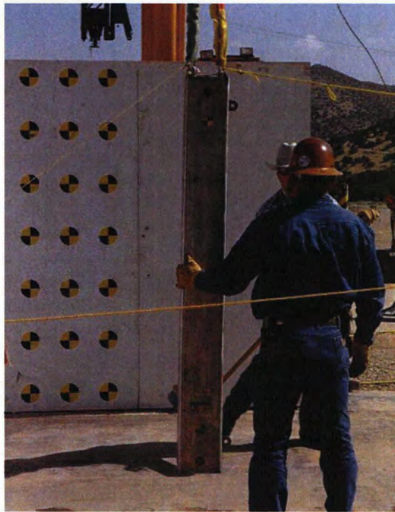
Figure 2.12.1-26 - CD4-1 Drop Orientation
