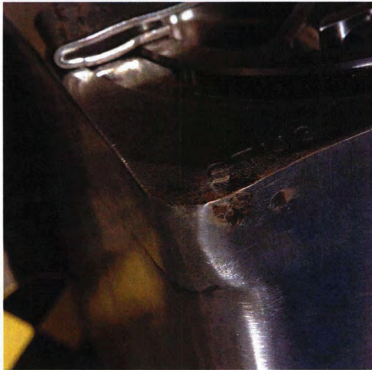
Figure 2.12.1-6 - CN1-1 Impact Damage
