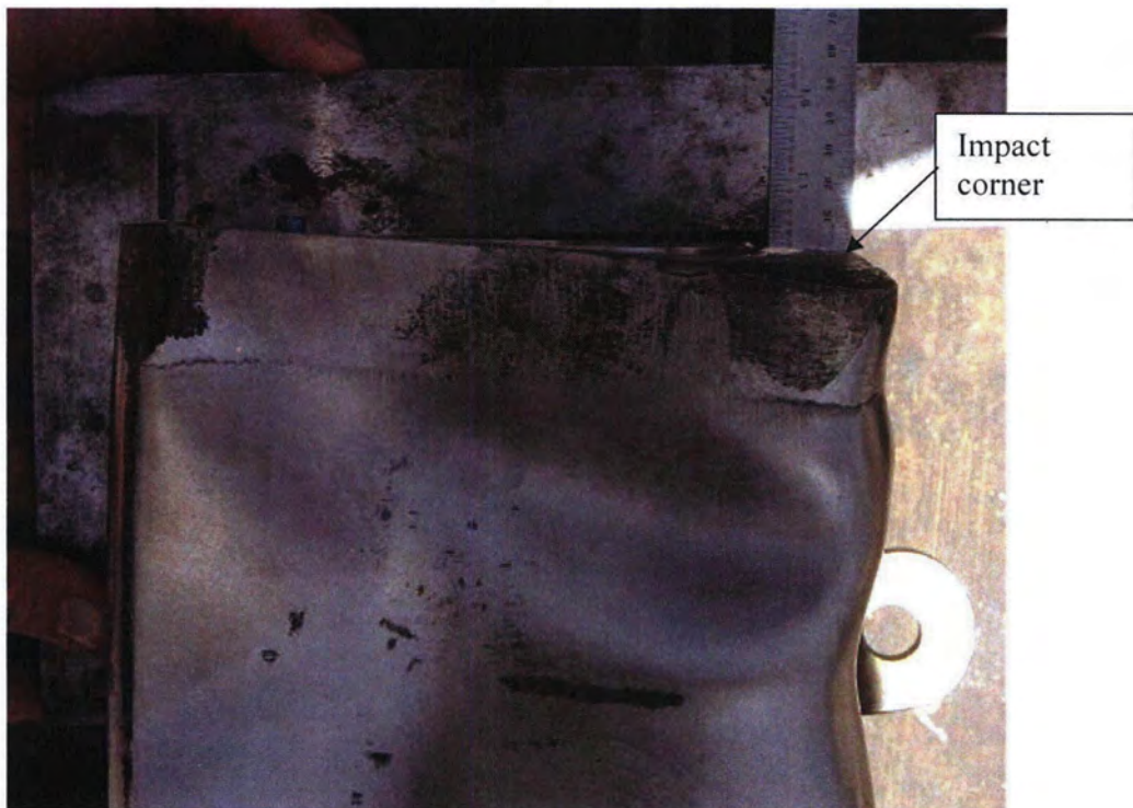
Figure 2.12.1-35 - CD5-1 Impact Damage on Closure End
