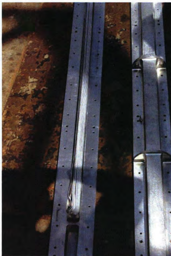
Figure 2.12.2-15 - CD4-2 Impact Damage to Simulated Fuel Plates
