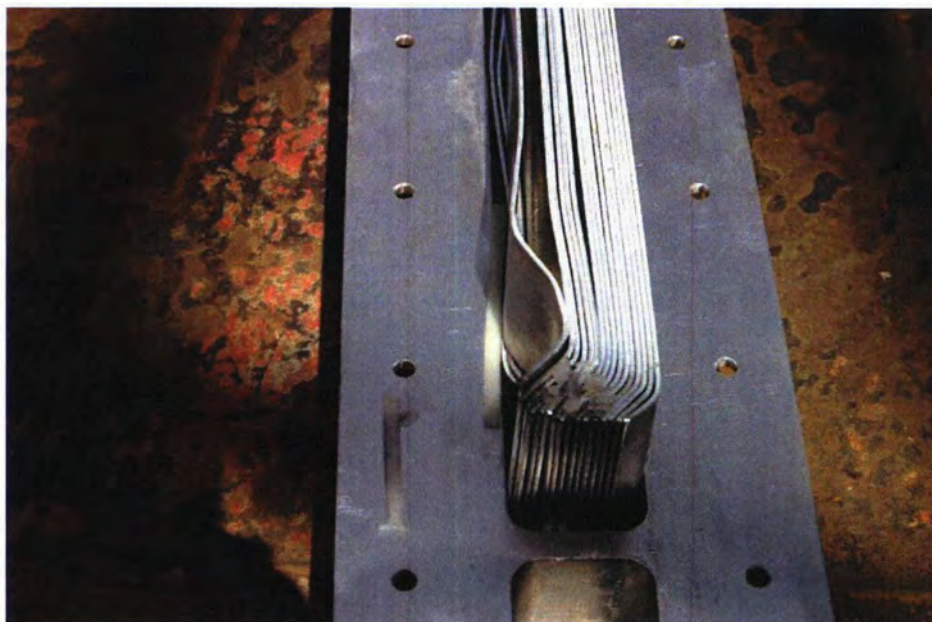
Figure 2.12.2-16 - CD4-2 Impact Damage to Simulated Fuel Plates (close up view)
