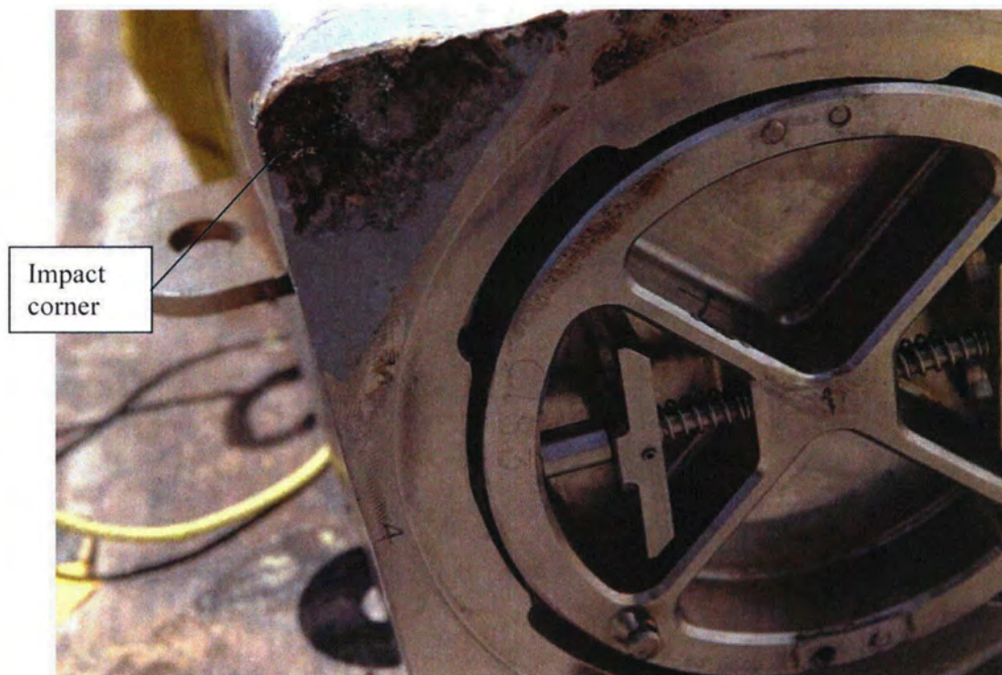
Figure 2.12.1-36 - CD5-1 Impact Damage on Closure Area
