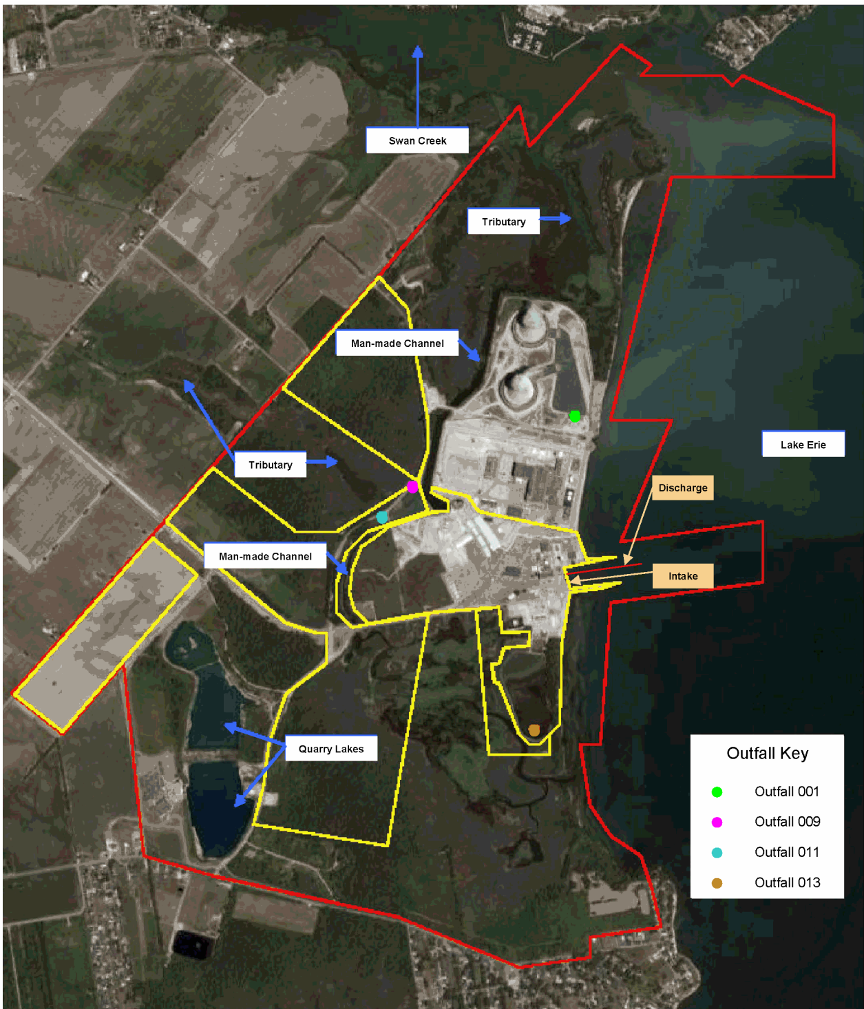
Figure 5.3-1 Station Layout with Intake, Discharge and Outfalls
