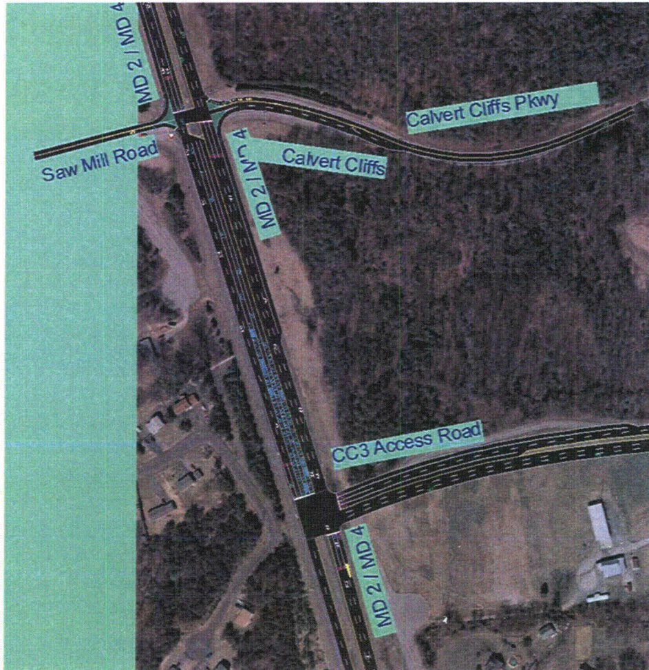
Figure 11 – Site Access Intersection – Triple Left Turn – Model Snapshot
