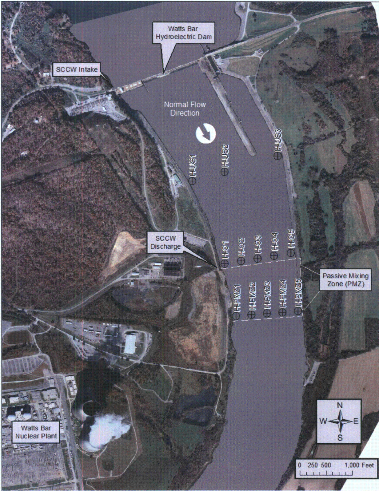
Figure 1. Locations of HOBOTemperature recorders along transects across from (H-O1, H-O2, H-O3, H-O4, H-O5), upstream (H-US1, H-US2, H-US3) and downstream (H-PMZ1, H-PMZ2, H-PMZ3, H-PMZ4, H-PMZ5) of the SCCW discharge.
