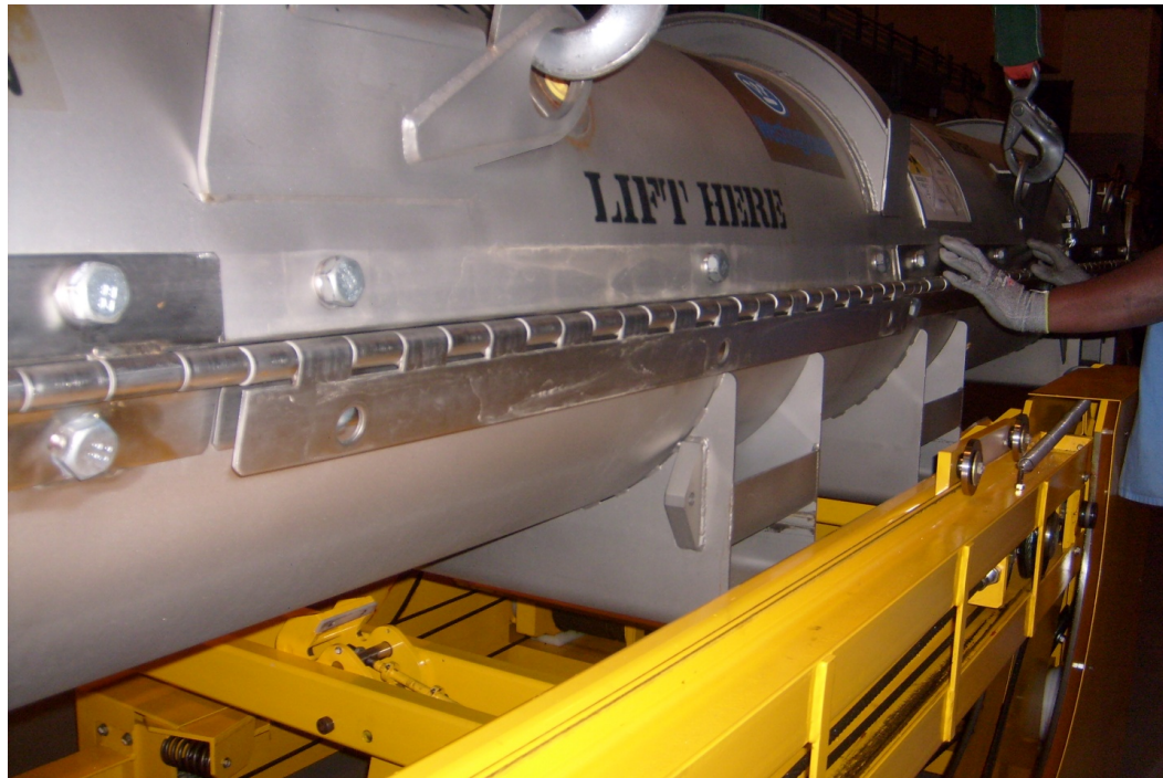
Figure 1 – TRAVELLER package closure hinge condition as transported
