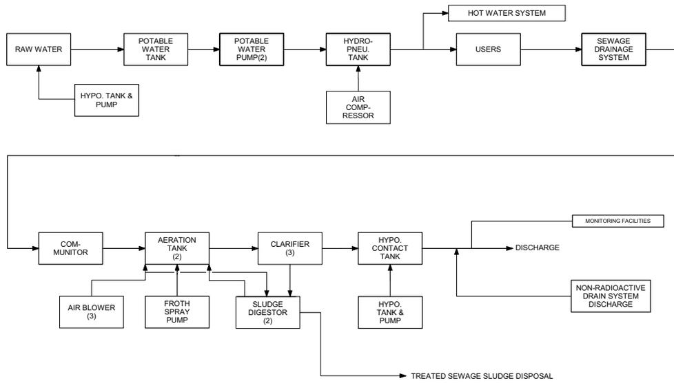
Figure 3.6-1 Potable and Sanitary Water System - Typical
