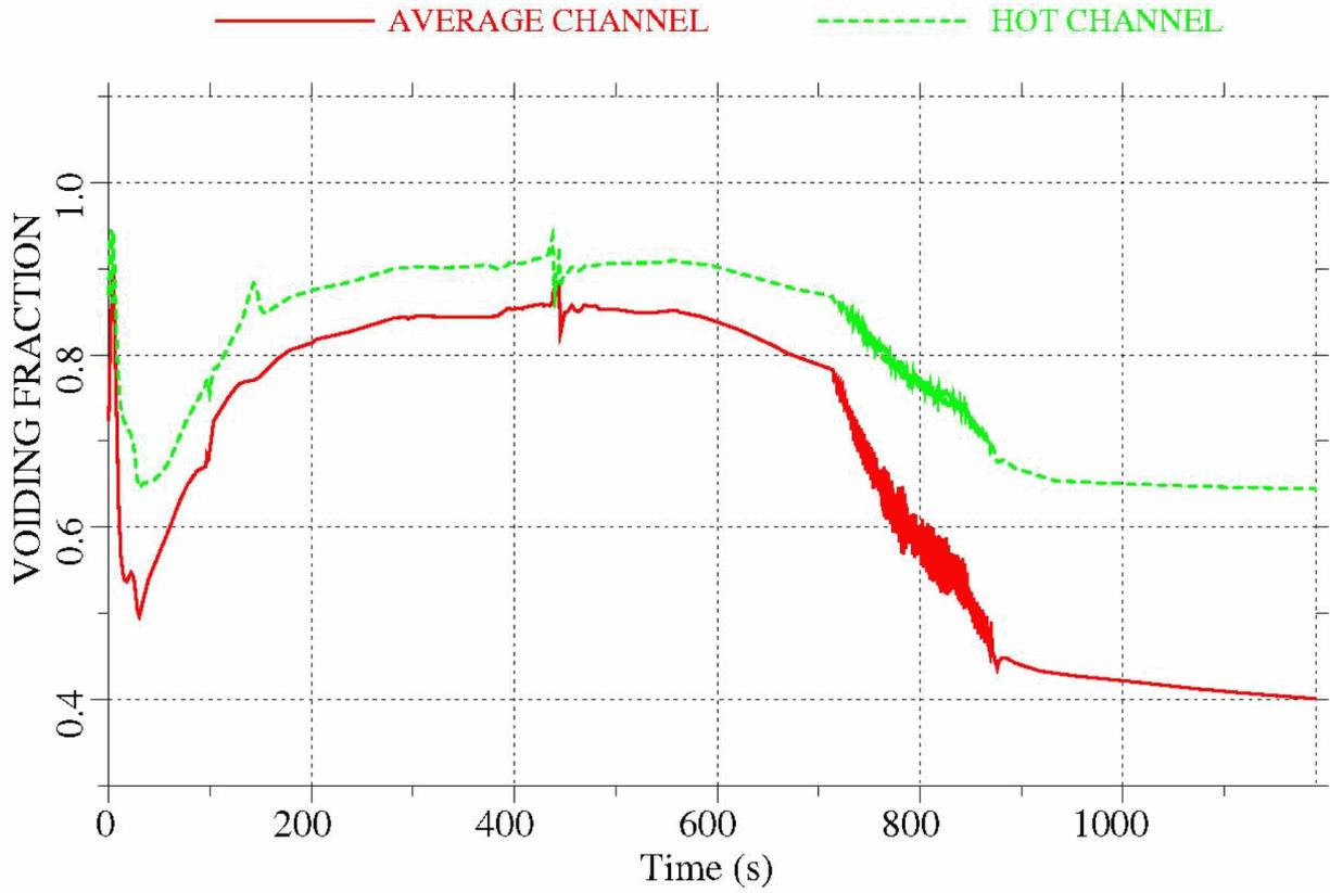
Figure 6C-4a Void Fraction for Unblocked Case
