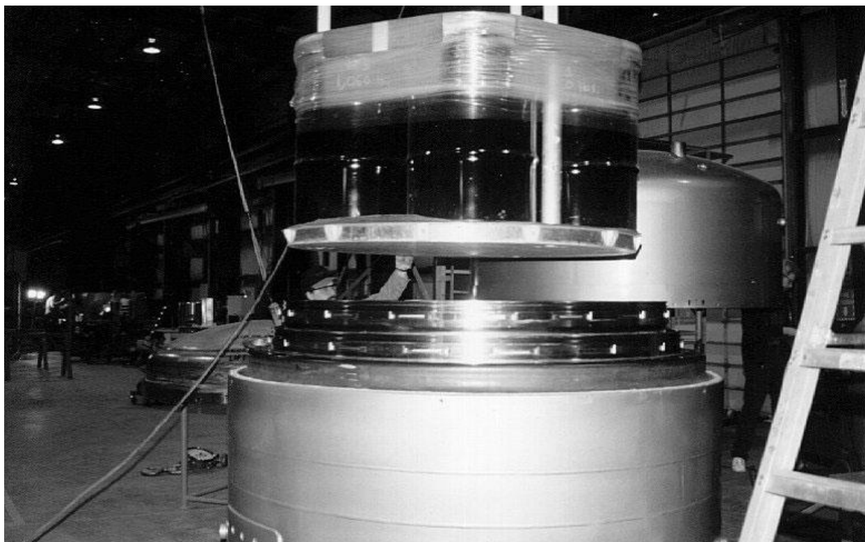
Figure 2.10.3-52 – CTU; Aligning 55-Gallon Drum Payload Assembly for Installation into ICV
