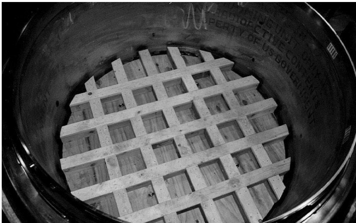
Figure 2.10.3-51 – CTU; 5 Inch Thick Payload Spacer (Wood Simulation) in Bottom of ICV
