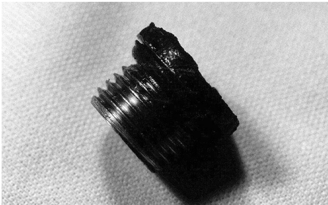
Figure 2.10.3-45 – ETU; View of OCV Seal Test Port Plug (As Removed; Not Cleaned)
