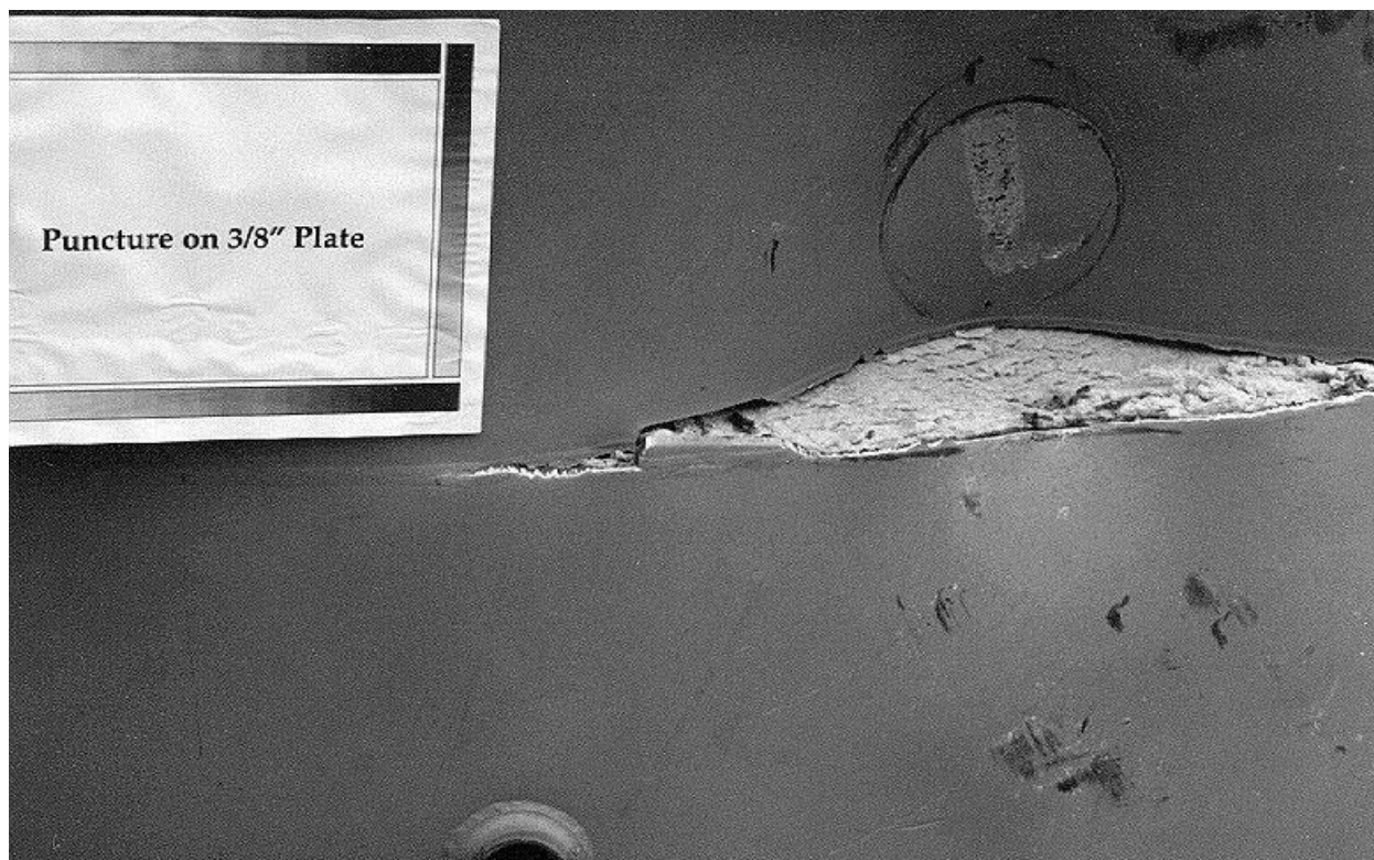
Figure 2.10.3-30 – ETU Puncture Drop Test 10; 3/8-to-1/4 Transition; ~27" Long Tear
