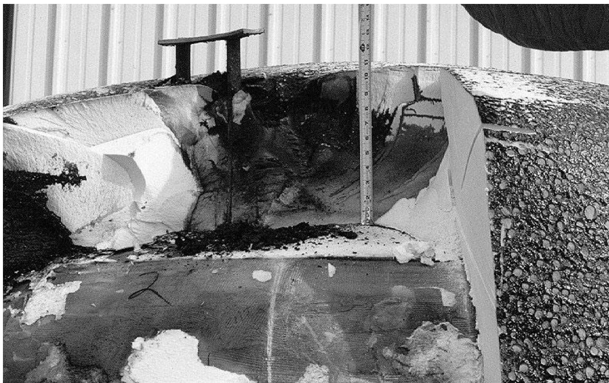
Figure 2.10.3-44 – ETU; Residual Foam in OCA Lid Top (~11")
