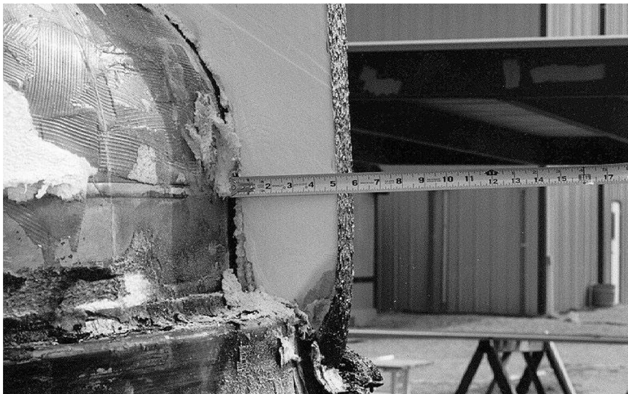
Figure 2.10.3-43 – ETU; Residual Foam in OCA Lid Side; Remote From Test Damage
