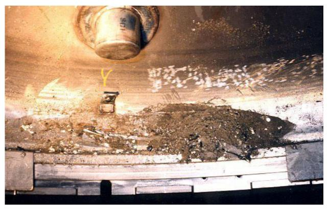
Figure 2.10.3-78 - CTU-2 Disassembly; Loose Debris in ICV Lid
