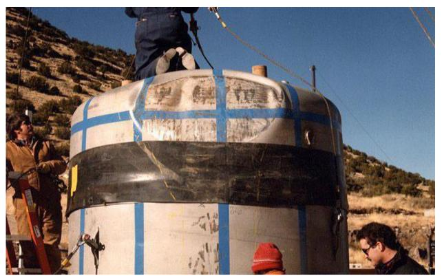
Figure 2.10.3-56 – CTU-2 Free Drop No. 1; Post-Drop Damage
