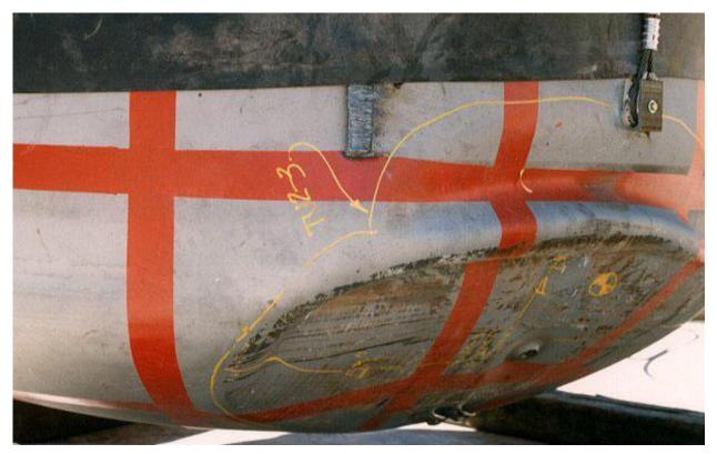
Figure 2.10.3-33 – CTU-1 Free Drop No. 3; Post-Drop Damage
