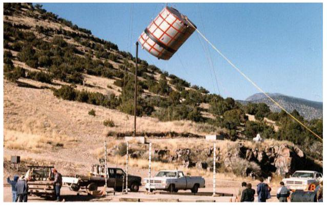
Figure 2.10.3-32 – CTU-1 Free Drop No. 3; Pre-Drop Positioning
