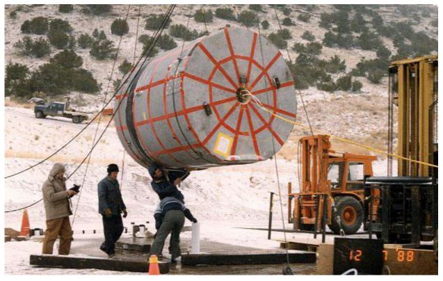
Figure 2.10.3-38 – CTU-1 Puncture Drop No. 6; Pre-Drop Positioning
