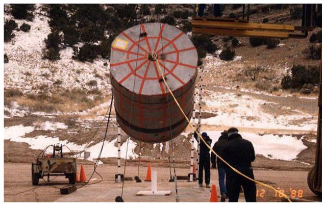
Figure 2.10.3-44 – CTU-1 Puncture Drop No. 9; Pre-Drop Positioning
