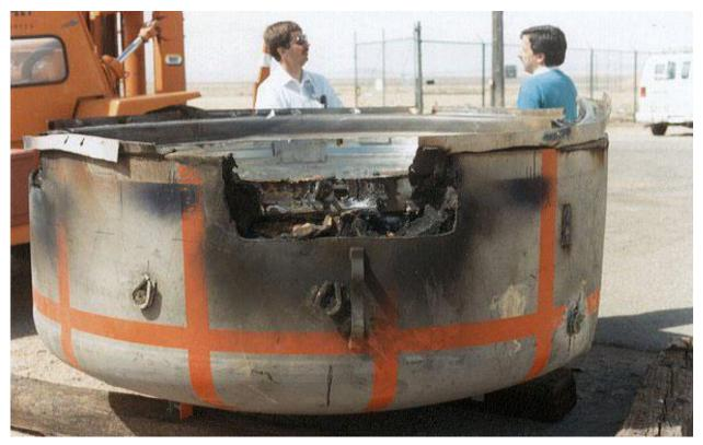
Figure 2.10.3-96 – CTU-3 Disassembly; OCA Lid
