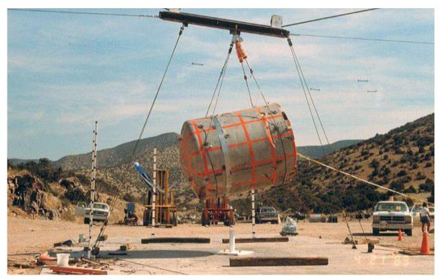
Figure 2.10.3-92 – CTU-3 Puncture Drop No. 7; Pre-Drop Positioning
