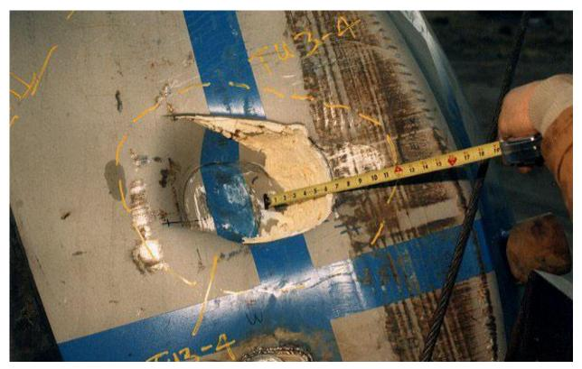
Figure 2.10.3-65 – CTU-2 Puncture Drop 4; Post-Drop Damage
