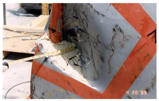
Figure 2.10.3-89 – CTU-3 Puncture Drop 5; Post-Drop Damage
