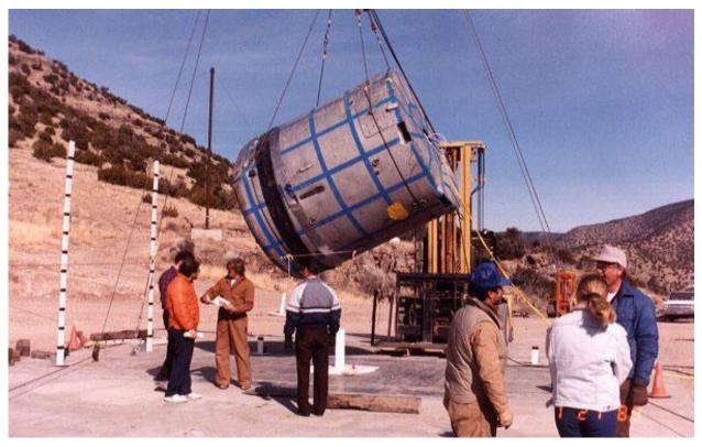
Figure 2.10.3-72 – CTU-2 Puncture Drop No. 8; Pre-Drop Positioning
