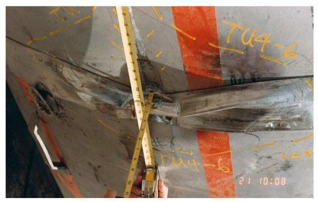
Figure 2.10.3-91 – CTU-3 Puncture Drop 6; Post-Drop Damage
