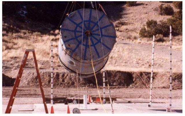
Figure 2.10.3-70 – CTU-2 Puncture Drop No. 7; Pre-Drop Positioning
