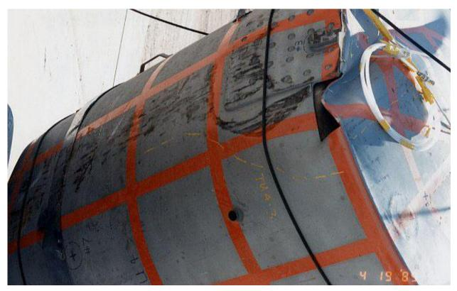
Figure 2.10.3-85 – CTU-3 Free Drop No. 3; Post-Drop Damage
