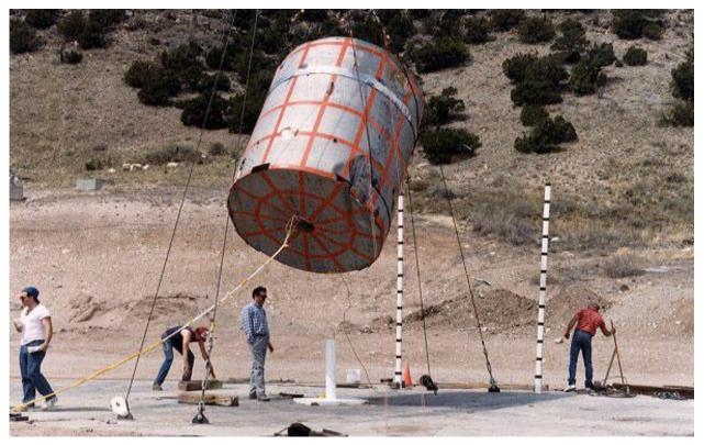
Figure 2.10.3-88 – CTU-3 Puncture Drop No. 5; Pre-Drop Positioning
