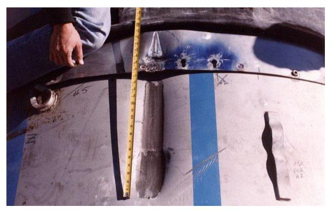
Figure 2.10.3-69 – CTU-2 Puncture Drop 6; Post-Drop Damage
