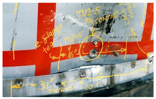
Figure 2.10.3-37 – CTU-1 Puncture Drop No. 5; Post-Drop Damage
