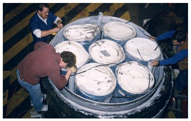
Figure 2.10.3-52 – CTU-1 Disassembly; Payload Drum Removal
