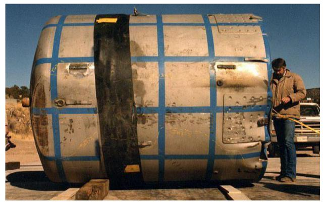
Figure 2.10.3-61 – CTU-2 Free Drop No. 3; Post-Drop Damage
