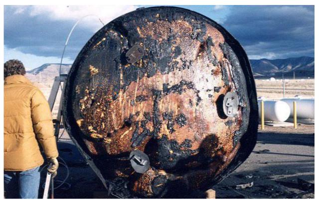
Figure 2.10.3-50 – CTU-1 Disassembly; OCA Lid Unburned Foam
