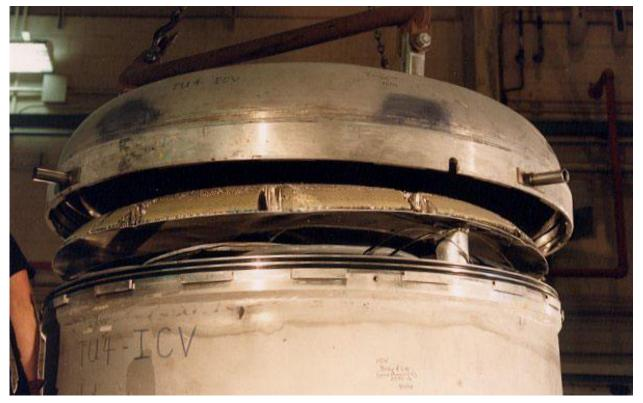
Figure 2.10.3-98 – CTU-3 Disassembly; ICV Lid Removal
