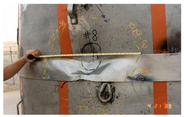
Figure 2.10.3-95 – CTU-3 Puncture Drop 8; Post-Drop Damage
