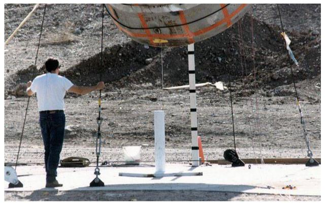
Figure 2.10.3-86 – CTU-3 Puncture Drop No. 4; Pre-Drop Positioning
