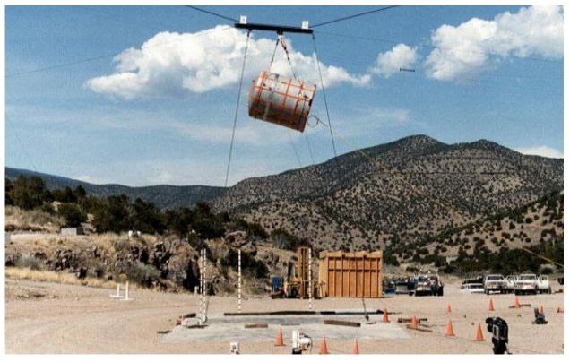
Figure 2.10.3-84 – CTU-3 Free Drop No. 3; Pre-Drop Positioning
