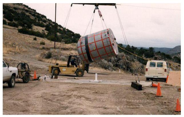
Figure 2.10.3-36 – CTU-1 Puncture Drop No. 5; Pre-Drop Positioning
