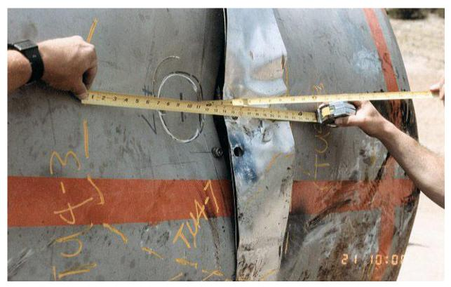
Figure 2.10.3-93 – CTU-3 Puncture Drop 7; Post-Drop Damage
