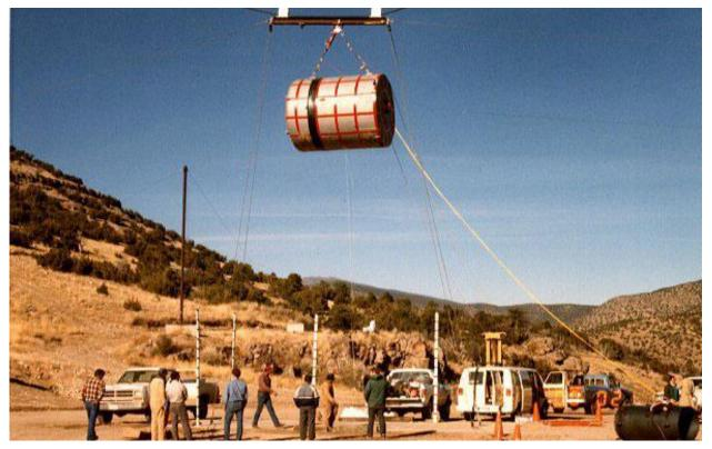
Figure 2.10.3-30 – CTU-1 Free Drop No. 2; Pre-Drop Positioning
