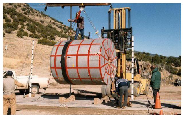
Figure 2.10.3-27 – CTU-1 Free Drop No. 1; Pre-Drop Positioning
