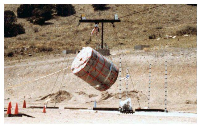
Figure 2.10.3-94 – CTU-3 Puncture Drop No. 8; Pre-Drop Positioning
