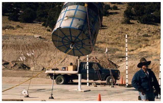
Figure 2.10.3-66 – CTU-2 Puncture Drop No. 5; Pre-Drop Positioning
