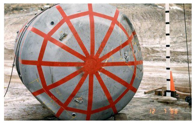
Figure 2.10.3-35 – CTU-1 Free Drop No. 4; Post-Drop Damage
