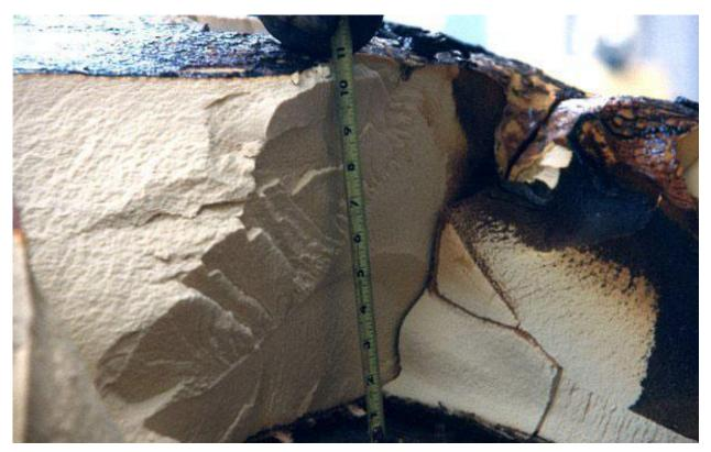
Figure 2.10.3-51 – CTU-1 Disassembly; OCA Lid Unburned Foam Thickness
