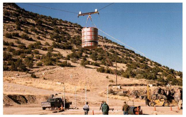
Figure 2.10.3-34 – CTU-1 Free Drop No. 4; Pre-Drop Positioning
