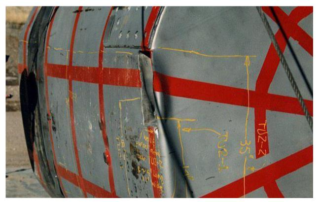
Figure 2.10.3-31 – CTU-1 Free Drop No. 2; Post-Drop Damage
