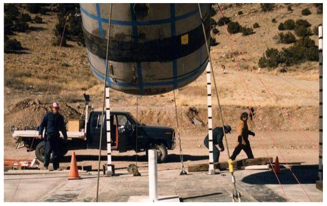
Figure 2.10.3-64 – CTU-2 Puncture Drop No. 4; Pre-Drop Positioning
