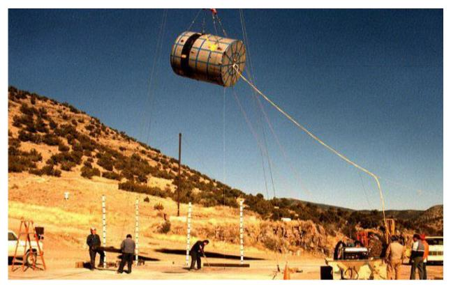
Figure 2.10.3-60 – CTU-2 Free Drop No. 3; Pre-Drop Positioning
