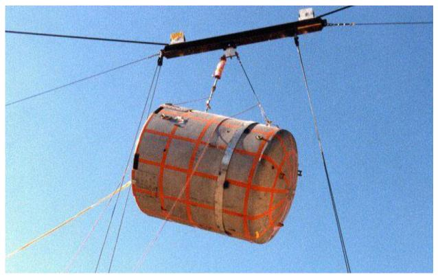
Figure 2.10.3-80 – CTU-3 Free Drop No. 1; Pre-Drop Positioning
