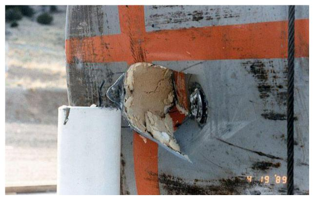
Figure 2.10.3-87 – CTU-3 Puncture Drop 4; Post-Drop Damage
