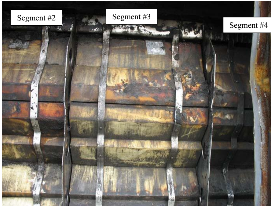
Figure 2.12.1-71 – Nylon 6,6 Segments #2, #3, and #4. Foam char is still visible on segment #3.
