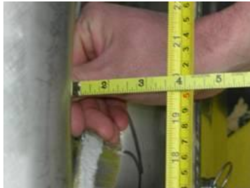
Figure 2.12.1-46 – CTU3 puncture depth measurement
