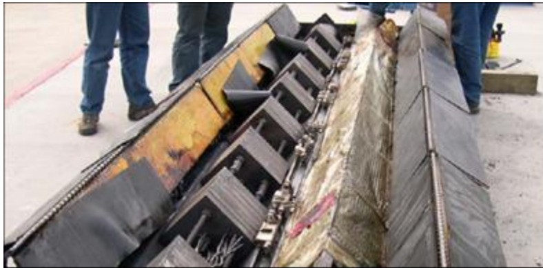
Figure 2.12.1-60 – Neoprene adhesive degradation during thermal test
