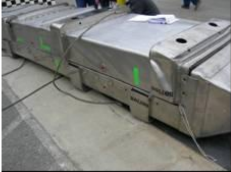
Figure 2.12.1-15 – CTU1 inverted for puncture test
