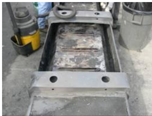
Figure 2.12.1-78 – Base liner with foam char removed
