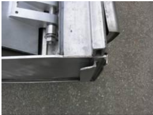
Figure 2.12.1-28 – No damage to bottom closure
