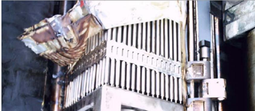
Figure 2.12.1-62 – Polypropylene sheet removal showing bright intact rods
