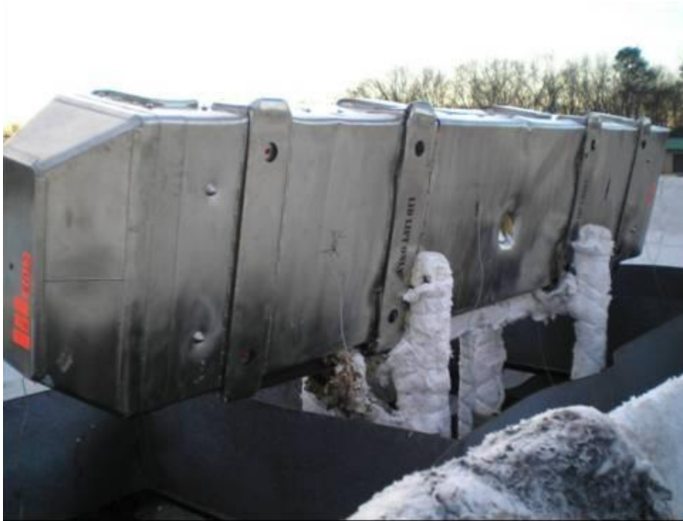
Figure 3-6 - MAP CTU 3 Mounted on Insulated Test Stand within Weir
