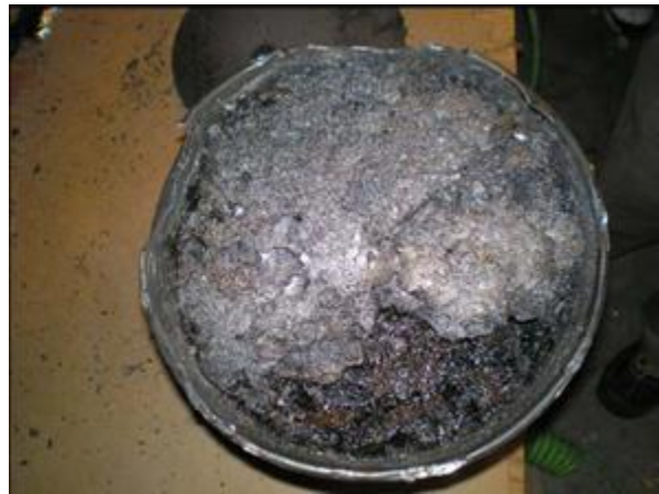
Figure 3-30 – Foam char under ceramic fiber paper
