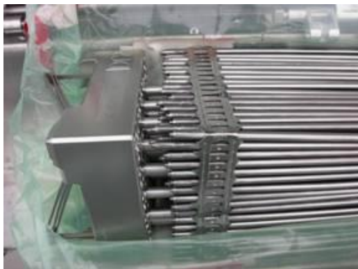
Figure 2.12.1-34 - Slight rod movement (top)
