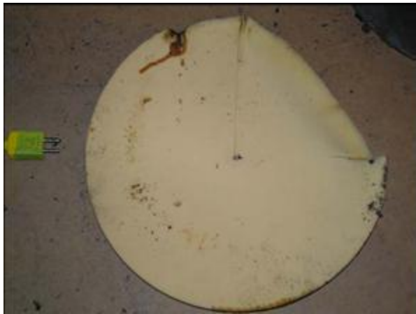
Figure 3-29 – Remaining 6 lb/ft 3 foam, backside
