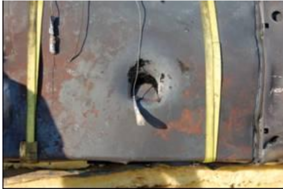
Figure 2.12.1-51 – Puncture area after thermal test
