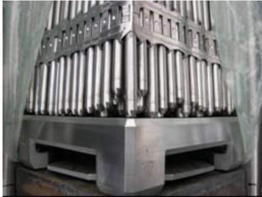
Figure 2.12.1-30 – Slight rod movement (bottom)
