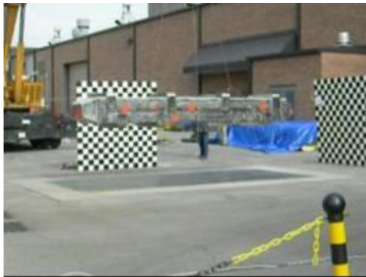
Figure 2.12.1-35 – CTU3 prior to NCT test
