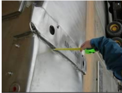
Figure 2.12.1-42 – CTU3 lid deformation measurement
