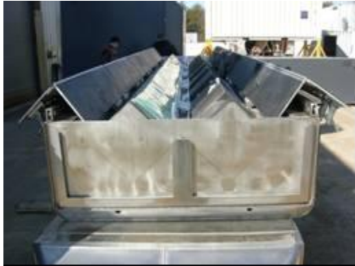
Figure 2.12.1-8 – Base interior after impact
