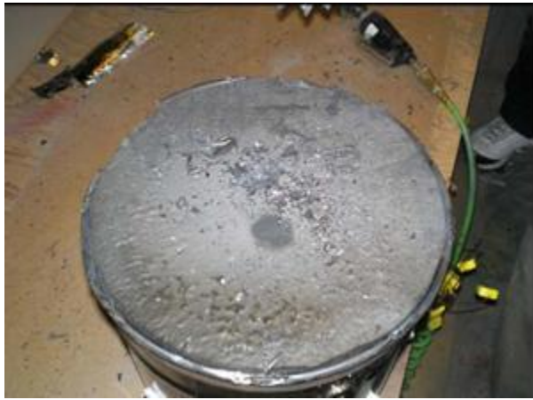
Figure 3-27 – Intact ceramic fiber following test
