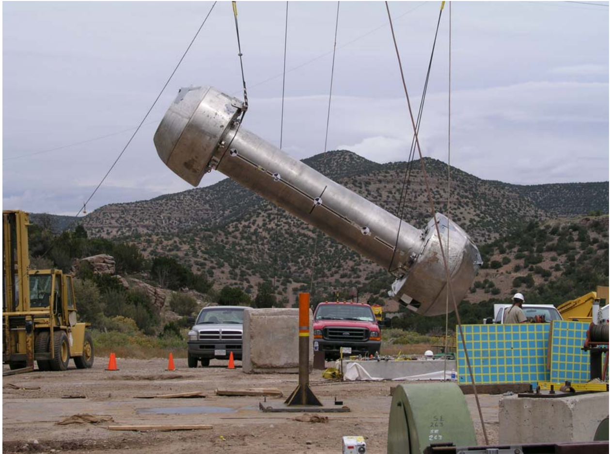
Figure 2.12.3-36 – Series 3, Test 4: HAC 30-Degree Puncture Drop
