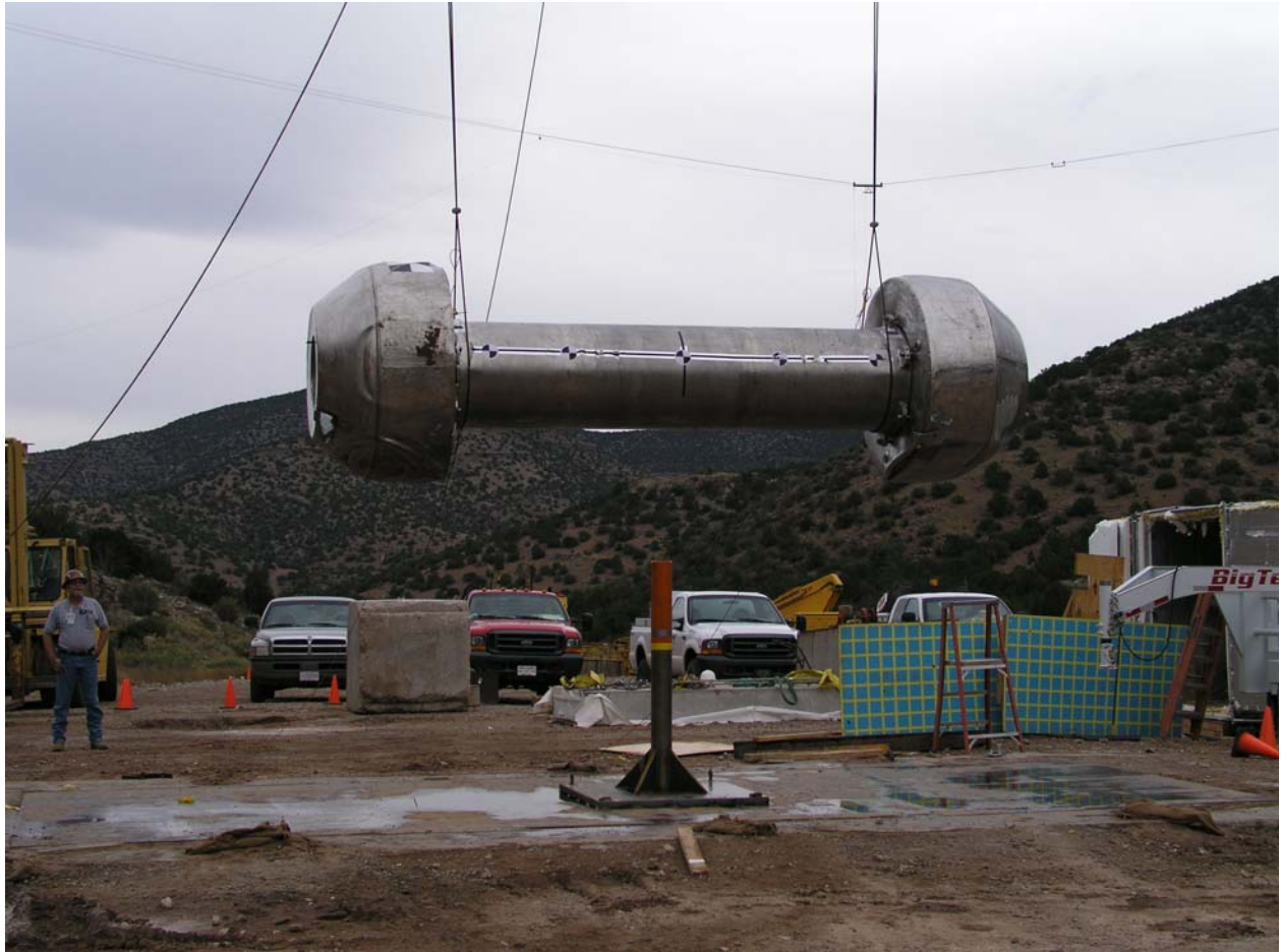
Figure 2.12.3-34 – Series 3, Test 3: HAC Horizontal Puncture Drop
