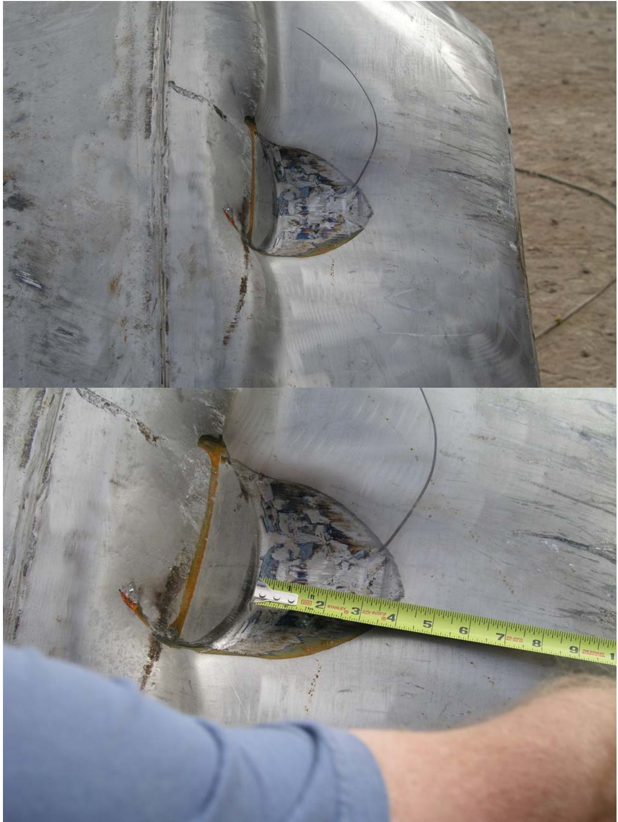
Figure 2.12.3-13 – Series 1, Test 4: Close-up Views of Puncture Damage (~4" Length)
