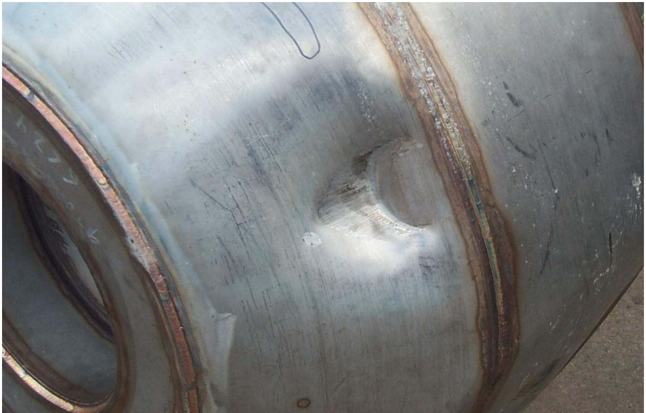
Figure 2.12.4-18 – ETU Test 8: View of Puncture Damage; ~2" Deep
