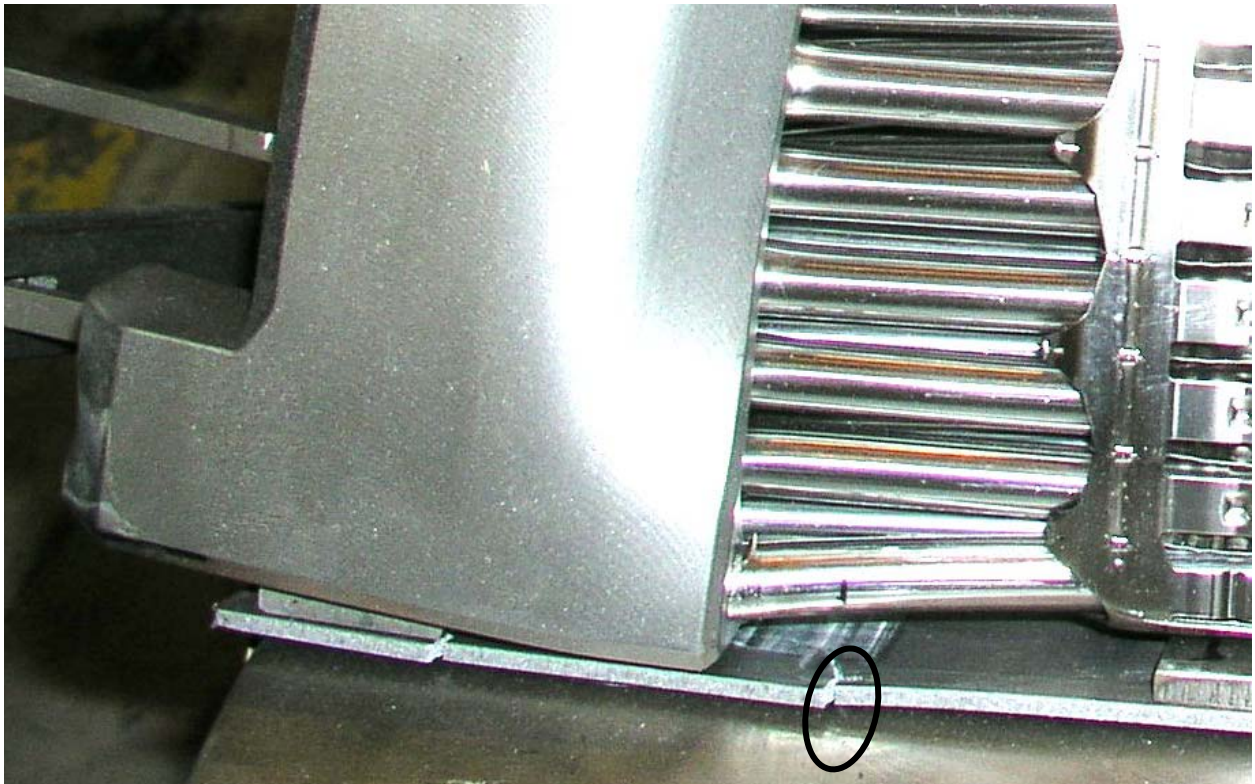
Figure 2.12.3-24 – Series 2: Worst-Case Neutron Poison Damage (Circled on Photo)
