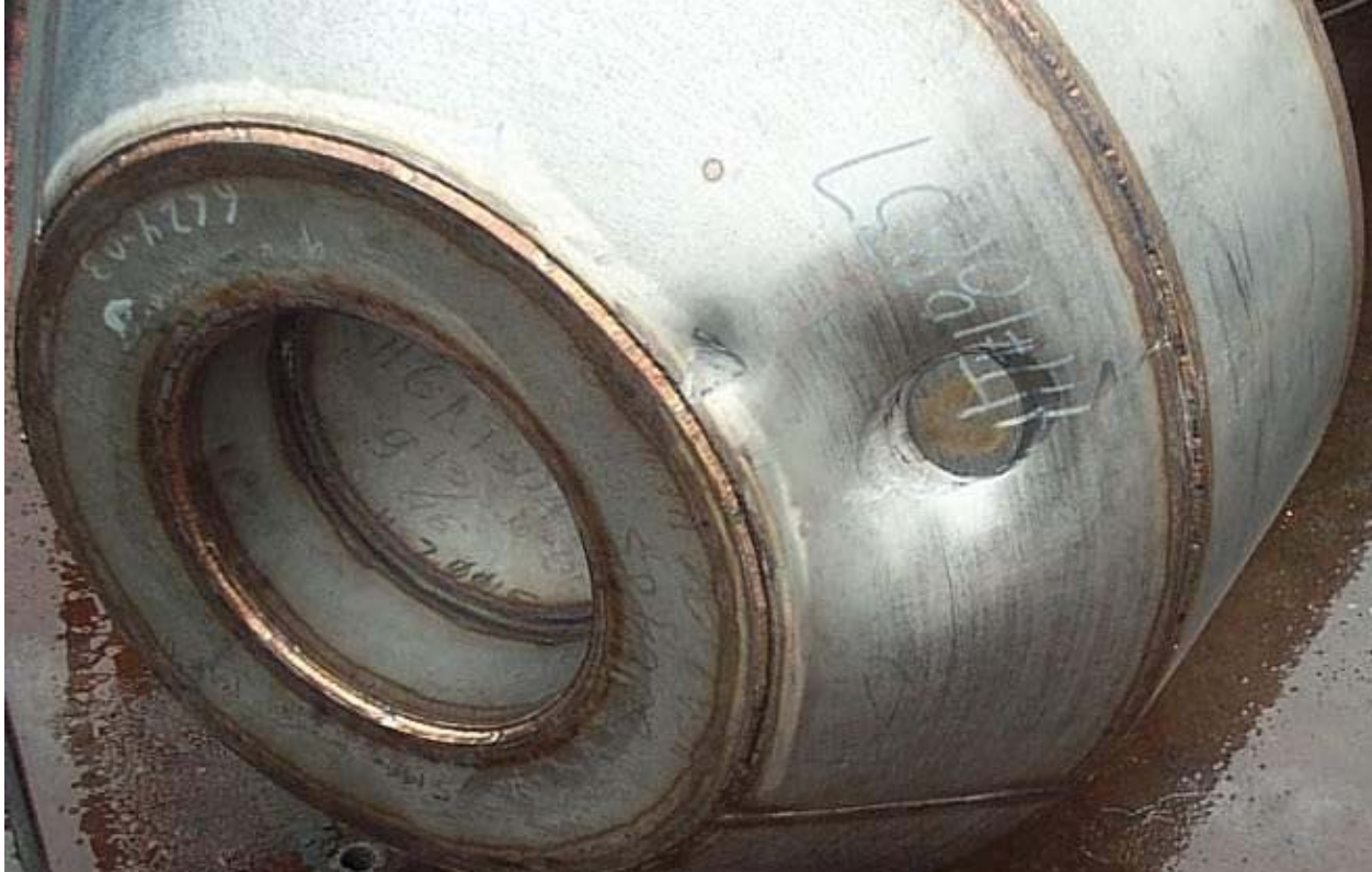
Figure 2.12.4-4 – ETU Test 1: View of Puncture Damage; ~1” Deep
