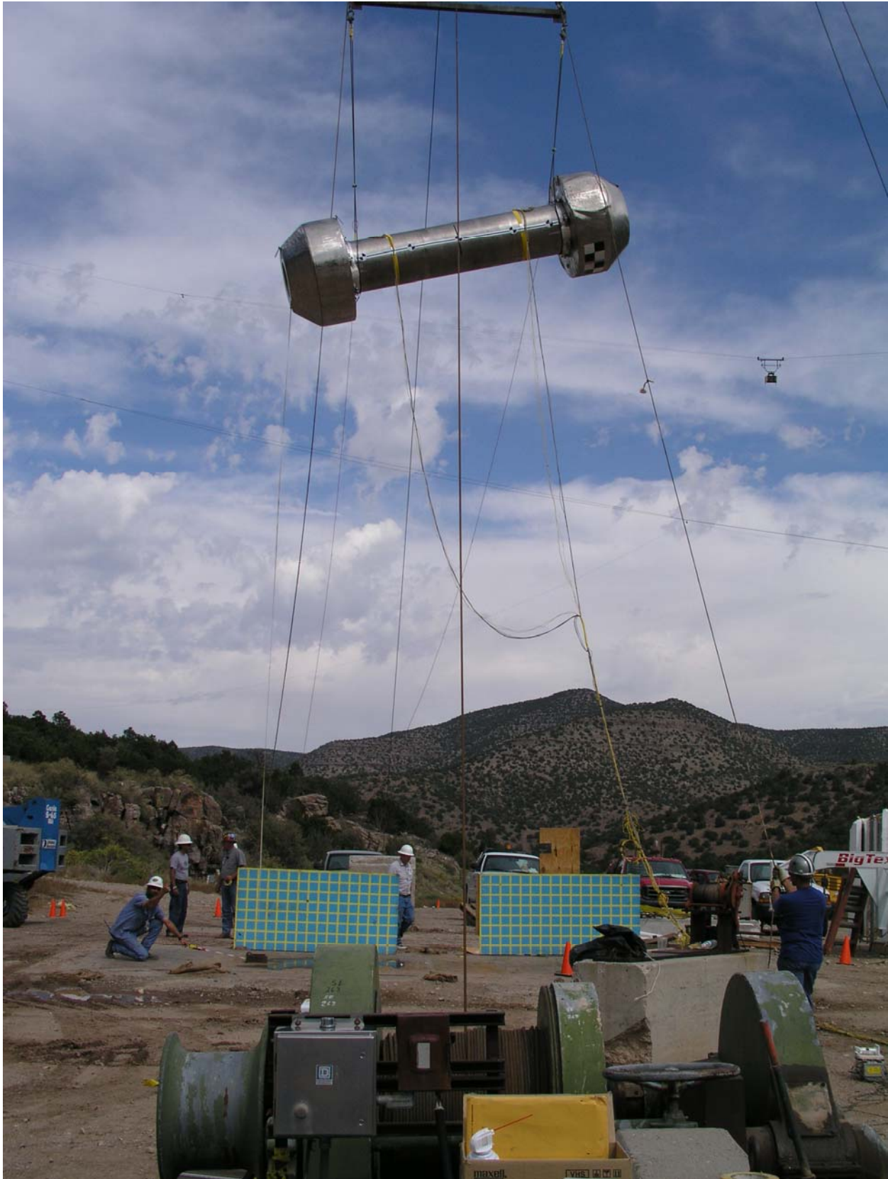
Figure 2.12.3-26 – Series 3, Test 1: HAC 15-Degree Slapdown 30-Foot Drop (Lid End Primary)
