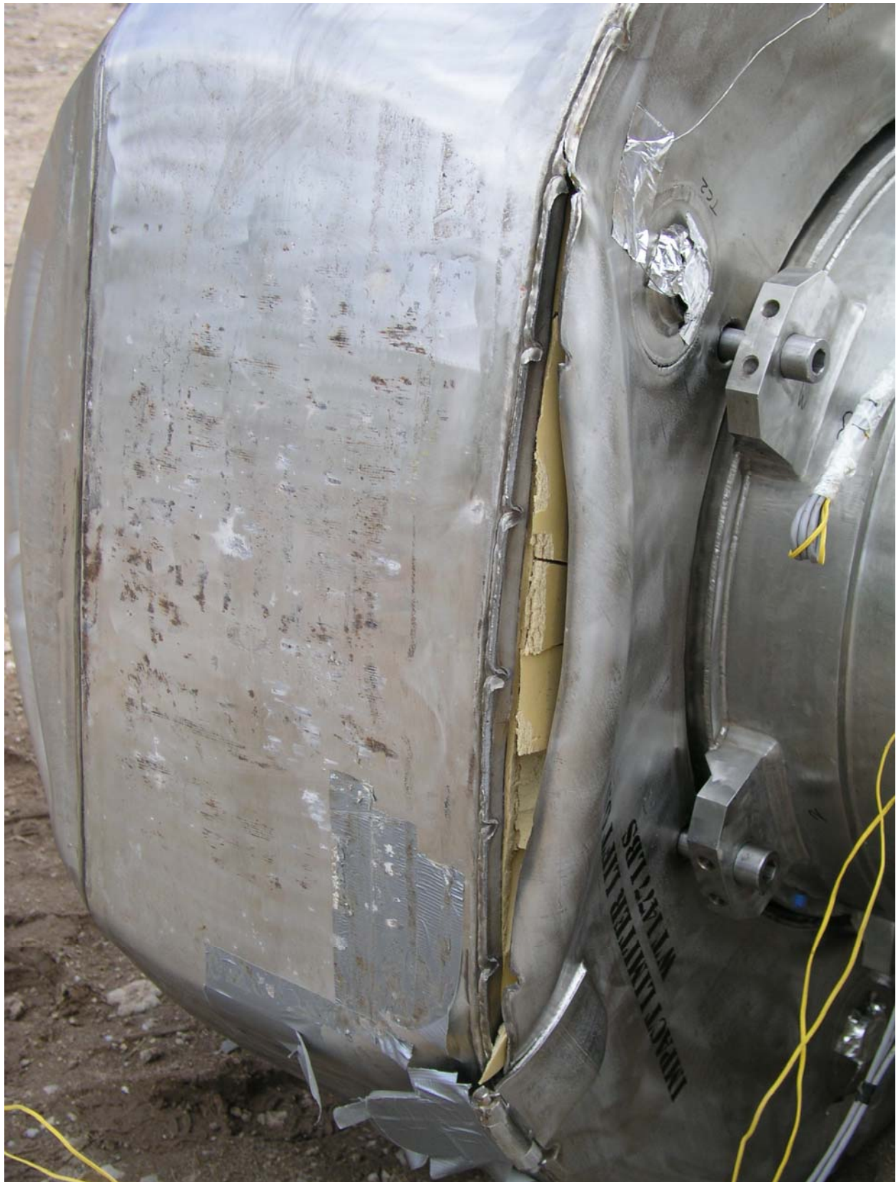
Figure 2.12.3-31 – Series 3, Test 2: Close-up View of Impact Limiter Damage (~31" Length)
