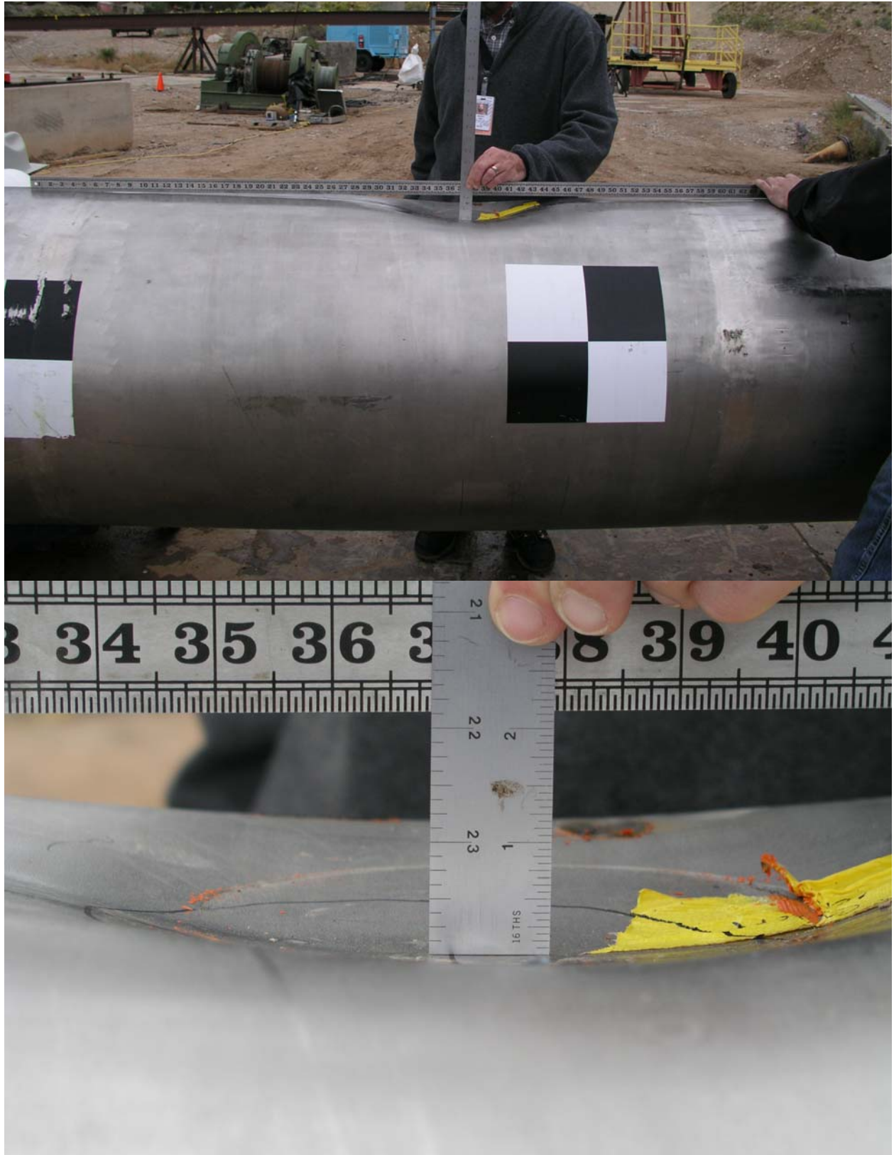
Figure 2.12.3-35 – Series 3, Test 3: Views of Shell Damage (~2 1/8" Deep)
