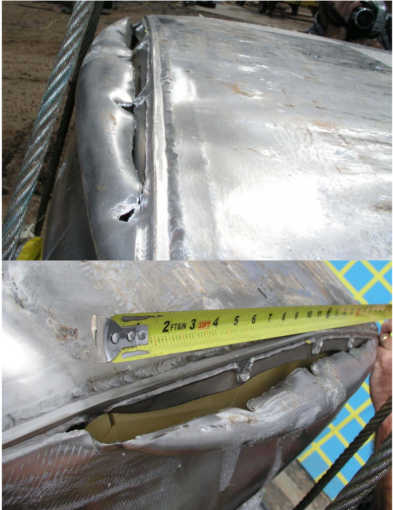
Figure 2.12.3-29 – Series 3, Test 1: Close-up View of Impact Limiter Damage (~21" Length)
