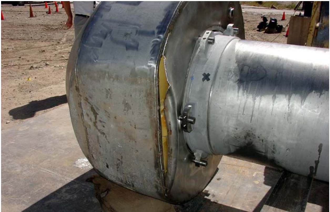
Figure 2.12.3-7 – Series 1, Test 1: View of Lid End Impact Limiter Damage (~28" Length)
