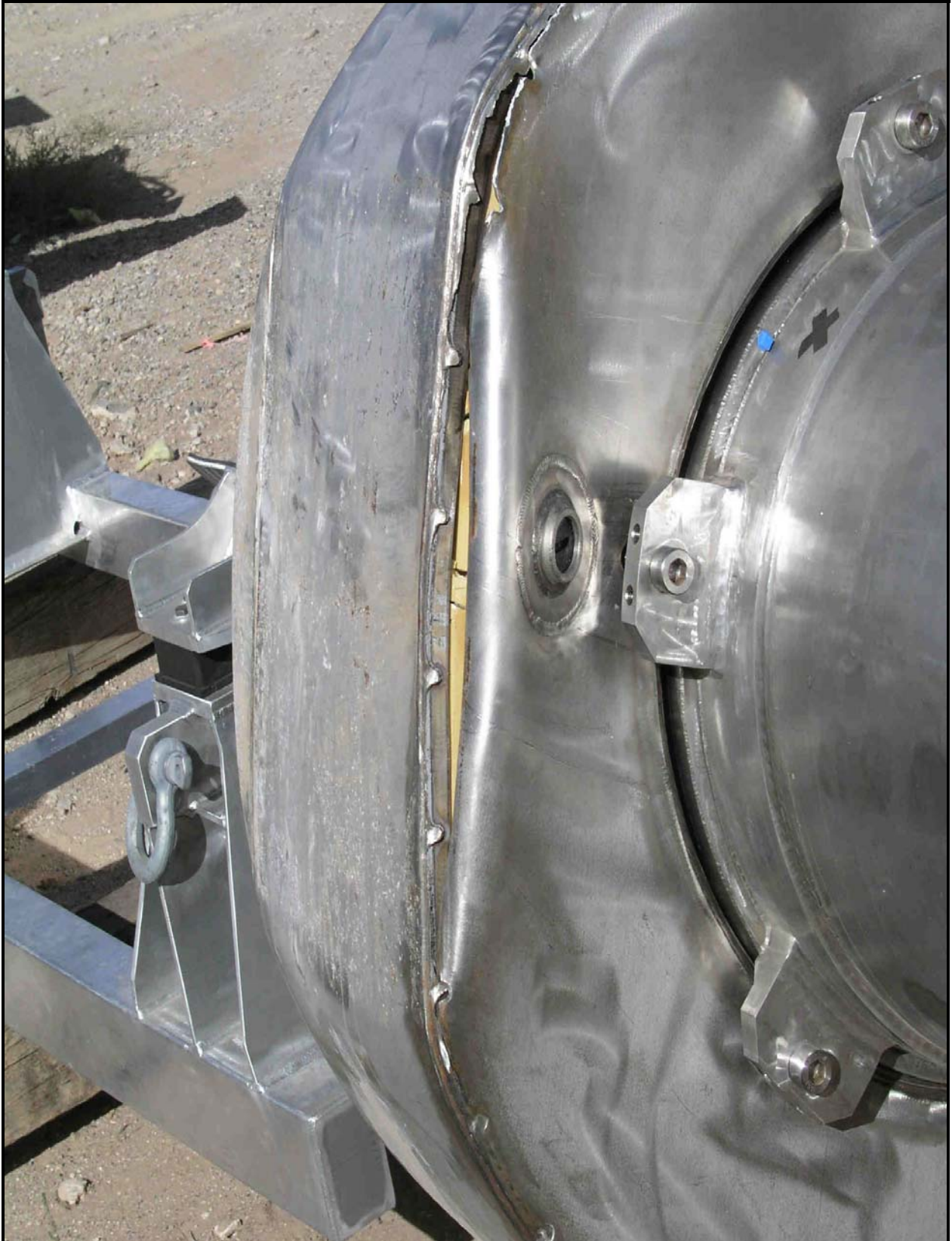
Figure 3.5-1 – CTU Impact Limiter Damage from Full-Scale Side 30-ft Free Drop Test
