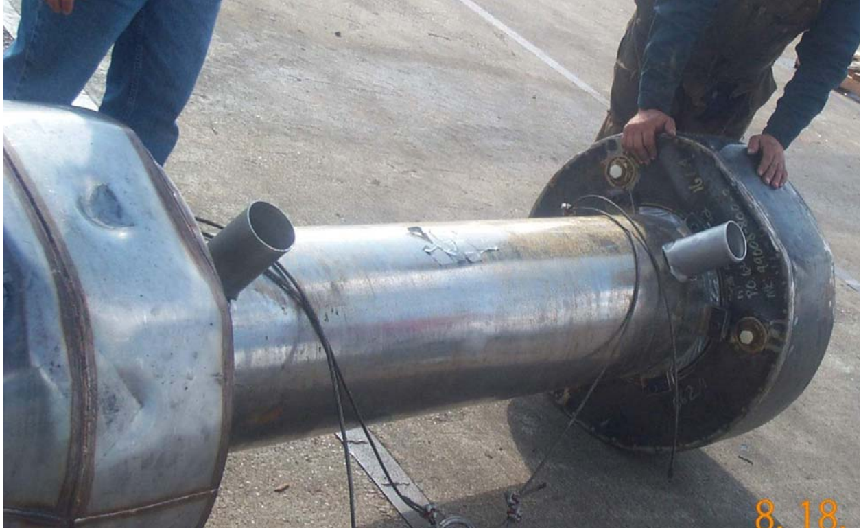
Figure 2.12.4-14 – ETU Test 6: View of Free Drop Damage
