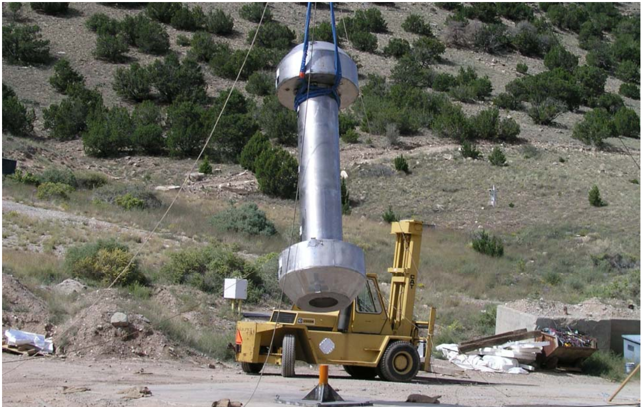
Figure 2.12.3-10 – Series 1, Test 3: HAC 65-Degree Oblique 40-Inch Puncture Drop
