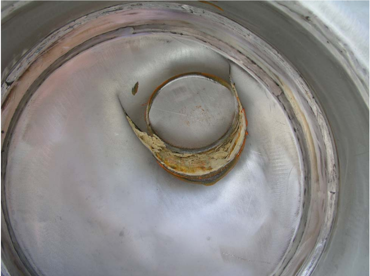
Figure 2.12.3-11 – Series 1, Test 3: Close-up View of Puncture Damage (~3" Deep)
