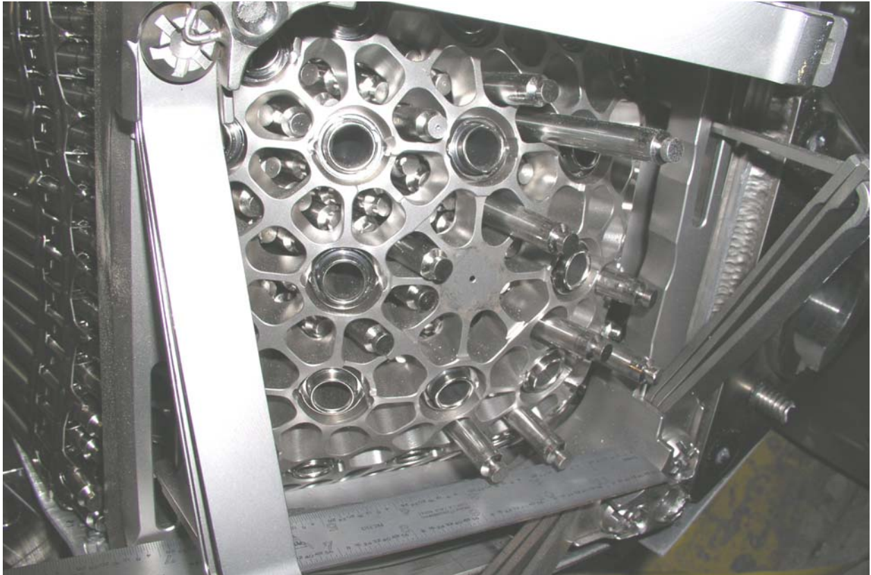
Figure 2.12.3-23 – Series 2: View of Top Nozzle Damage of the Prototypic Fuel Assembly
