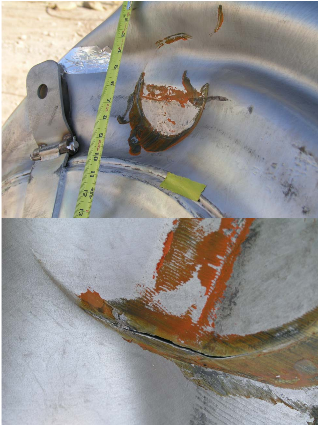
Figure 2.12.3-18 – Series 2, Test 2: Overall and Close-up Views of Damage (~1½” Deep)
