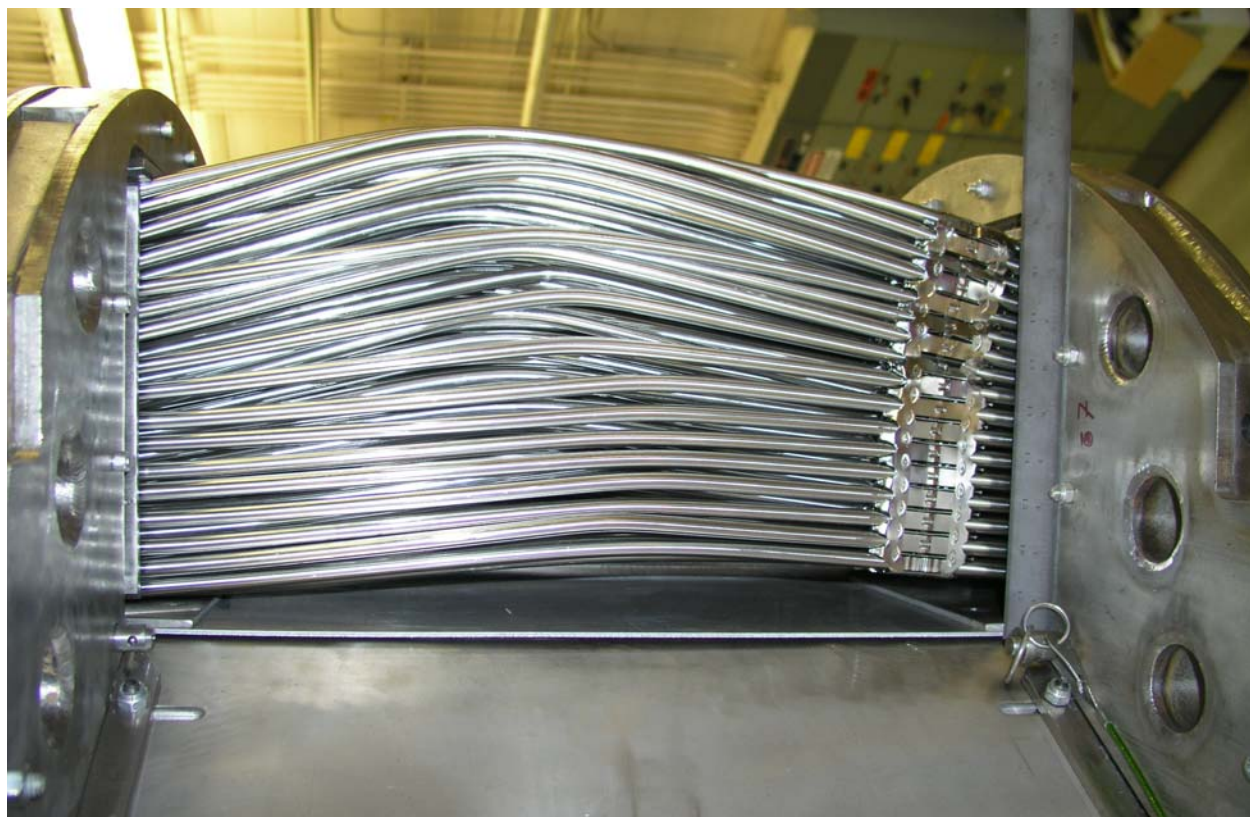
Figure 2.12.5-2 – Buckled Shape of Fuel Rod from Certification Test
