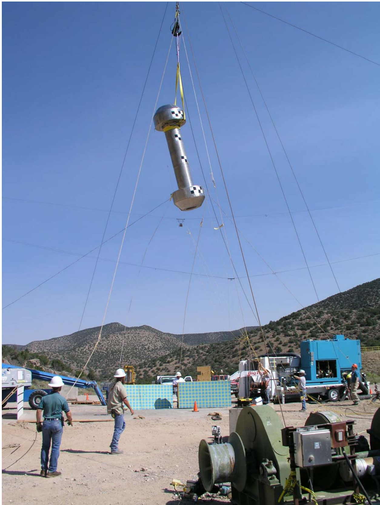
Figure 2.12.3-14 – Series 2, Test 1: HAC 80-Degree Oblique C.G.-Over-Corner 30-Foot Drop
