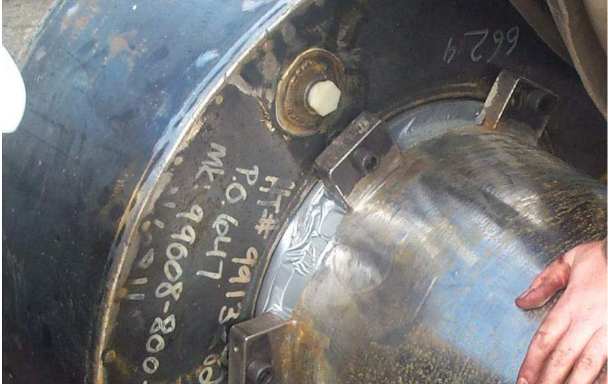
Figure 2.12.4-10 – ETU Test 4: View of Puncture Damage; ~3/8” Deep
