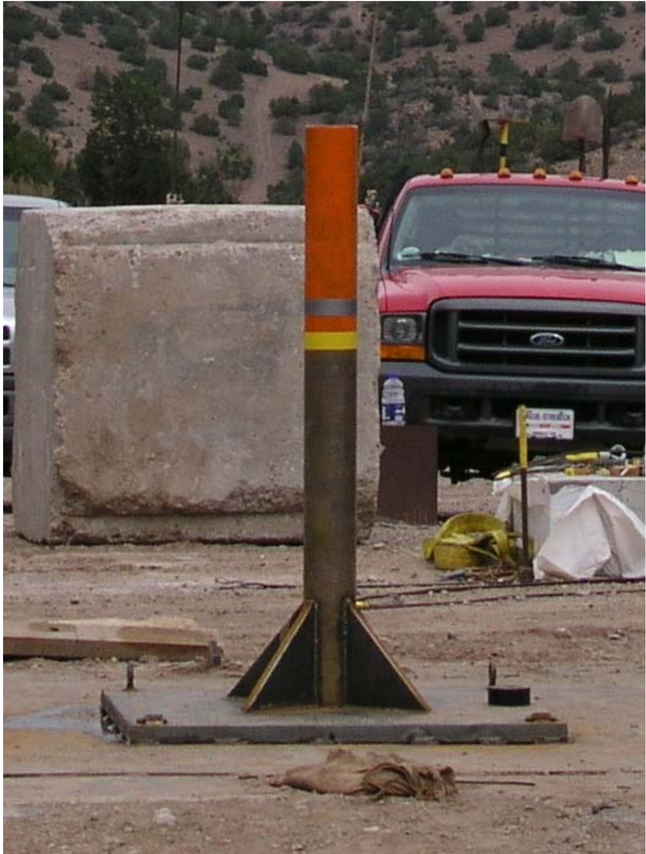
Figure 2.12.3-1 – Attachment of Puncture Bar Assembly to Drop Pad
