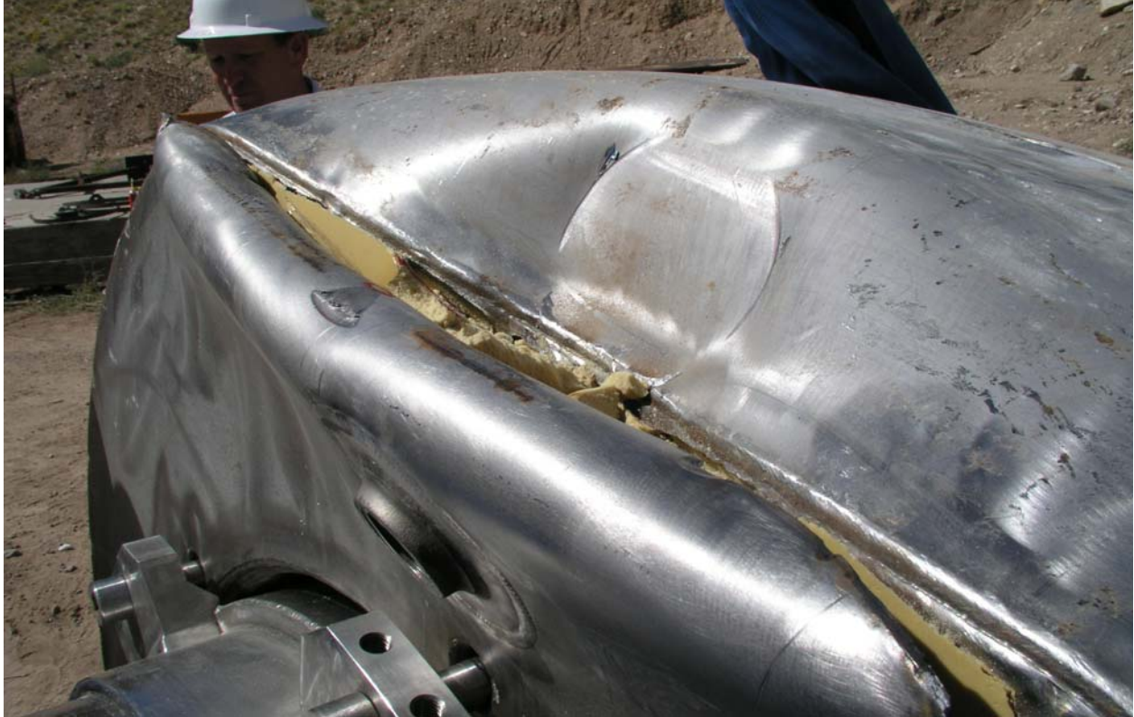
Figure 2.12.3-9 – Series 1, Test 2: Close-up View of Puncture Damage
