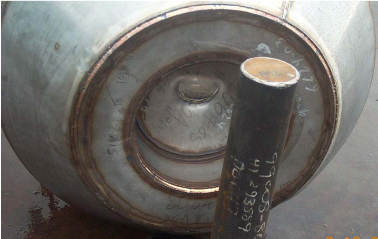
Figure 2.12.4-8 – ETU Test 3: View of Puncture Damage; ~1 \frac{1}{8} " Deep
