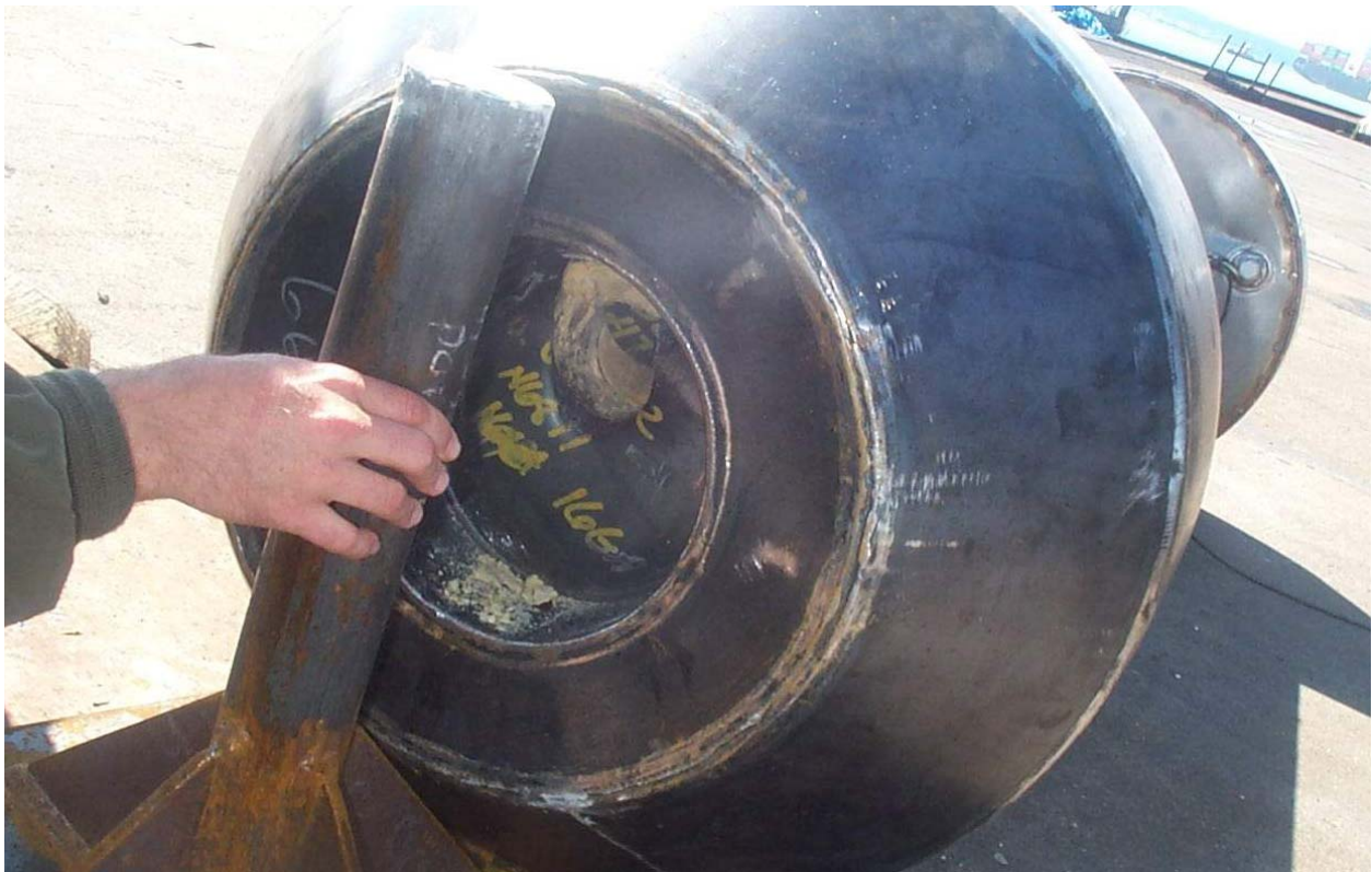
Figure 2.12.4-12 – ETU Test 5: View of Puncture Damage; ~2 3 / 4 " Deep
