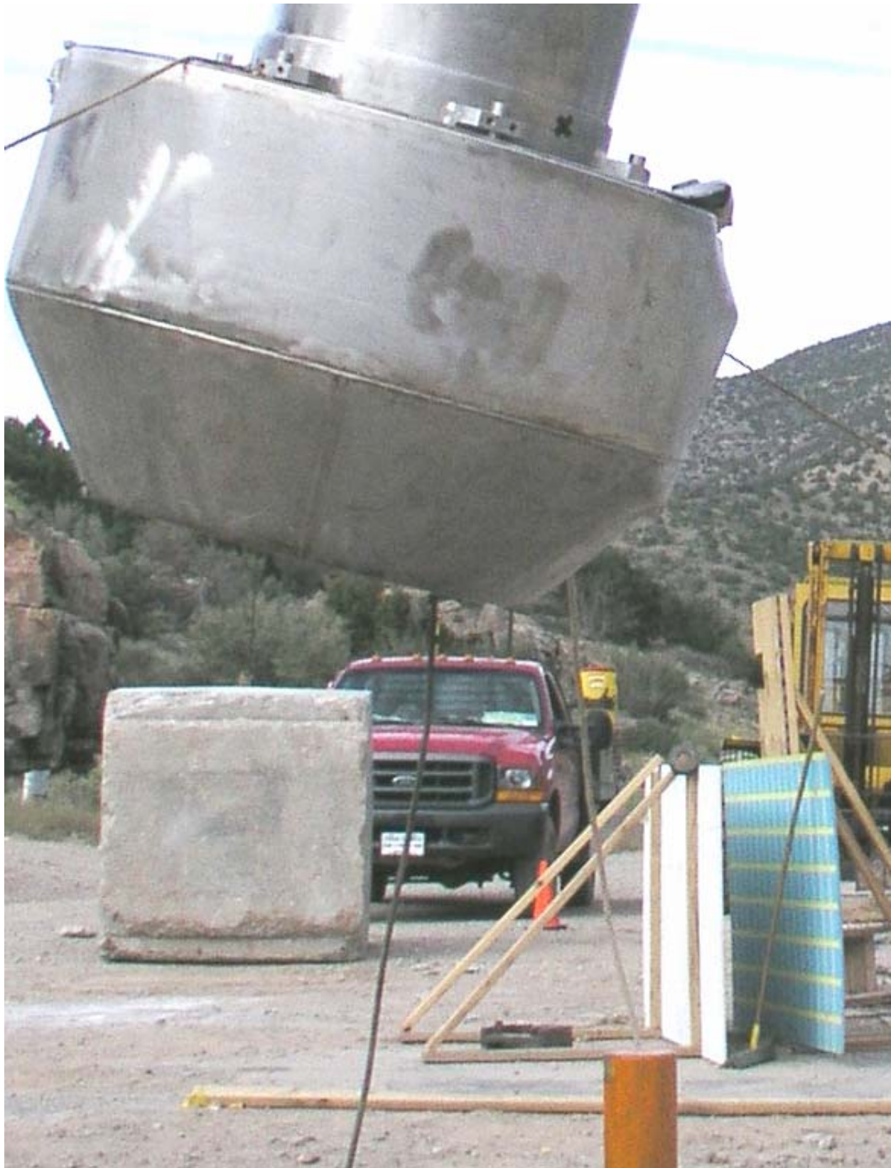
Figure 2.12.3-12 – Series 1, Test 4: HAC 75-Degree Oblique 40-Inch Puncture Drop
