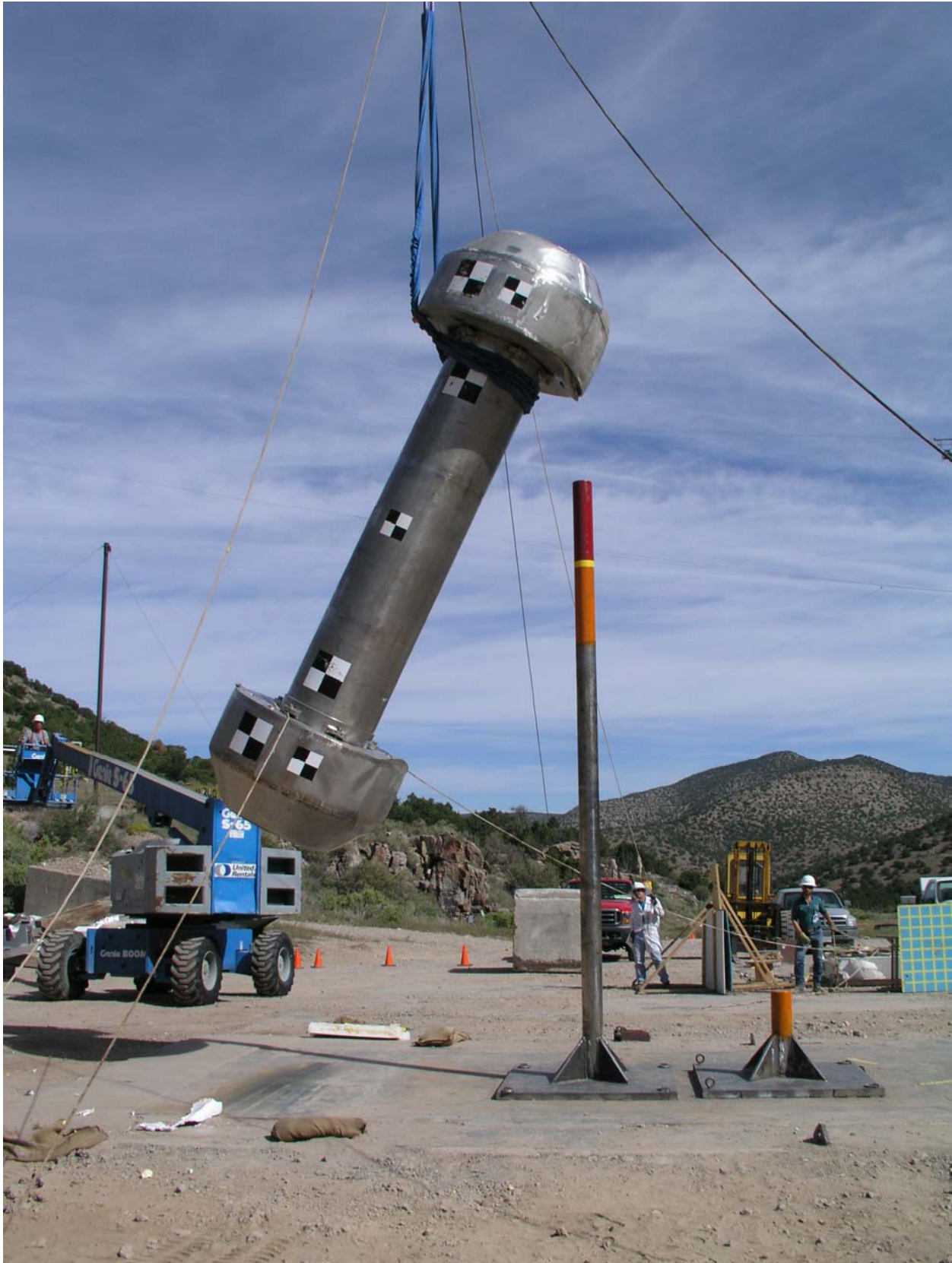
Figure 2.12.3-8 – Series 1, Test 2: HAC 40-inch Near Vertical Puncture Drop
