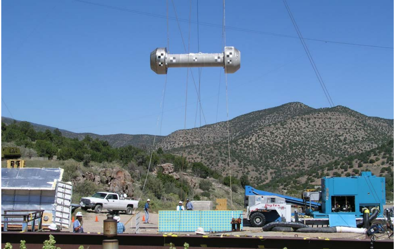
Figure 2.12.3-6 – Series 1, Test 1: HAC 30-Foot Free Side Drop
