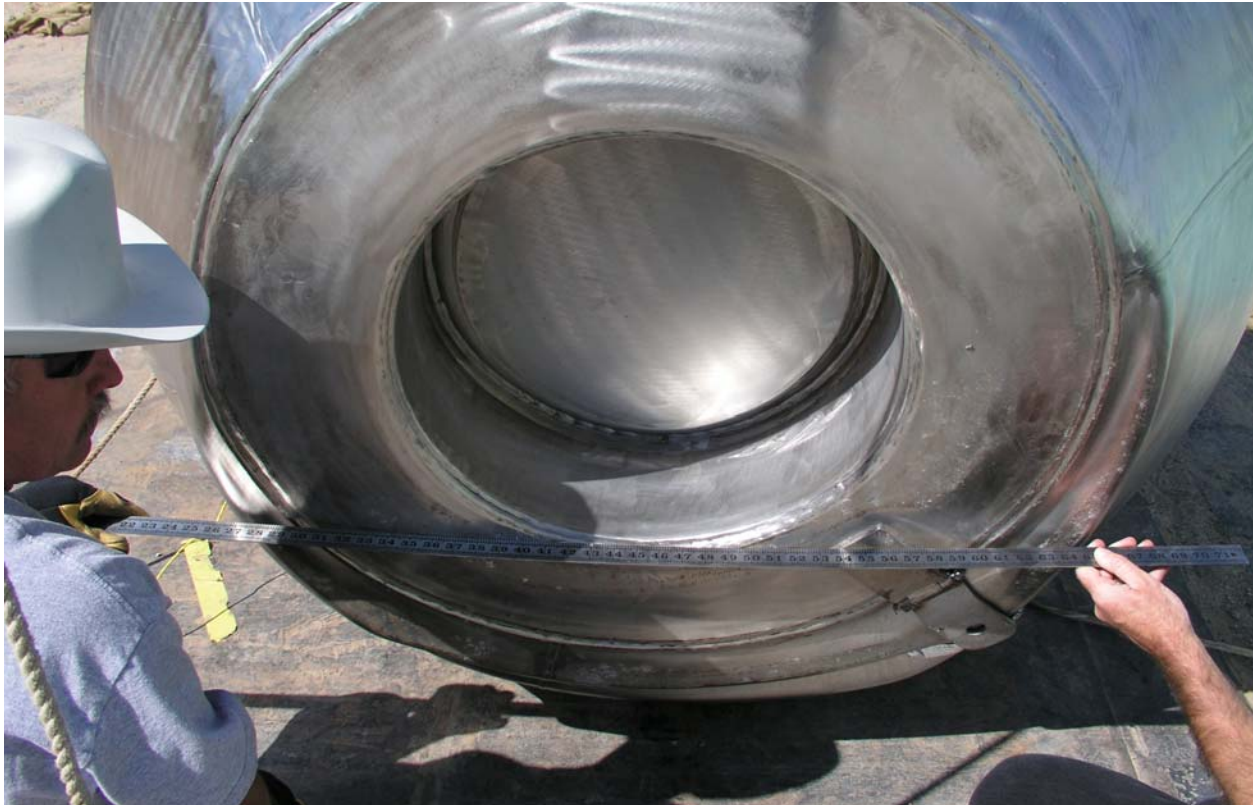
Figure 2.12.3-15 – Series 2, Test 1: Overall View of Impact Limiter Damage
