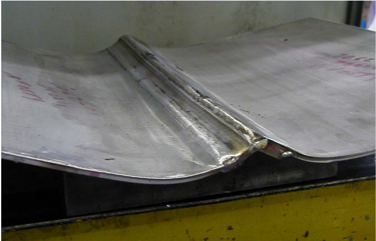
FIGURE 2.12.7-4 – View of V-Groove Weld of TS-1 (No weld cracks)
