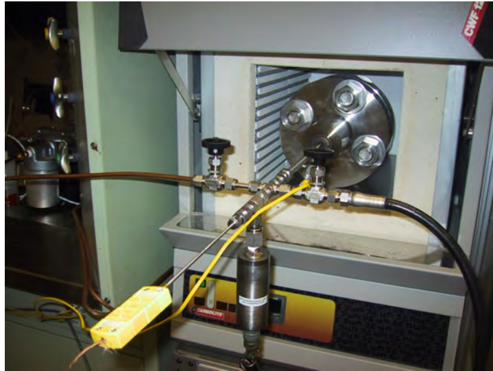
Figure 2: Test rig: test vessel inside the furnace with thermocouple and pressure transducer in place
