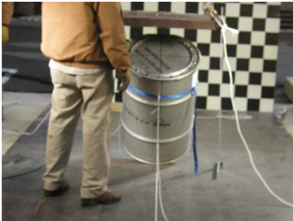
Figure H 18. Close-up aligning the 500 kg crush weight above the TU-4 package.
