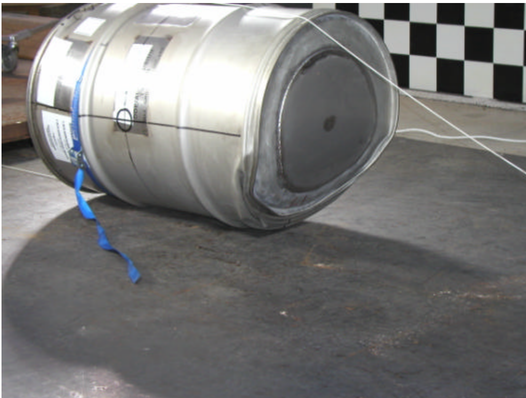
Figure H 23. View of damage to the bottom of TU-4 from the crush test.
