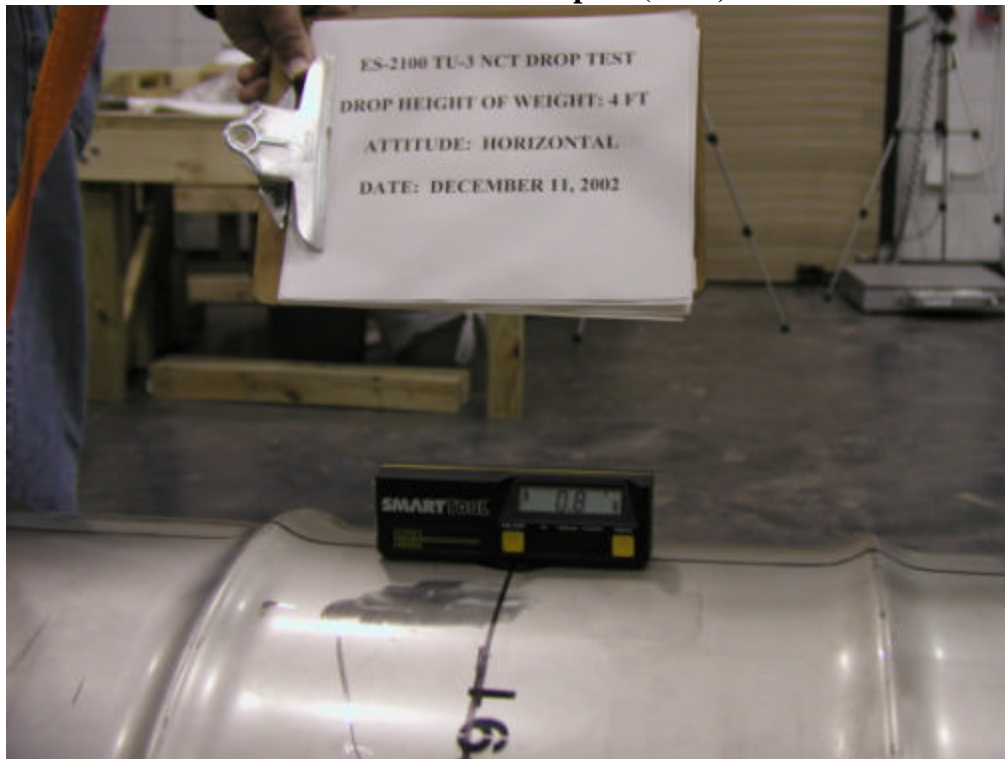
Figure G 9. Measuring how close TU-3 is to horizontal prior to the drop.
