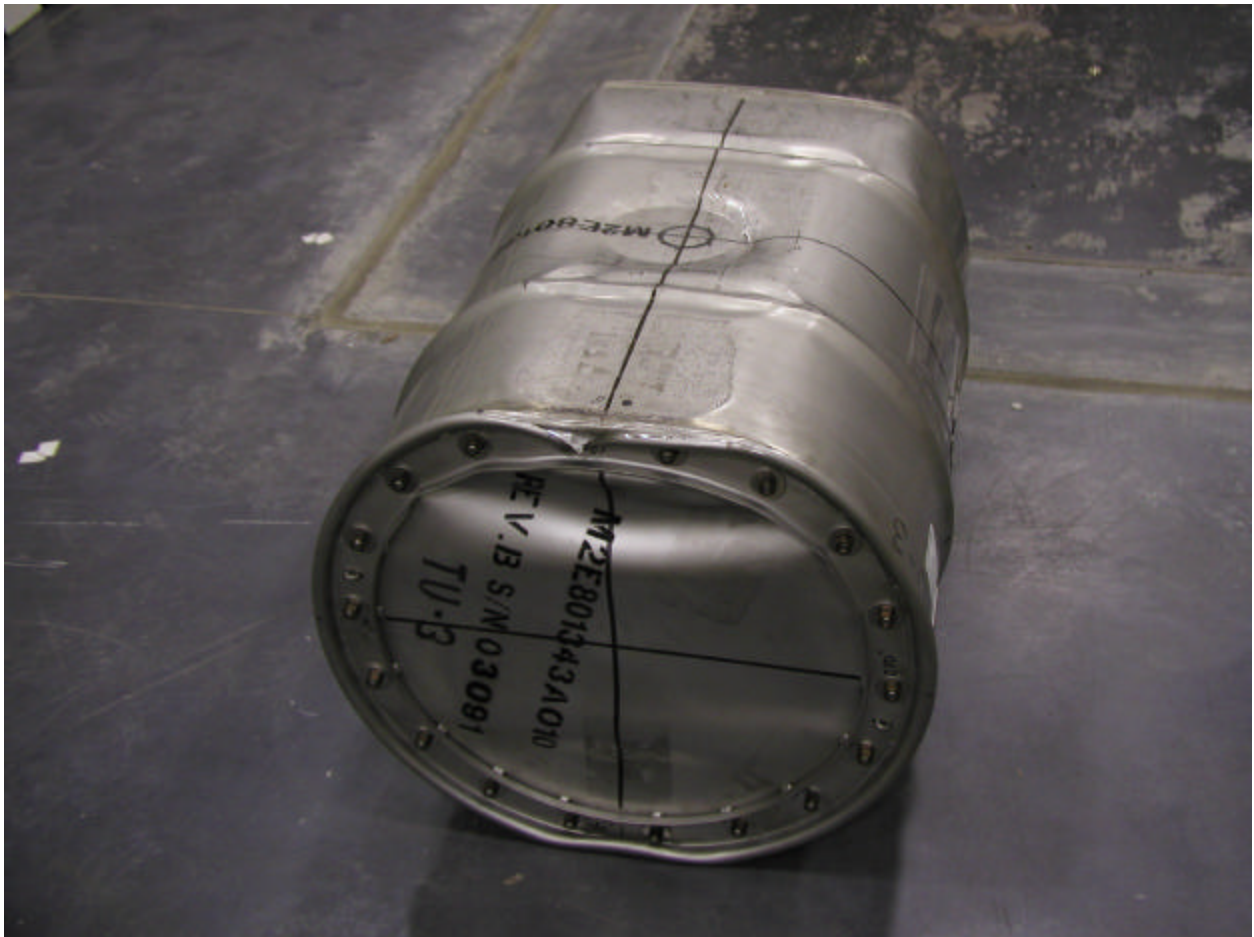
Figure 3-19 Damage produced from previous tests plus the punch test of TU-3.
