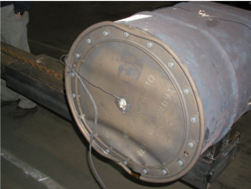
Figure G 21. End of TU-3 Thermocouple attached.
