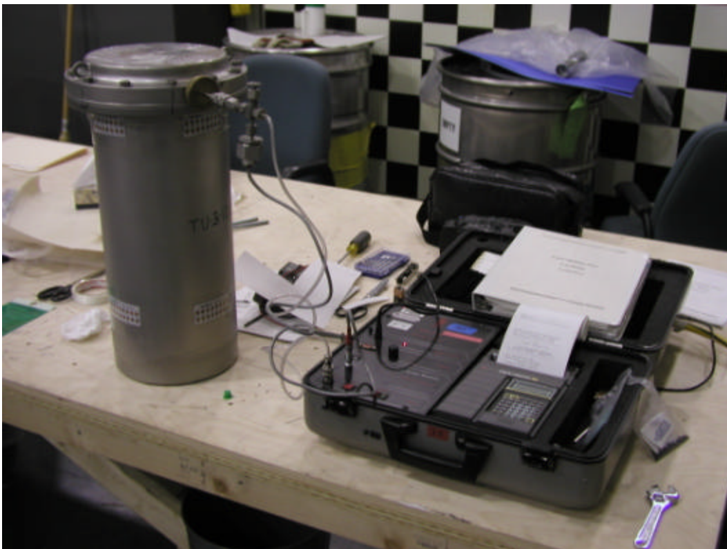
Figure G 4. Leak testing the sealed CV.
