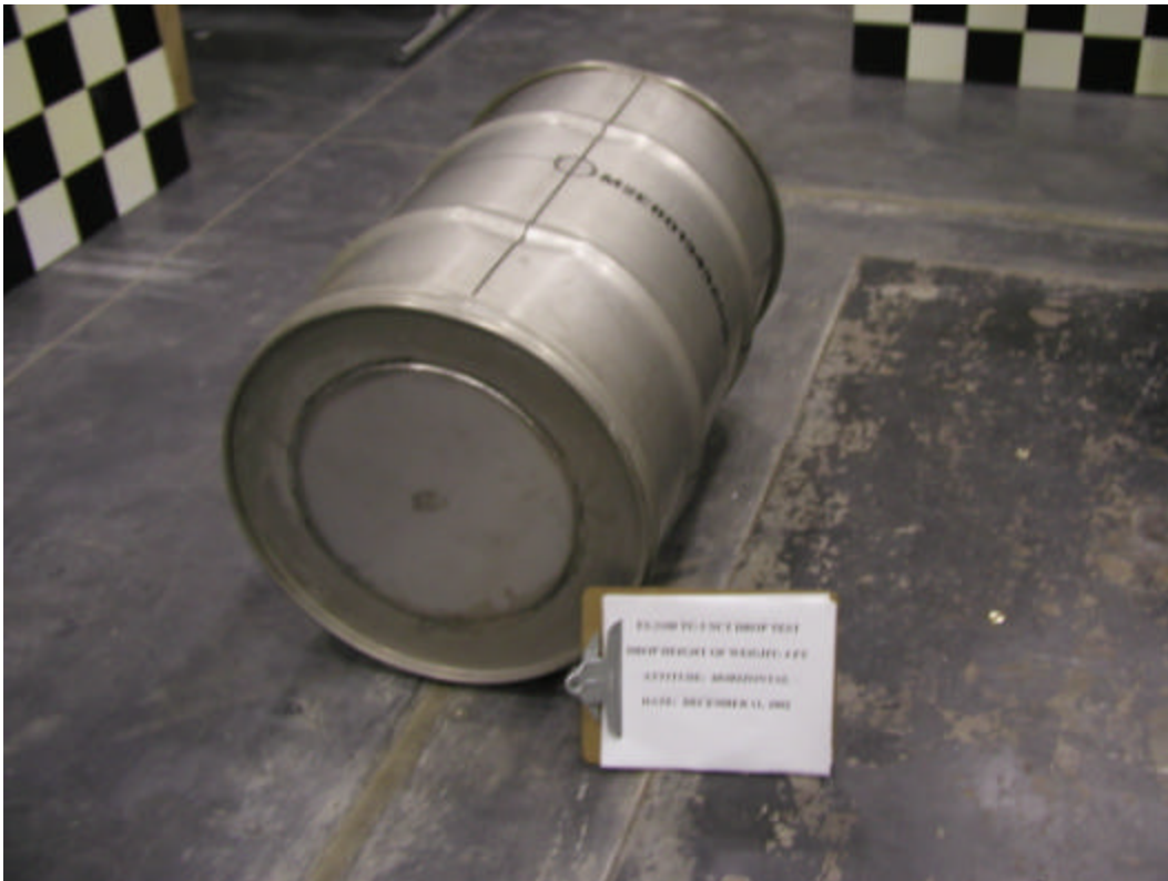
Figure G 12. Bottom end view of damage to TU-3 on the 0° line – package has been rolled 180°.
