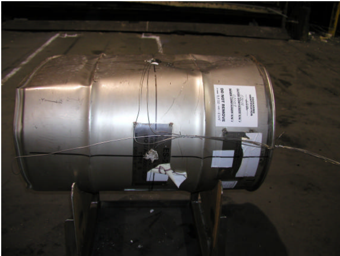
Figure 4-3 Thermocouples installed and ready to put into furnace.
