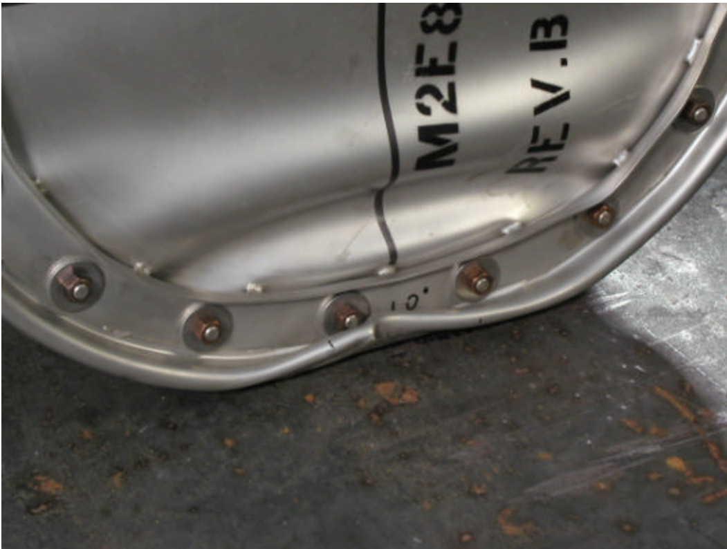
Figure E 22. Close up of damage to the lid end on the 0° line from the crush test.
