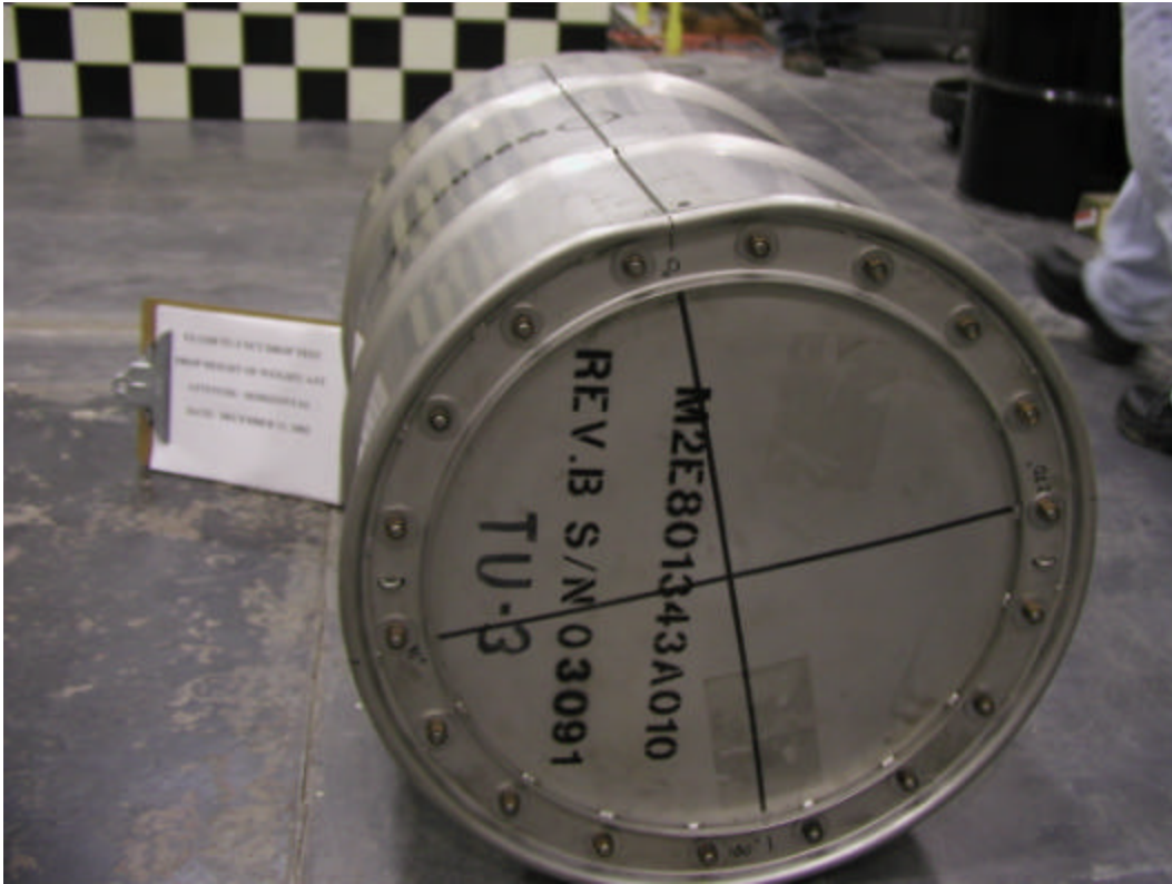
Figure G 11. Top end view of damage to TU-3 on the 0° line – package has been rolled 180°.
