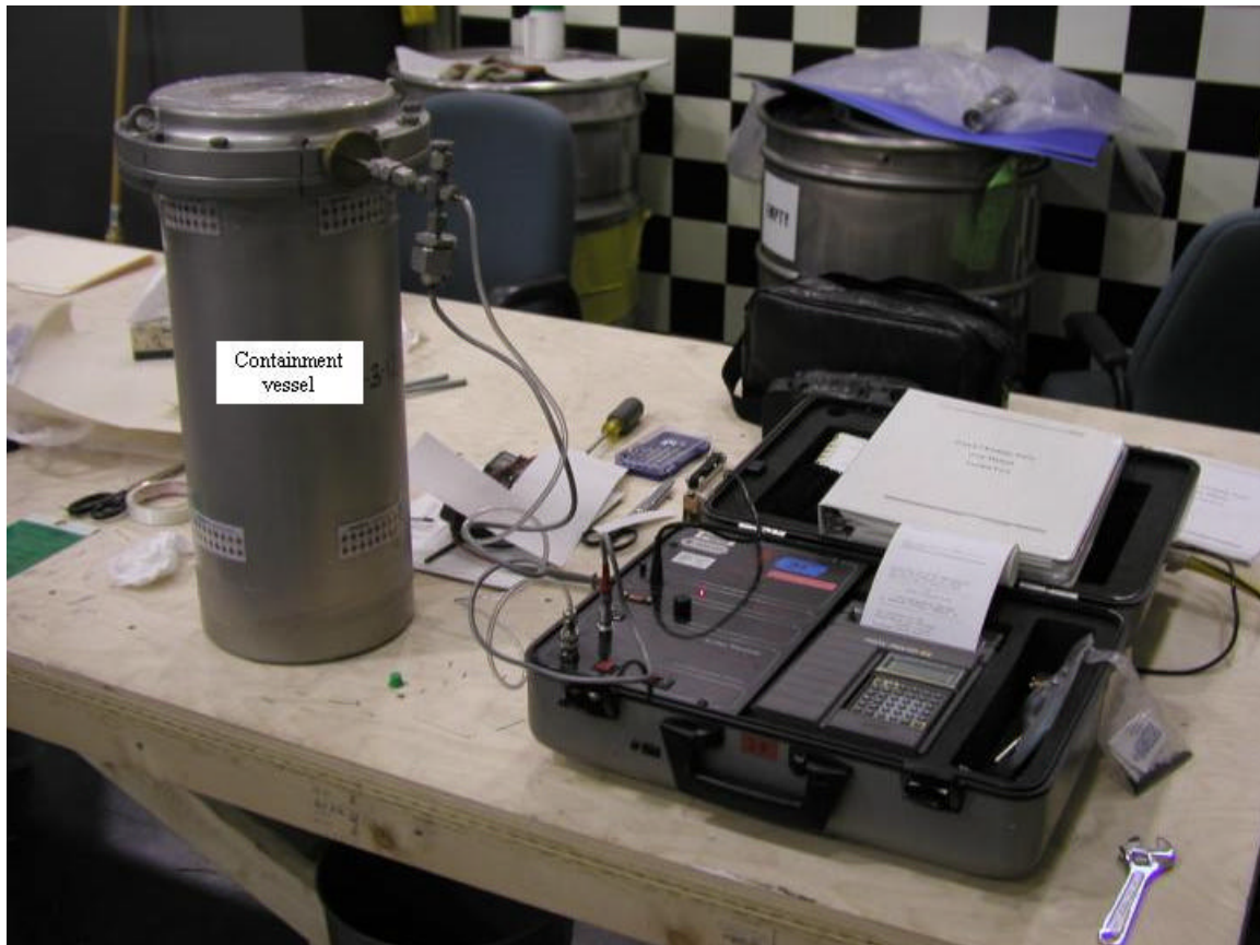
Figure 2-2 Checking the leak rate of an ES-2100 containment vessel with a CALT 5 leak tester.
