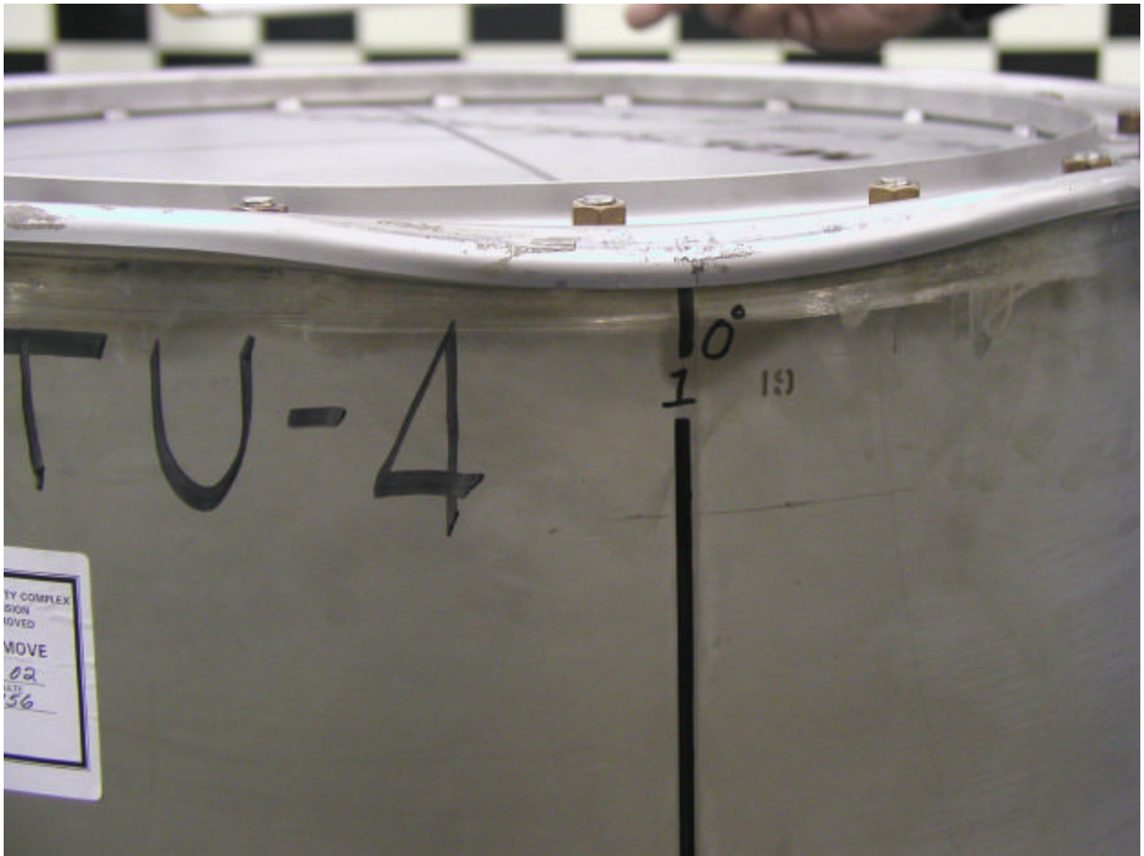
Figure 3-3 Photo of the damage to the top ring on the closure of TU-4 resulting from the NCT drop test.
