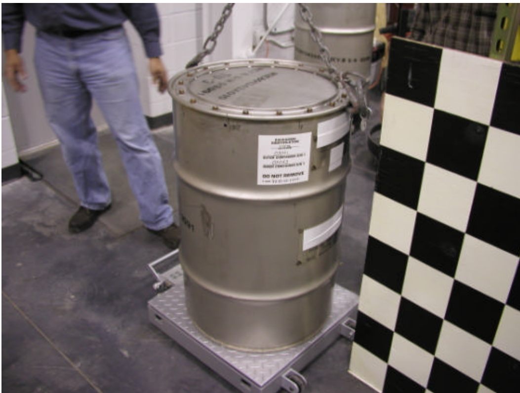
Figure G 8. Weighing the completed TU-3 package.
