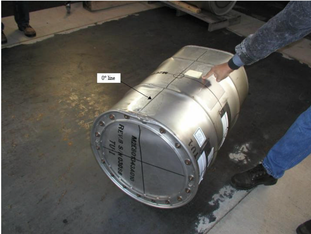
Figure E 17. View of damage along the 0° line from lid end.
