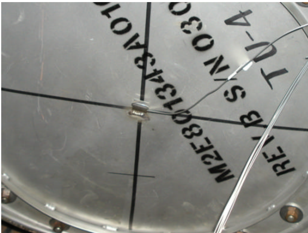
Figure H 34. Close-up of thermocouple on lid of TU-4.
