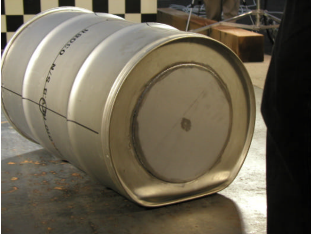
Figure E 15. End view of TU-1 bottom after the HAC 30-ft drop on the 0° line.
