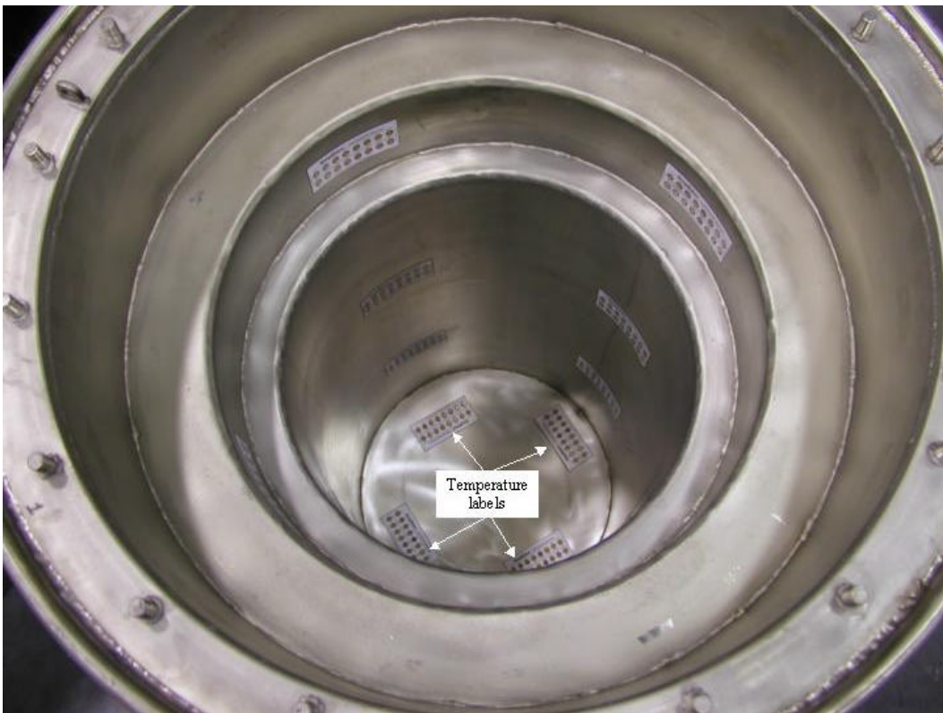
Figure H 5. Preparation of TU-4 containing temperature labels and ready to accept the CV.
