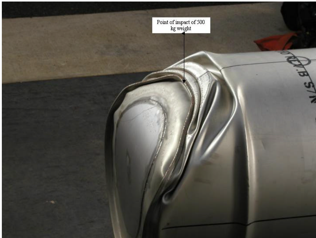
Figure F 29. Close-up of damage to the bottom of TU-2 at point of impact.
