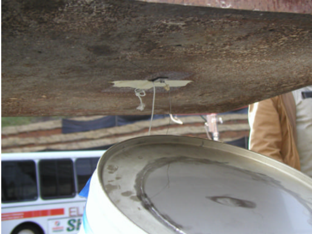
Figure F 27. Aligning the 500 kg weight to the bottom edge of TU-2.
