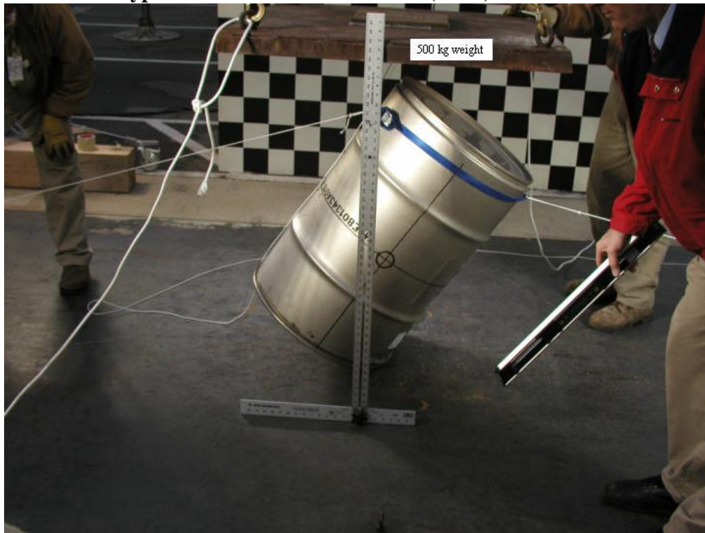
Figure F 25. Set-up for the crush test with TU-2 balanced on edge of lid and held with nylon cords.
