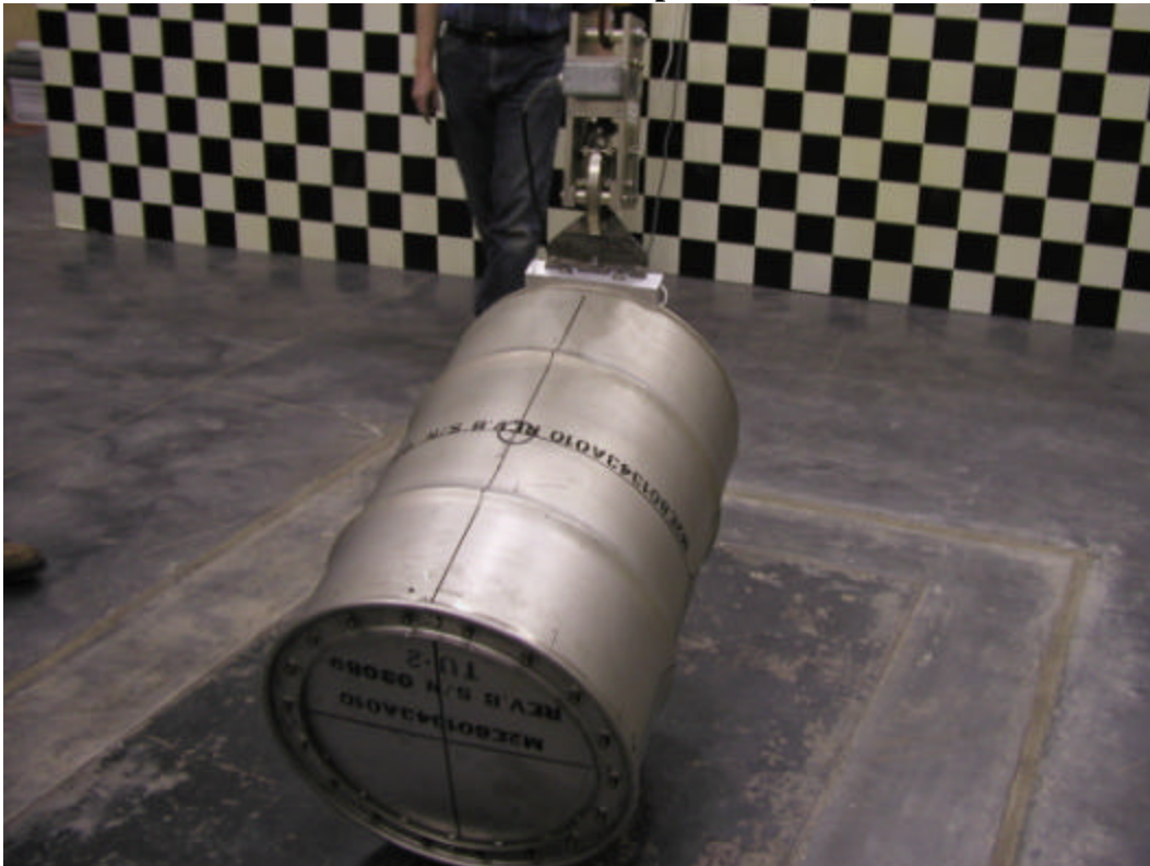
Figure F 11. Preparing TU-2 for a CG-over-corner drop
