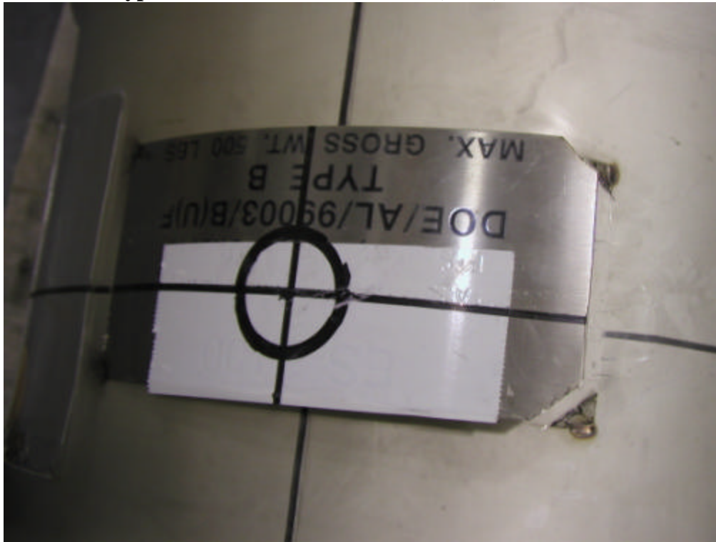
Figure F 32. Removal of the name plate in preparation for the punch test of TU-2.
