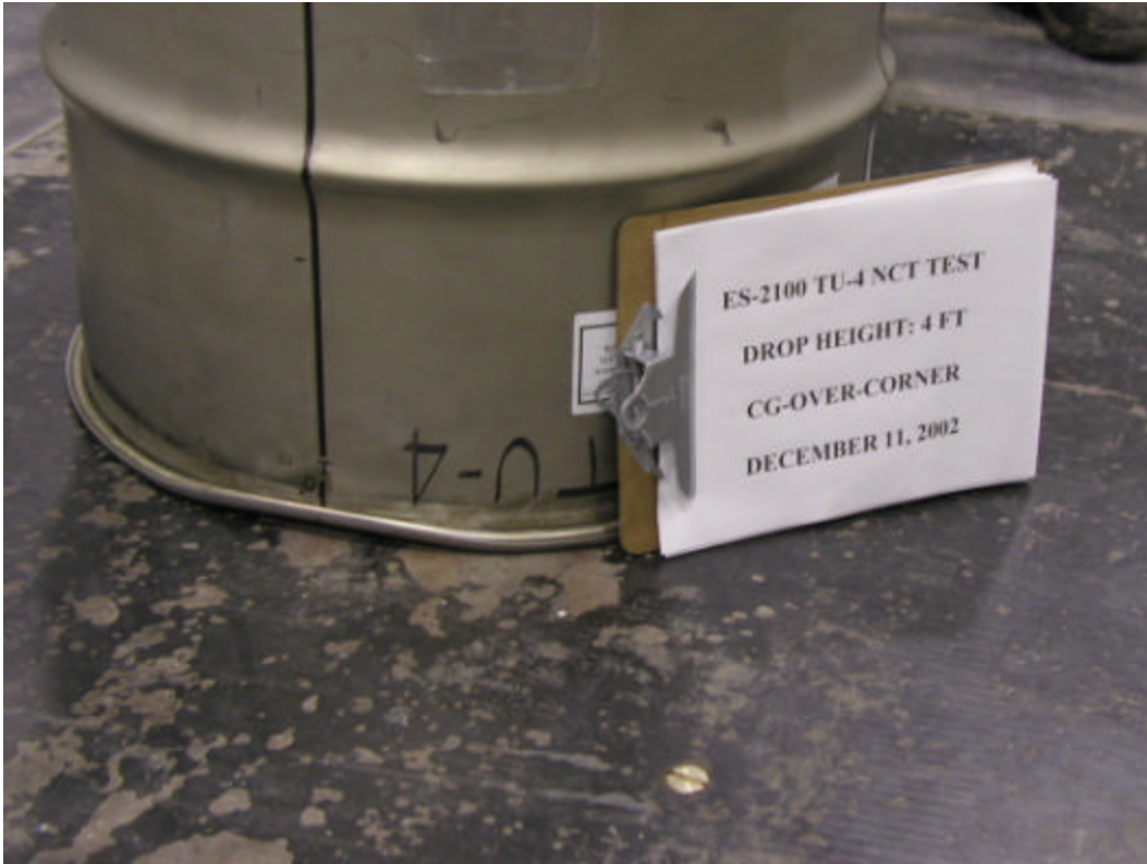
Figure H 13. Damage to lid end from the NCT CG-over-corner drop.
