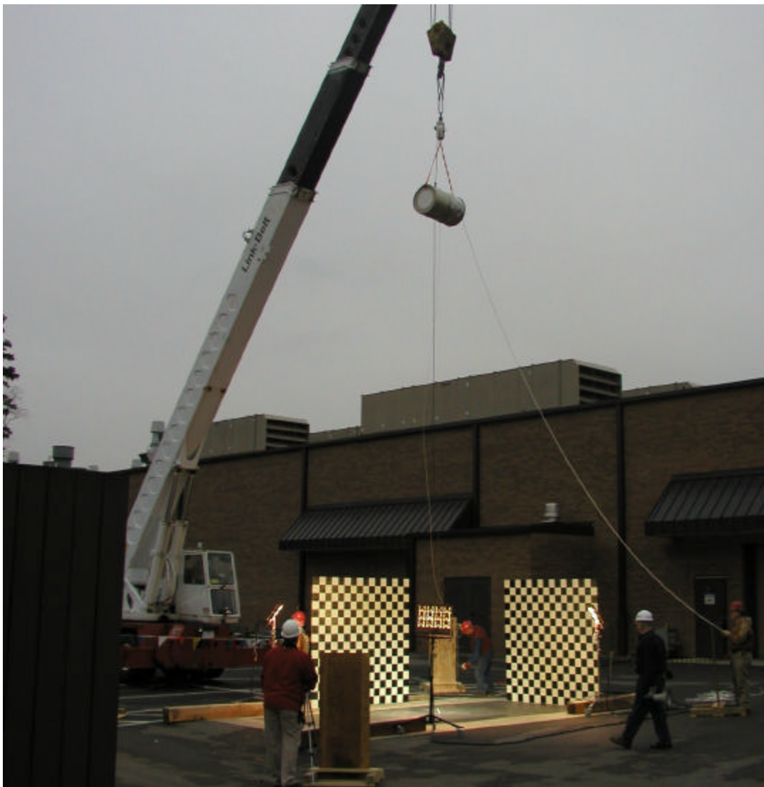
Figure 3-4 Photo showing the test setup for the HAC 9-m free drop of TU-1.
