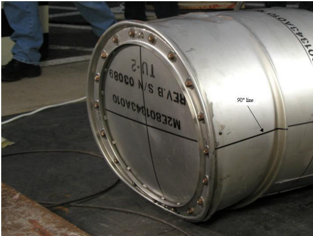
Figure 3-11 Damaged top of TU-2 resulting from the dynamic crush test.
