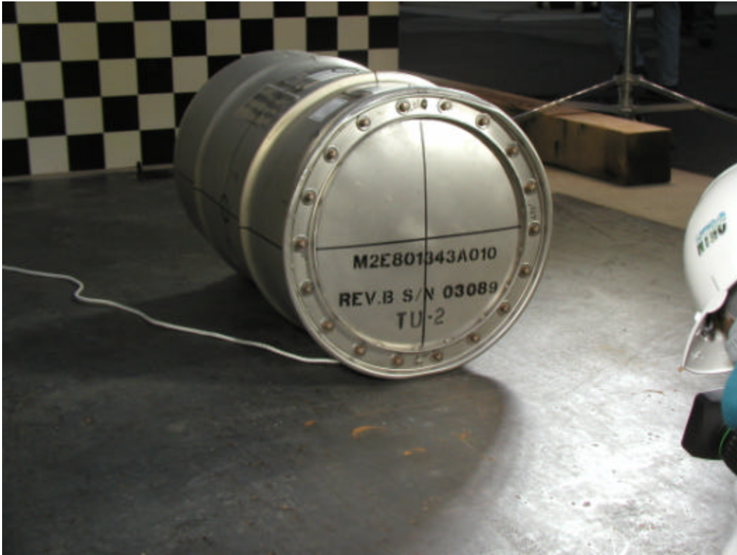
Figure F 21. End view of TU-2 lid after HAC 30-ft drop on the 0° line.
