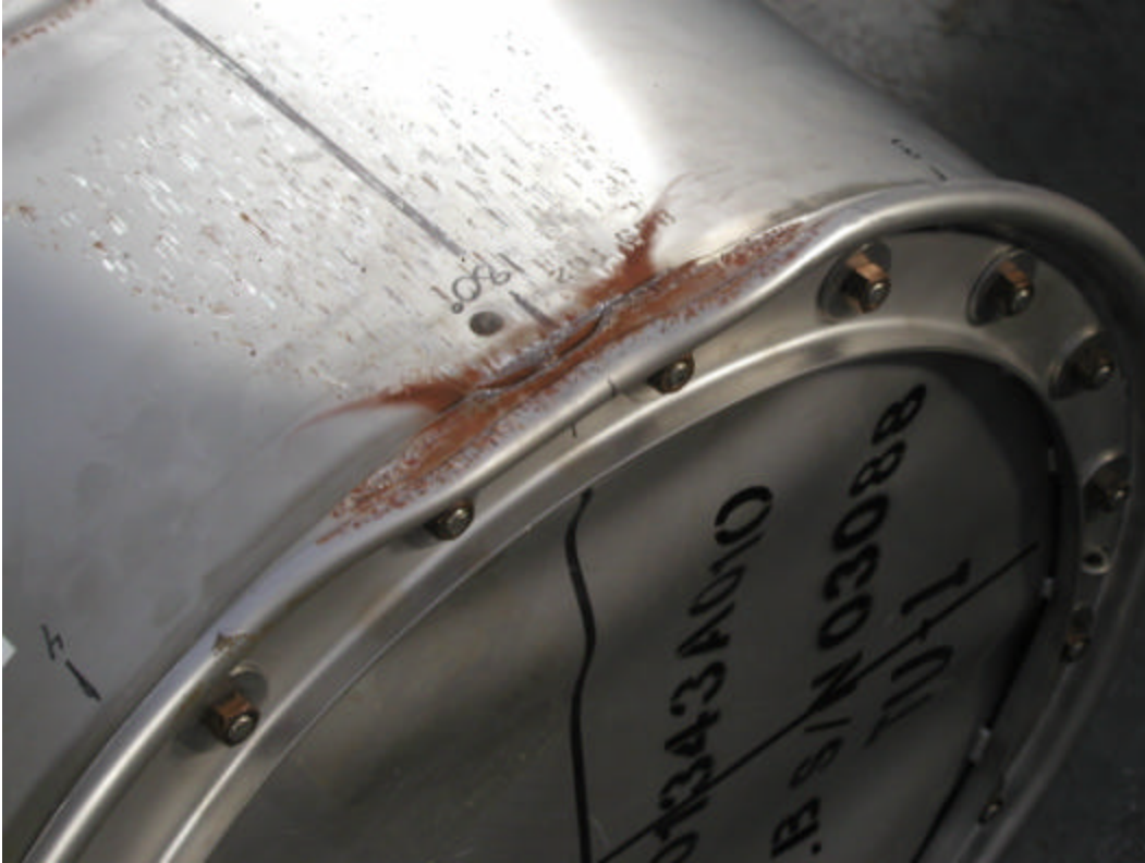
Figure E 21. Close up of damage to the lid end on the 180° line from the crush test.
