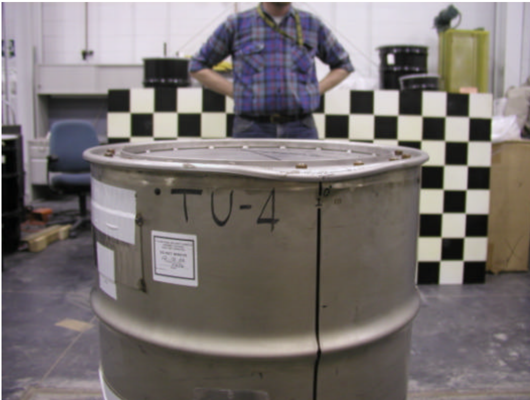
Figure H 14. Top view of damage to the lid from the NCT CG-over-corner drop.
