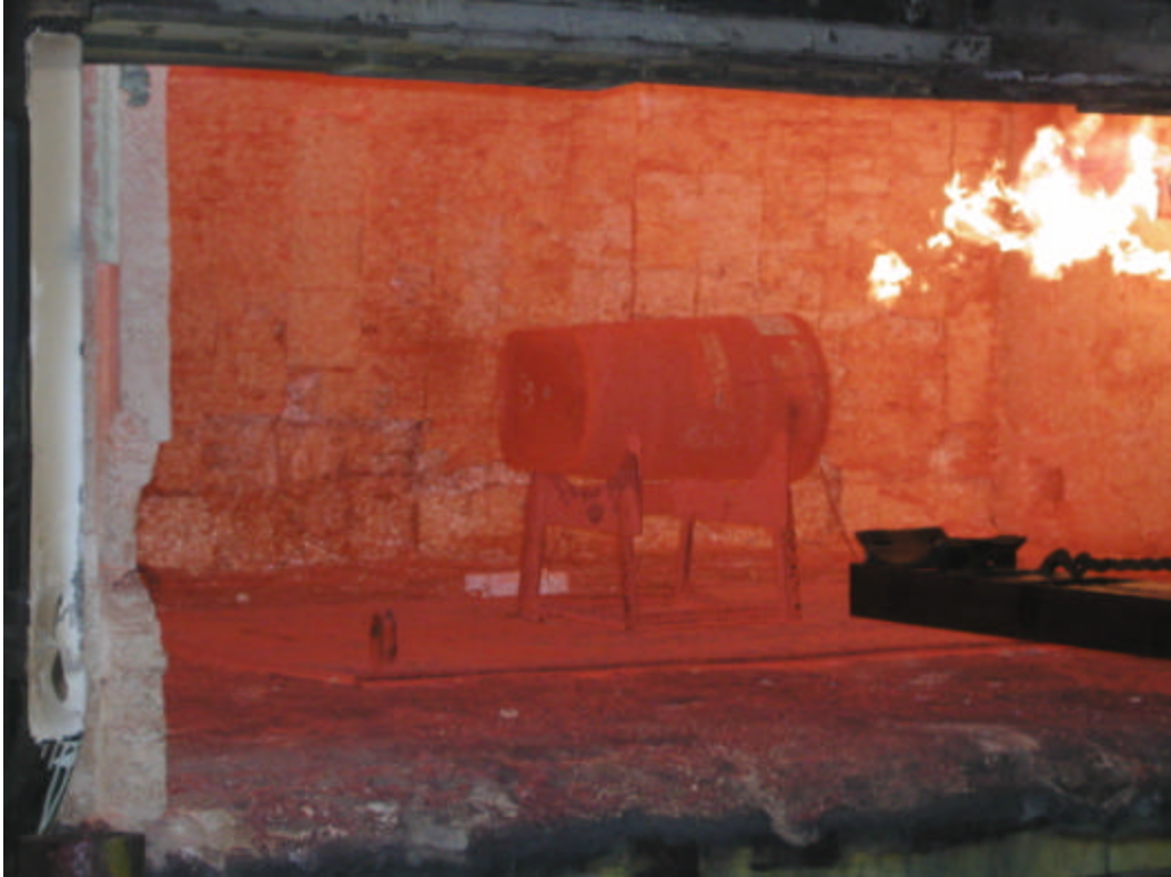
Figure G 22. Furnace Door opened to remove TU-3 from Furnace.
