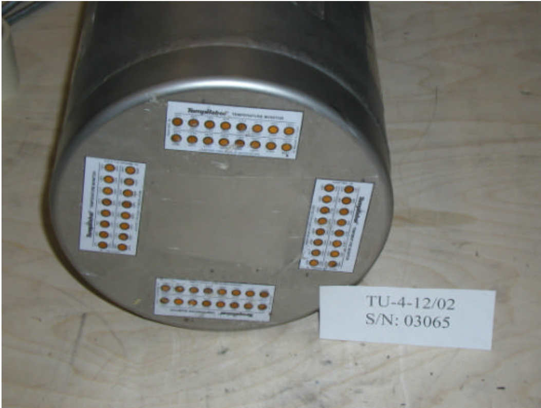
Figure H 4. Bottom of CV for TU-4 with temperature labels in place.
