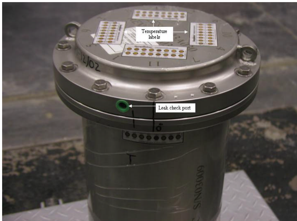
Figure E 3. Closed containment vessel (CV) showing temperature labels and leak check port
