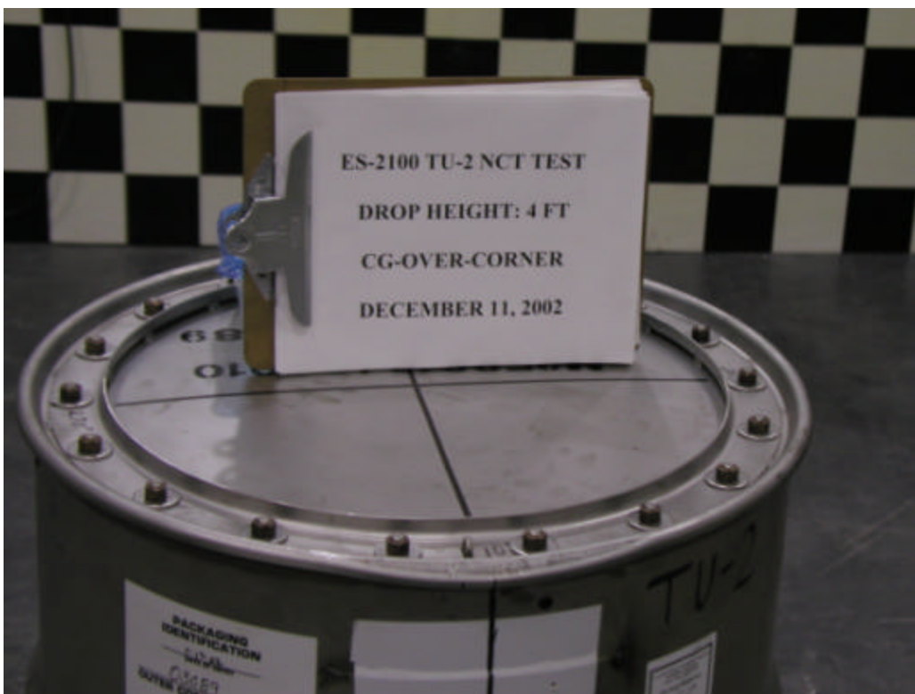
Figure F 16. Top view of damage to the lid from the NCT CG-over-corner drop.
