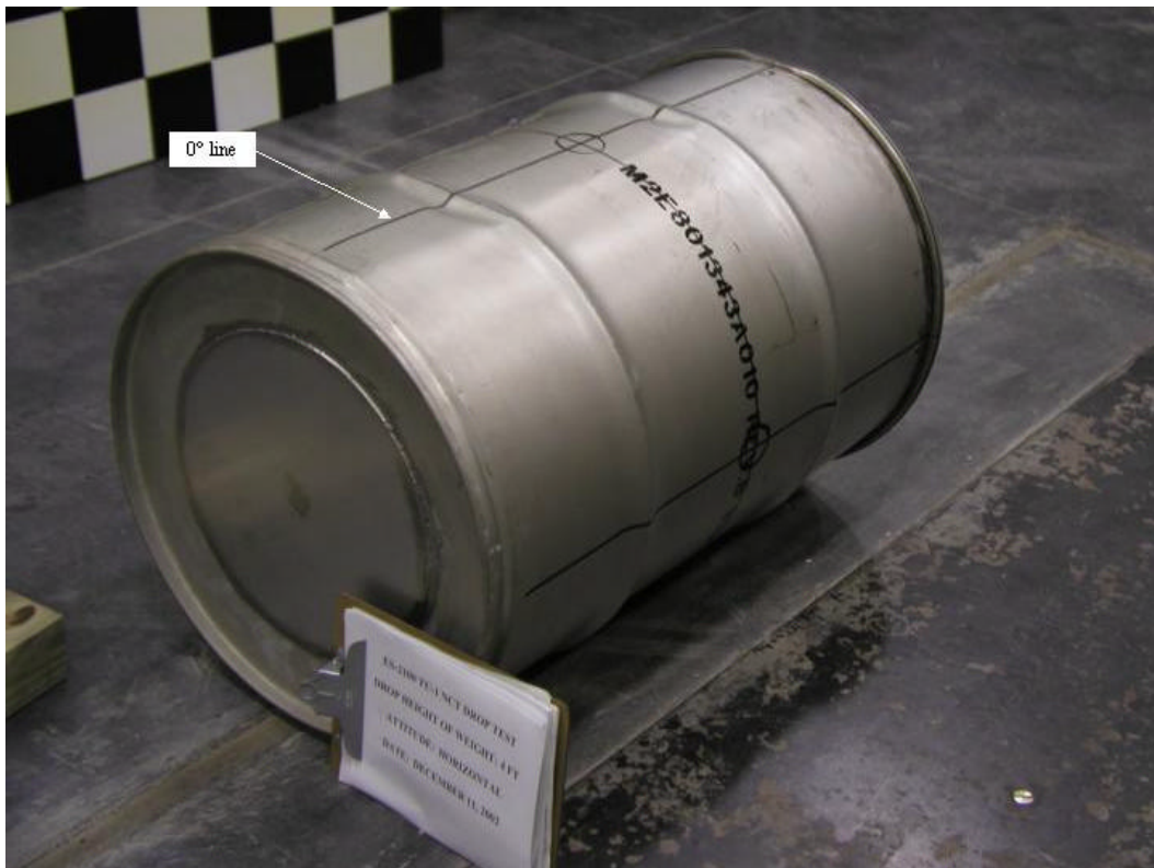
Figure E 12. Bottom end view of damage to TU-1 on the 0° line – package has been rolled 180°.
