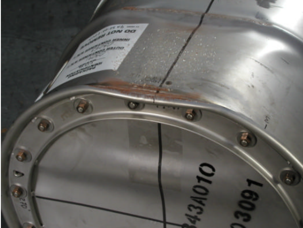
Figure G 17. Close up of damage to lid end of TU-3 along the 180° line.
