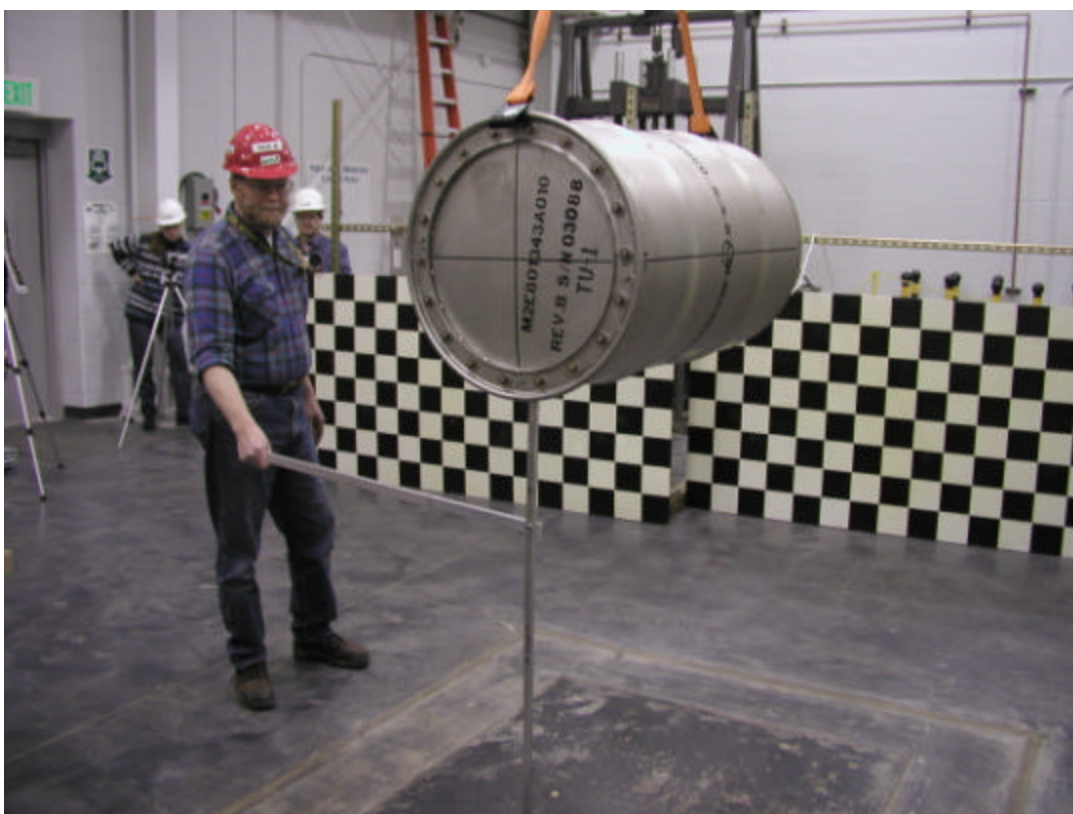
Figure 3-1 Measuring the drop height of TU-1 for the NCT drop test.
