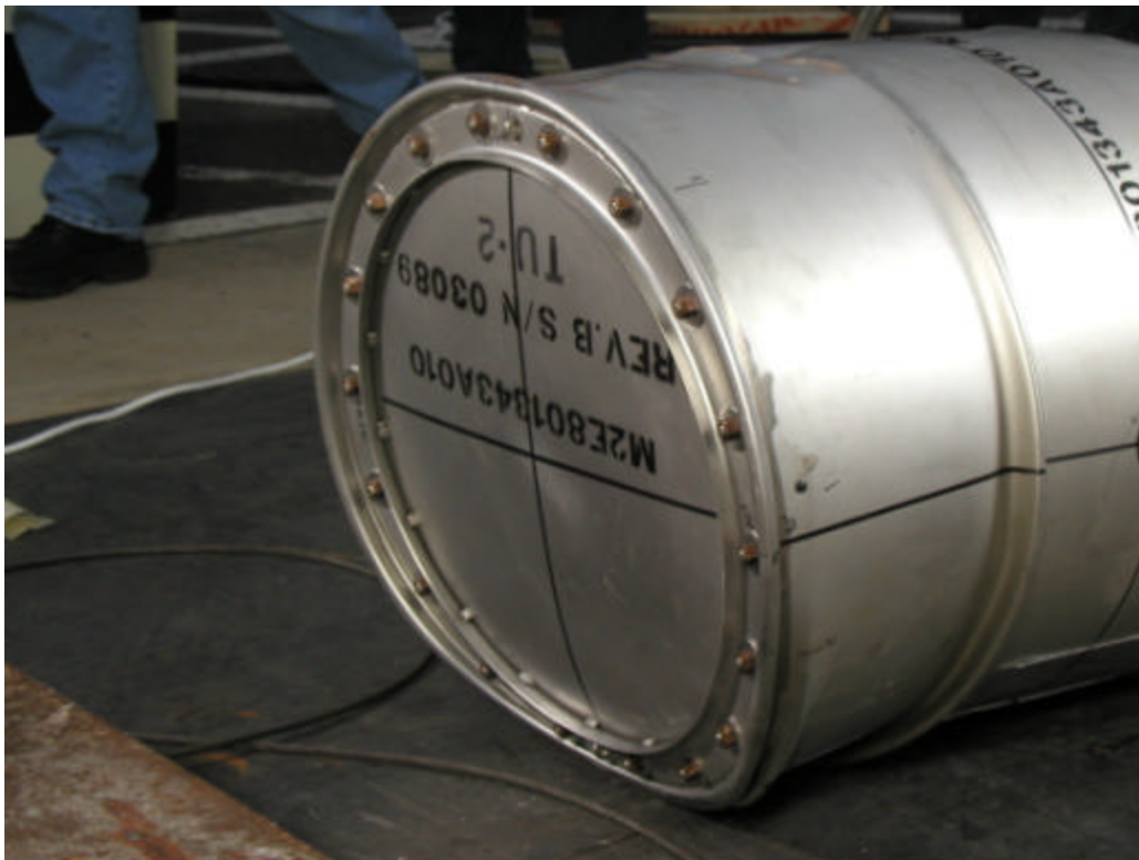
Figure F 30. View of TU-2 lid following the HAC crush test.
