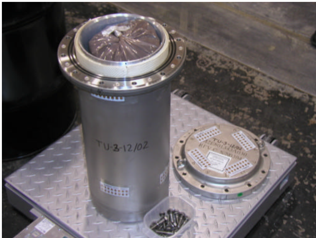
Figure G 2. Weighing the CV, Al sleeve, cap, and surrogate payload (steel shot).
