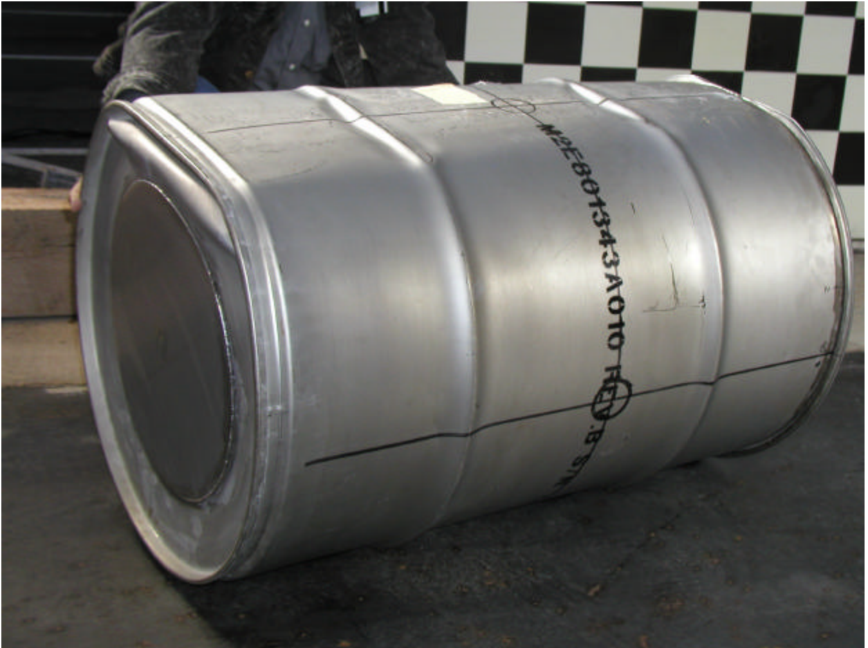
Figure 3-5 Results of dropping the TU-1 package from 9 -m onto the solid unyielding surface.
