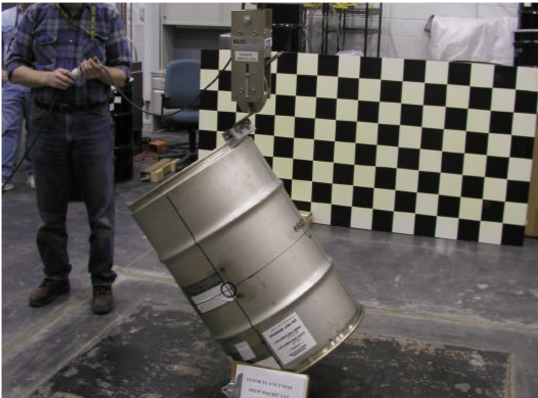
Figure H 10. Readyng TU-4 for the NCT drop test.
