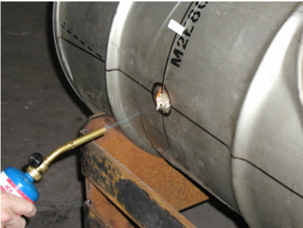
Figure 4-2 Testing thermocouple after installation.
