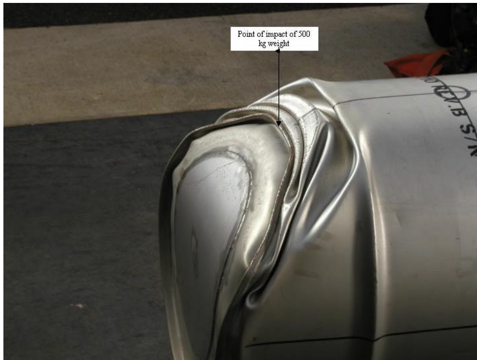
Figure 3-10 Damaged bottom of TU-2 resulting from the dynamic crush test.
