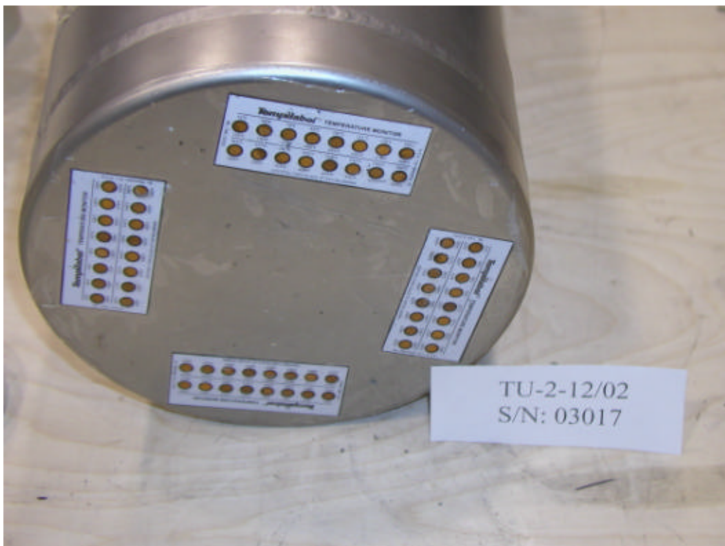
Figure F 4. Bottom of CV for TU-2 with temperature labels in place.
