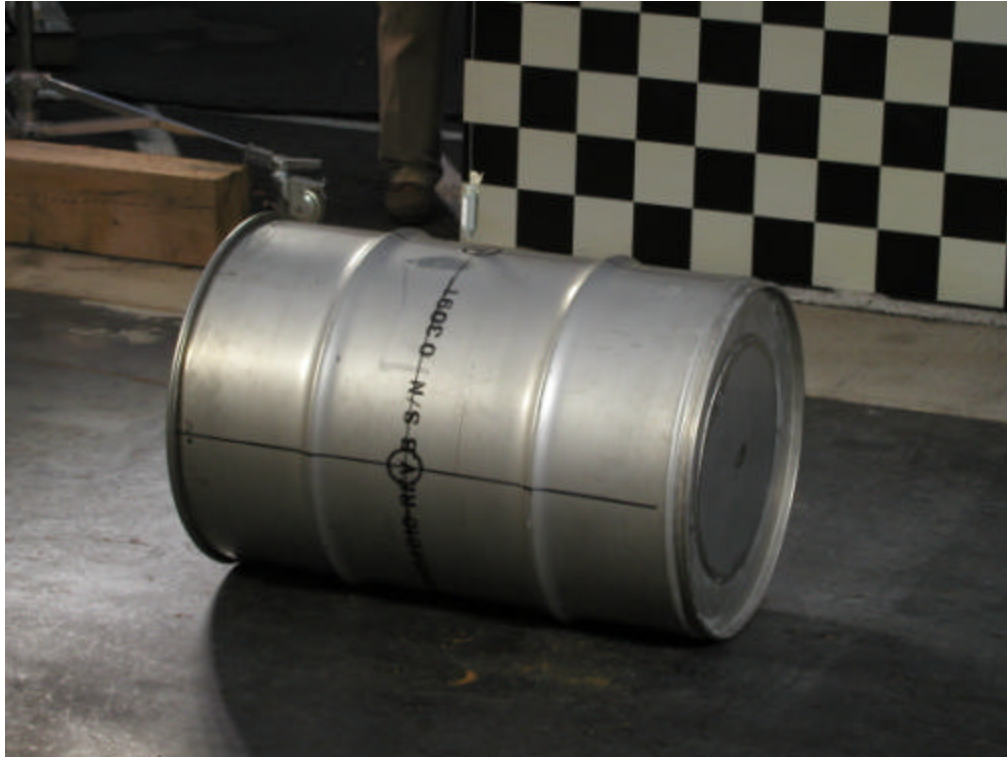
Figure G 13. Aligning the center of the 500-kg weight with the center of TU-3 prior to test.
