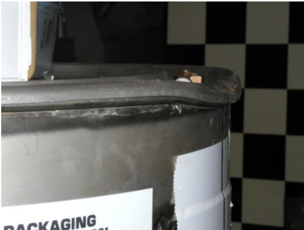
Figure F 18. Close-up of damage to edge of the lid from the CG-over-top-corner drop – side view.
