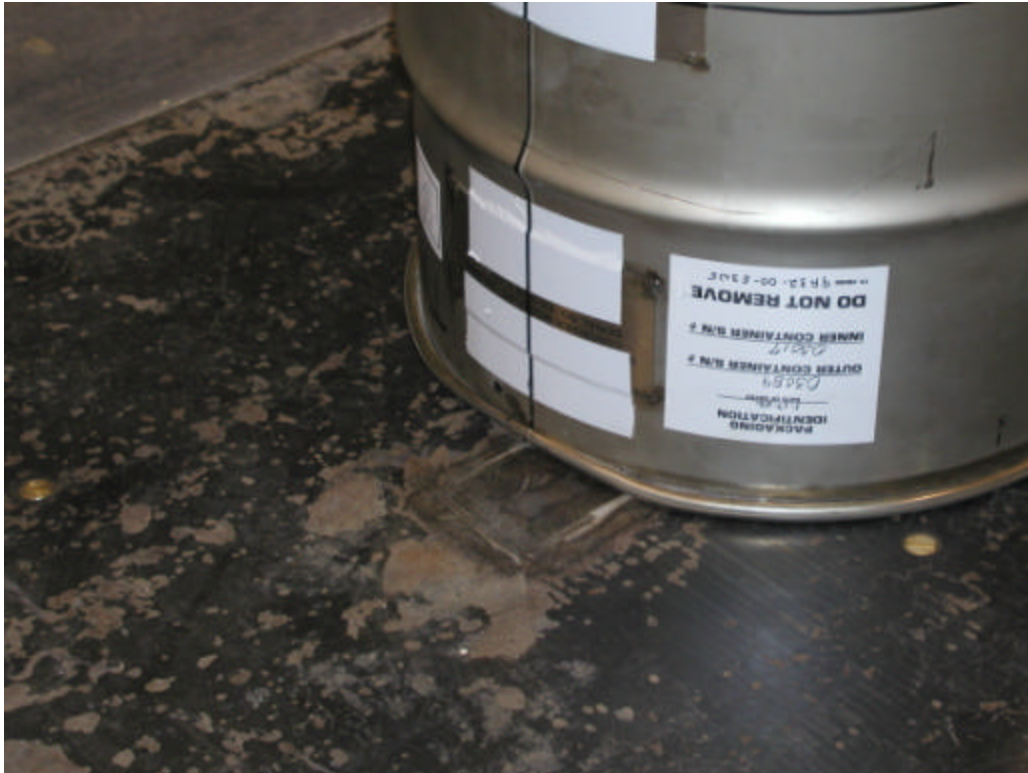
Figure F 15. Damage to the lid end from the NCT CG-over-corner drop.
