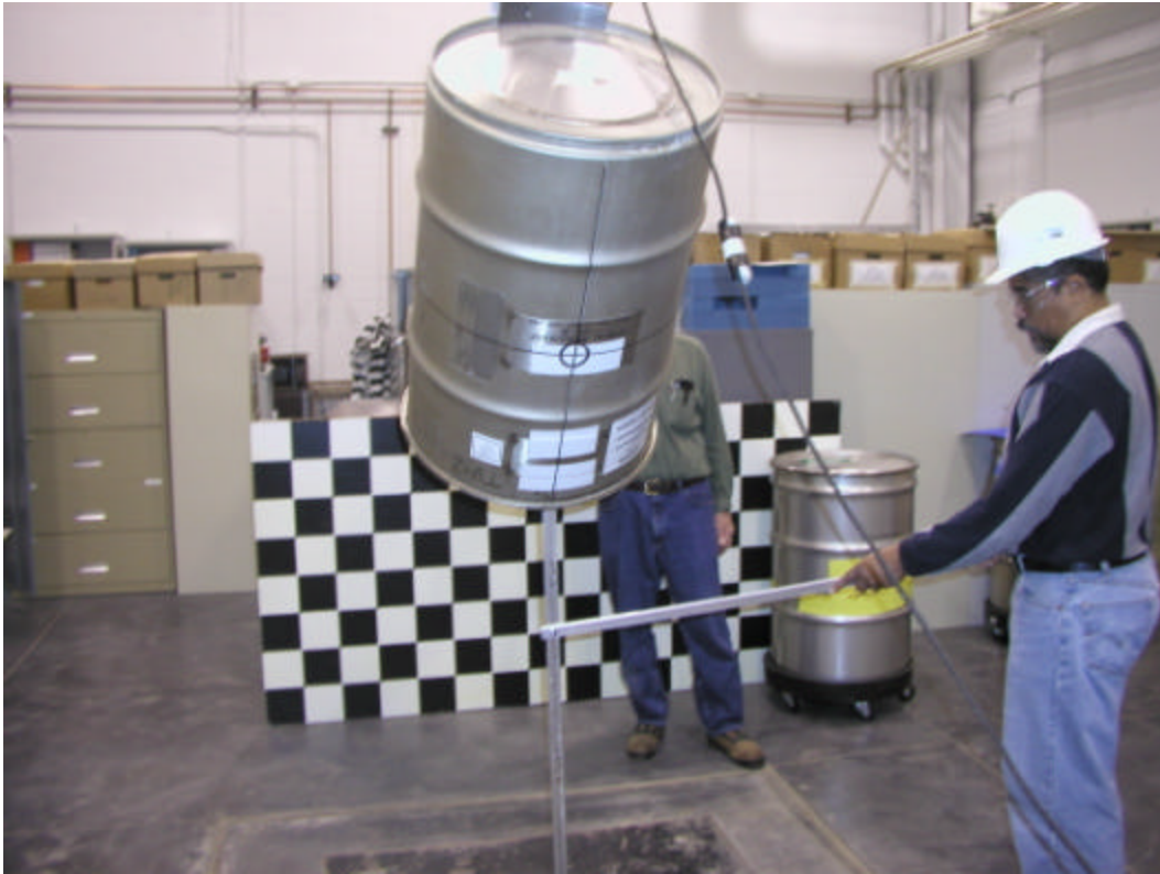
Figure F 13. Measuring the drop height of TU-2.
