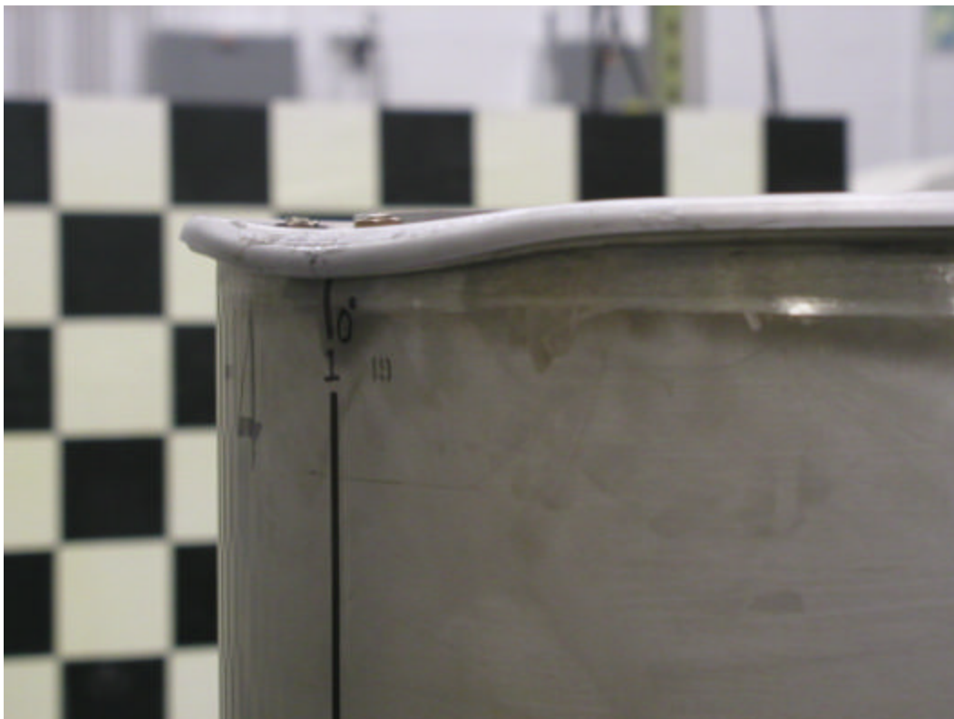
Figure H 16. Close-up of damage of the lid from the CG-over-corner drop – right side view.
