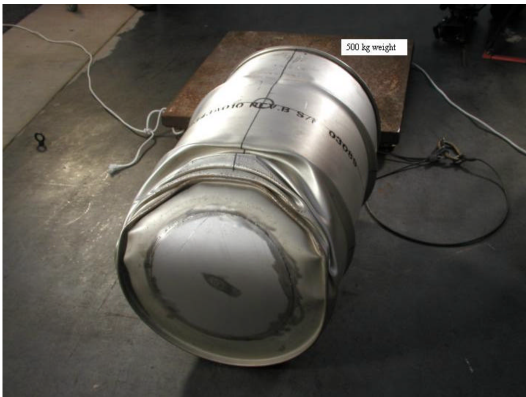
Figure F 28. Damage to the bottom edge of TU-2 after being hit with the 500 kg crush weight.
