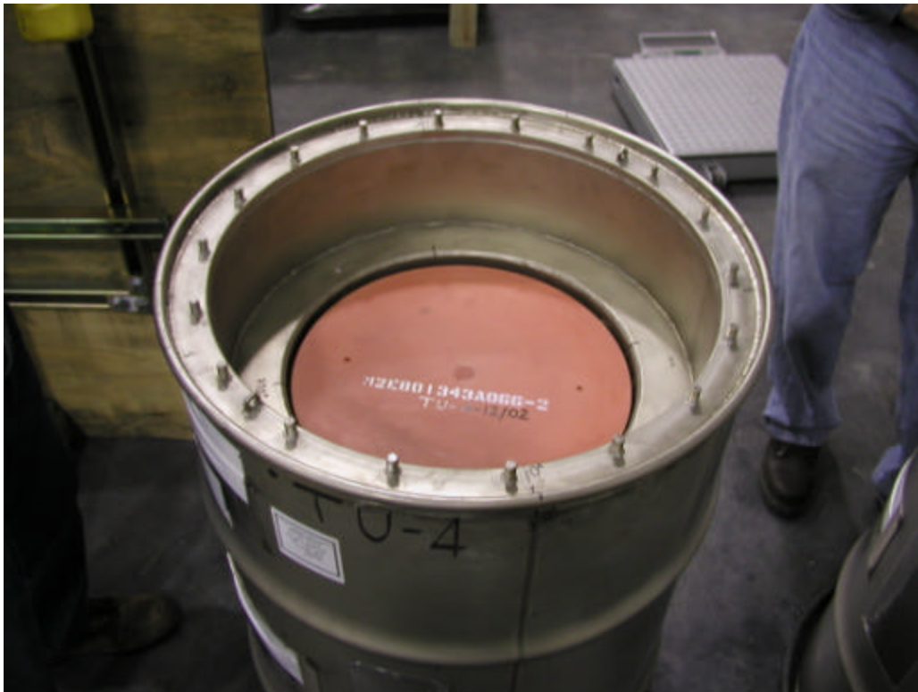
Figure H 7. View of open TU-4 with polyurethane top in place above the CV.
