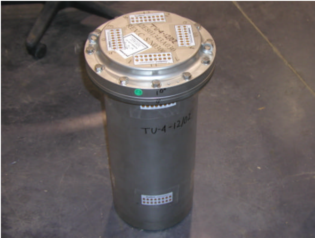
Figure H 3. Sealed CV for TU-4 with temperature labels in place.
