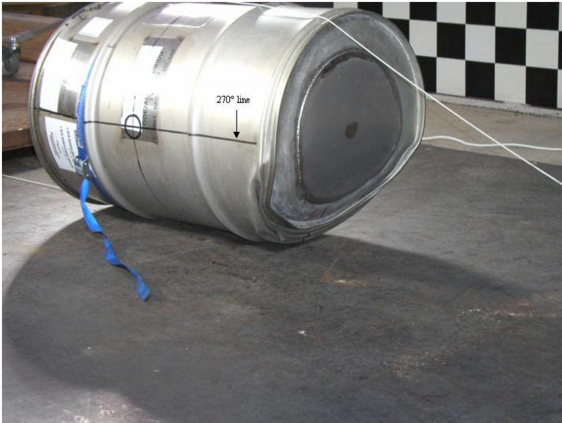
Figure 3-15 Results of the dynamic crush test as viewed from the bottom end of TU-4.
