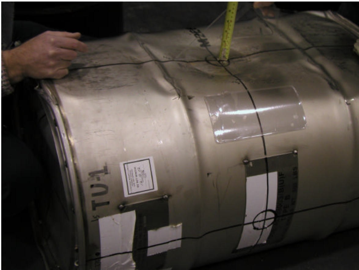
Figure 3-16 Damage produced in the first puncture test of TU-1.
