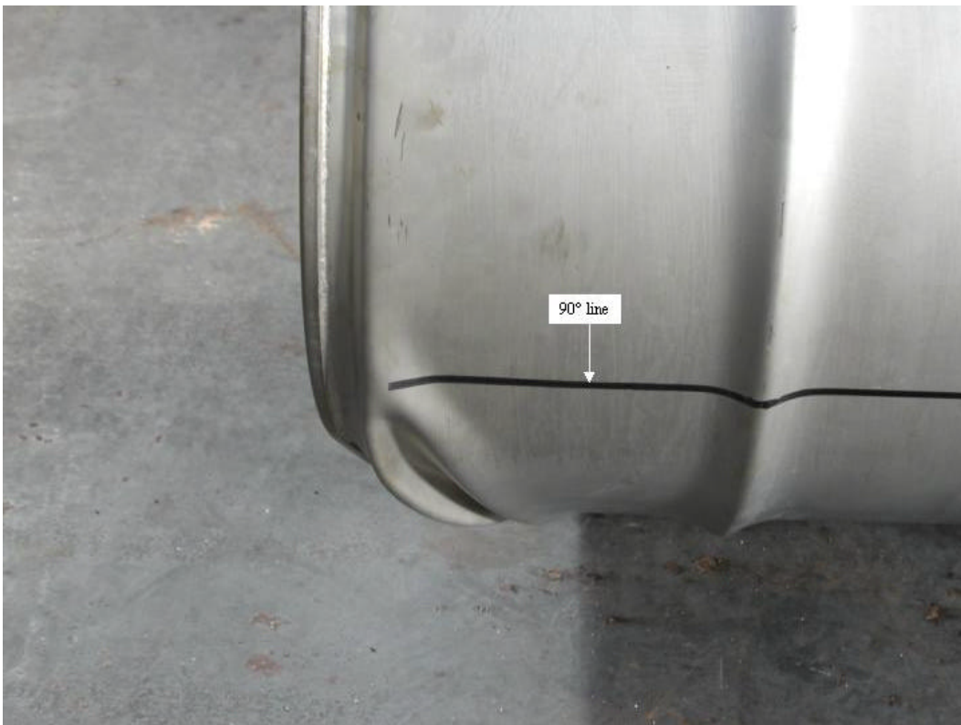
Figure H 25. Detail of the damage to the bottom of TU-4 from the crush test.
