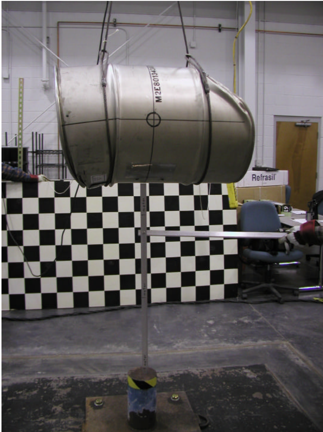
Figure F 35. Measuring the height of TU-2 above the punch.
