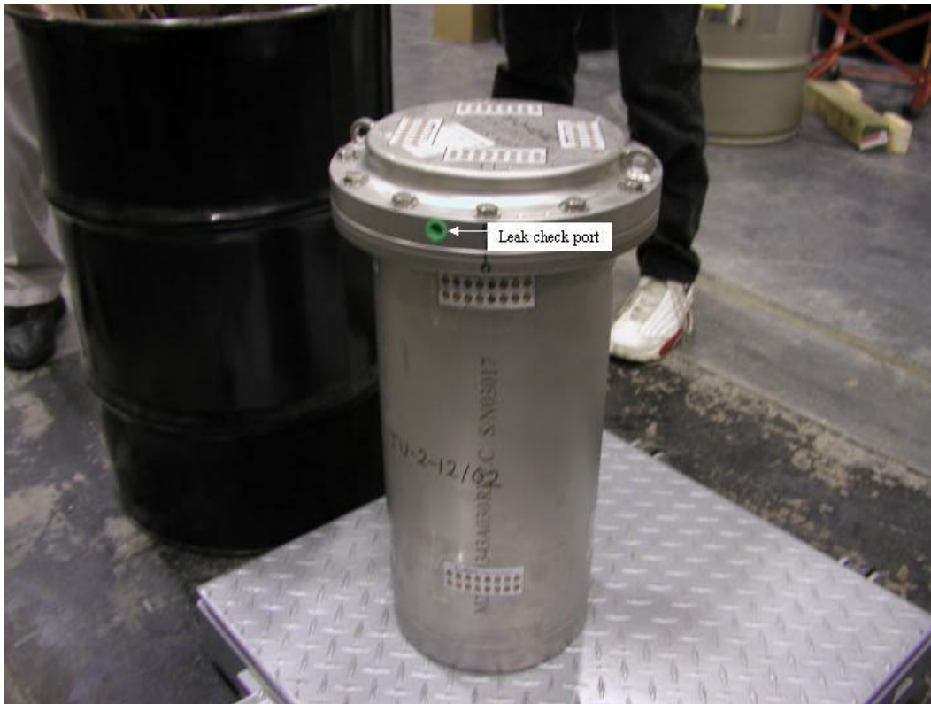
Figure F 3. Sealed CV for TU-2 with temperature labels in place.
