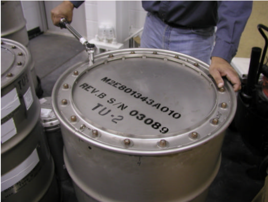
Figure F 9. Torquing the bolts on TU-2.
