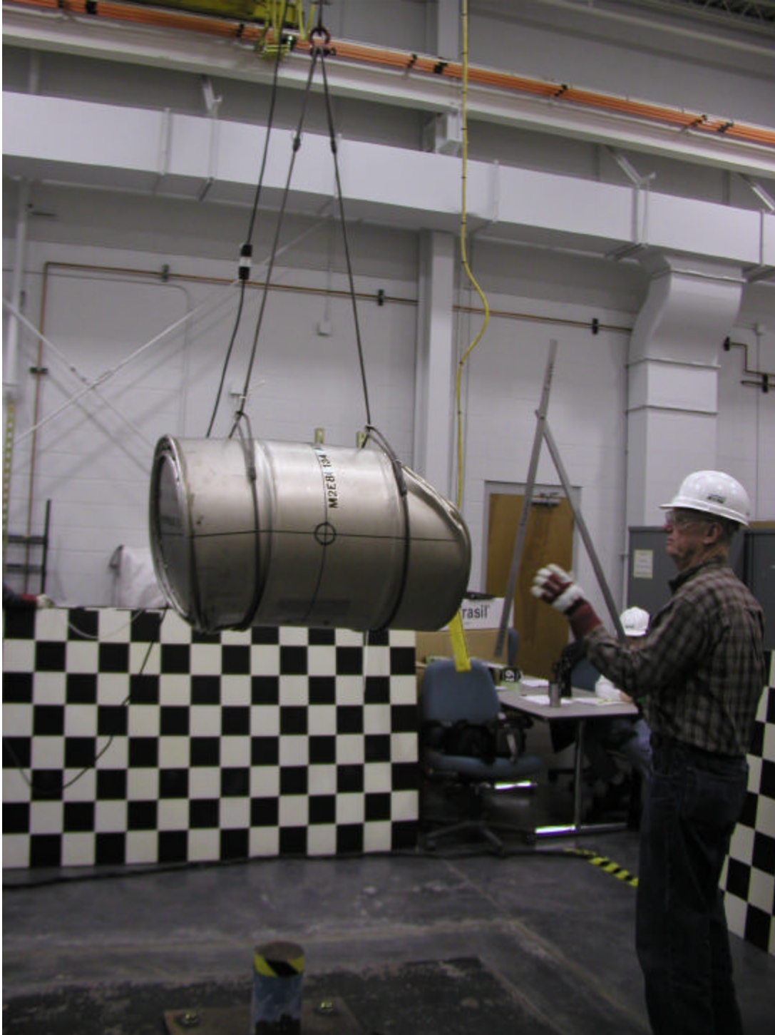
Figure F 34. Positioning TU-2 over the punch.
