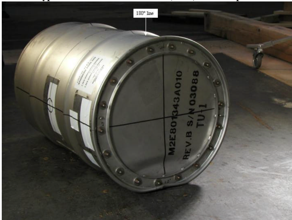
Figure E 13. End view of TU-1 lid after the HAC 30-ft drop on the 0° line.
