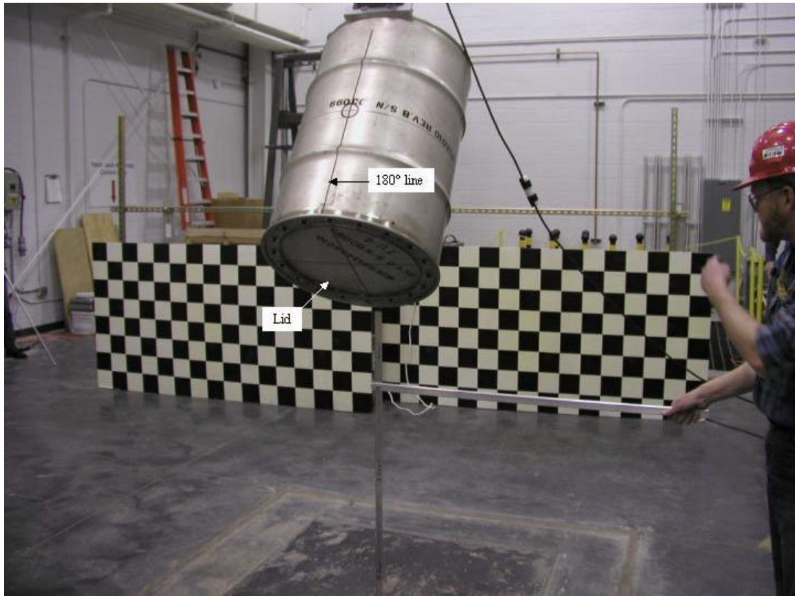
Figure 3-2 Measuring the drop height to the top of TU-4 for the NCT drop test.
