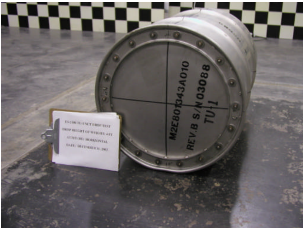
Figure E 10. TU-1 package on the drop pad after NCT drop test.
