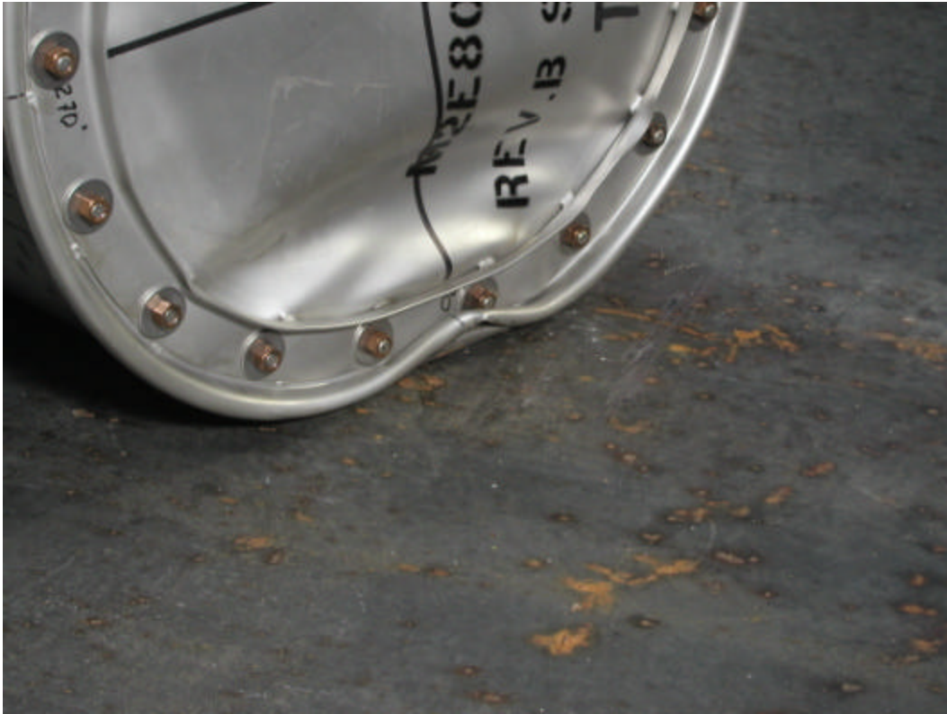
Figure G 15. Close up of damage to the lid end on the 0° line from the crush test.
