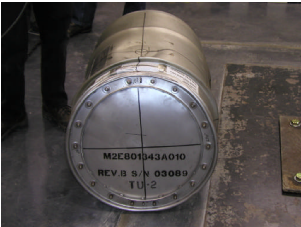
Figure F 38. Damage to TU-2 from the punch test as viewed from the top end of the package.
