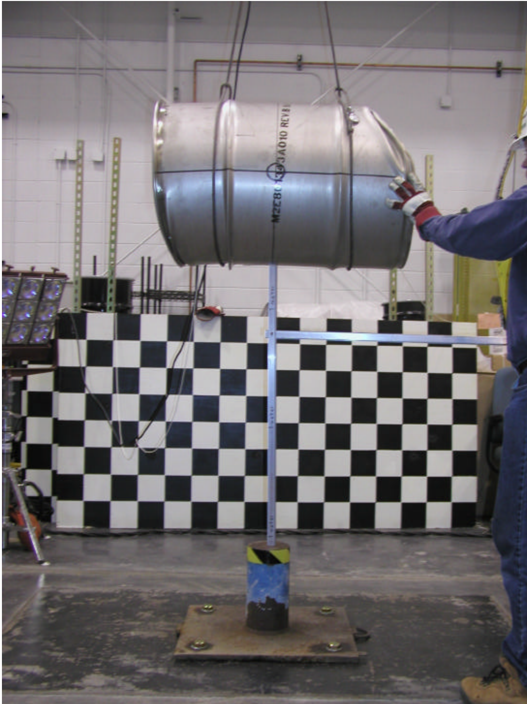
Figure H 28. Measuring the drop height above the punch.
