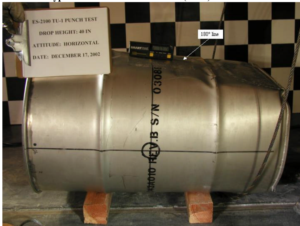
Figure E 26. Measuring the angle of the of the top (180° line) surface relative to the horizontal 0° line.
