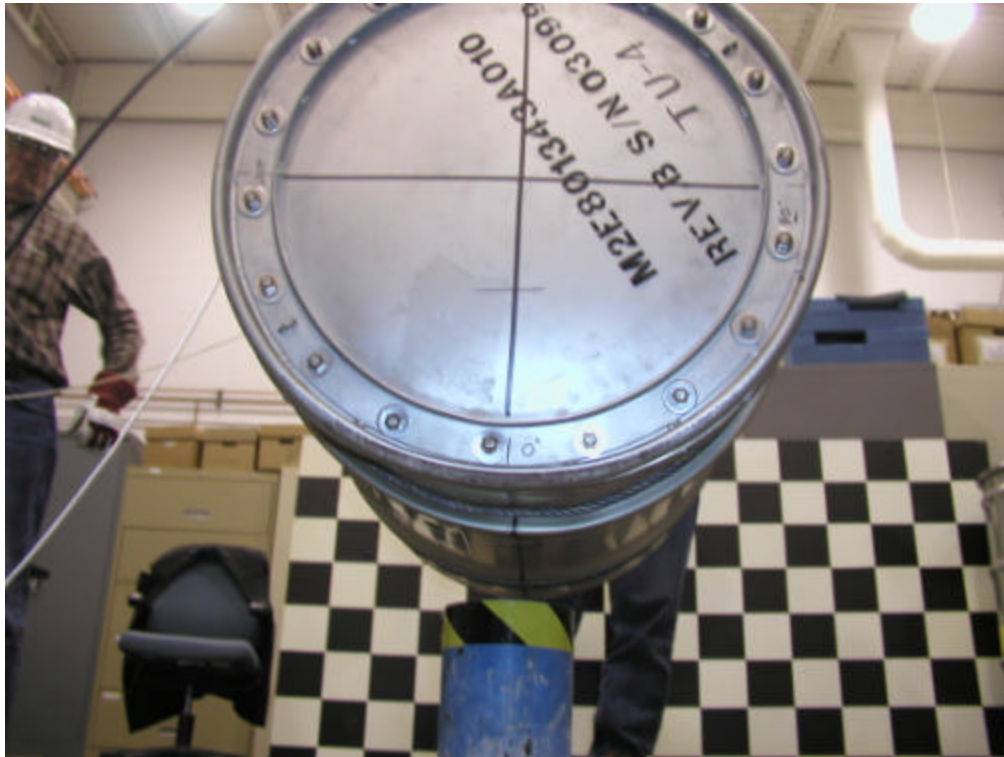
Figure H 26. Alignment of TU-4 package over the punch.
