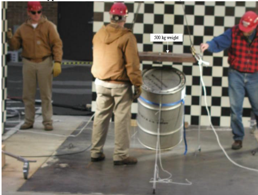
Figure H 17. Aligning the 500 kg crush weight above the TU-4 package.
