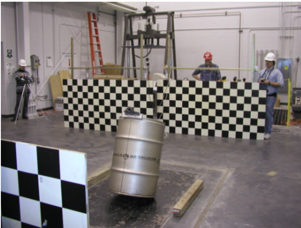
Figure F 14. View of the drop test of TU-2 at the moment of impact.
