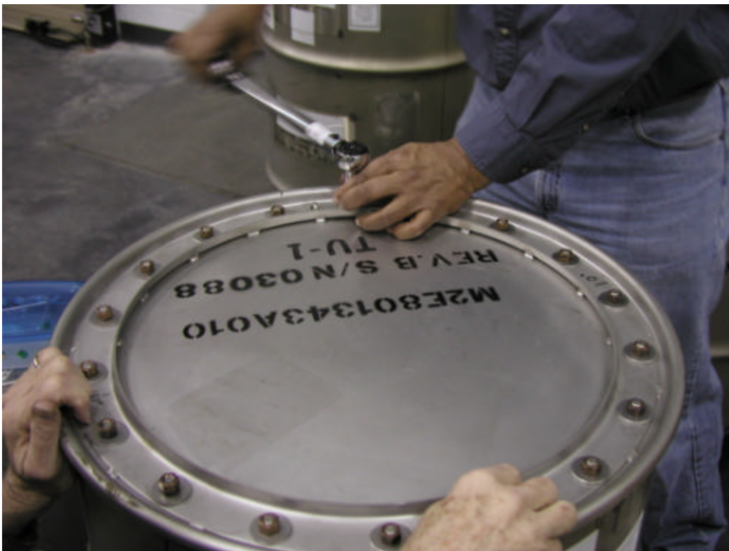
Figure E 8. Torquing the bolts on TU-1 lid.
