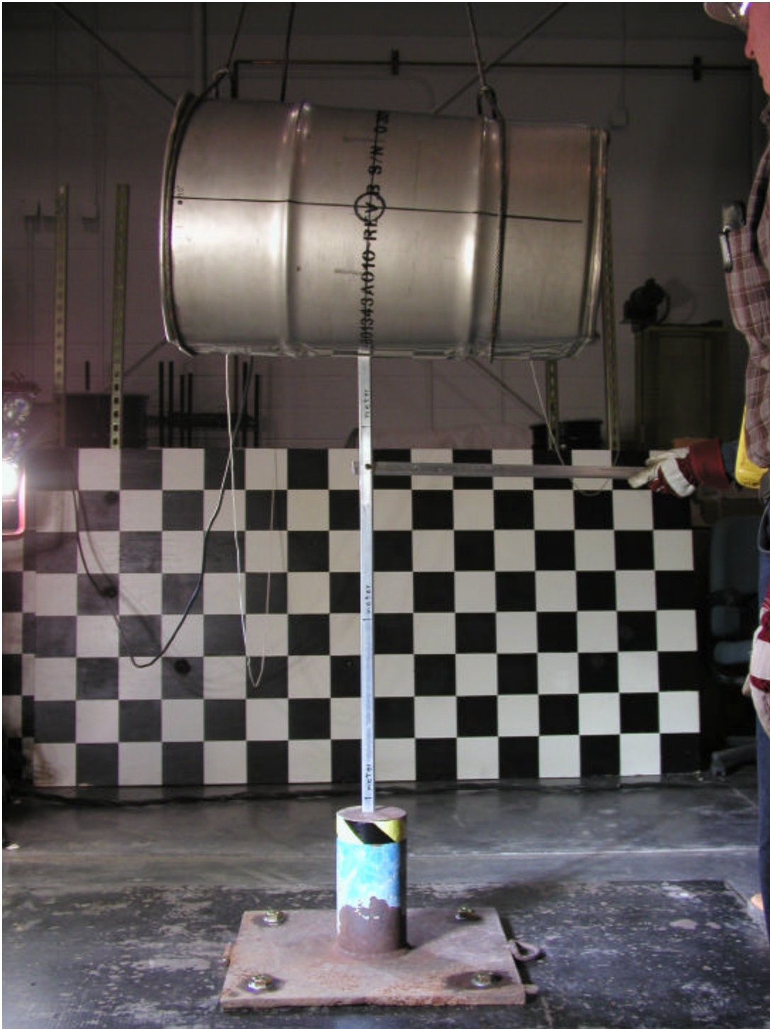
Figure G 18. Measuring the drop height of TU-3 prior to dropping on the steel punch.
