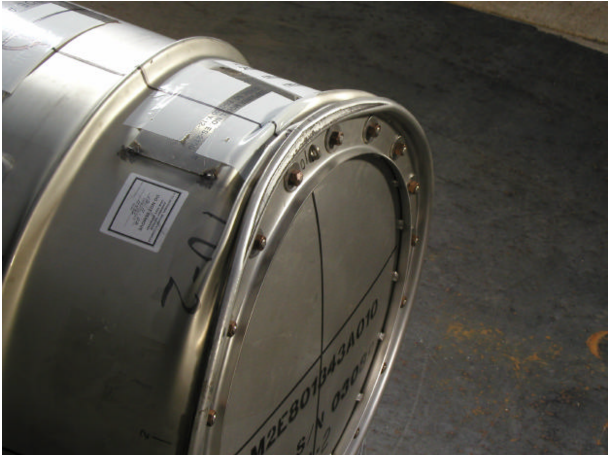
Figure 3-7 Results of dropping TU-2 in a CG-over-corner drop from 9 m.
