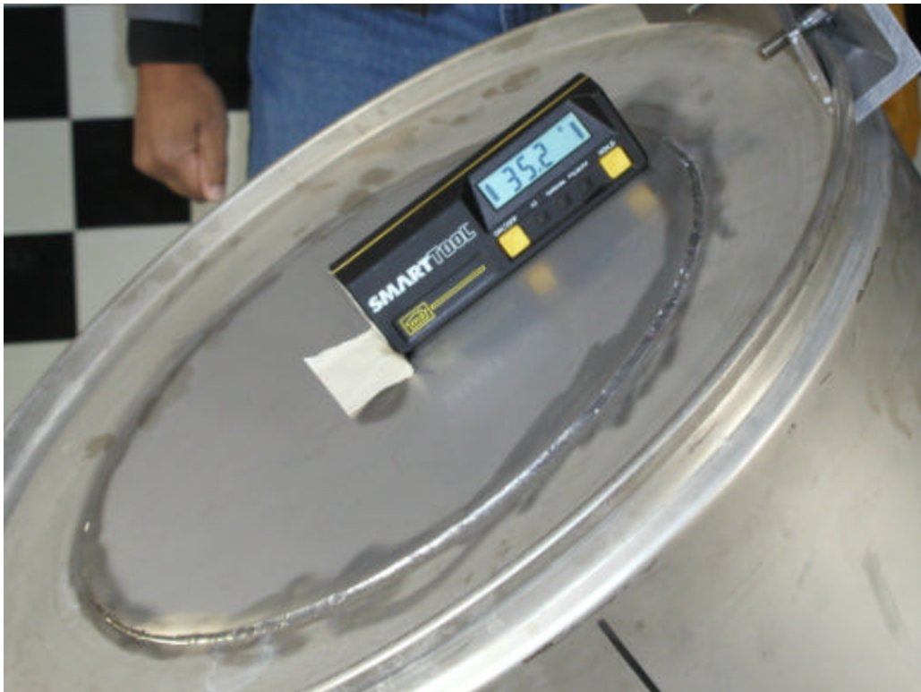
Figure F 20. Measuring the drop angle on the bottom of TU-2 prior to drop test.
