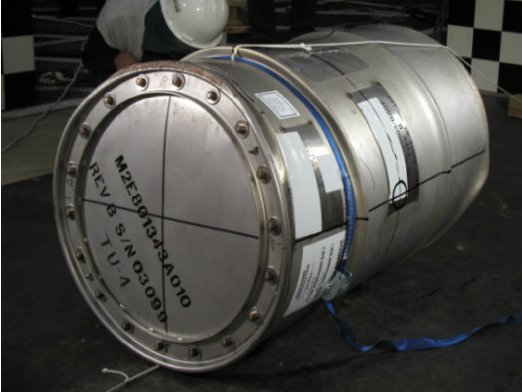
Figure H 20. View of TU-4 lid following the HAC crush test.
