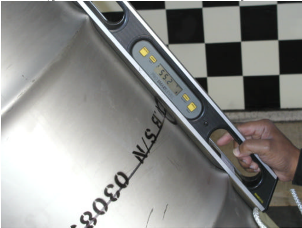
Figure F 19. Measuring the drop angle on the side of TU-2 prior to drop test.
