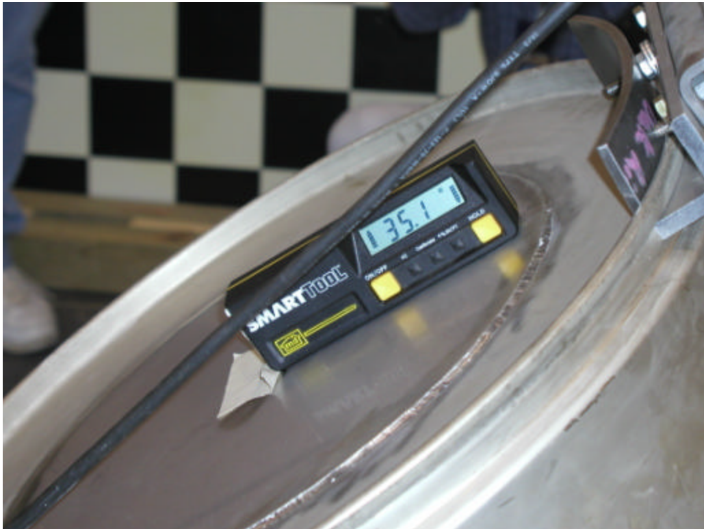
Figure F 12. Measuring the drop angle on the bottom of TU-2.
