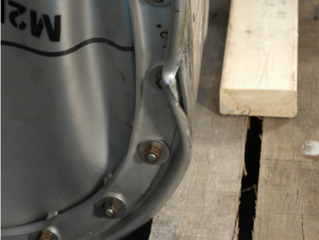
Figure E 23. Detail of damage to the lid at the 0° line after the crush test.
