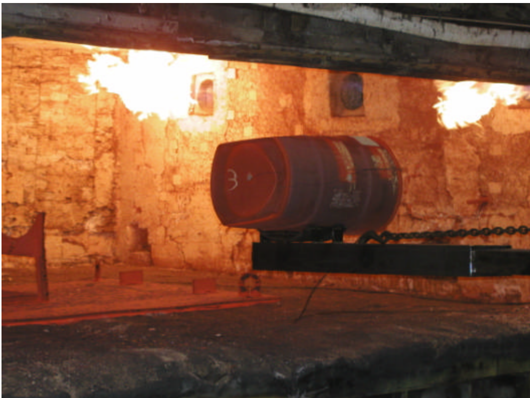
Figure G 23. Removing TU-3 from Furnace.
