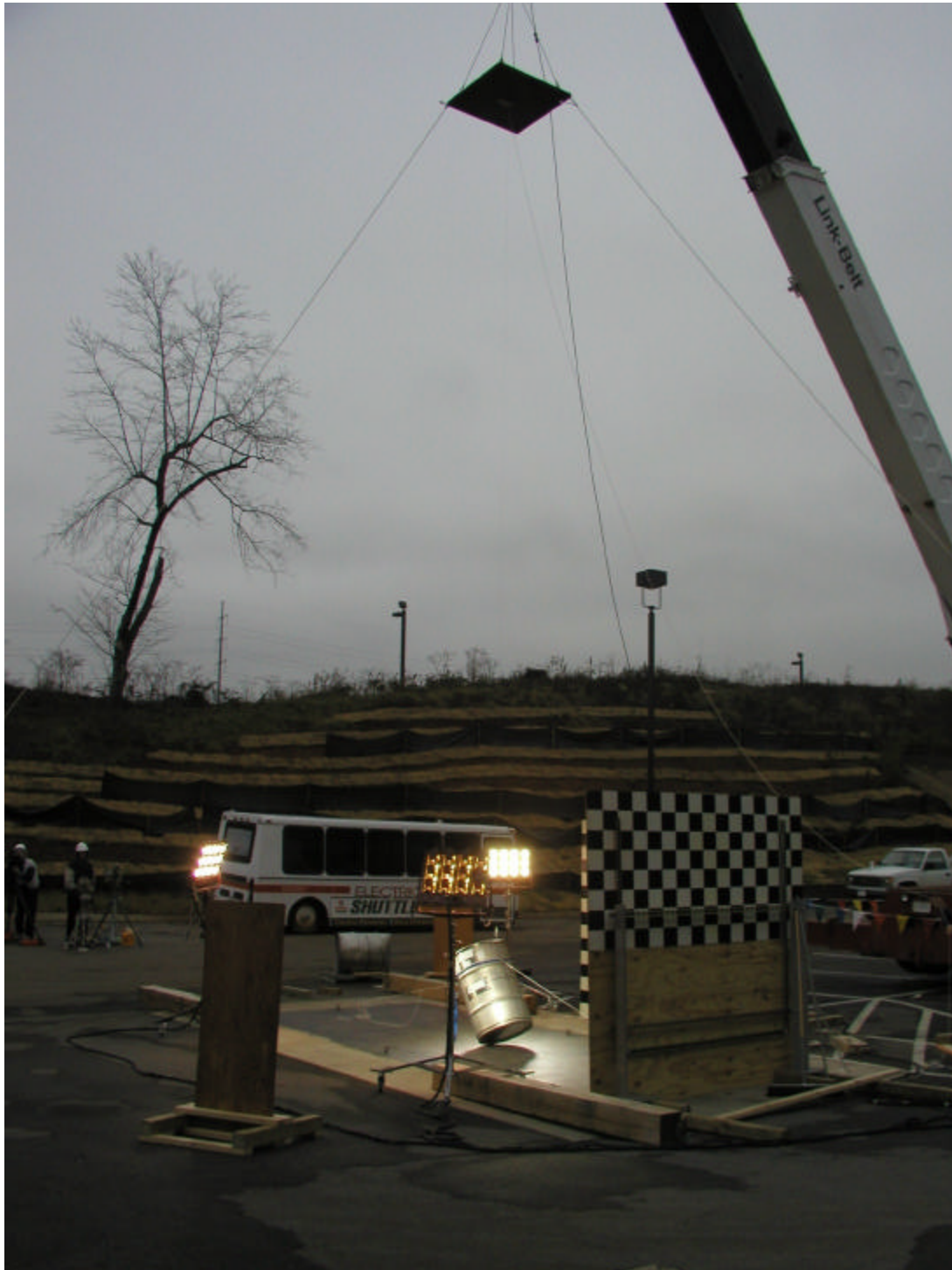
Figure H 19. Overall setup for the dynamic crush test on TU-4 package.
