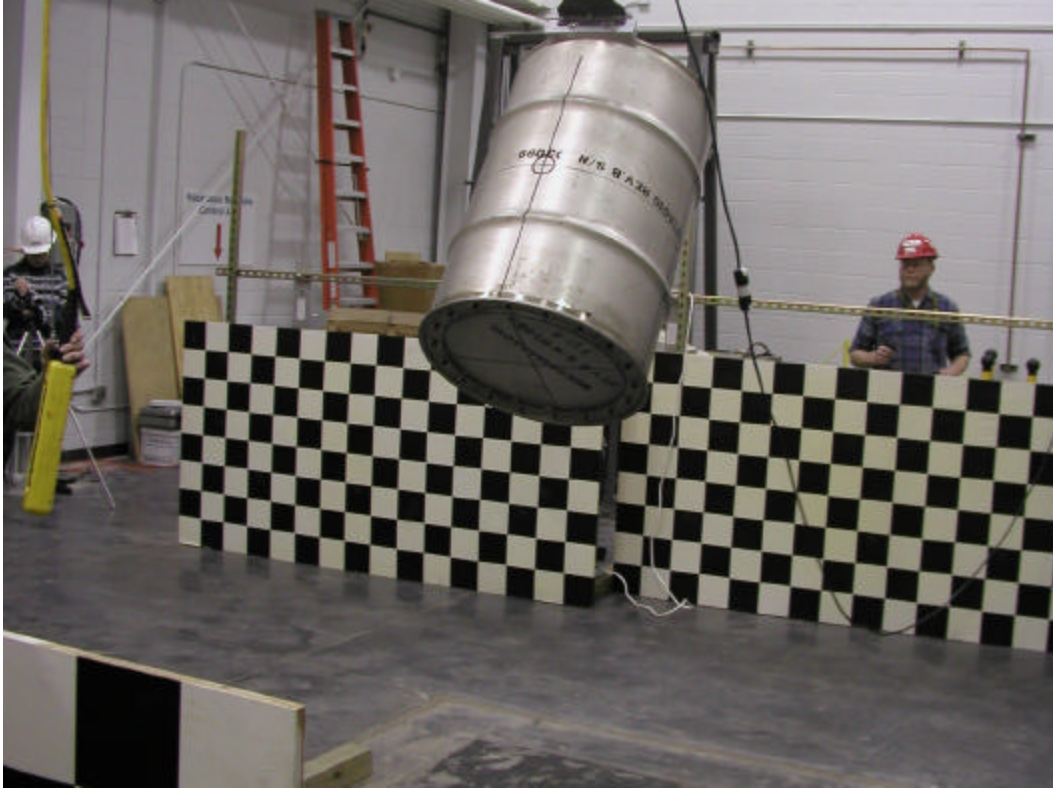
Figure H 11. TU-4 suspended just prior to drop.
