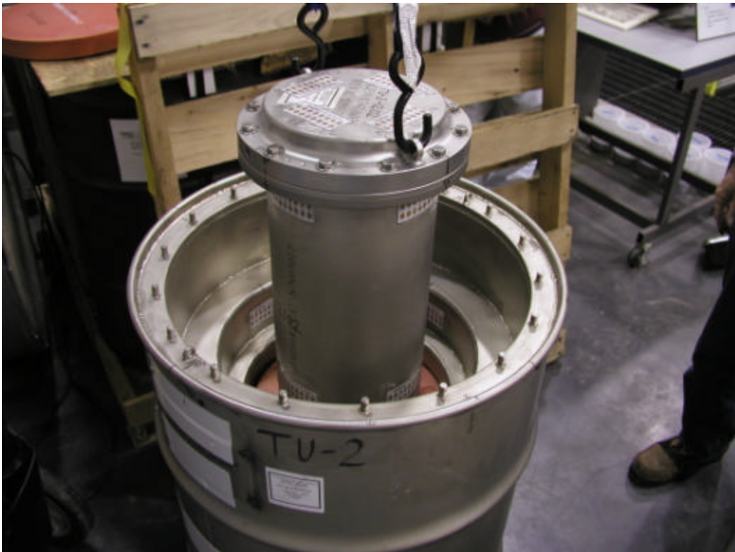
Figure F 6. Lowering the CV into TU-2.
