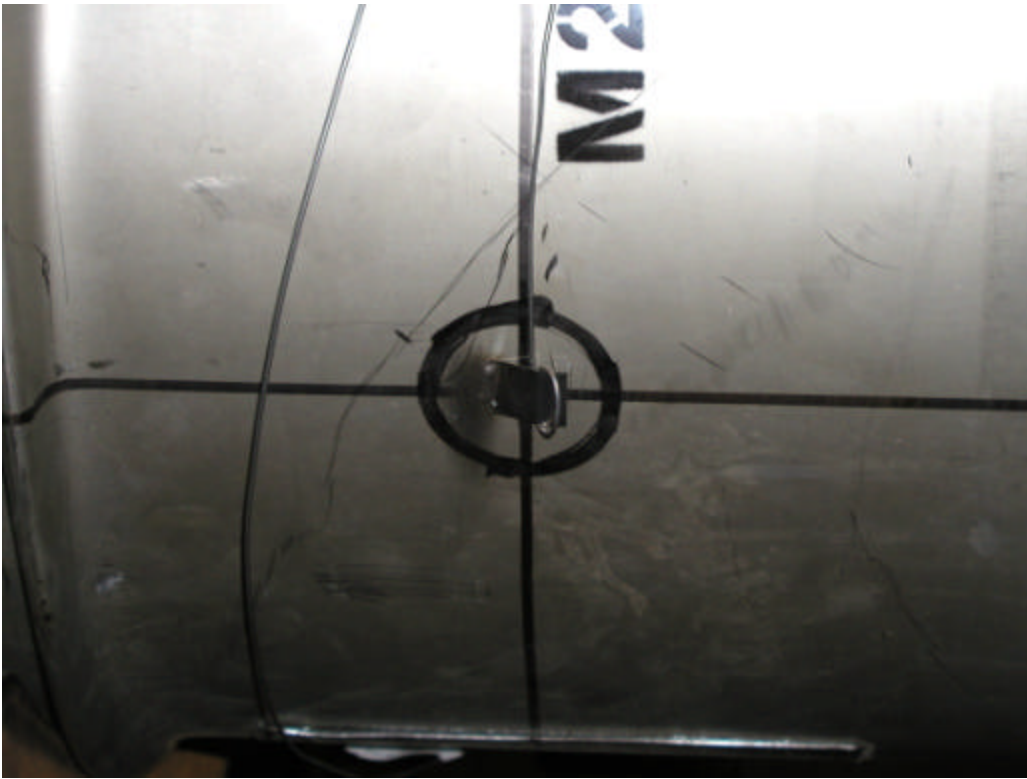
Figure 4-1 Installation of thermocouple under retainer clip.
