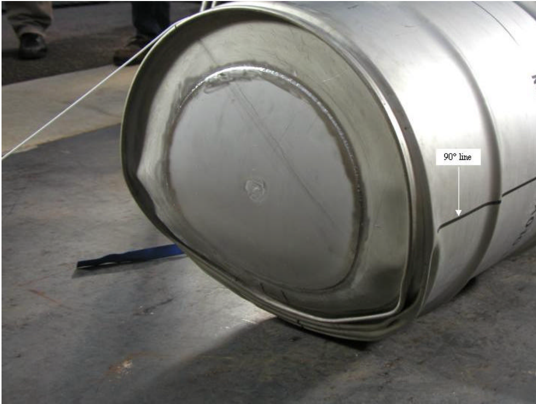
Figure H 24. Close-up of damage to the bottom of TU-4 from the crush test.
