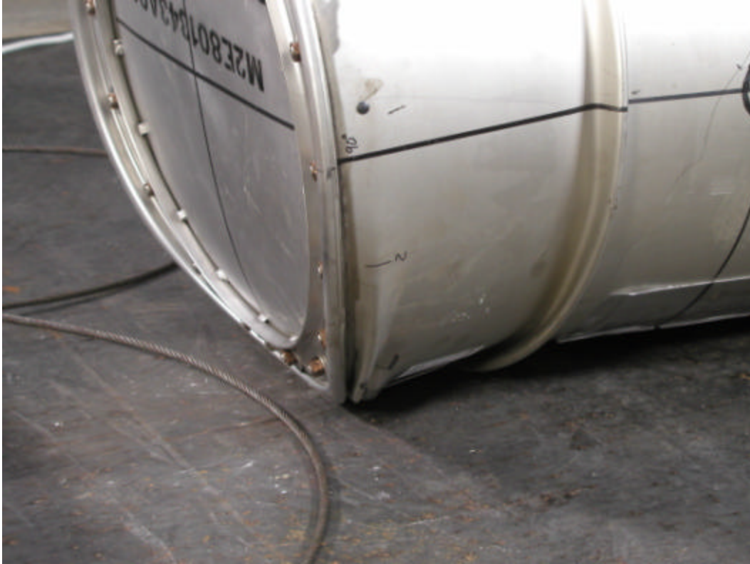
Figure F 31. Close-up of damage to lid of TU-2 following the crush test.
