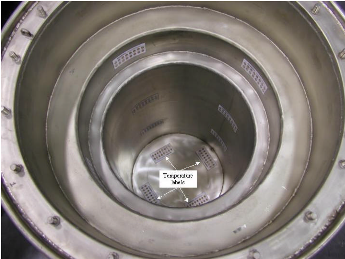
Figure 2-3 Preparation of drum with affixed temperature labels.
