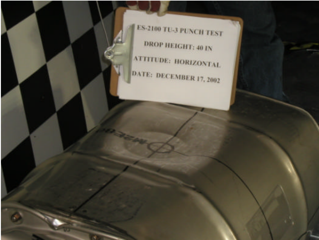
Figure G 20. Damage to TU-3 from the drop onto a punch over the CG on the 0° line.
