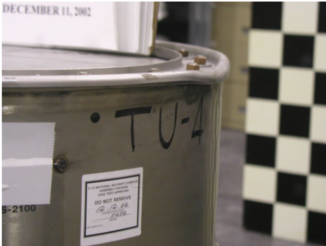
Figure H 15. Close-up of damage of the lid from the CG-over-corner drop – left side view.
