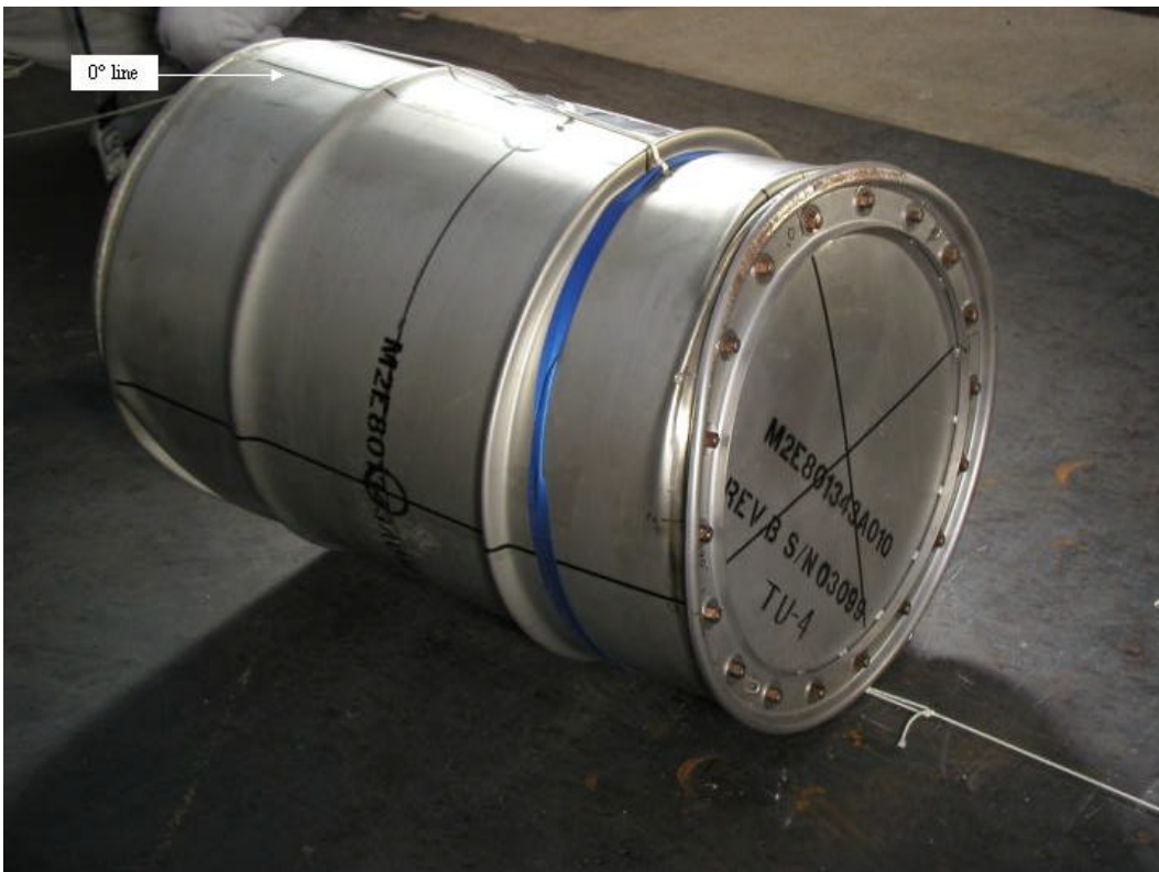
Figure H 21. Side view of TU-4 lid following the HAC crush test.
