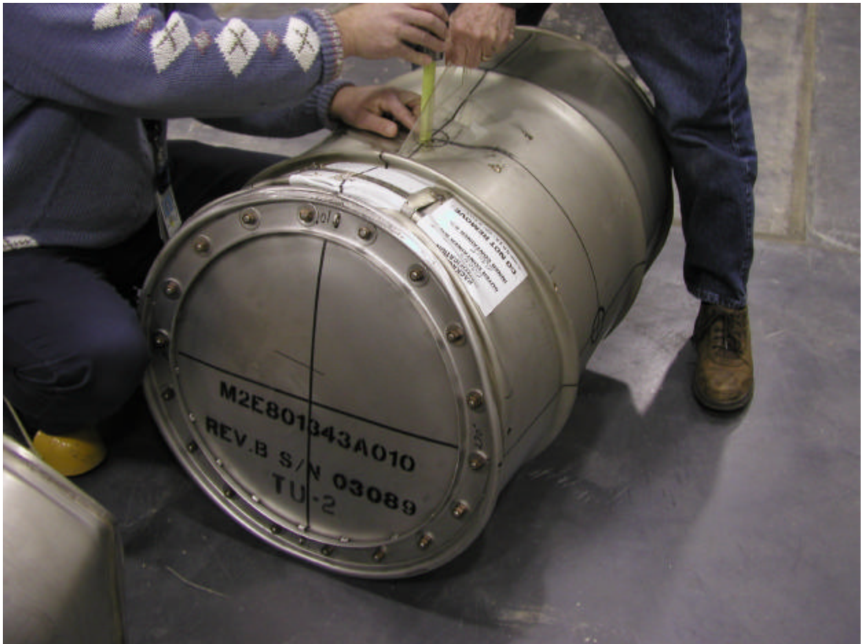
Figure 3-18 Measuring the indentation produced in the puncture test of TU-2.
