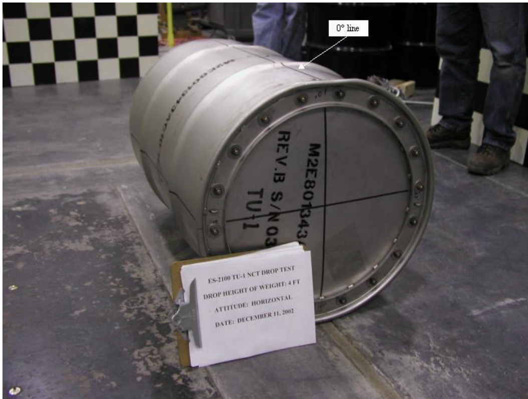
Figure E 11. Top end view of damage to TU-1 on the 0° line – package has been rolled 180°.
