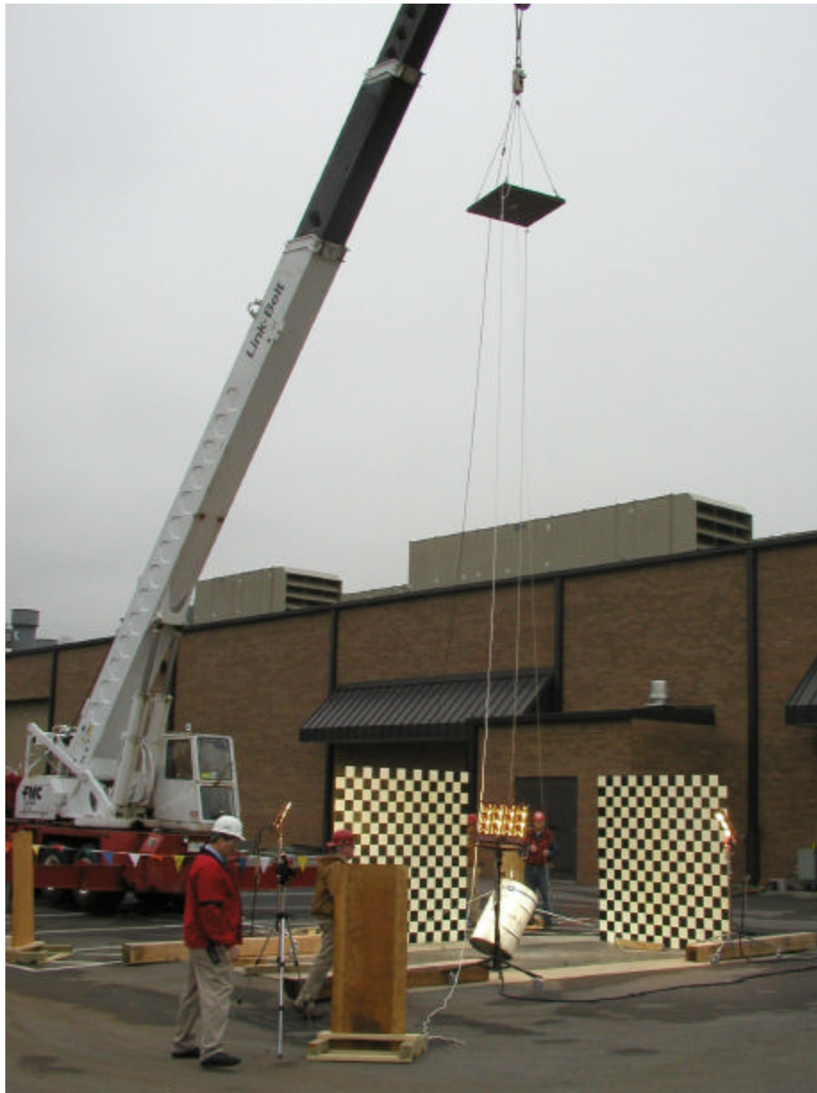
Figure 3-9 Test setup for the dynamic crush test of TU-2.
