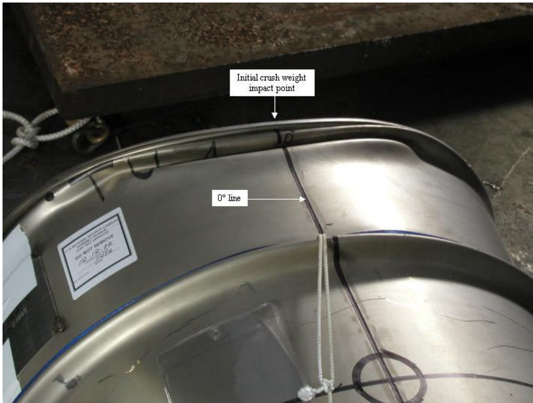
Figure H 22. Detail of top lid damage at the 0° line.
