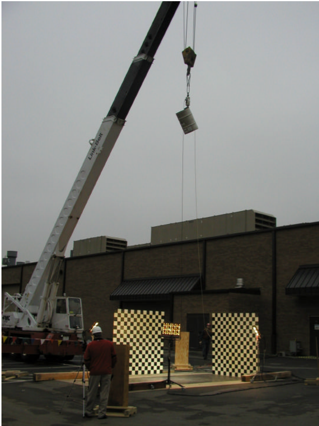
Figure 3-6 Photo showing the test setup for the HAC 9-m drop of TU-2.
