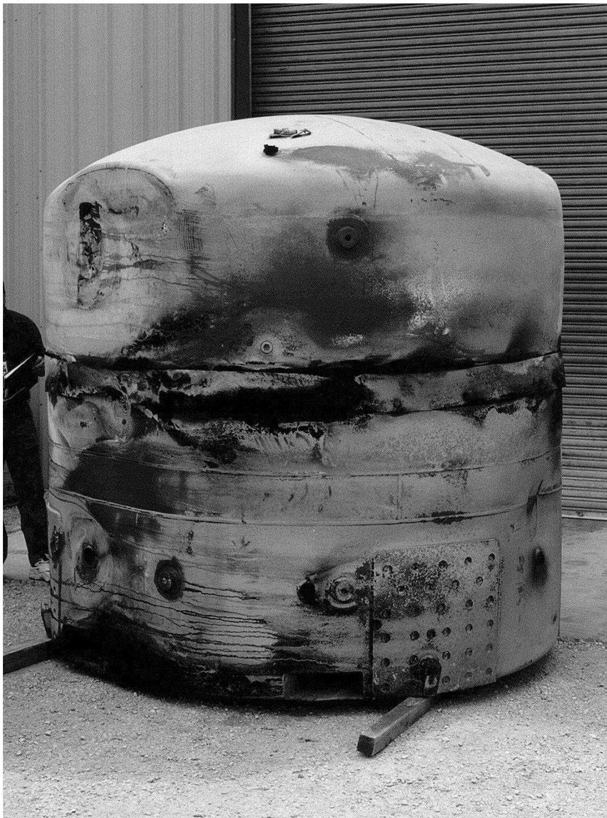
Figure 2.10.3-78 – CTU; View Before Disassembly (OCV Seal Test Port in Foreground)
