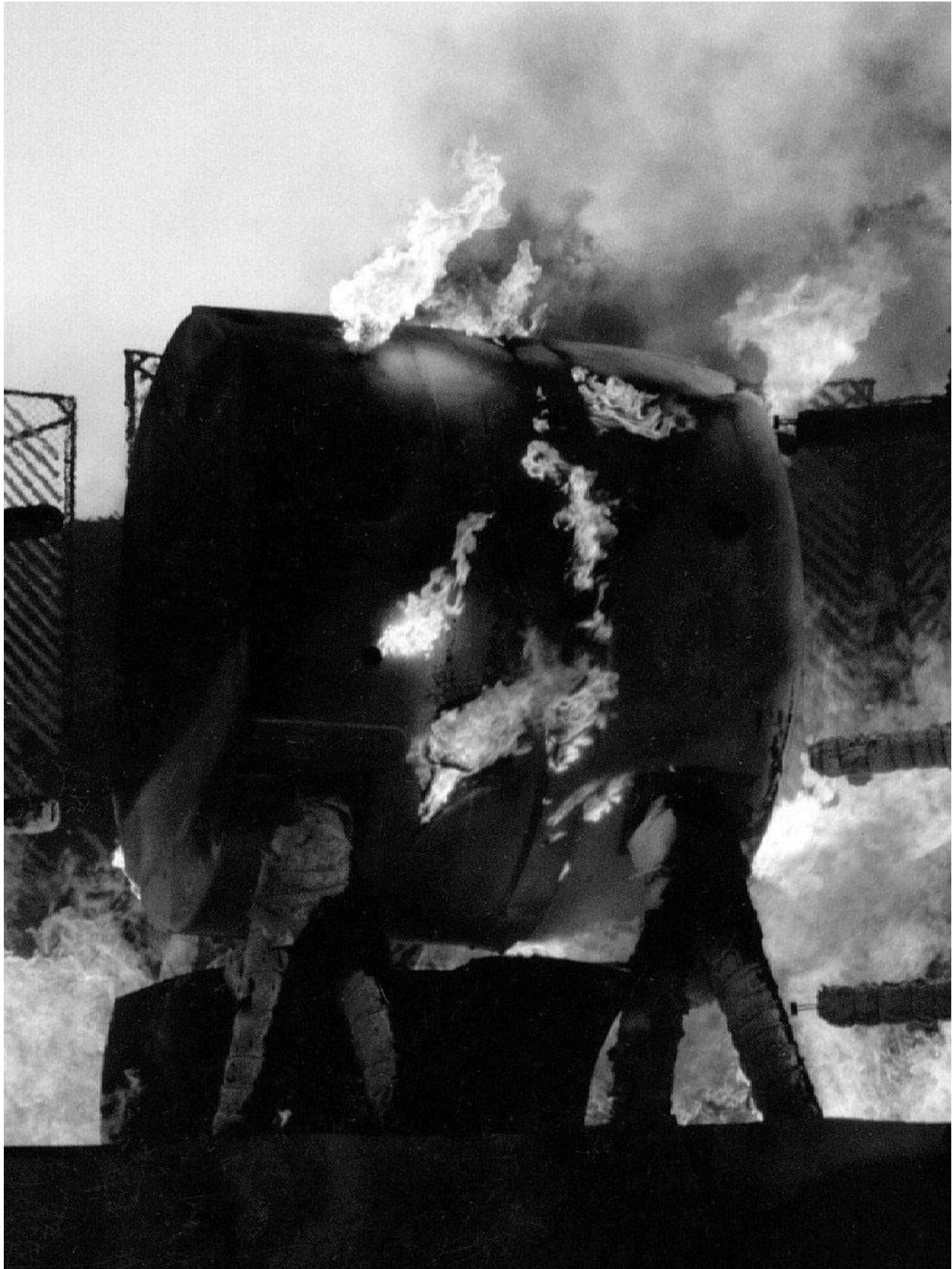
Figure 2.10.3-76 – CTU Fire Test 7; Side 2 View ~33 Minutes after Start (End of Fire)
