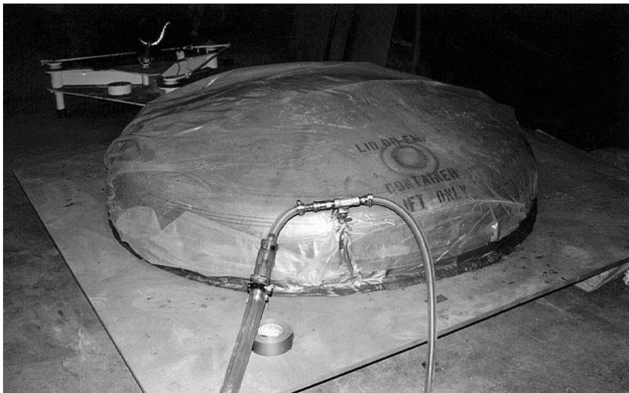
Figure 2.10.3-92 – CTU; Helium Leakage Rate Testing the ICV Lid Structure
