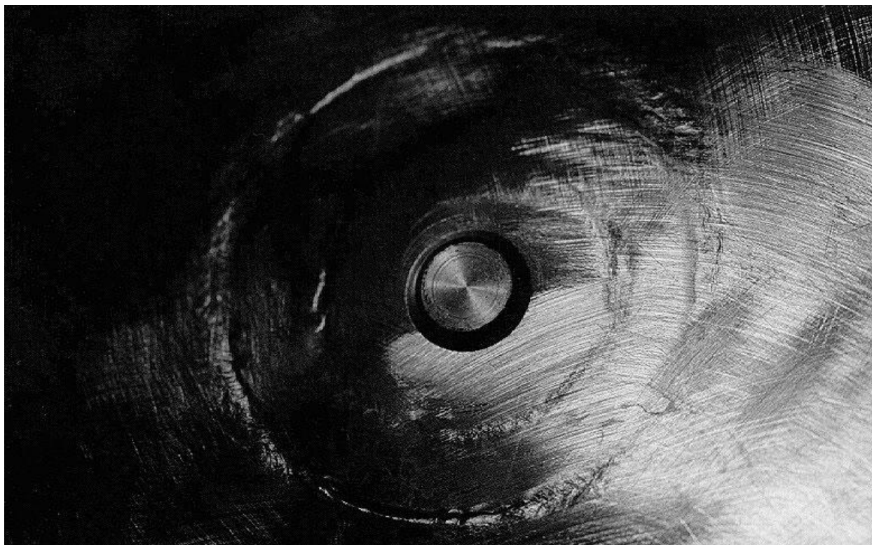
Figure 2.10.3-94 – CTU; Close-up View of Cracked OCV Vent Port Coupling Inner Weld
