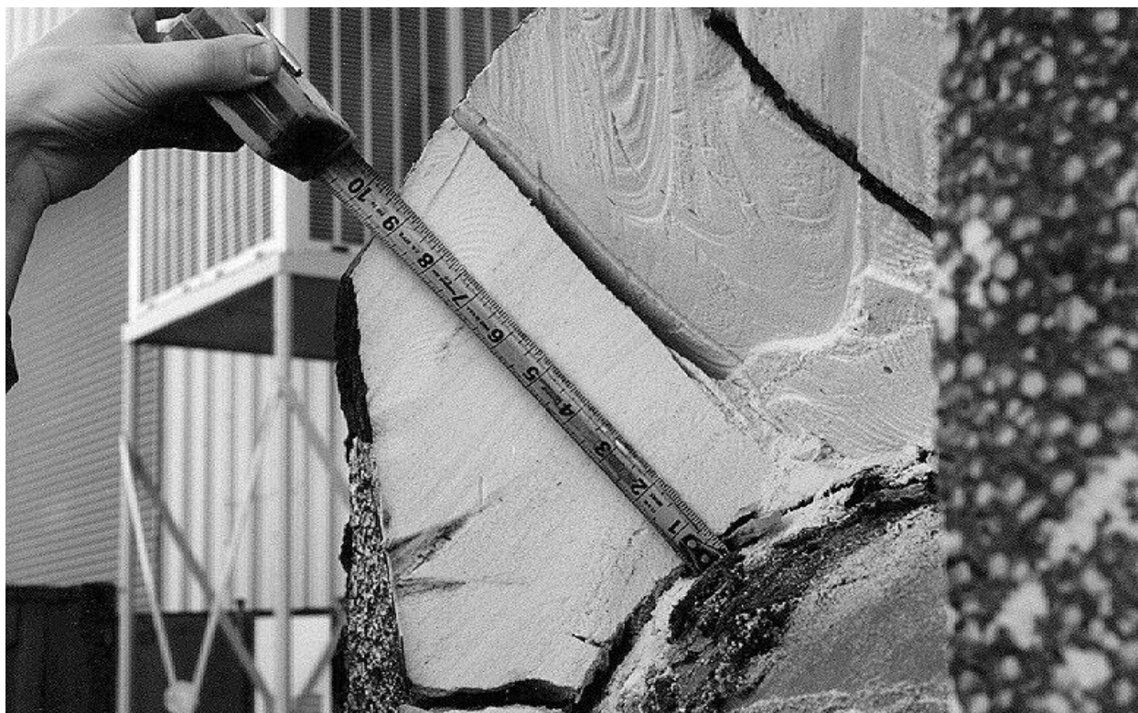
Figure 2.10.3-81 – CTU; Residual Foam in OCA Lid Knuckle; Aligned with Test 1, 2, & 4 Damage
