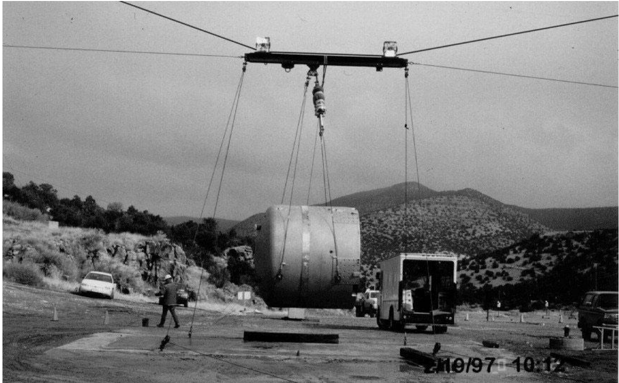
Figure 2.10.3-16 – ETU Free Drop Test 3; View Just Prior to NCT Free Drop Test
