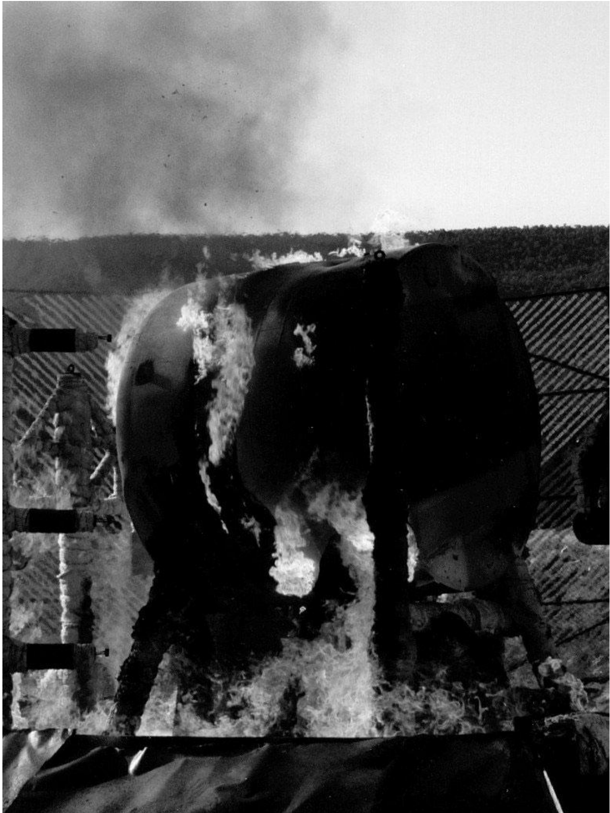
Figure 2.10.3-75 – CTU Fire Test 7; Side 1 View ~33 Minutes after Start (End of Fire)
