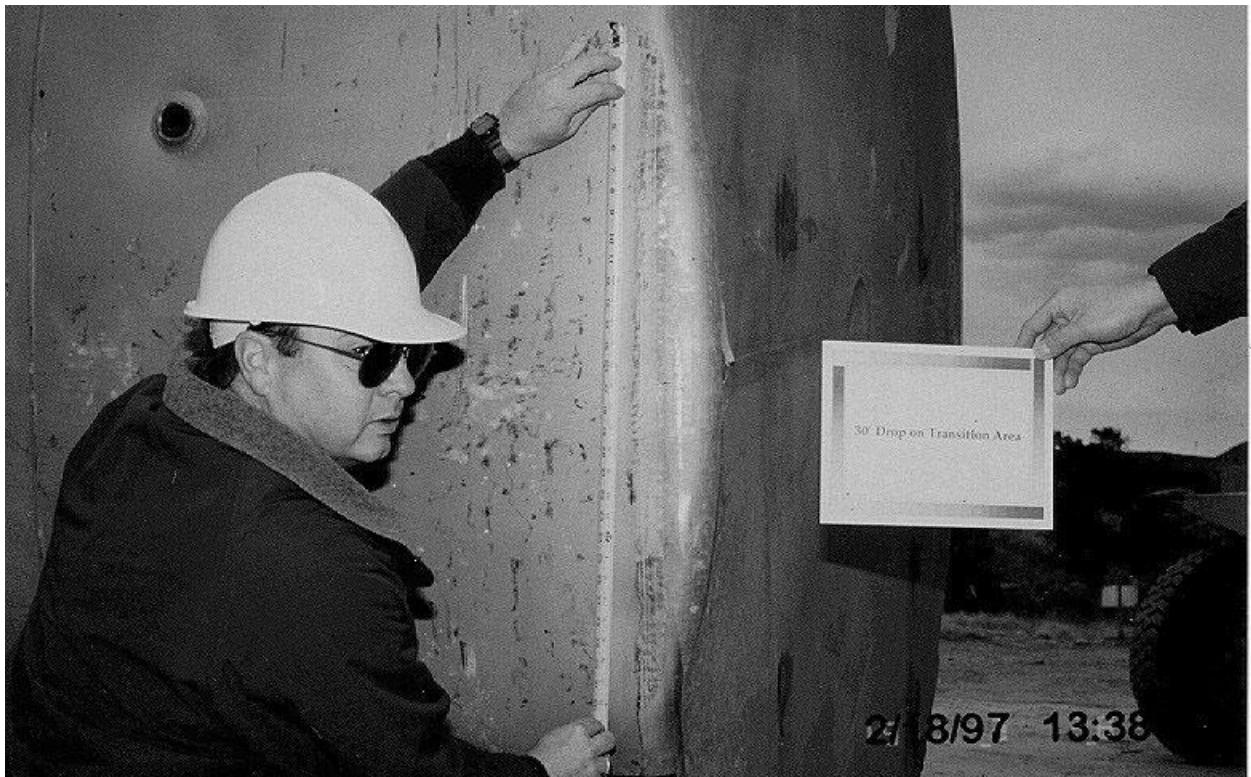
Figure 2.10.3-15 – ETU Free Drop Test 2; Bottom-End Damage; ~33" Wide Flat
