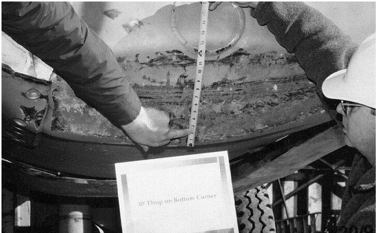
Figure 2.10.3-23 – ETU Free Drop Test 6; Bottom Corner Damage; ~12" Deep Flat
