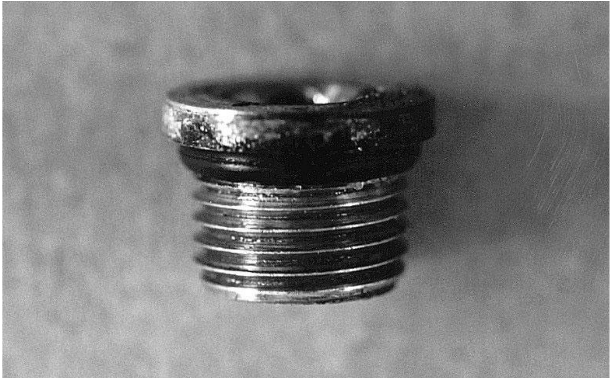
Figure 2.10.3-84 – CTU; Close-up of OCV Seal Test Port Plug (As Removed/Not Cleaned)
