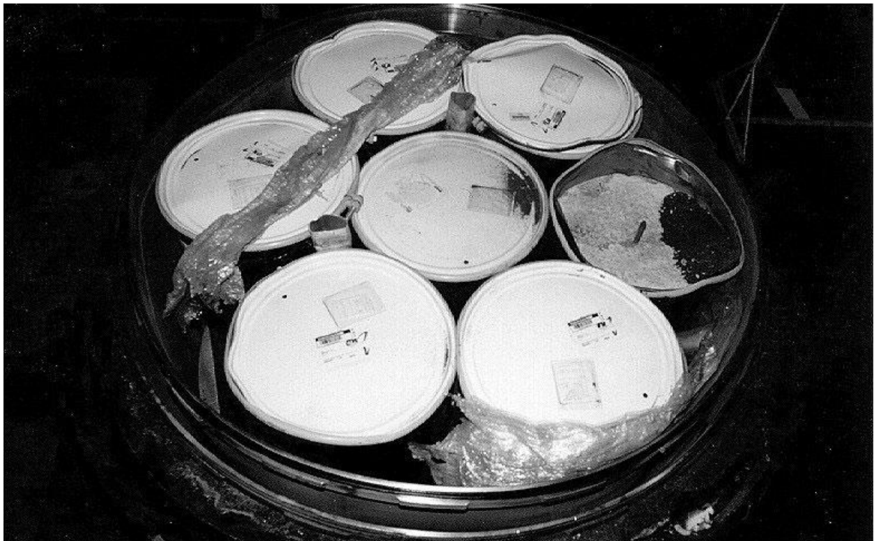
Figure 2.10.3-48 – ETU; View of 55-Gallon Payload Drums Following ICV Lid Removal
