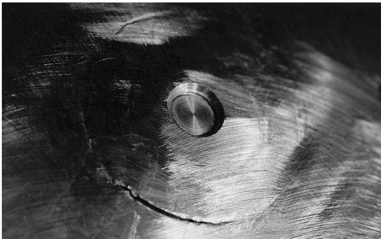
Figure 2.10.3-95 – CTU; Close-up View of Cracked OCV Vent Port Coupling Inner Weld
