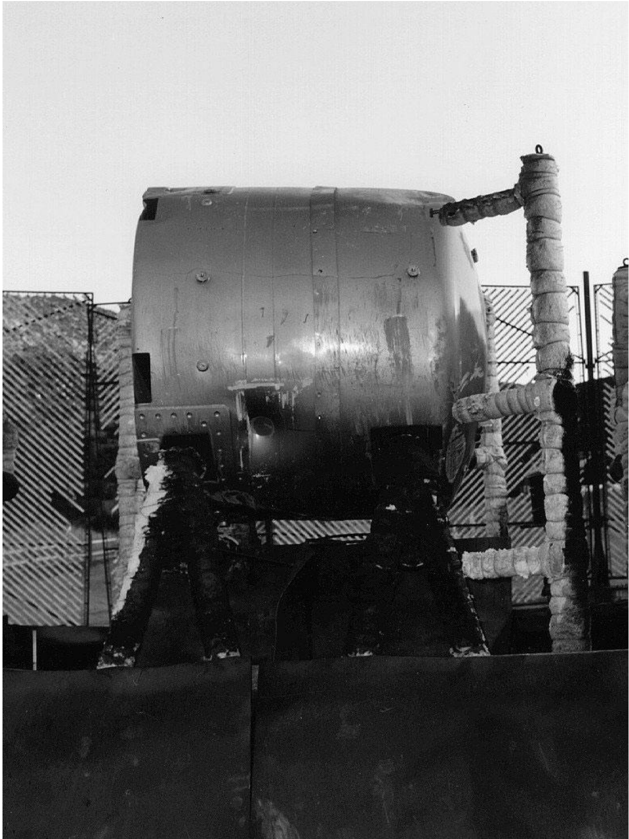
Figure 2.10.3-70 – CTU Fire Test 7; Side 2 View Before Fire Showing Test 5 Damage
