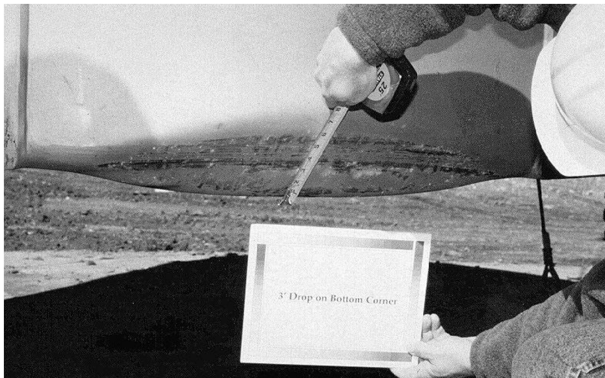
Figure 2.10.3-21 – ETU Free Drop Test 5; Bottom Corner Damage; ~5½" Deep Flat
