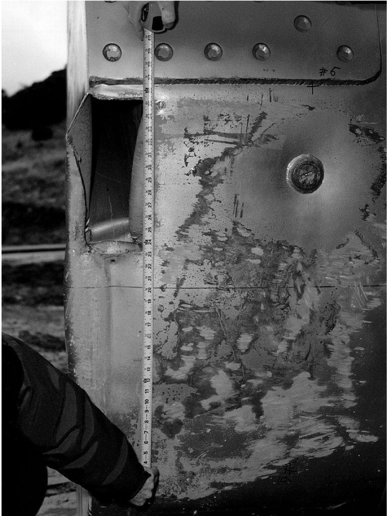
Figure 2.10.3-59 – CTU Free Drop Test 2; Bottom-End Damage; ~37" Wide Flat
