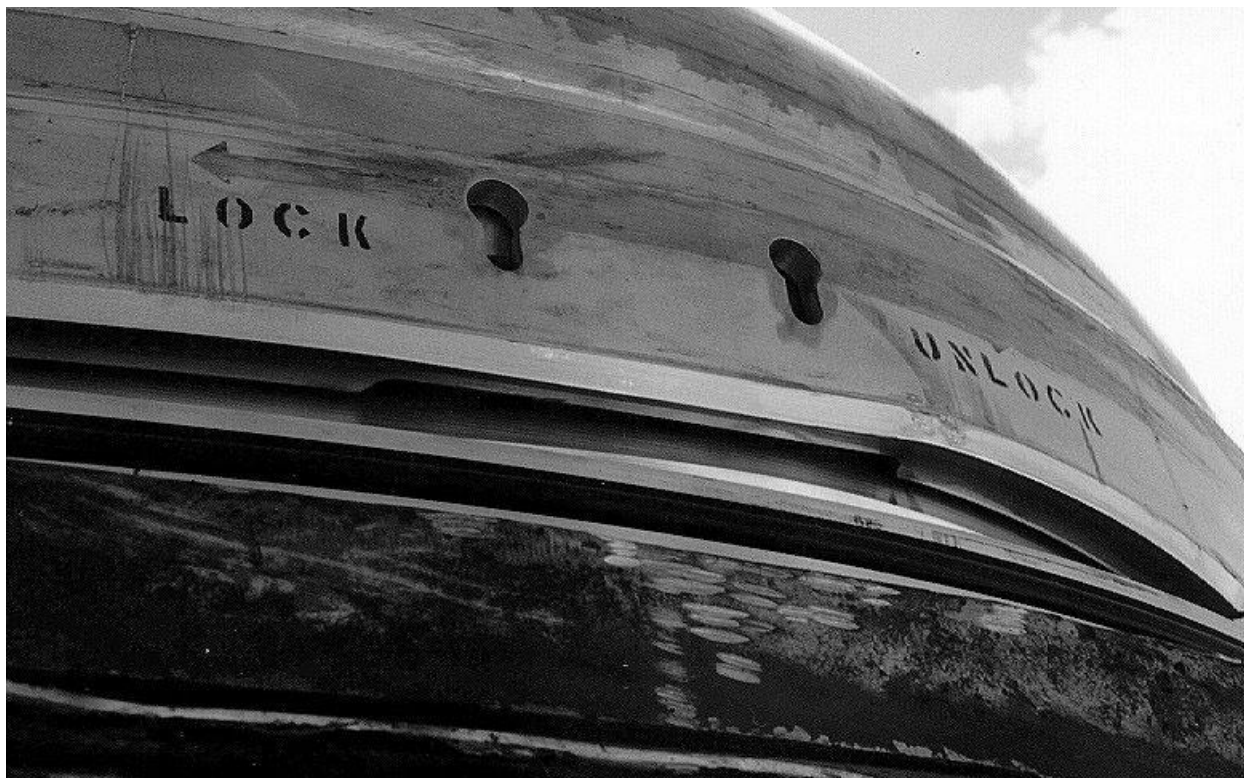
Figure 2.10.3-88 – CTU; Close-up of Damage to ICV Locking Ring
