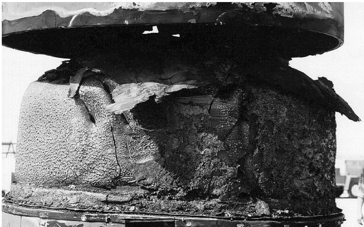
Figure 2.10.3-41 – ETU; Removal of the OCA Lid Outer Shell (Note Crumbling Foam Char)
