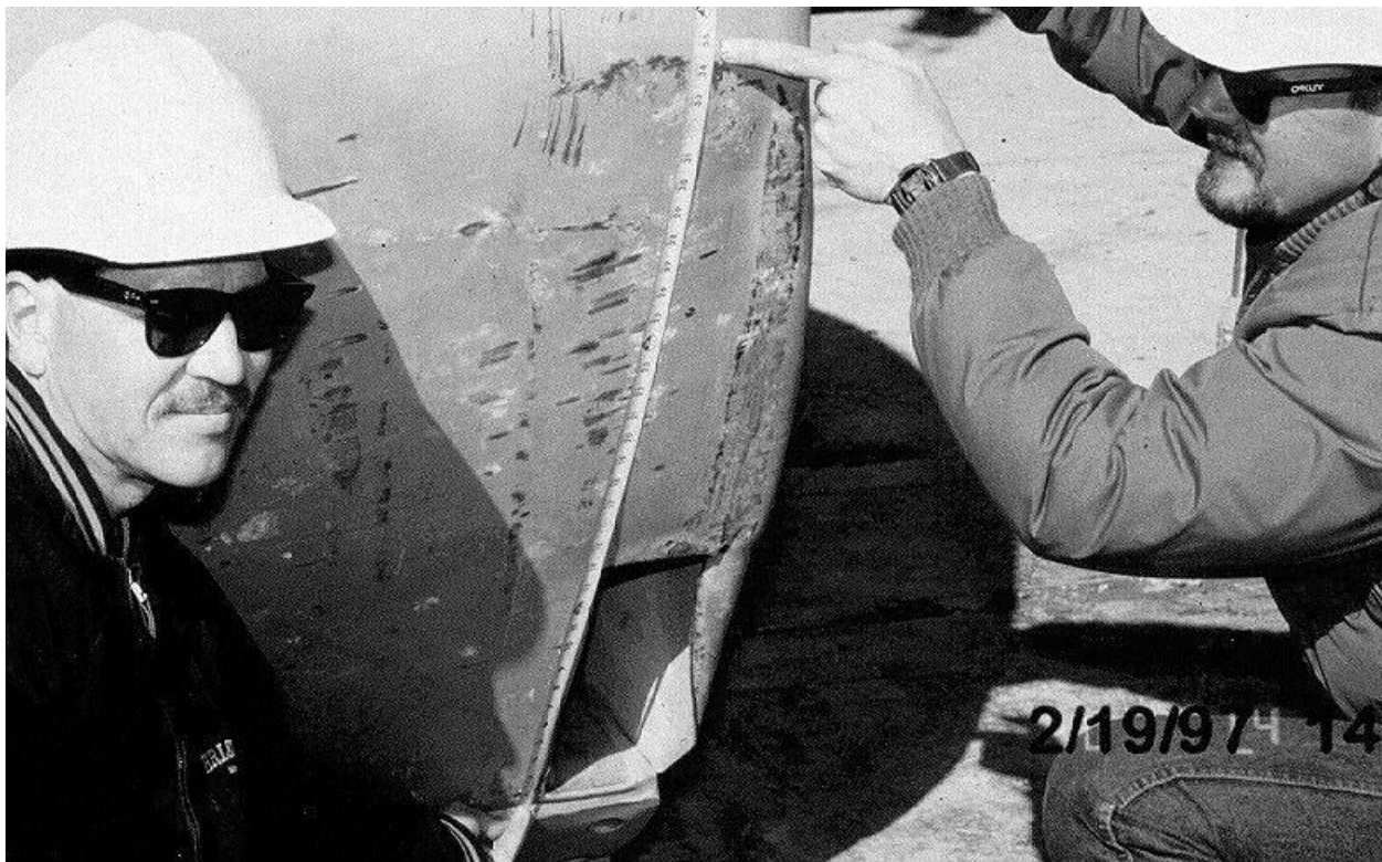
Figure 2.10.3-19 – ETU Free Drop Test 4; Bottom-End Damage; ~34" Wide Flat
