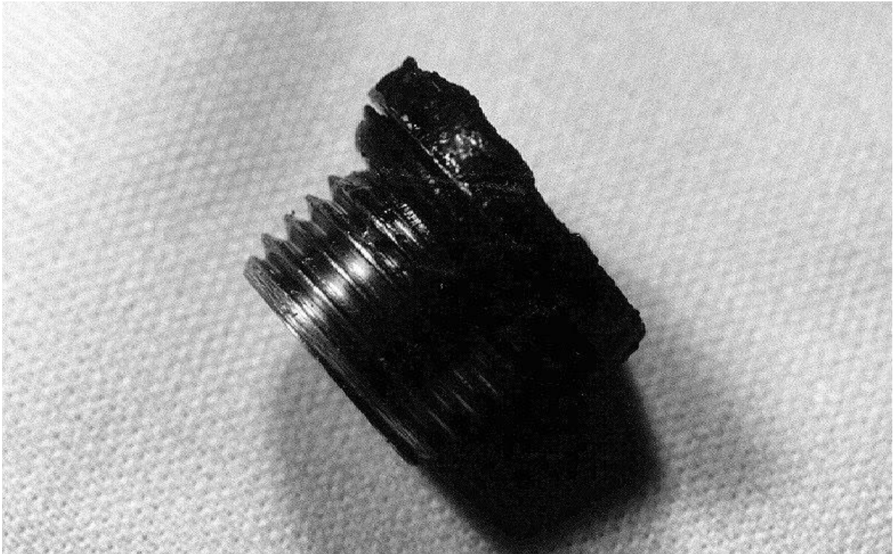
Figure 2.10.3-45 – ETU; View of OCV Seal Test Port Plug (As Removed; Not Cleaned)
