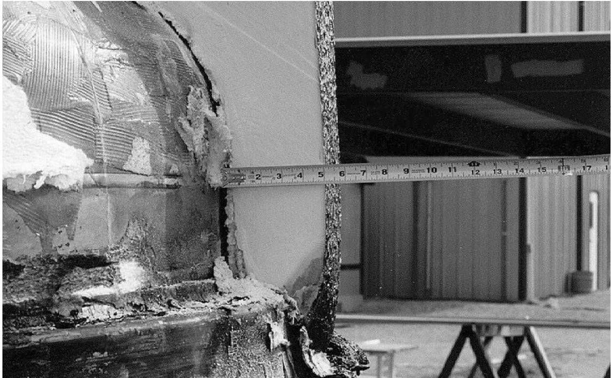
Figure 2.10.3-43 – ETU; Residual Foam in OCA Lid Side; Remote From Test Damage
