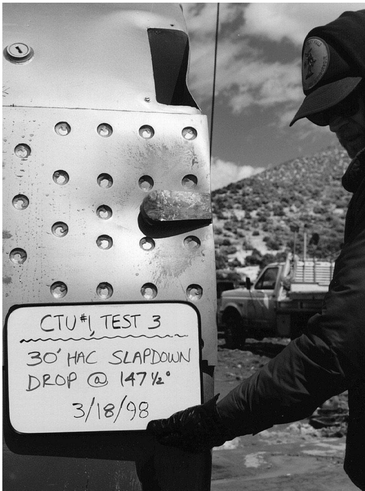
Figure 2.10.3-61 – CTU Free Drop Test 3; Bottom-End Damage
