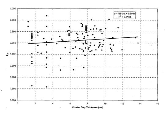
Figure 6.A.5.3-8 k<sub>eff</sub> versus <sup>10</sup>B Plate Loading
