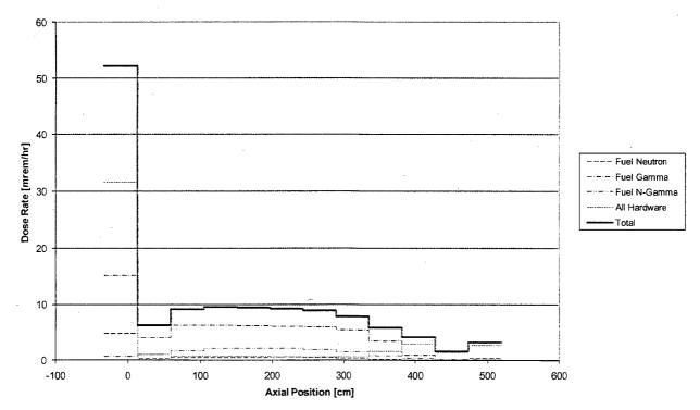
Figure 5.A.7.3-11 Concrete Cask Top Dose Rate Profiles
