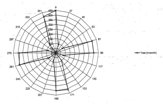
Figure 5.A.6-5 Transfer Cask Radial Dose Rate Profiles
