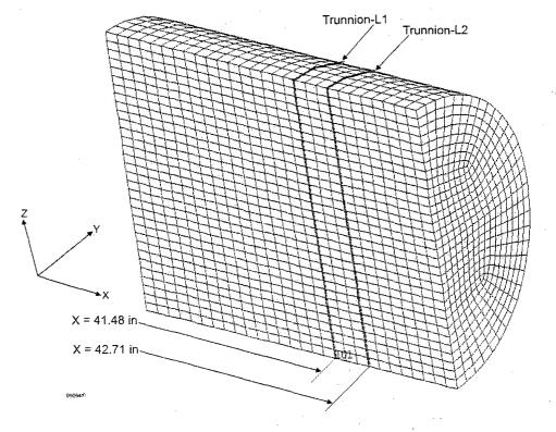
Figure 3.A.4.3.3-3 Retaining Block ANSYS Model for Evaluation of Inadvertent Canister Lift
