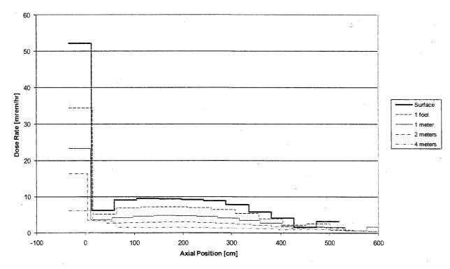
Figure 5.A.7.3-10 Concrete Cask Side Surface Dose Rate Profile by Source
