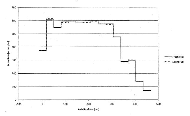
Figure 5.A.7.2-9 Comparison of Response Method to Direct Solution: Concrete Cask Radial Surface – 45 GWd/MTU, 4.1 wt % <sup>235</sup>U
