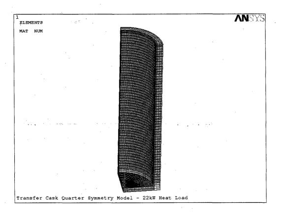
Figure 4.A.4.1.2-3 Modeling Details of the Quarter-Symmetry Transfer Cask Model
