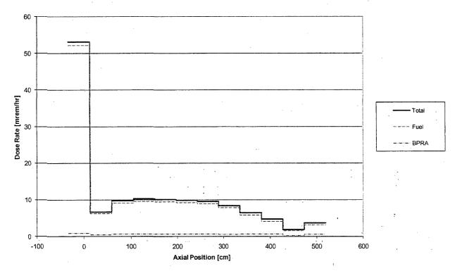
Figure 5.A.7.4-2 Thimble Plug Concrete Cask Radial Surface Dose Rate Profile
