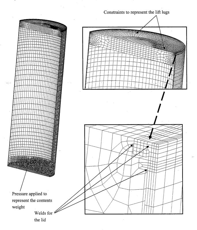
Figure 3.A.4-2 Base Weldment Finite Element Model
