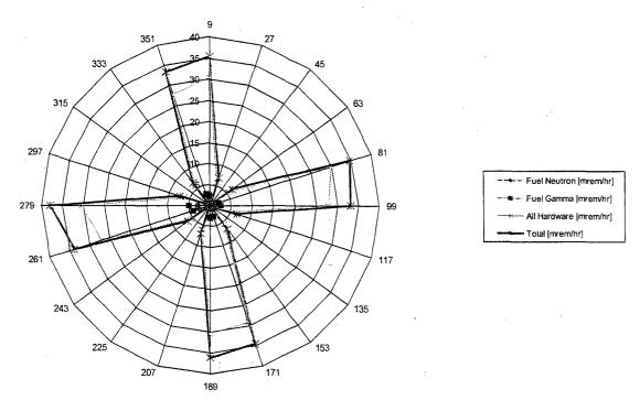
Figure 5.A.7.3-14 Concrete Cask Air Inlet Elevation Dose Rate Profile
