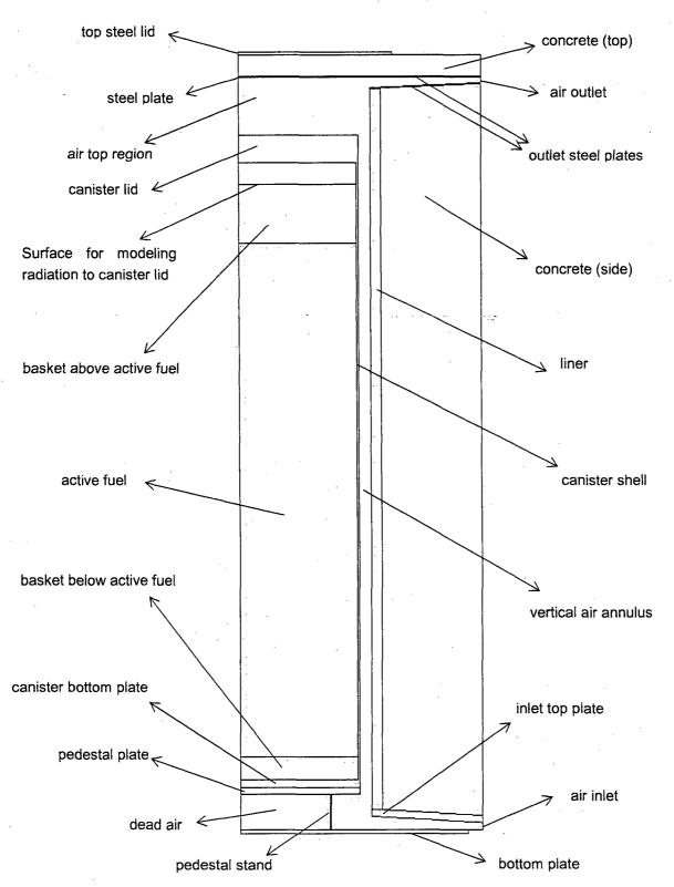
Figure 4.A.4.1.1-2 FLUENT Computational Fluid Dynamics Model for UNITAD Storage System (Canister and Concrete Cask)
