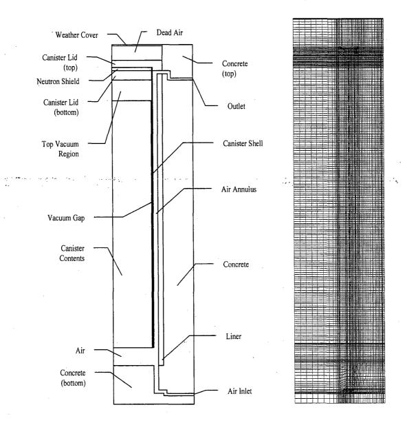
Figure 4.A.4.8-2 ANSYS Model for Effective Properties Calculation
