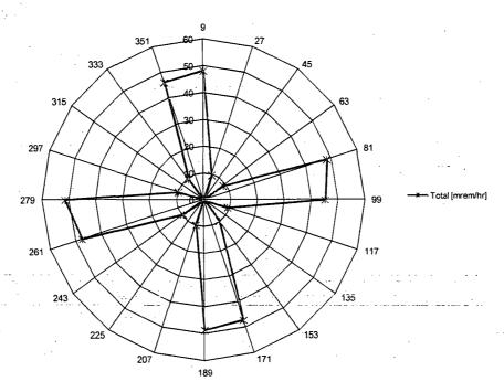
Figure 5.A.6-4 Air Inlet Elevation Surface Dose Rate Profile
