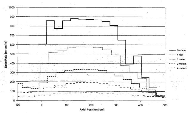
Figure 5.A.6-6 Transfer Cask Top Axial Dose Rate Profiles
