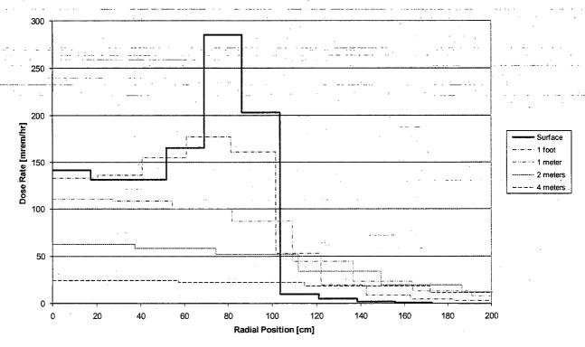
Figure 5.A.6-3 Air Outlet Elevation Surface Dose Rate Profile
