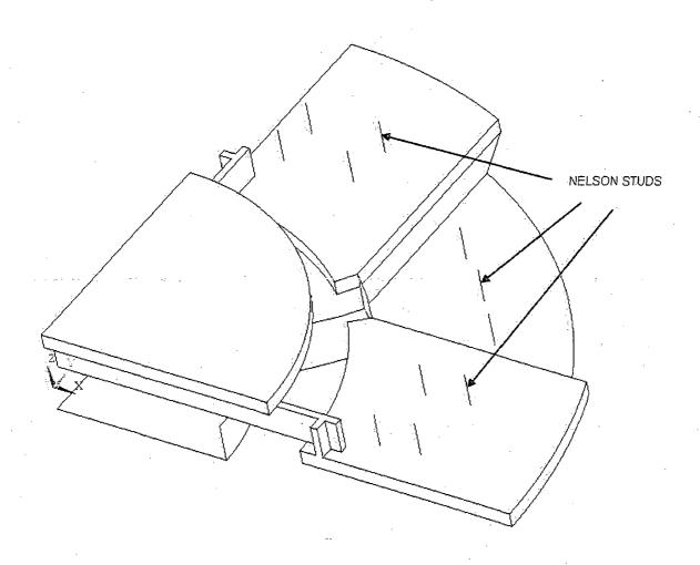
Figure 3-A.4-4 Gap Elements, View 1 – Base Weldment Finite Element Model
