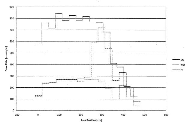
Figure 5.A.7.8-1 Canister Flood Study – Radial Surface Dose Rate Profile <sup>a</sup>
