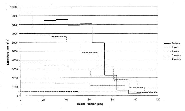
Figure 5.A.7.3-8 Transfer Cask Bottom Surface Dose Rate Profile by Source
