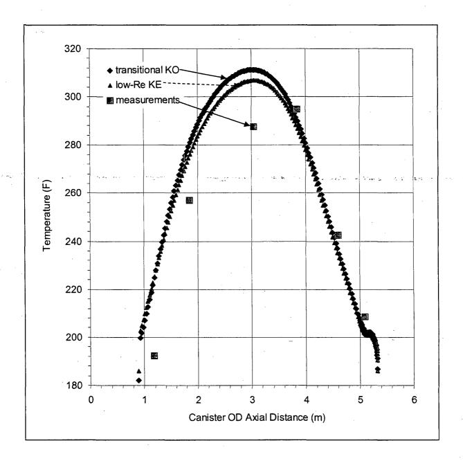
Figure 4.A.4.8-4 Temperature Profiles for the Concrete Liner Surface
