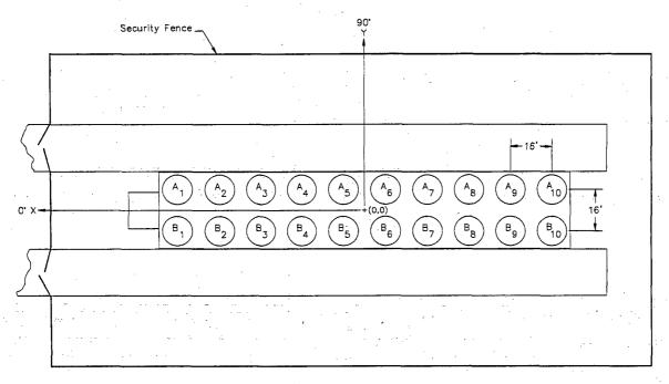
Note: A pitch of 16 ft is conservative when considering array self-shielding.
