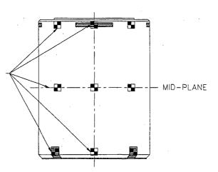
Figure A 3-2 CONCRETE CASK Surface Dose Rate Measurement for UNITAD STORAGE SYSTEM
