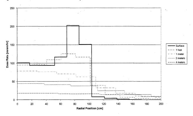
Figure 5.A.7.3-12 Concrete Cask Top Surface Dose Rate Profile by Source
