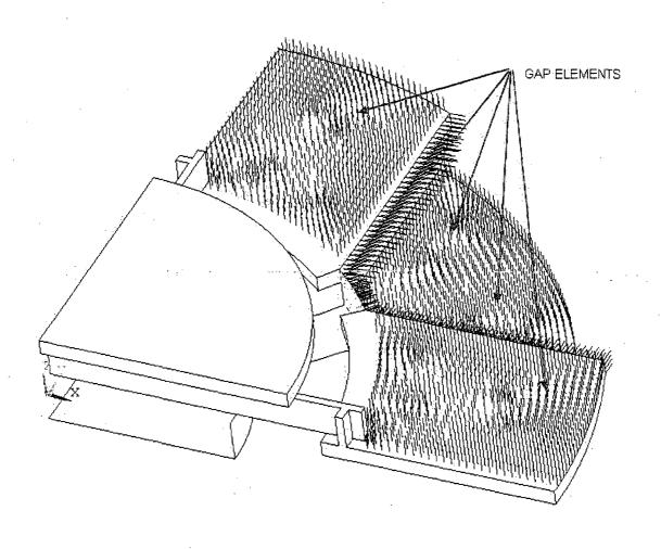
Figure 3.A.4-5 Gap Elements, View 2 – Base Weldment Finite Element Model
