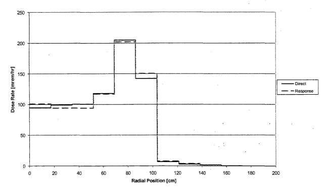
Figure 5.A.7.2-5 Comparison of Response Method to Direct Solution: Transfer Cask Radial Surface – Bounding Source Term
