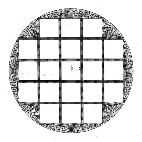
Figure 3.A.5-4 Basket Support Disk Sections for Stress Evaluations
