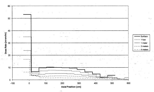
Figure 5.A.6-2 Concrete Cask Top Axial Dose Rate Profiles
