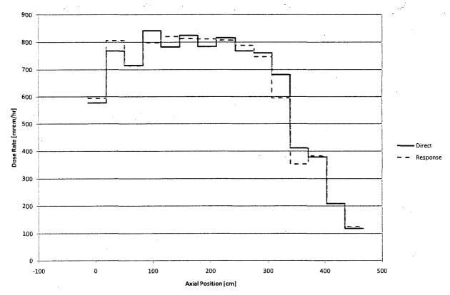
Figure 5.A.7.2-6 Comparison of Response Method to Direct Solution: Transfer Cask Top Surface – Bounding Source Term
