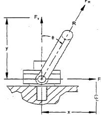
A maximum sling angle ( $\theta$ ) of 30° corresponds to a minimum sling length (R) of:
