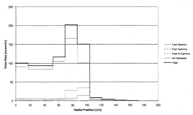
Figure 5.A.7.3-13 Concrete Cask Air Outlet Elevation Dose Rate Profile
