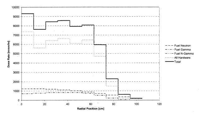
Figure 5.A.7.3-9 Concrete Cask Side Dose Rate Profiles
