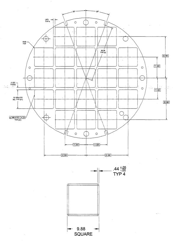
Figure 6.A.3-2 UNITAD Canister
