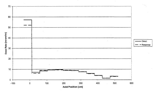
Figure 5.A.7.2-4 Comparison of Response Method to Direct Solution: Concrete Cask Top Surface – Bounding Source Term
