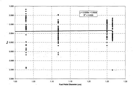
Figure 6.A.5.3-4 k<sub>eff</sub> versus Fuel Rod Outside Diameter
