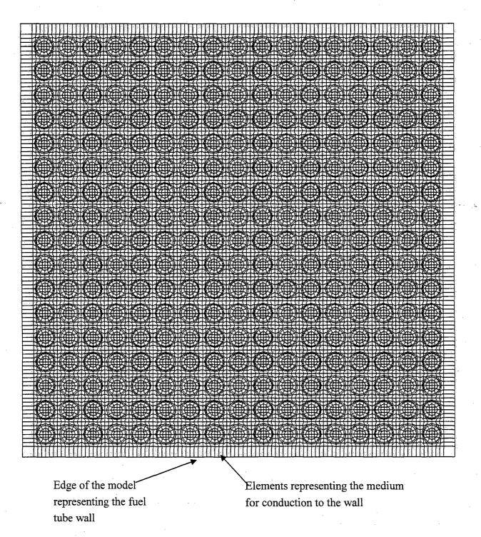
Figure 4.A.4.1.4-2 Pin and Pellet Fuel Model
