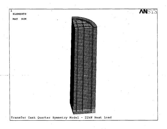
Figure 4.A.4.1.2-2 Model of the Transfer Cask
