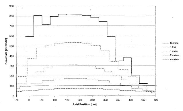
Figure 5.A.7.3-4 Transfer Cask Side Surface Dose Rate Profile by Source
