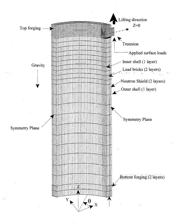
Figure 3.A.4.3.3-2 Definition of Stress Cross-Sections on the Top Ring
