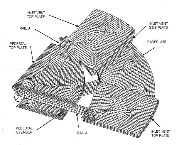
Table 3.A.4-3 Nelson Studs – Base Weldment Finite Element Model
