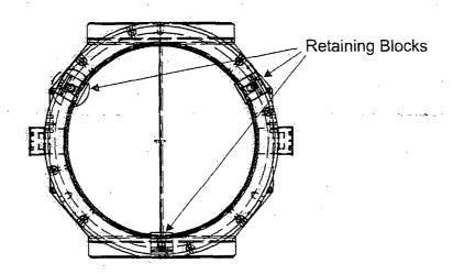
An inadvertent lift of the transfer cask by the Canister is an ASME Service Level C condition. The allowable stresses based on ASME Code, Section III for the Service Level C condition is used in this analysis. The temperature of the cask at the top is less than 200°F. A temperature of 200°F is assumed for allowable stress limits.
