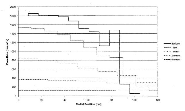
Figure 5.A.7.3-6 Transfer Cask Top Surface Dose Rate Profile by Source
