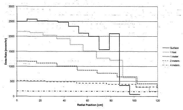
Figure 5.A.6-7 Transfer Cask Bottom Axial Dose Rate Profiles
