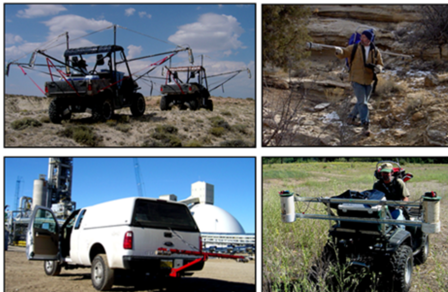
Figure 2: 3-detector OHV systems (top left); 2-detector backpack system (top right); 2- or 3-detector truck system (bottom left); 2-detector ATV system (bottom right).
