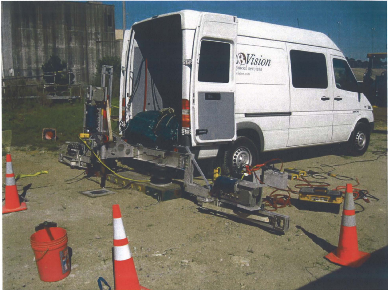
Figure 2: Downhole P- and S_H -wave energy source (Triple Whammy)
