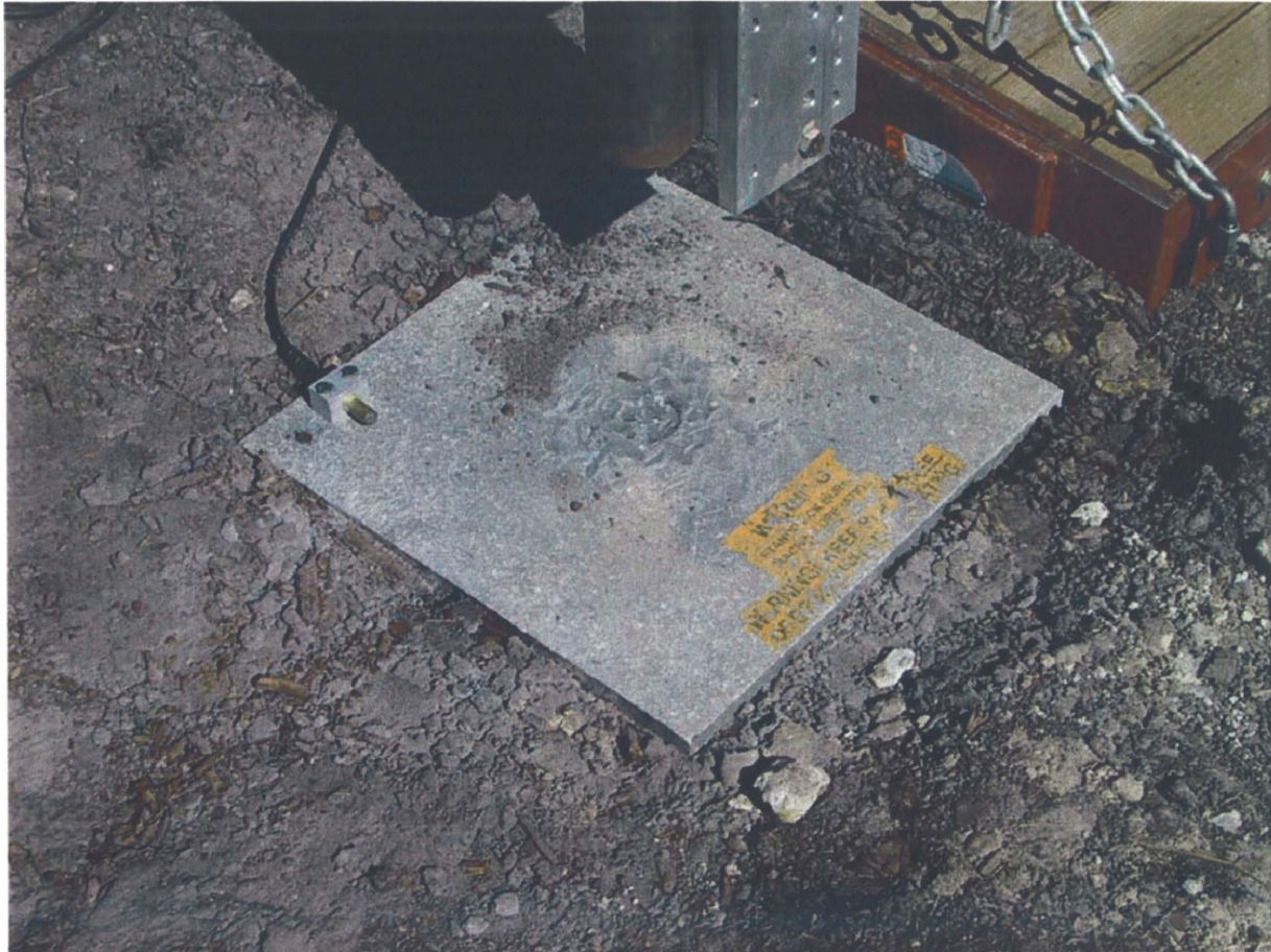
Figure 3: Downhole P-wave striking plate with hammer switch
