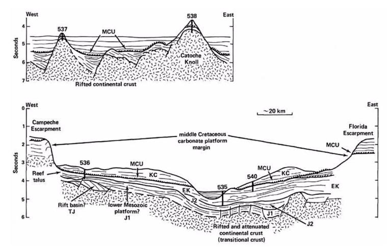
Notes: Schematic cross section for DSDP Leg 77 drill sites (Sites 535-538 and 540). MCU is the mid-Cretaceous unconformity. TJ, J1, J2, EK, and KC are seismic units described in Subsection 2.5.1.1.2.1.1.
