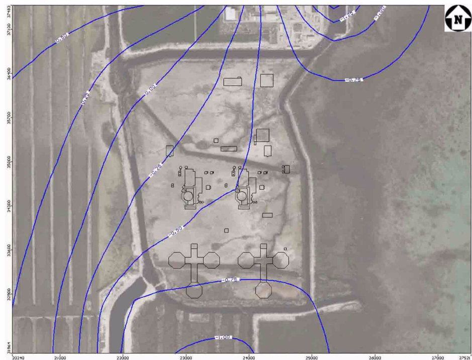
Figure 2CC-240 Post-Construction Groundwater Contours in Key Largo Limestone — Plan
