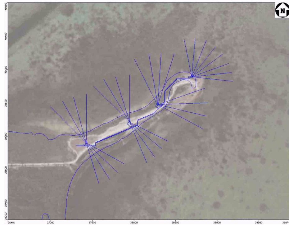
Figure 2CC-231 Location of Radial Collector Wells and Laterals
