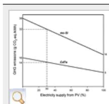
Figure 6. Greenhouse gas emissions profile for PV modules when using a PV breeder that supplies electricity for PV production. Insolation of 1700 kWh/m<sup>2</sup>/yr, performance ratio of 0.8, and lifetime of 30 yrs are assumed. BOS is not included. In 2005, the total (100%) electricity corresponded to 250 kWh/m<sup>2</sup> for mc-Si and 59 kWh/m<sup>2</sup> for CdTe PV.
